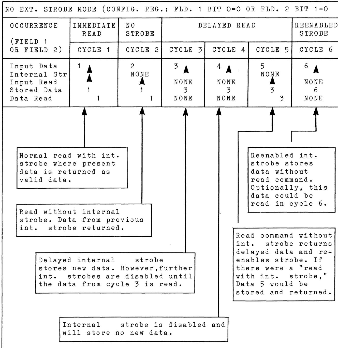
Figure 12-4. Non-External Strobe Mode Operation
