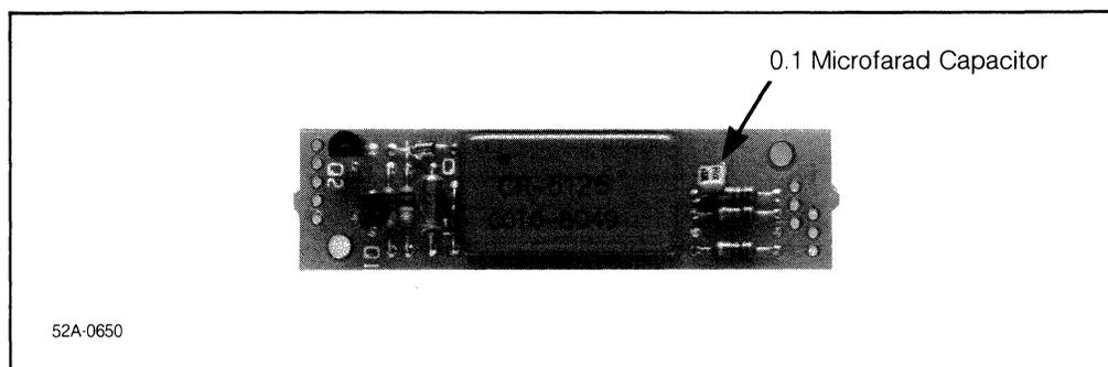
Figure 7-4. Modification to Relay Module (refer to text)
