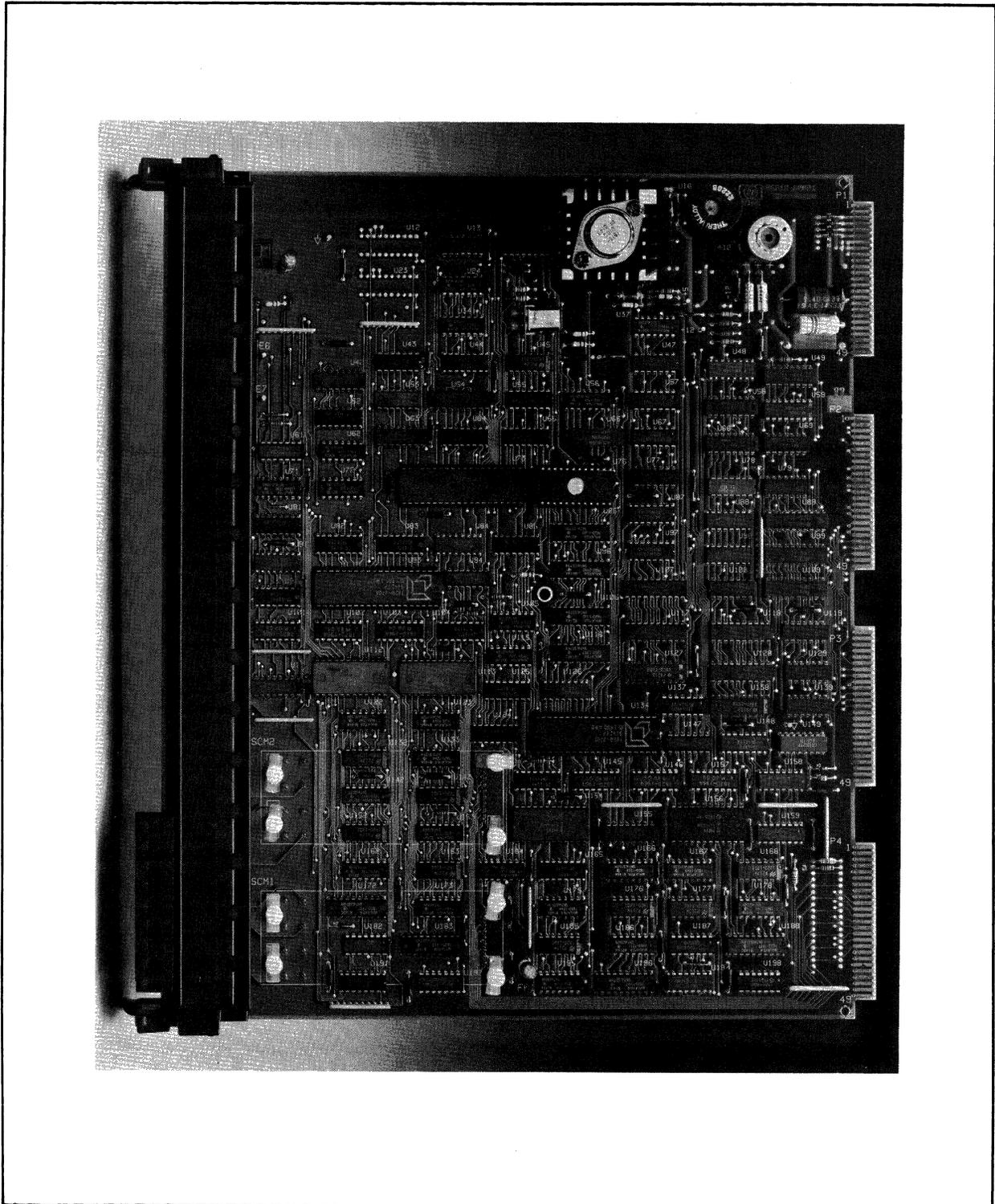
Figure 15-1. HP 25512 Counter Input Card
