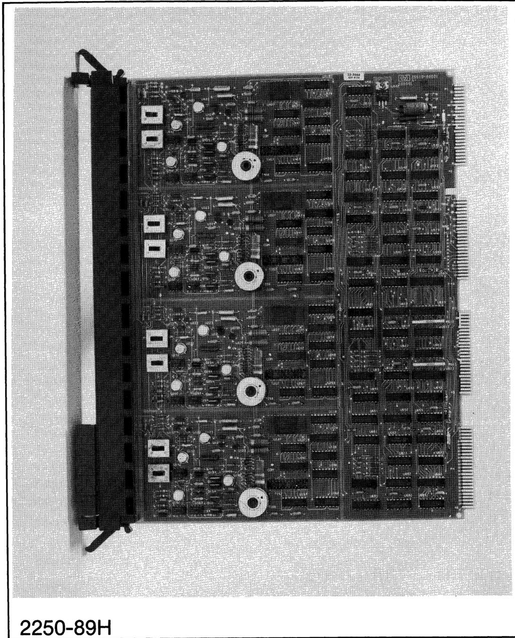
Figure 8-1. HP 25510A 4-Channel Voltage/Current Analog Output
