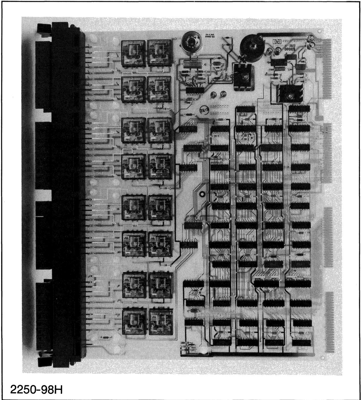
Figure 11-1. HP 25514A 16-Point Relay Output
