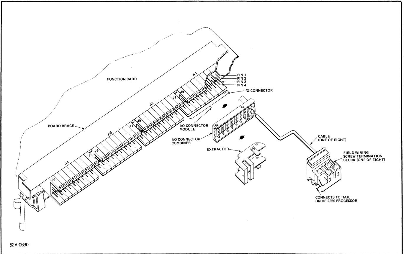
Figure 3-11. Connector Modules and Cable Assembly
