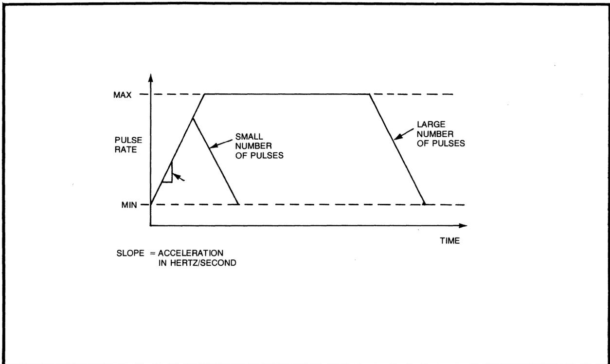
Figure 7-2: Pulse Rate vs. Time Profile in Pulse Generation Mode
