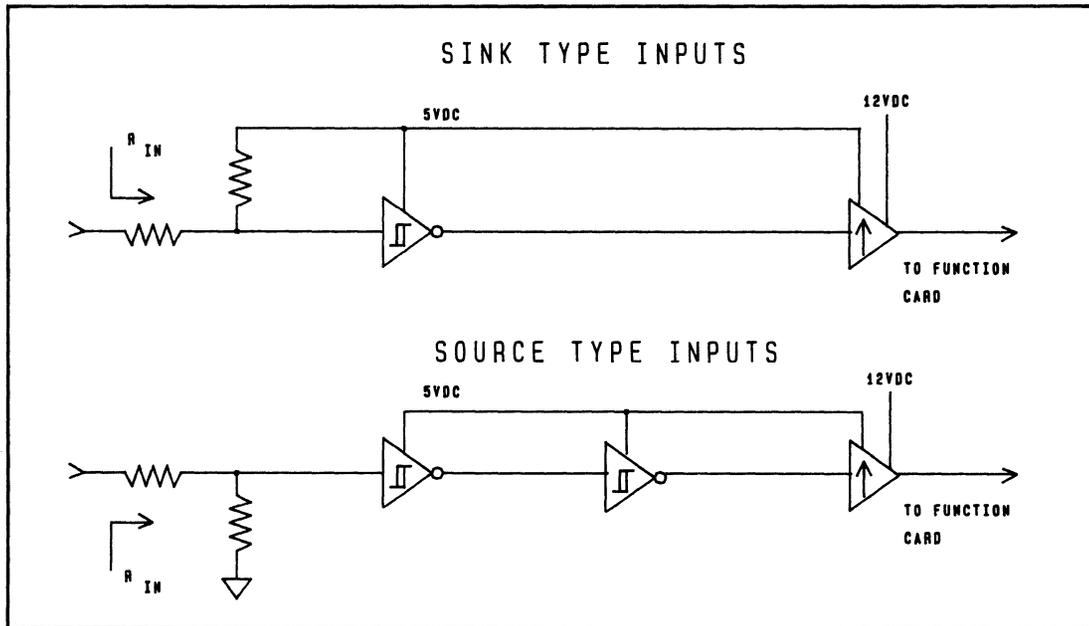
Figure 14-19. HP 25536 Schematic Diagram
