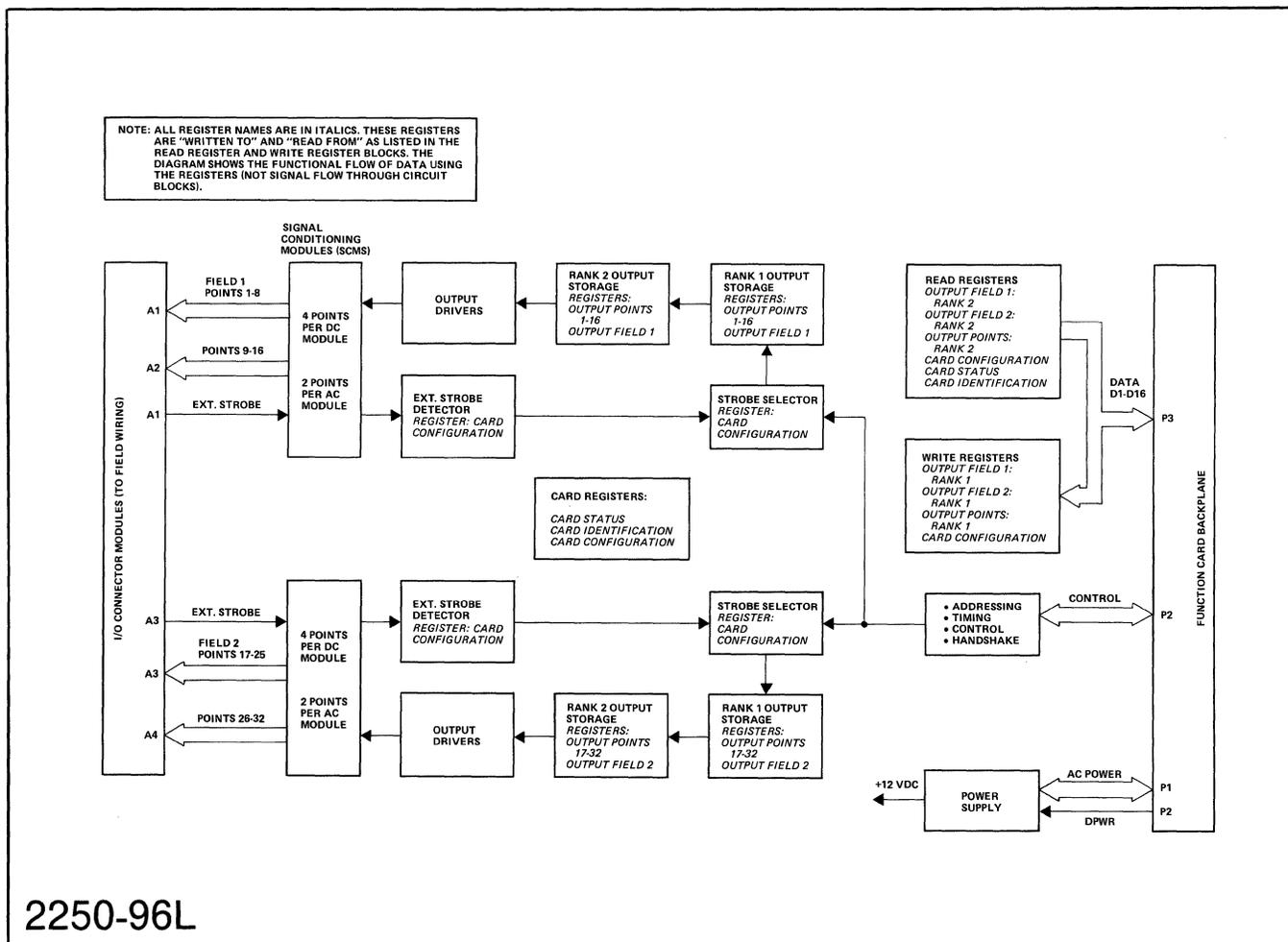
Figure 10-2. HP 25513A Functional Block Diagram
