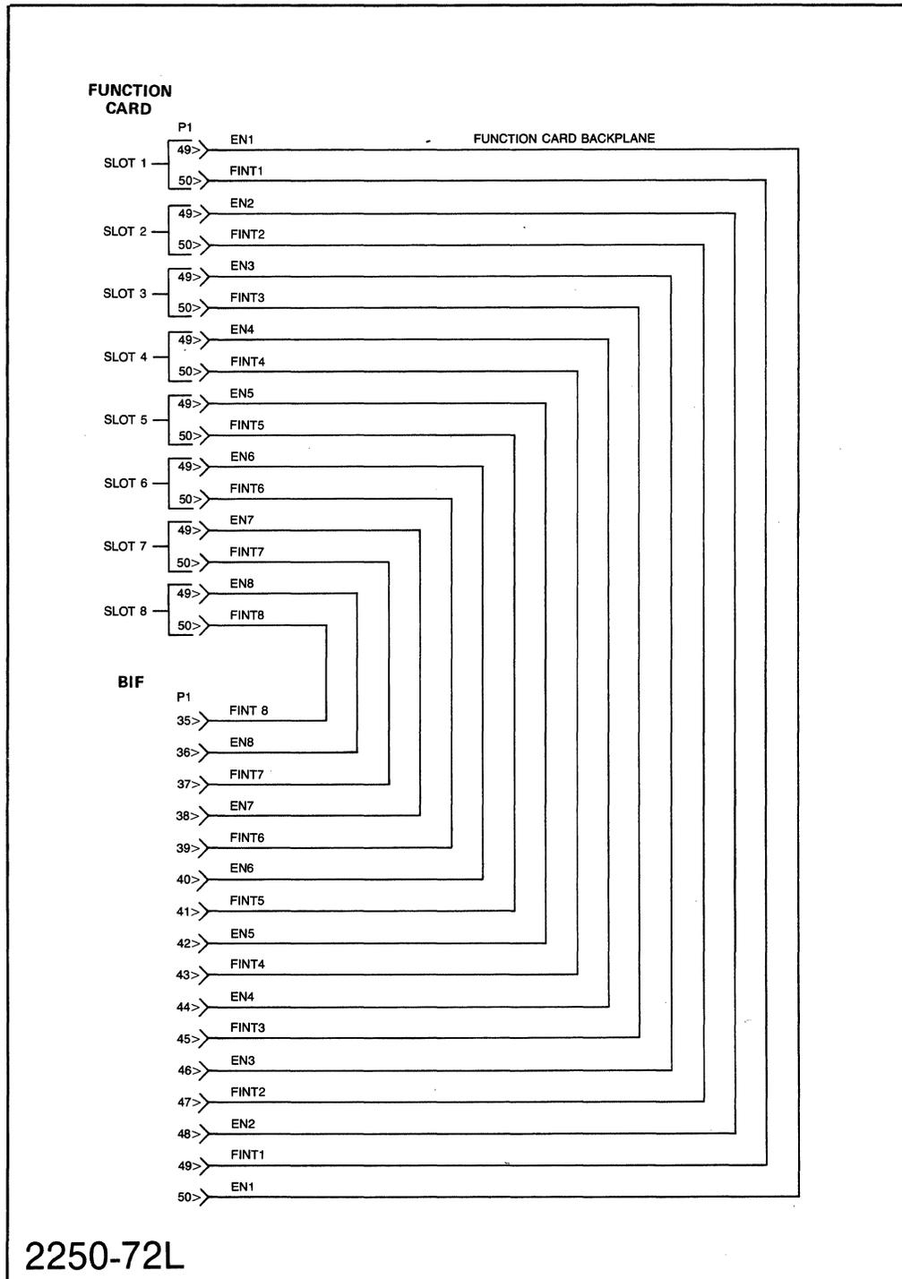
Figure 3-8. Distribution of Enable and Interrupt Lines
