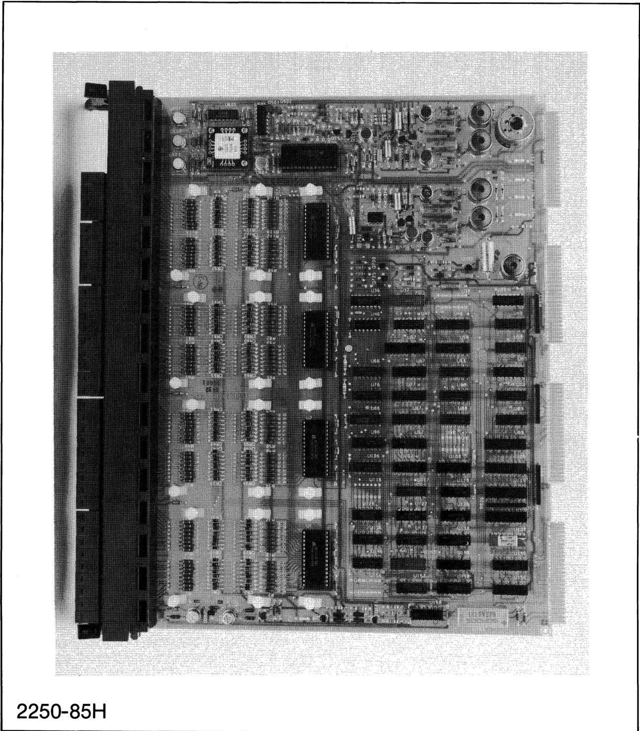
Figure 6-1. HP 25503A 32-Channel Low-Level Multiplexer
