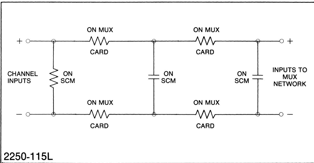
Figure 14-9. HP 25540 Schematic Diagram
