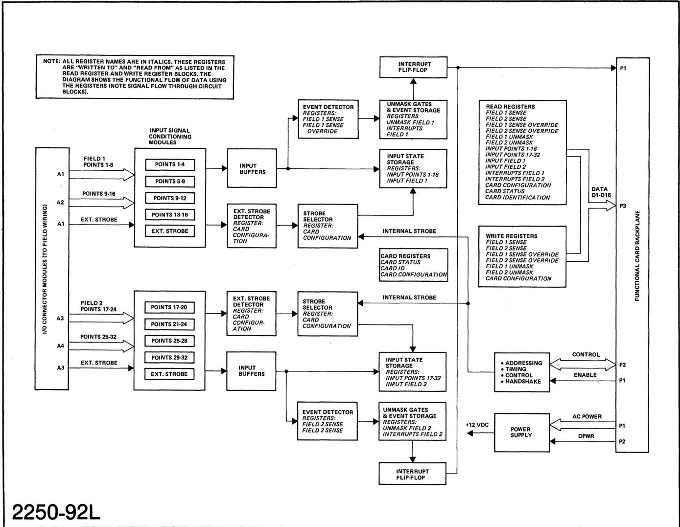
Figure 9-2. HP 25511A Functional Block Diagram
