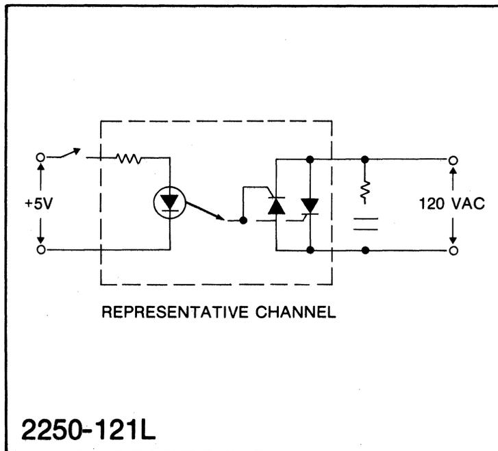
Figure 14-15. HP 25545A Schematic Diagram
