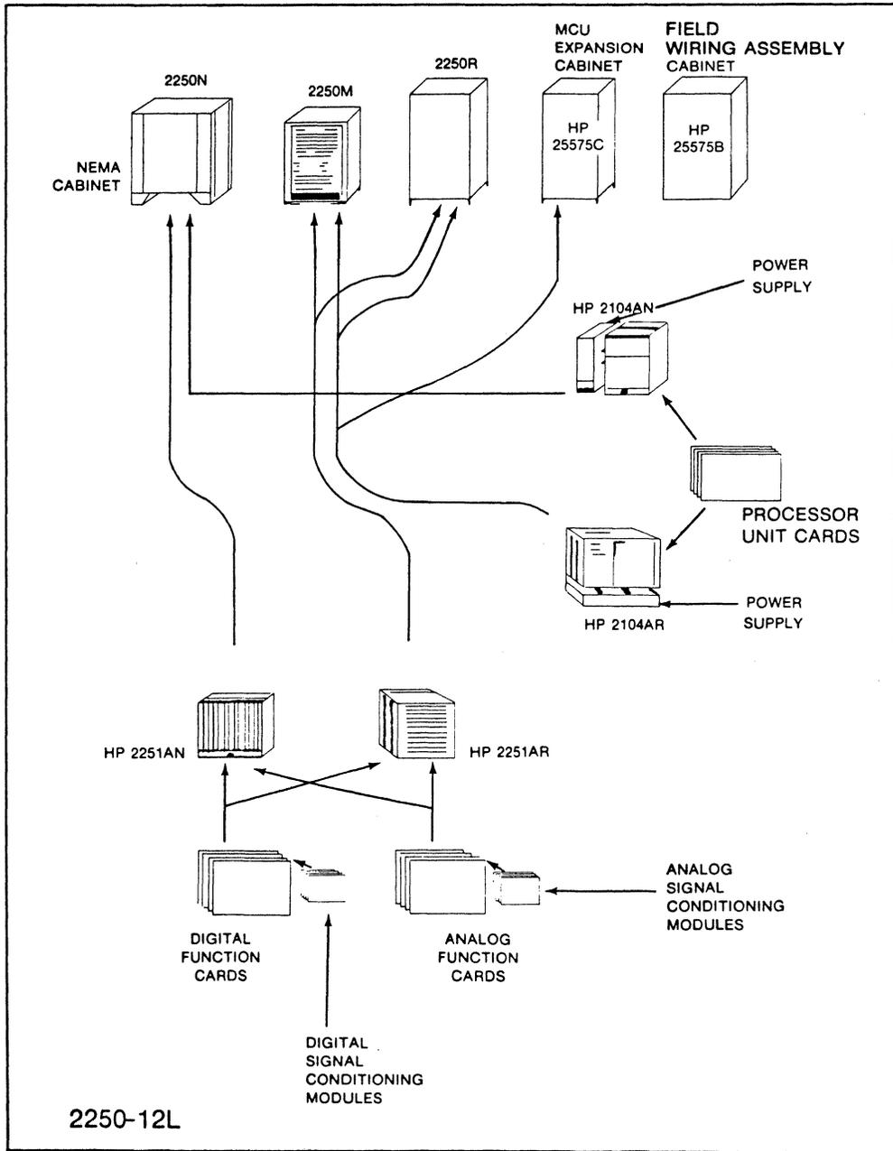
Figure 1-1. HP 2250 Measurement and Control Processor Components
