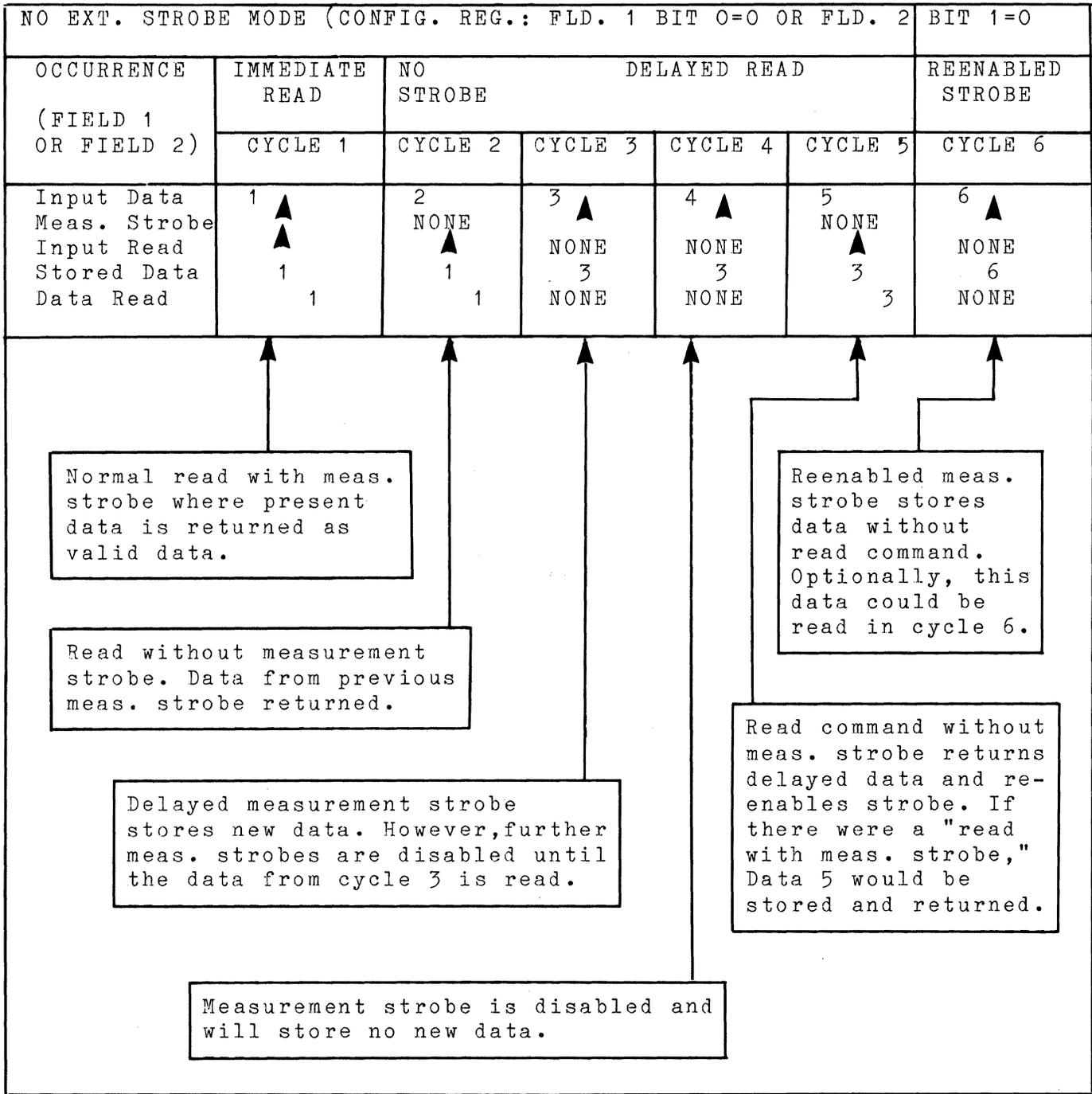
Figure 9-3. Non-External Strobe Mode Operation
