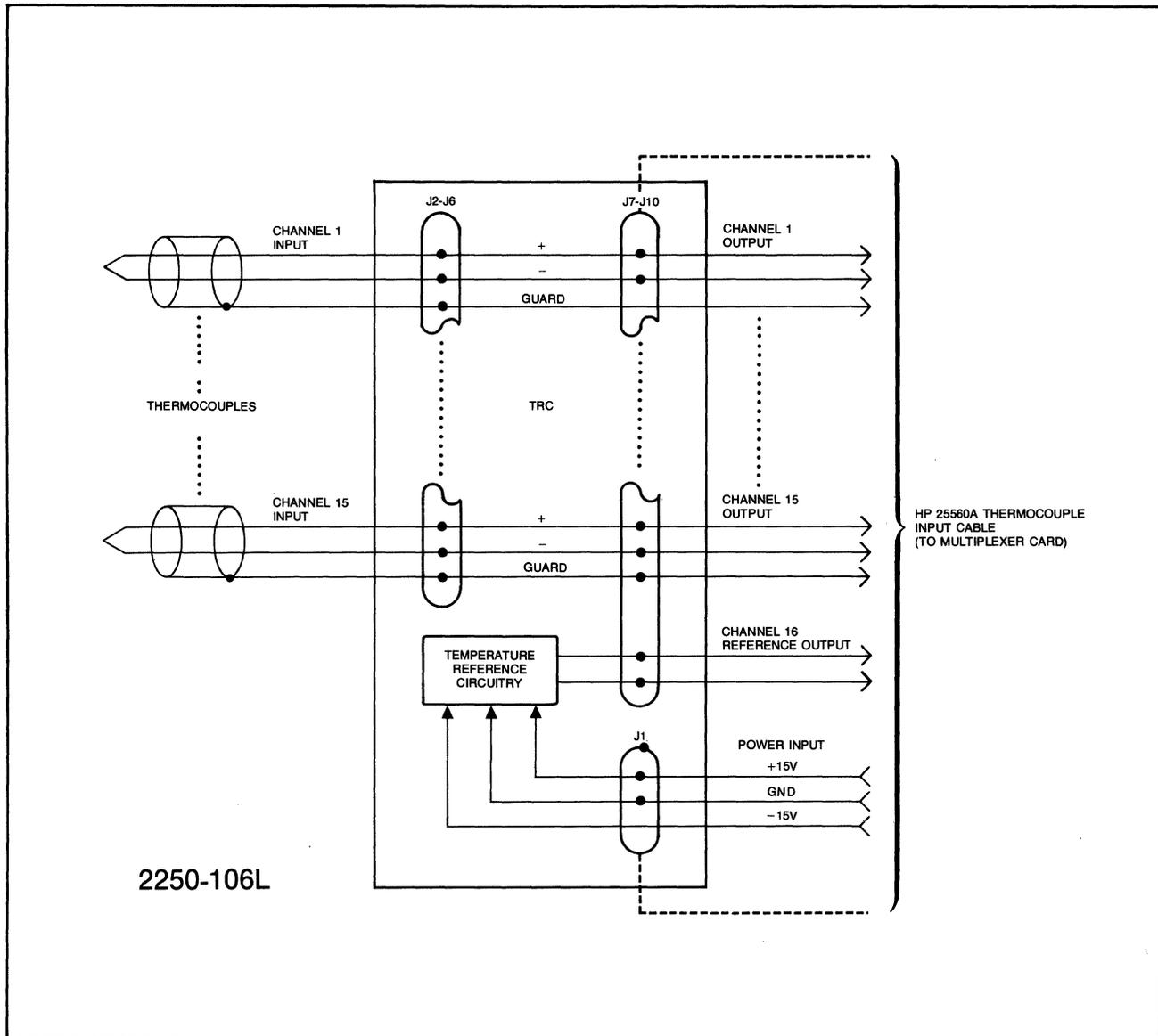
Figure 13-2. HP 25594A Functional Block Diagram
