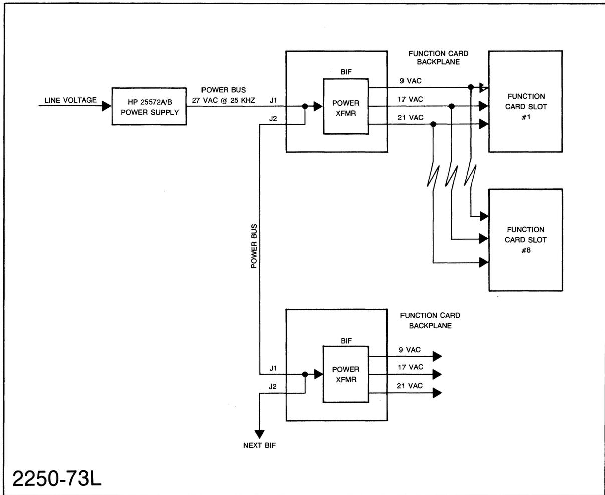
Figure 3-9. Power Distribution Diagram
