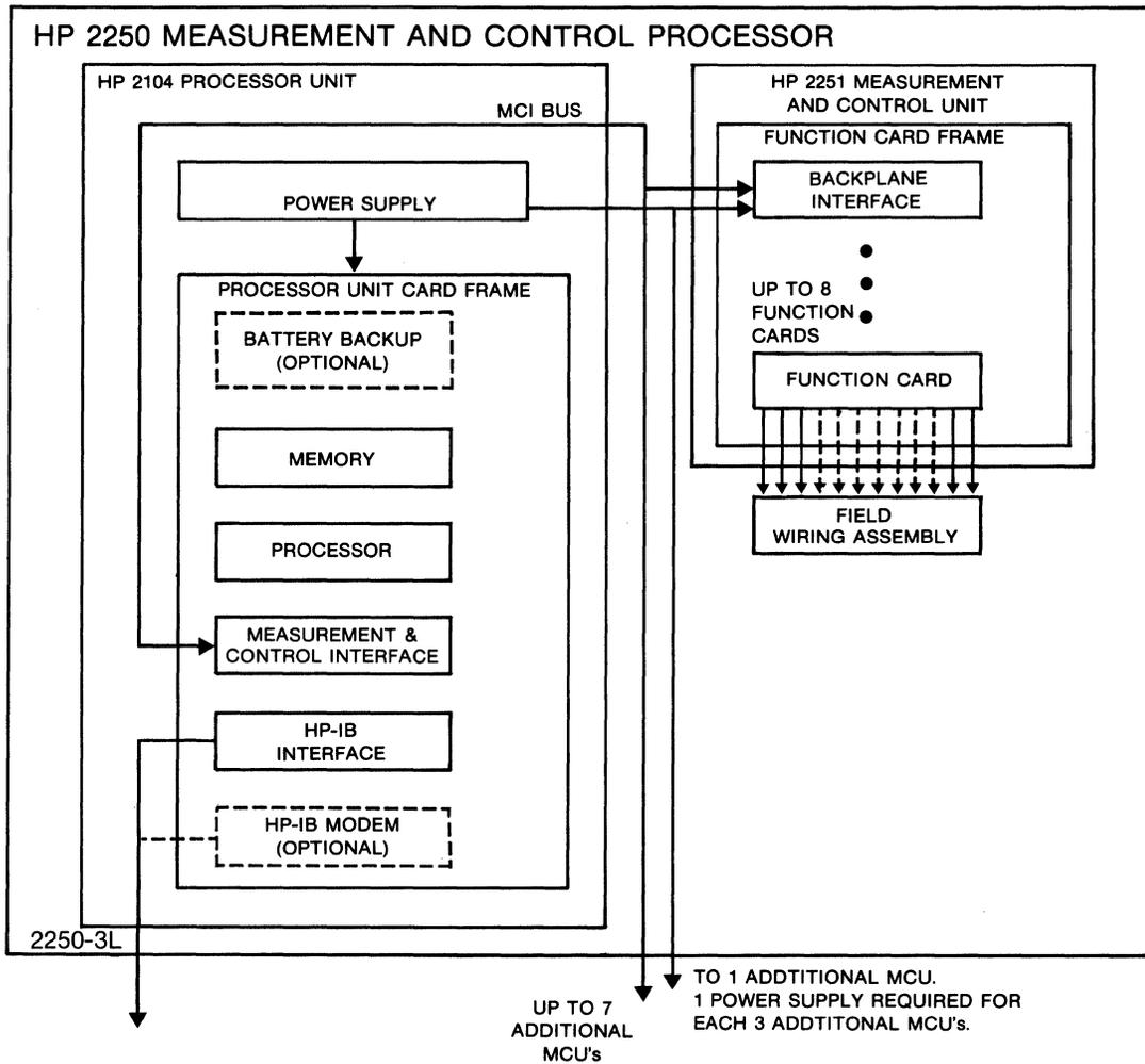
Figure 1-3. HP 2250 Functional Block Diagram
