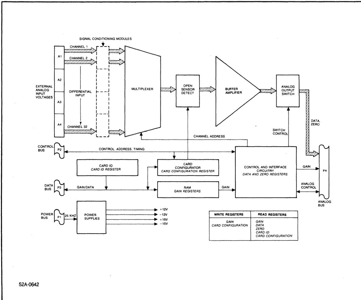
Figure 5-2. HP 25502A Functional Block Diagram
