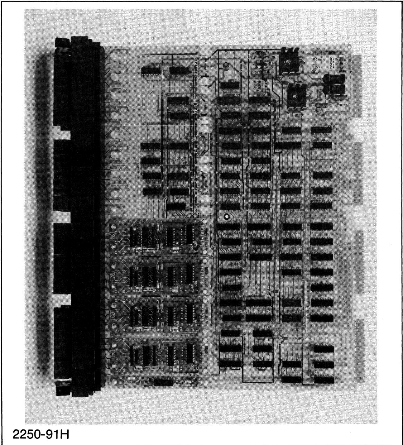
Figure 9-1. HP 25511A 32-Point Digital Input
