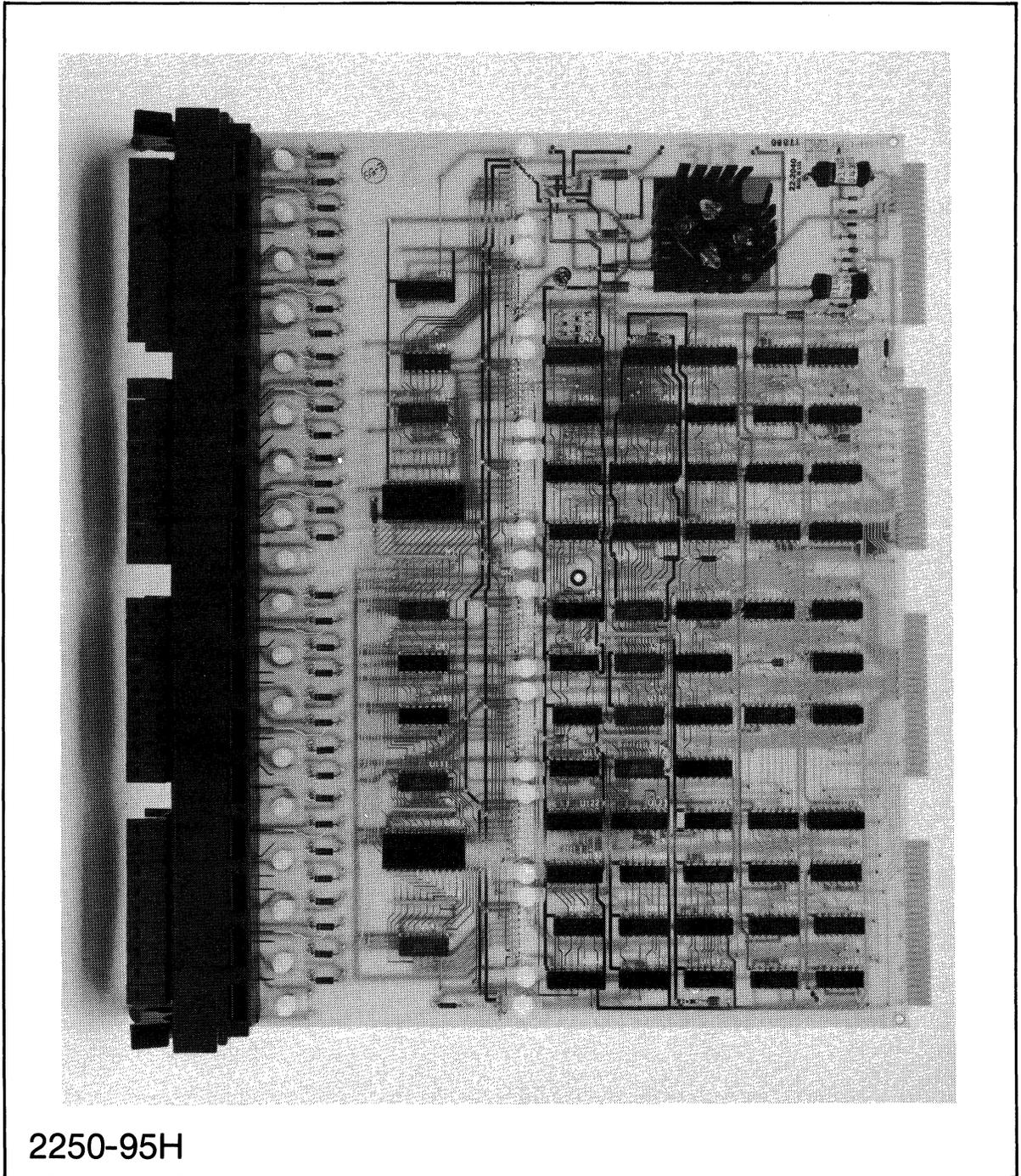
Figure 10-1. HP 25513A 32-Point Digital Output
