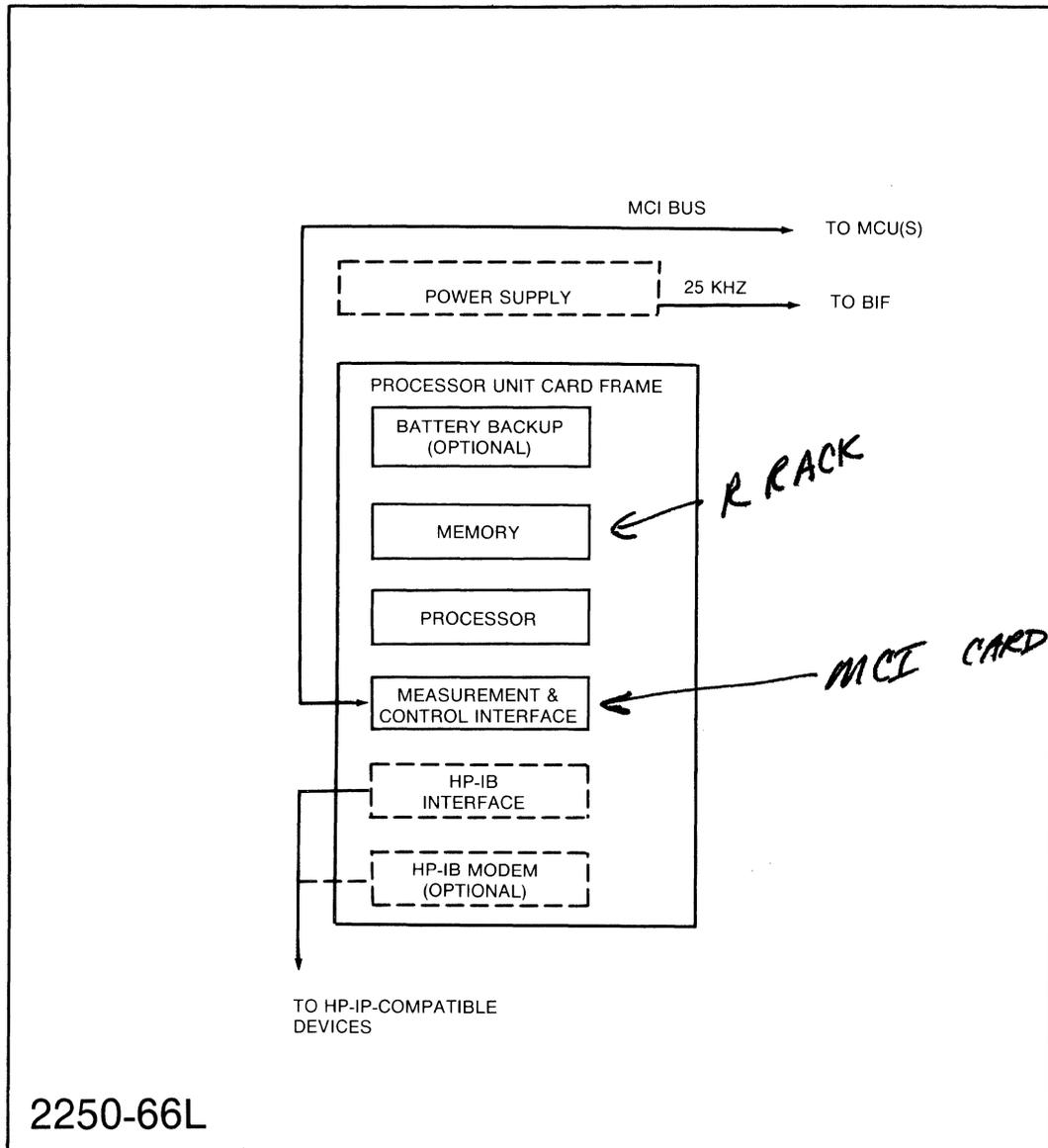
Figure 2-3. HP 2104 Processor Unit Functional Block Diagram
