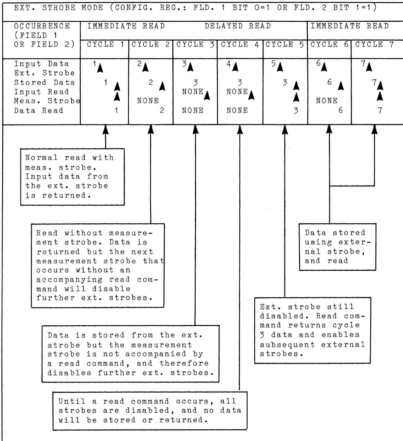
Figure 9-4. External Strobe Mode Operation
