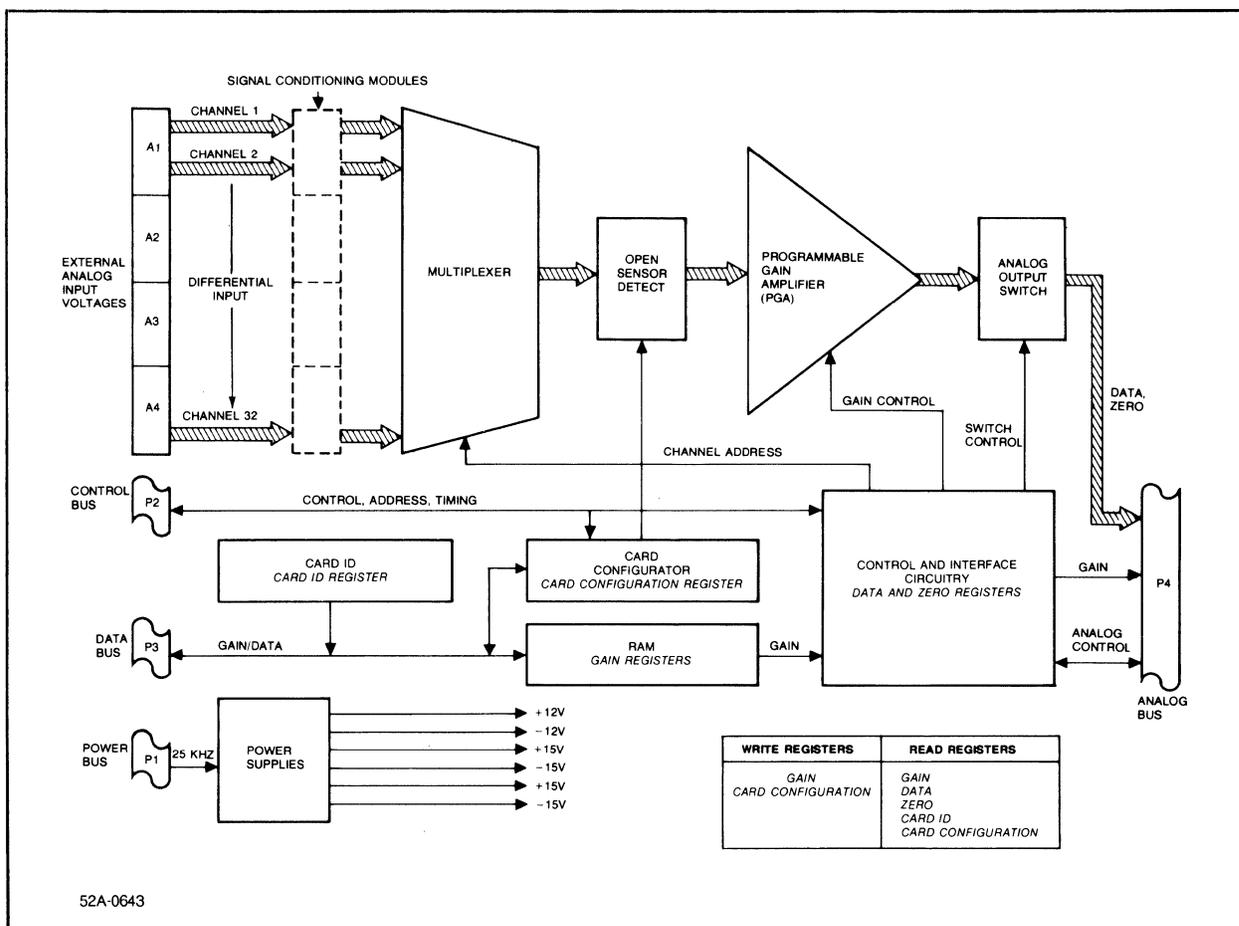
Figure 6-2. HP 25503A Functional Block Diagram
