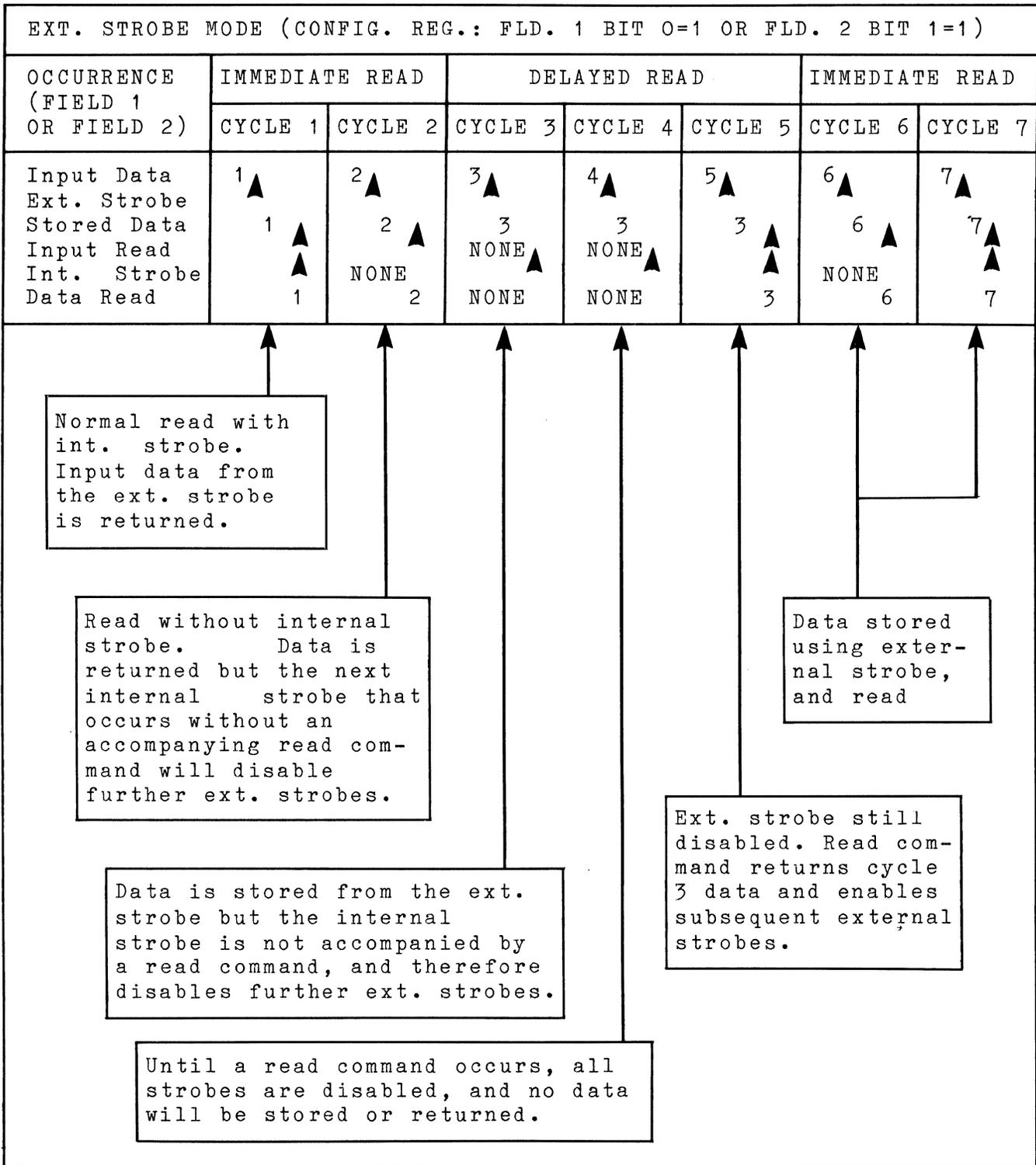
Figure 12-5. External Strobe Mode Operation
