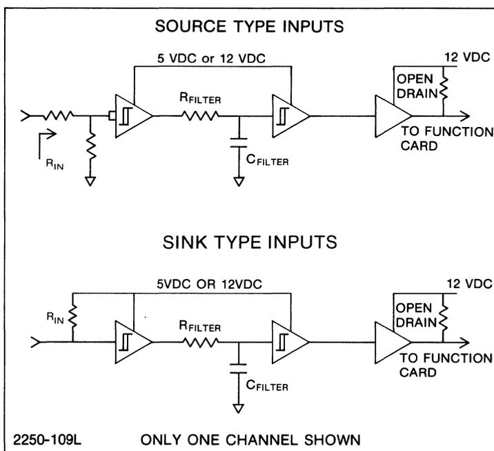
Figure 14-3. HP 25531/25535 Schematic Diagram
