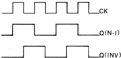
6.3.2 With the 5-MHz signal's rising edge lining up to the 10-MHz clock's rising edge, input the 5-MHz clock to I/O pins 10 and 37.
