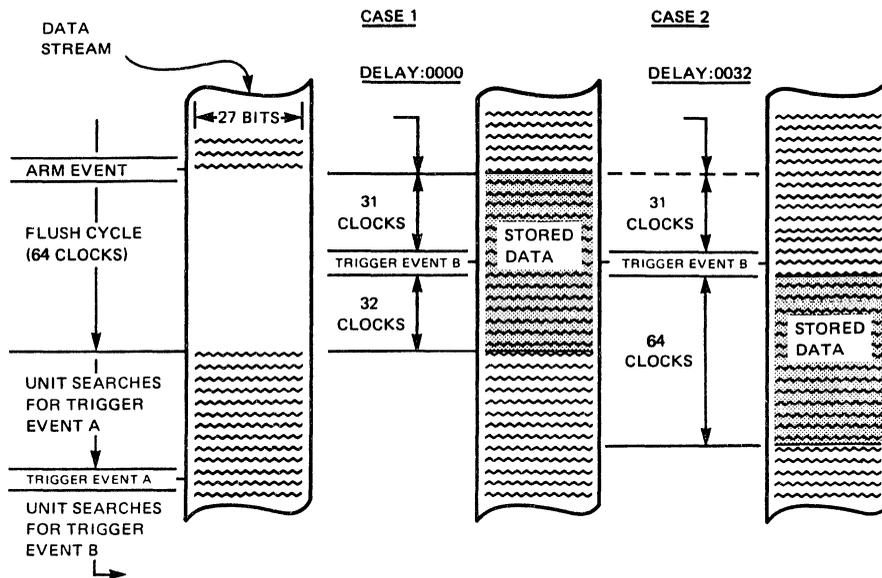
**Figure 3.1. Illustration of Delay by Clocks. Case 1: DLYC = 0000. Case 2: DLYC = 0032 (range: 0-9999 Decimal). This feature allows you to slide the memory window downstream of the trigger event.**
