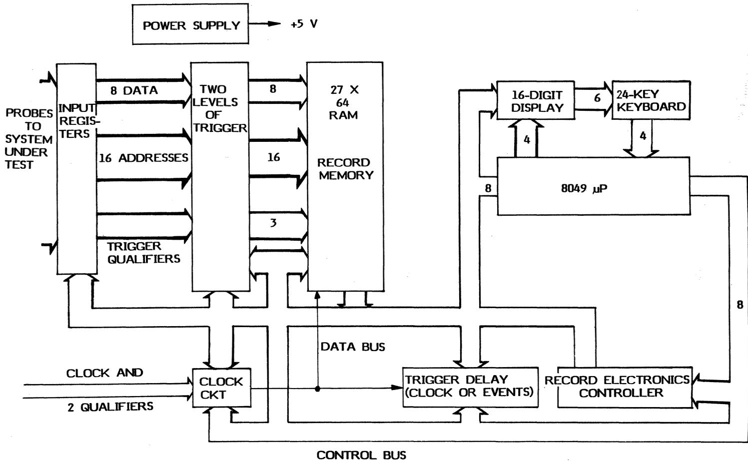
Figure 4.1 2710 Block Diagram
