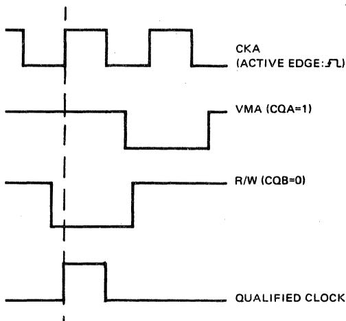
**Figure 3.3 Illustration of Selective Qualification of the Record Clock.** This feature allows you to achieve effective data compression by eliminating unwanted or repetitive data from a recording.
