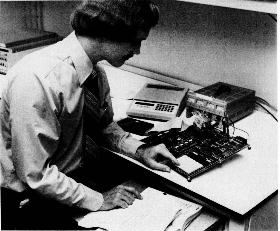
The above photograph shows the Model 2710 Logic Analyzer being used with its companion accessory, the Model 2710 MPU Adapter, on an Intel SDK 8085A board.
