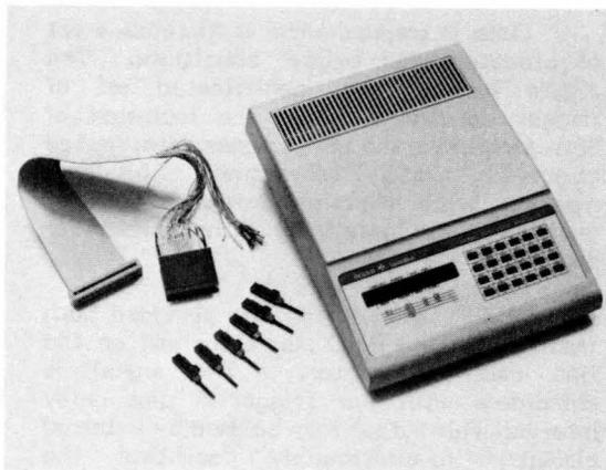
**Figure 1.1 The Model 2710 Logic Analyzer is supplied with a flying lead ribbon cable, six hook-type grabbers, and a 40-pin dip clip for easy connection to your system.**
