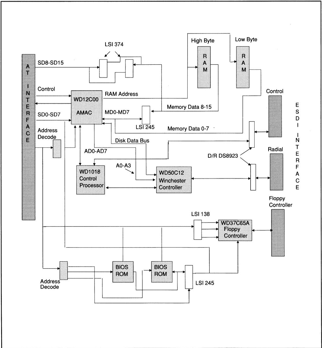
FIGURE 1. WD1007A-WA2 BLOCK DIAGRAM
