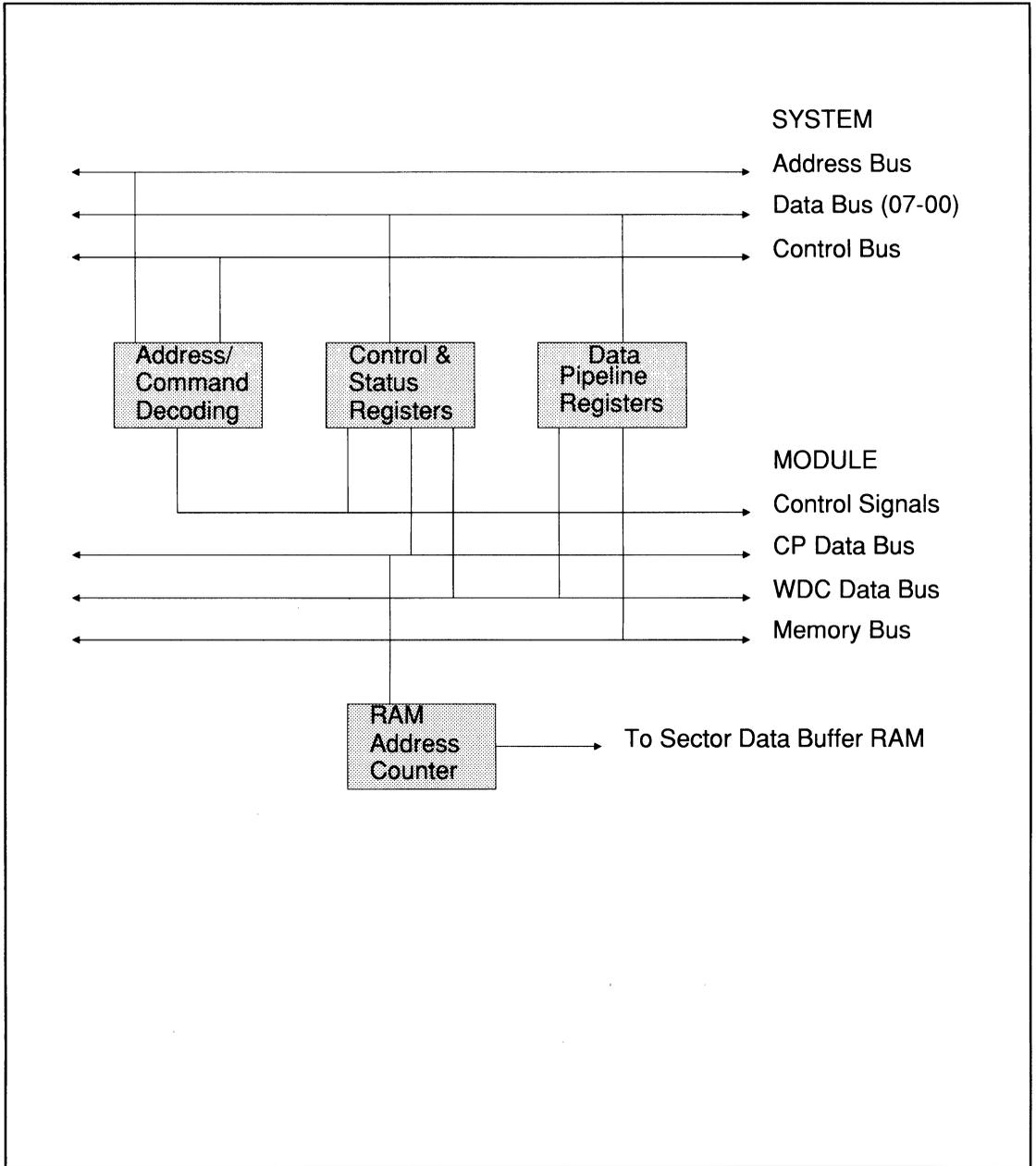
FIGURE 2. AMAC BLOCK DIAGRAM
