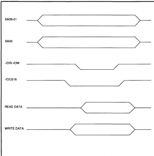
FIGURE 4. SYSTEM BUS SIGNALS - PROGRAMMED I/O CONTROL
