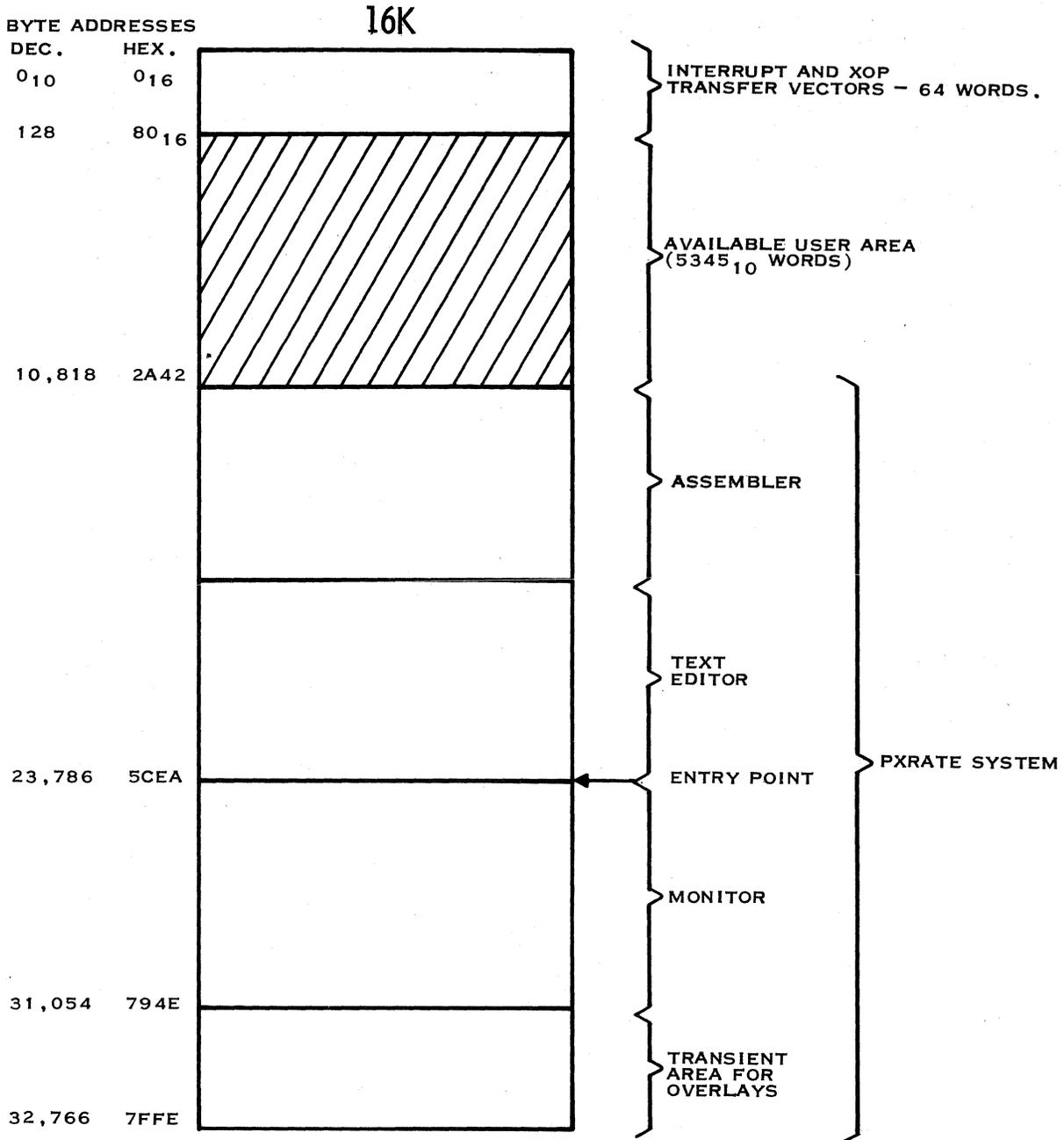
NOTE: LINKING LOADER OVERLAY IS AUTOMATICALLY LOADED IN OVERLAY AREA WHEN PXRATE CASSETTE IS LOADED.
