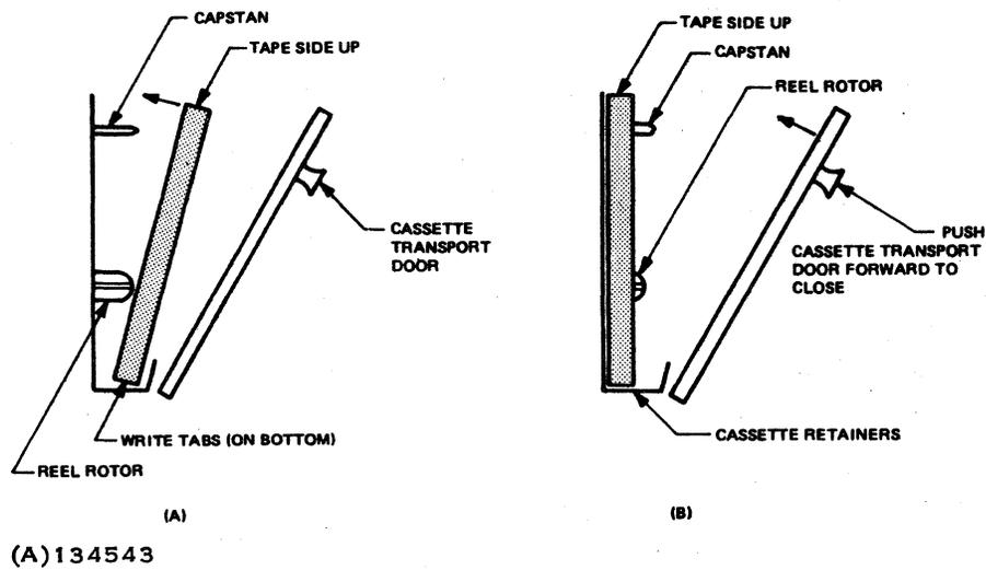
Figure 2-3. Tape Cassette Installation
