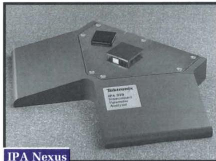
Figure 8. The IPA Nexus is a precision multi-line interface to standard IC packages.
