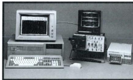
The Digitizing Camera consists of a C1002 Video Camera, a DX01 Frame Store Board inside the PC, DSC01 software, and cables. The system shown includes the DSC01, TEK2467B scope under GPIB control from the DSC01 software, and a DX05 video monitor.
