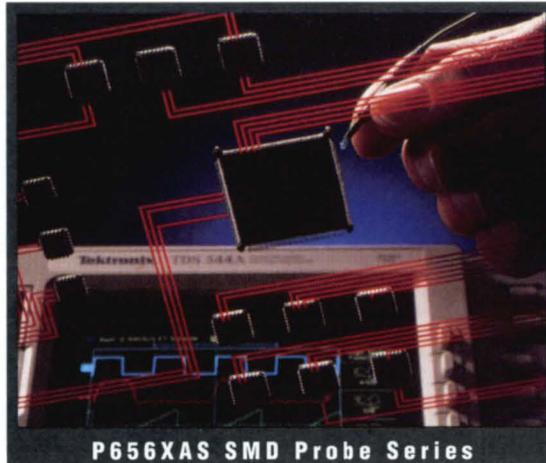
SureFoot™ is an integral probe tip and miniature guide that enables fault-free hand-probing of fine-pitch SMD packages. Using the IC's leads as guides, SureFoot's non-conductive tines align with the leads before the probe tip can contact the device, thus preventing the probe tip from shorting adjacent pins.
