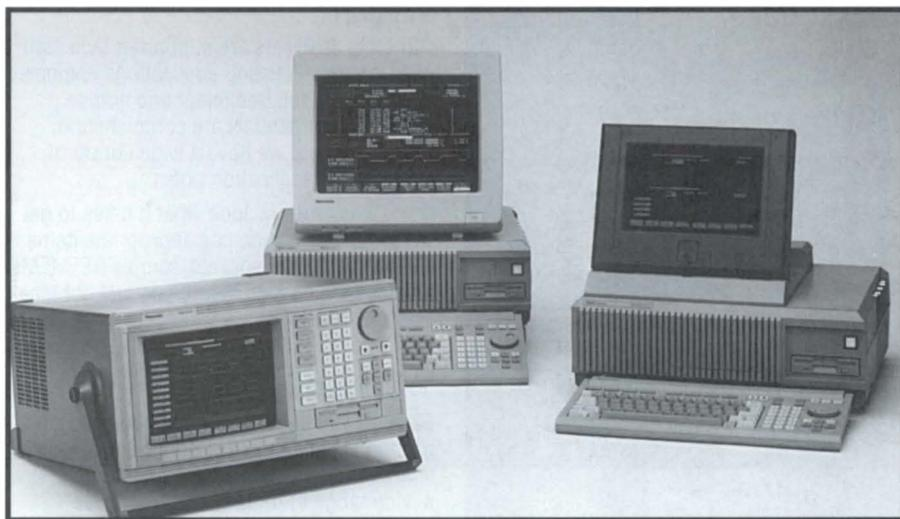
The Tektronix family of general-purpose logic analyzers: the portable 3001GPX; and the modular 3002 series that includes a desktop (3002C) and a portable (3002P) model. All offer a wide range of communications, hard disk storage, and expansion-slot options.
