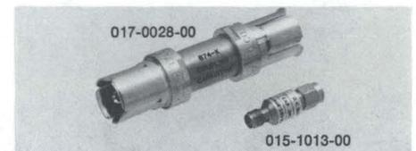
The coupling capacitor is a short length of coaxial line with a disk capacitor (4700 pF, ±20%) in series with the inner conductor. Reflection ratio (in 150 ps tr system), is 0.03 maximum. Voltage rating is 200 V.
