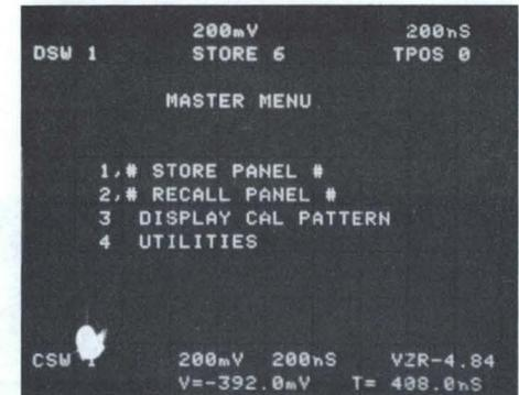
The master menu offers a convenient way to enable special functions such as the STORE and RECALL of front panel settings and also allows you to branch-out to other menus.
