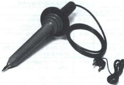
The High Voltage Probe will measure dc voltages from 1 kV to 40 kV with an accuracy of 1% at 25 kV. The division ratio is 1000:1. Common uses include measuring anode voltages on monitors or oscilloscopes. Probe plugs directly into the front end of the multimeter.
