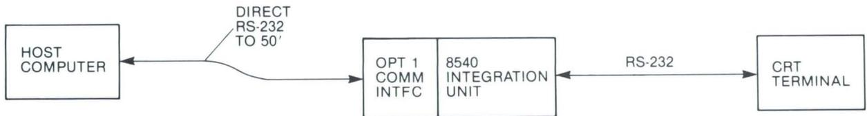
Figure 3a. Direct RS-232 Configuration
