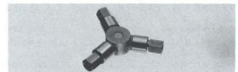
This coaxial tee is designed for use in broad-band 50 Ω systems where the mismatch introduced by ordinary "Tee" connectors is undesirable. Load isolation is nominally 6 dB while the voltage attenuation ratio is nominally 2X (input to either load arm, other load arm terminated in a standard 50 Ω termination). Maximum vswr is 1.50 from dc to 12.00 GHz and 1.90 from 12.01 to 18.00 GHz.
