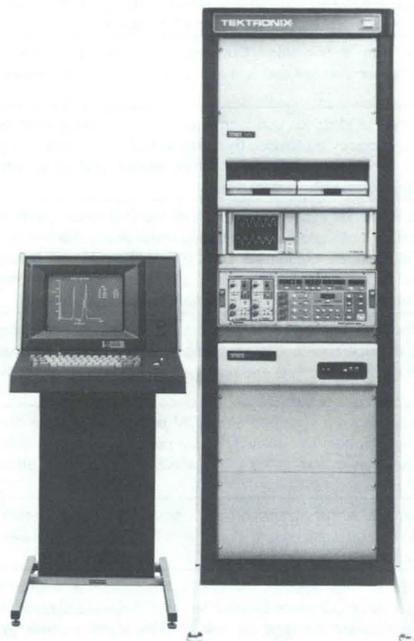
Tektronix WP3202 Signal Processing System using TEK SPS BASIC and a DEC PDP-11 Minicomputer
