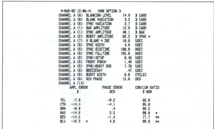
Figure 6. Measurement results are displayed in an easy-to-read format indicating the time, signal source, measurement, and whether the measured value exceeded caution (\*) or alarm (\*\*) limits. This same format is also used for printing errors during the monitoring process, and for reporting manual measurements.
