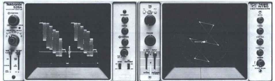
1420 NTSC Vectorscope shown side-by-side with a 528A Waveform Monitor
