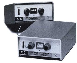
The 2701 and 2703 Step Attenuators are laboratory quality, bench top instruments for attenuation of large value radio frequency signals. The 2701 50  $\Omega$  Attenuator is particularly useful in making receiver sensitivity and distortion measurements. The range of attenuation is 0 to 79 dB, selected in 1 dB steps with tens and units cam switches. A front-panel switch selects DC, AC, or DC TERM (a 50  $\Omega$  precision termination).
