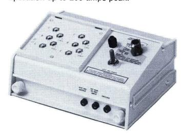
One of the features that sets the 576 apart from the 577 is the display area READ-OUT. Adjacent to the 576's crt are alphanumeric indicators of vertical and horizontal deflection factor, step amplitude, and Beta/div or gm/div. The Beta or gm readout saves the operator from the arithmetic usually necessary to arrive at these parameters. The READ-OUT also provides a permanent record of major knob settings in 576 crt photographs.
