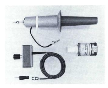
The P6015 provides 1000X attenuation for oscilloscope measurements up to 40 kV peak. Voltage or duty cycle derating is necessary for rf voltages at frequencies over 100 kHz, or in temperatures above 25°C.
