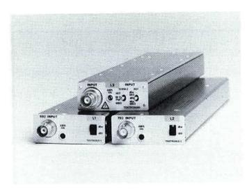
Changeable modules permit the 7L5 user to adapt to new measurement requirements. Modules now available are the 50  $\Omega$  L1, 75  $\Omega$  L2, and 1 M $\Omega$  L3. The probe-compatible L3 offers selectable internal 50  $\Omega$ , 1 M $\Omega$ , or 600 $\Omega$  impedance, while the L3-1 offers 75 $\Omega$ , 1 M $\Omega$ , or 600 $\Omega$ . The module you select calibrates displays for the impedance in use.
