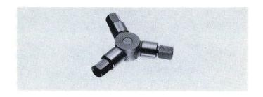
This coaxial tee is designed for use in broad-band 50  $\Omega$  systems where the mismatch introduced by ordinary "Tee" connectors is undesirable. Load isolation is nominally 6 dB while the voltage attenuation ratio is nominally 2X (input to either load arm, other load arm terminated in a standard 50  $\Omega$  termination). Max vswr is 1.50 from dc to 12.00 GHz and 1.90 from 12.01 to 18.00 GHz.
