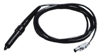
The P6430 Temperature Probe is used with the DM 502 for sensing temperature from  $-55^{\circ}\text{C}$  to  $+150^{\circ}\text{C}$ . The temperature sensing element consists of a transistor and is installed in the probe's nose tip. Temperature is measured by applying the flat surface of the probe's tip to the device being mea-
