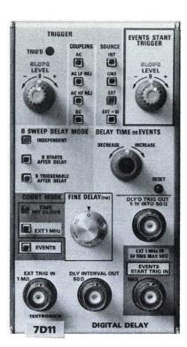
sweep (see Fig 2). When used in the A horizontal compartment, the 7D10/7D11 B sweep delay mode controls will permit the B sweep to run after the delay generated by the 7D10/7D11. This delay interval is also available at the front panel for such uses as gated interval counter measurements and generating pulses of highly accurate width.
