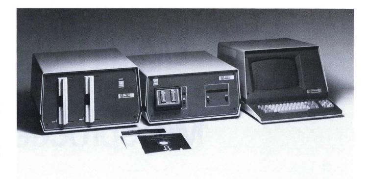
The 8002 Microprocessor Lab consists of the 8002 mainframe; the dual flexible disc unit; an optional system terminal (TEKTRONIX CT8100 or CT8101 recommended); and two sets of assembler software for two different microprocessors, chosen from the microprocessors supported at time of purchase. An emulator processor module for each microprocessor the system supports, and its associated prototype control probe, are offered as options.
