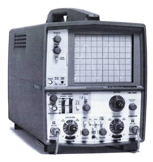
T932A 35 MHz Dual-Trace Oscilloscope
