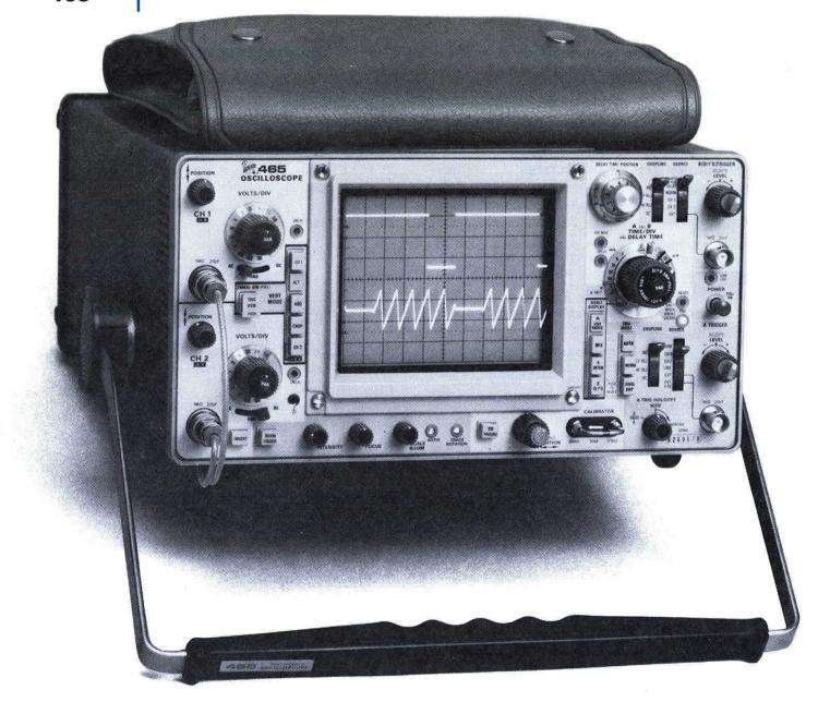
Except for the TIME/DIV and VOLTS/DIV controls, the 465 pictured above is identical in appearance to the 475 and 475A.
