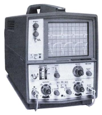
T922 15 MHz Dual-Trace Oscilloscope
