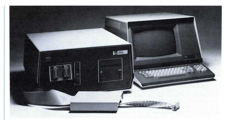
The 8001 Microprocessor Lab consists of the 8001 mainframe; an optional system terminal (TEKTRONIX CT8100 or CT8101 recommended); and a Microprocessor Support Package for the microprocessor selected. A support package includes an emulator ROM, an emulator processor, and a prototype control probe.
