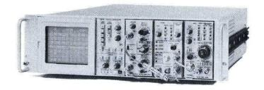
The R7313 requires only 51/4 in of rack height in a standard 19 in rack. It is fan cooled and comes complete with slide-out chassis tracks.
