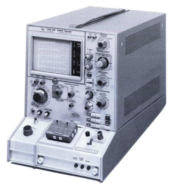
The TEKTRONIX 576 Curve Tracer System continues to hold the title "standard of the industry." The 576 accepts three different test fixtures: the Standard Test Fixture, 172 Programmable Test Fixture (described on p 204), and the 176 Pulsed High-Current Fixture (described on p 205). The 576 is an excellent general-purpose curve tracer system that performs well in applications where high current testing is required.
