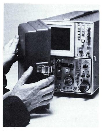
Option 08 protective front cover is shown on 7613 Mainframe.
