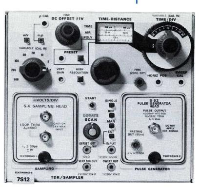
Pulse Amplitude — At least +400 mV into  $50 \Omega$ .
