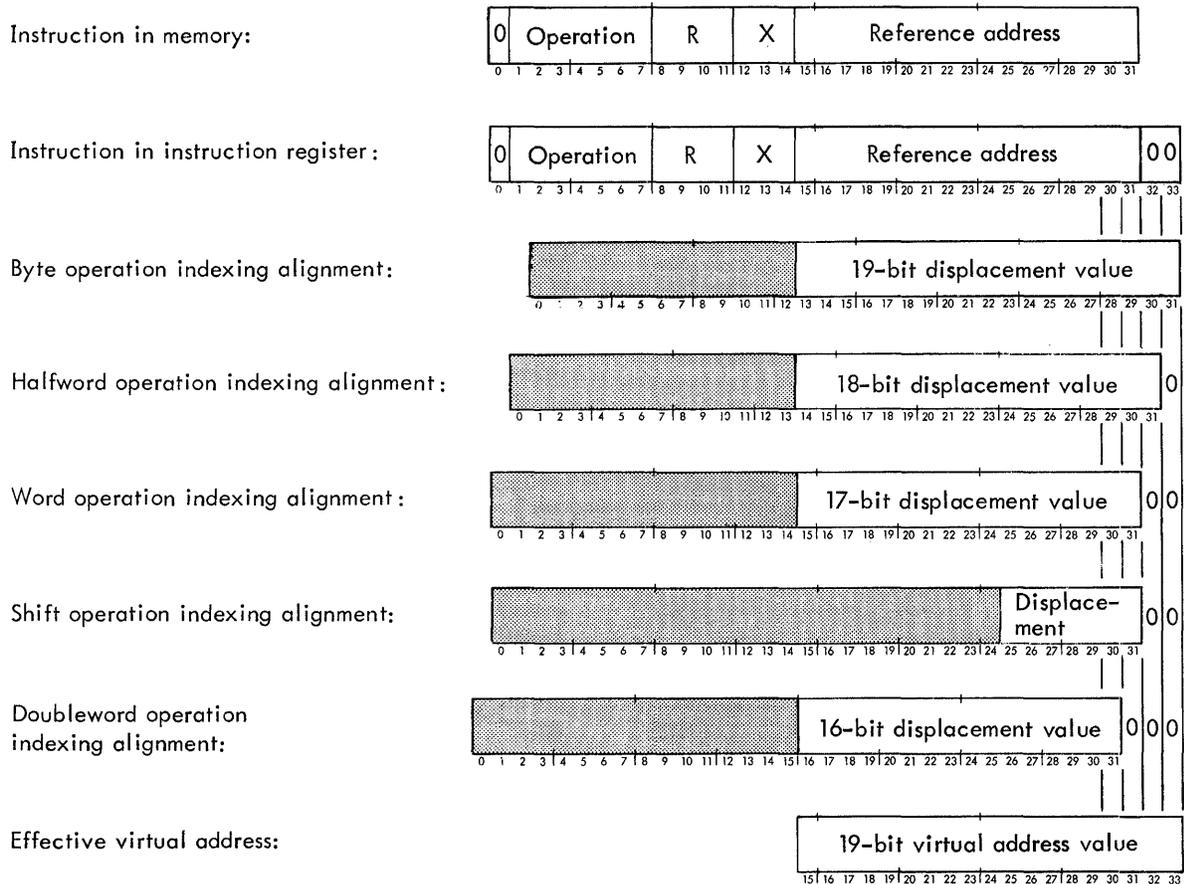
Figure 4. Index Displacement Alignment
