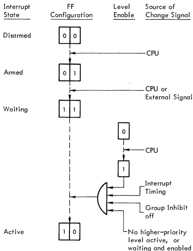
Figure 7. Interrupt Level Operation
