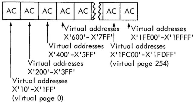
The memory page address and access control codes can be changed only by means of the privileged instruction MOVE TO MEMORY CONTROL (see "Control Instructions").
