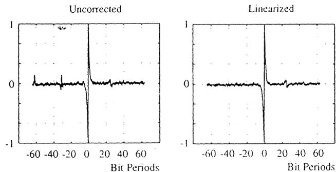
Fig. 4. Dipulse response of the uncorrected channel shows many additional “echos” due to nonlinear readback. Density is 110 kfci.
