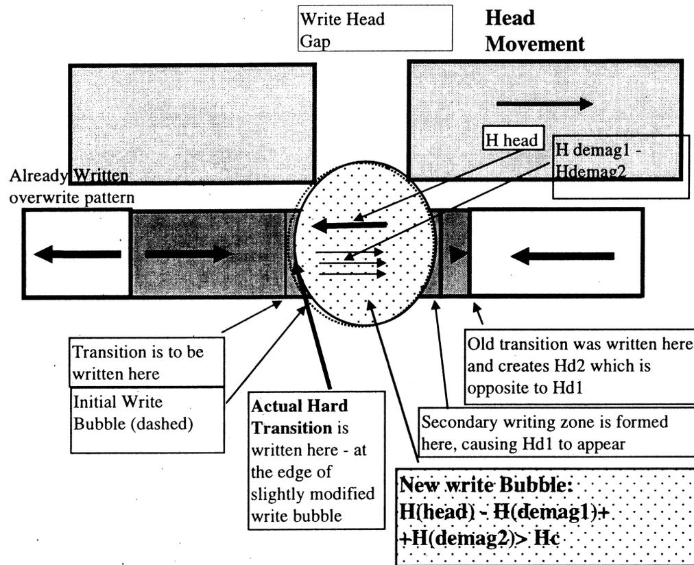
When a new transition of the HF pattern is written in the proximity of the old transition of the LF pattern, the demagnetization field of the old transition reduces the effective value of  $H_{TS}$ . This effect is statistical and becomes negligible at low density
