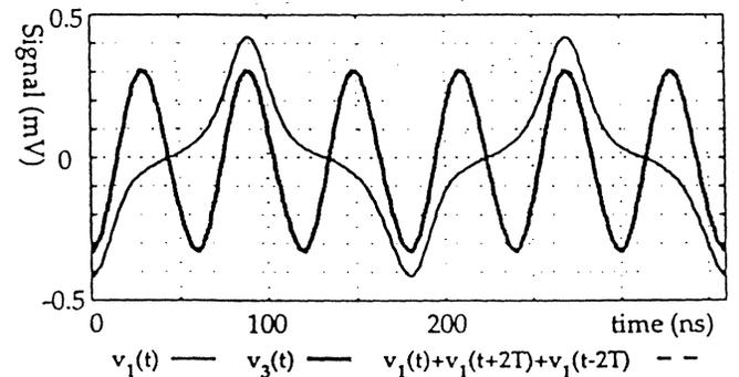
FIG. 3. MR read signals after applying the inverse MR transfer function. Note that the high frequency linearized signal is equal to the sum of three low frequency linearized signals and that peak amplitudes are symmetrical.
