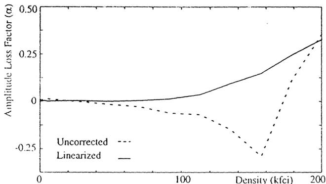
Fig. 2. Partial erasure amplitude loss factor measured using the third harmonic ratio method. Negative values of amplitude loss factor at moderate density are an artifact of nonlinear readback. Linearizing the channel eliminates this effect.
