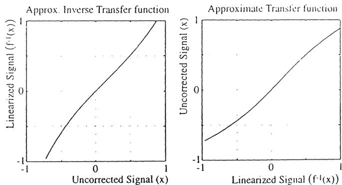
Fig. 1. Polynomial approximation for the inverse transfer function. Axes are scaled so that the height of a positive isolated peak is one unit.
