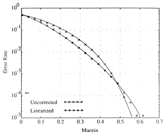
Fig. 7. Sequence amplitude margin at 100kfci with and without linearization. Linearization before equalization shows improved performance for small margins.
