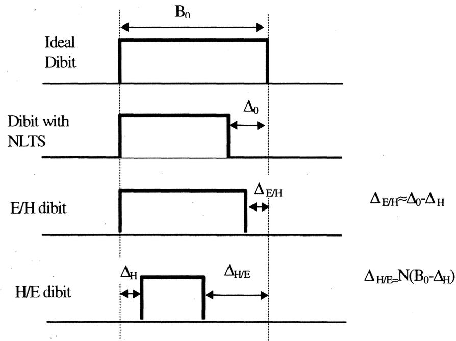
Figure 6.10 Interactions of NLTS with Hard Transition Shift
