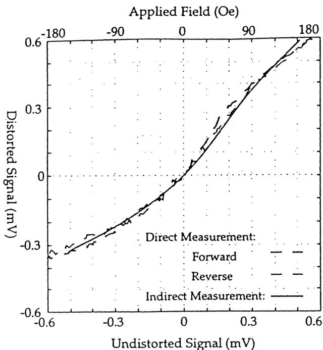
FIG. 4. The MR transfer function. The dashed lines were obtained directly by applying a known field to the head with a MR head tester. The solid line was obtained using the method described here using a 4th order polynomial to model the inverse transfer function. The field strength above the medium was inferred by comparing peak signal amplitude with the direct measurements of the MR transfer curve.
