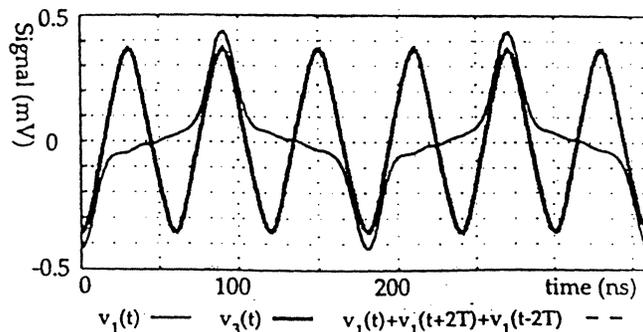
FIG. 1: Read signals obtained experimentally using an inductive head (averaged over 1000 sweeps). Read-back with an inductive head is a linear process and superposition applies. Note that the high frequency signal is equal to the sum of three low frequency signals.
