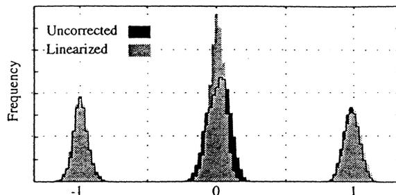
Fig. 6. Histogram of sample values for recording at 100kfci. Linearization before equalization produces a slimmer distribution.
