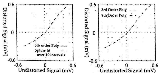
FIG. 5. MR transfer curves obtained using different functions to model the inverse transfer function.
