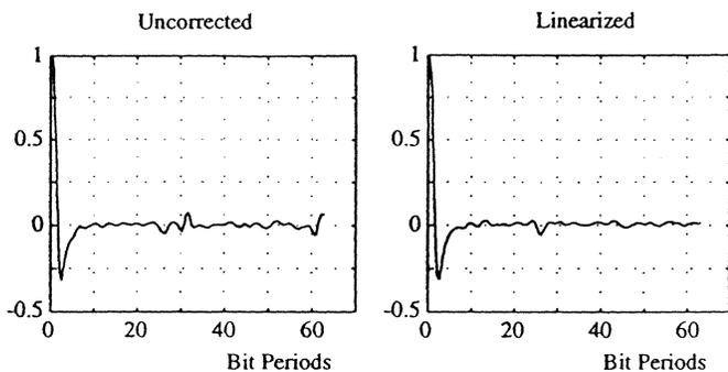
Fig. 5. Read signal autocorrelation function for a pseudorandom pattern. Nonlinear readback produces a strong “echo” which overlaps the echo due to NLTS. Linearizing the channel eliminates this “echo”. Density is 110 kfci.
