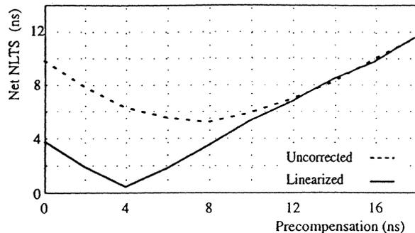
Fig. 3. NLTS estimated by 5th harmonic elimination. For the uncorrected channel net NLTS appears to remain high regardless of precompensation. Bit period is 36 ns. Density is 90 kfci
