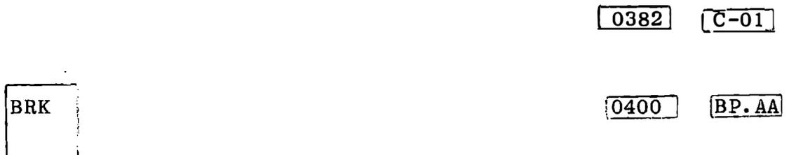
The value displayed at the right hand two digits is a check sum for the content of the PROM memory. It should be AA for all versions of the monitor. Check the monitor version number by:
