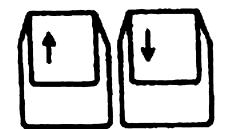
Pressing the **Vertical** (Up and Down) **Arrow** keys, moves the cursor in the direction the arrow is pointing. You can quickly move the cursor any number of lines by holding the key down. When the cursor is located at the position you want, release the key and the cursor stops moving. These keys do not move any of the characters on the screen. They position the cursor only.
