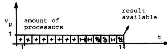
fig. 5: Space-time diagram for one processor
