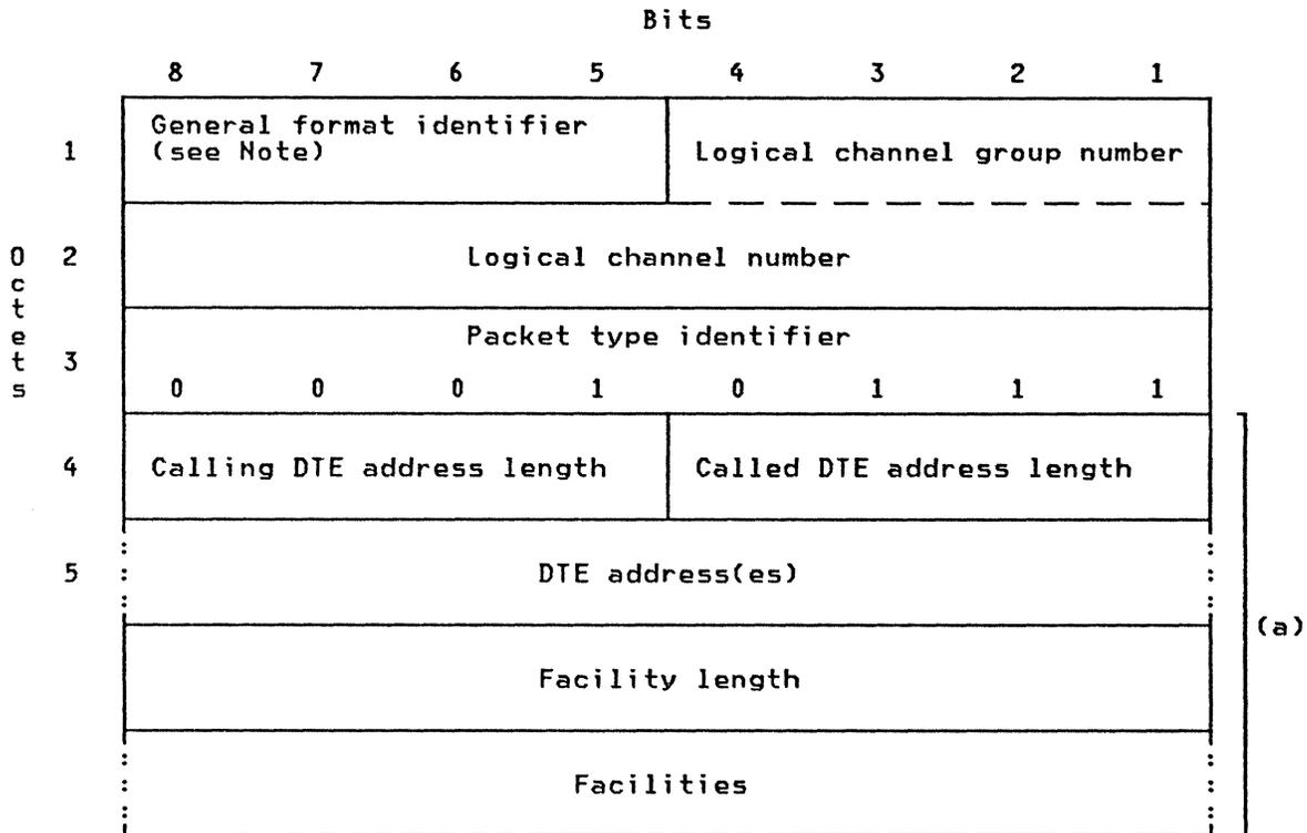
(a) Used only in the extended format of DCE clear confirmation packets.
