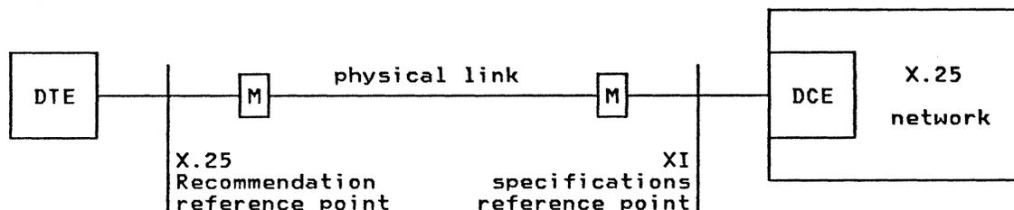
**Note:** This example shows an access link with an analog transmission line and a pair of modems (M). The access link can also be a leased digital circuit with an X.21 interface.
