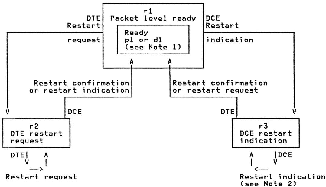
Note 1 - State p1 for virtual calls or state d1 for permanent virtual circuits.
