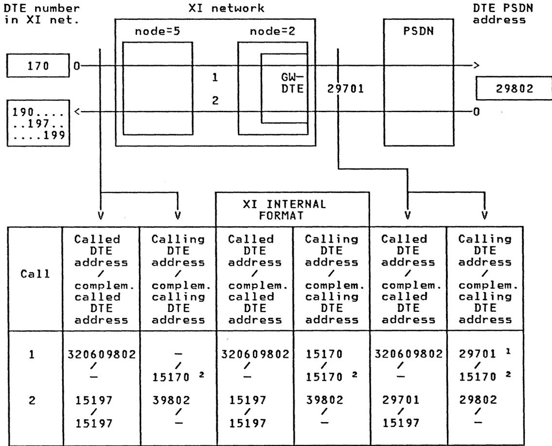
**Note 1** - The calling DTE address is not given by the GW-DTE, but inserted by PSDN.
