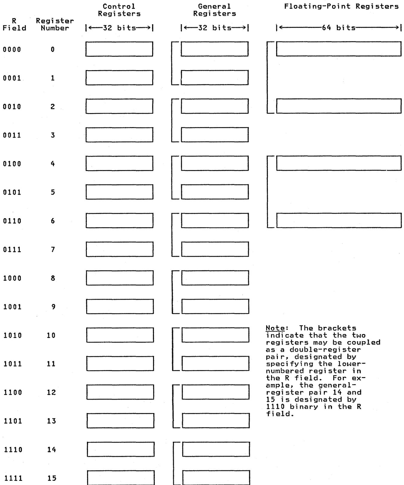
Note: The brackets indicate that the two registers may be coupled as a double-register pair, designated by specifying the lower-numbered register in the R field. For example, the general-register pair 14 and 15 is designated by 1110 binary in the R field.
