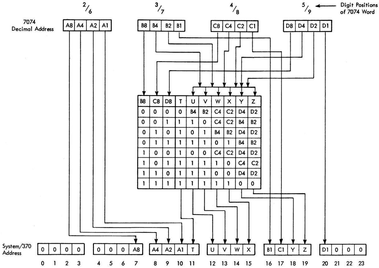
Figure A1. 7074 to System/370 Address Conversion
