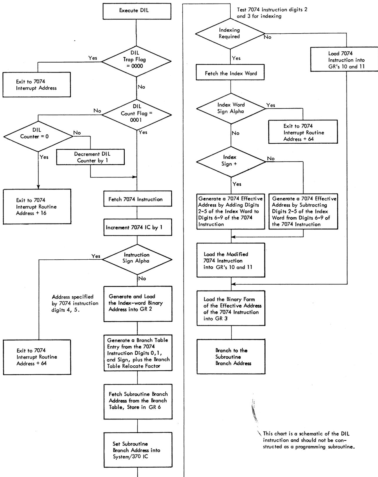
This chart is a schematic of the DIL instruction and should not be constructed as a programming subroutine.
