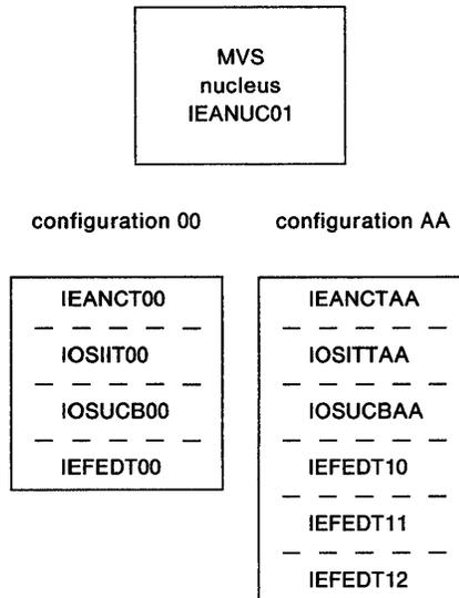
Figure 1-5. MVS/SP Version 3 Multiple I/O Configuration Support
