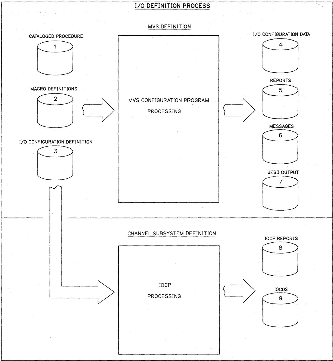
Figure 1-2. MVS and Channel Subsystem I/O Definition Process
