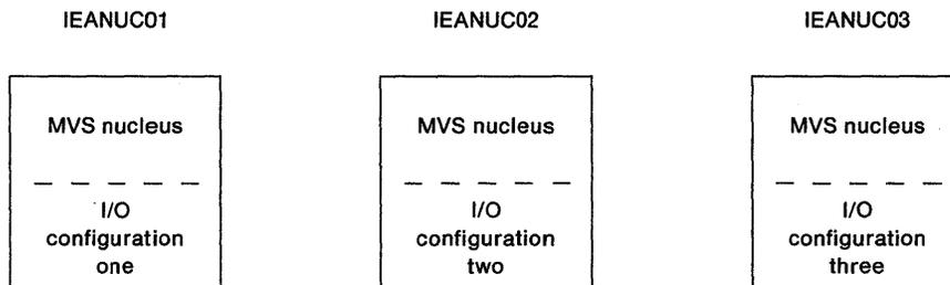
Figure 1-1. Multiple I/O Configuration Support before MVS/SP2.2.0
