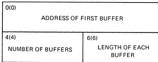
Figure 64. Fields of the QISAM Buffer Control Block
