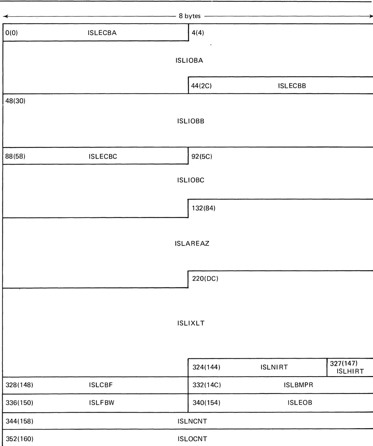
Figure 66 (Part 1 of 2). QISAM Load Mode DCB Work Area
