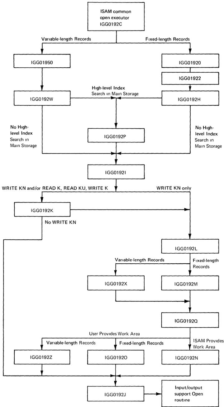
Figure 28. Flow of Control through BISAM Open Executors
