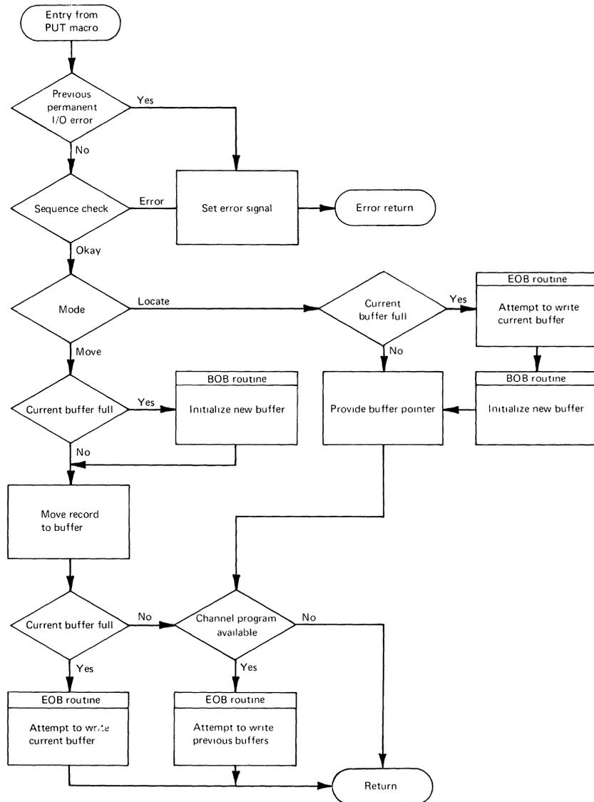
Figure 6. Load Mode Put Routine
