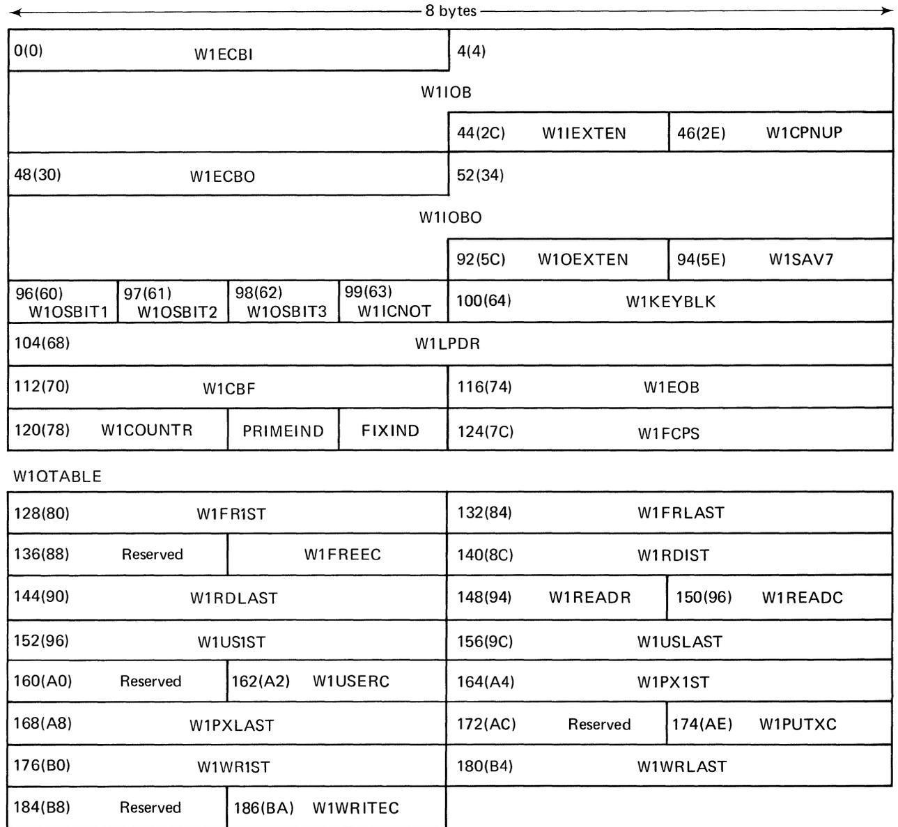
Figure 68 (Part 1 of 2). QISAM Scan Mode DCB Work Area
