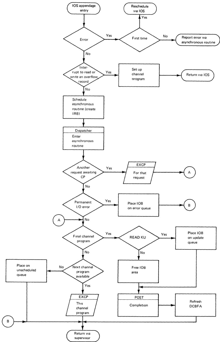
Figure 31. BISAM Appendage and Asynchronous Routines
