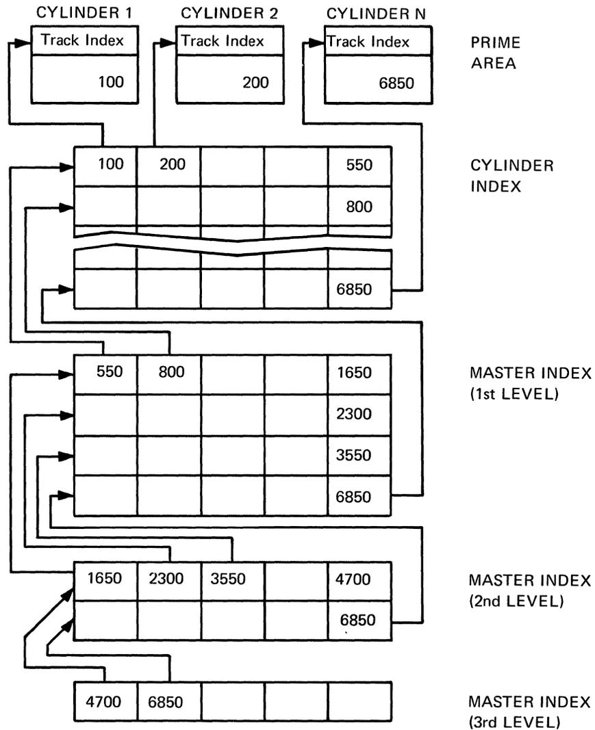
Figure 75. Indexed Sequential Data Set Structure
