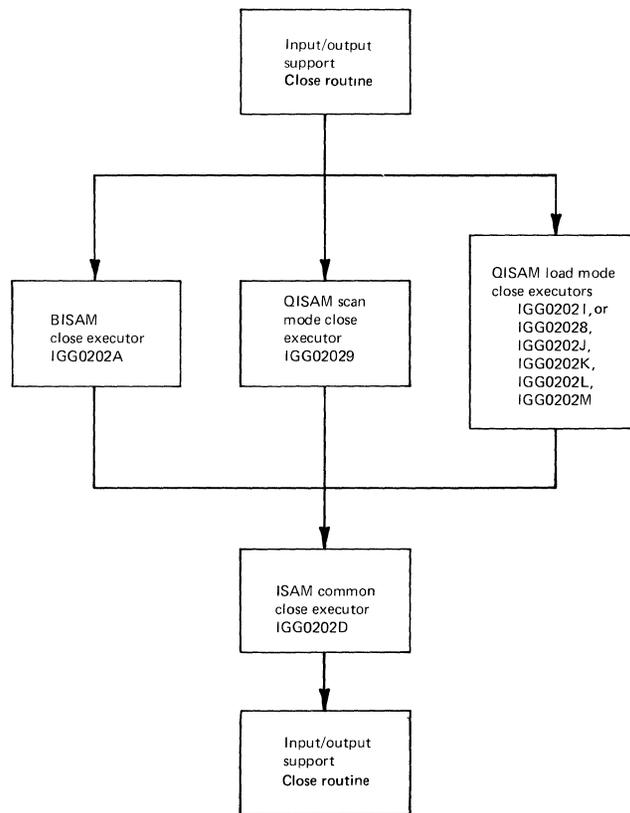
Figure 4. Flow of Control through the Close Executors
