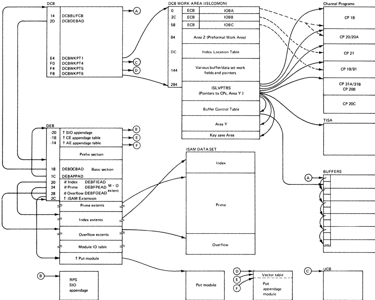
Figure 14. Load Mode Control Blocks and Work Areas
