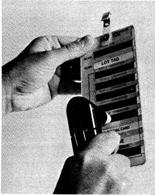
**Figure H-5. Magnetic Hand Scanner (3278 and 3279 Attachments)**
