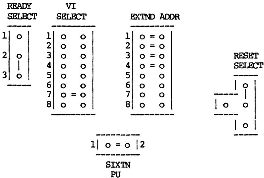
\* The node ID on the LANC ID jumper will change for each board. Refer to the following page to determine the proper jumper configuration for each node.
