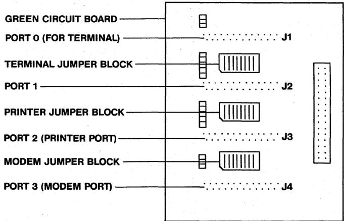
**INSIDE VIEW OF SERIAL PORT I/O BOARDS
