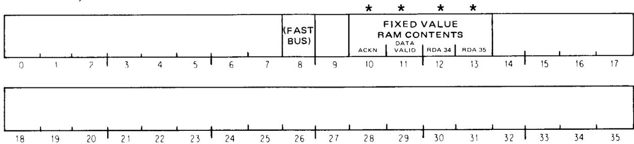
Each controller has a set of four RAMs for supplying logic signals whose values are fixed by the program for the characteristics of the particular system. These RAMs give the acknowledge and data valid signals for the bus, and various configurations of the two least significant read address bits for determining which word to read next during processing of a quad-word. Bits 20-27 of the function word select among the 256 locations in the
