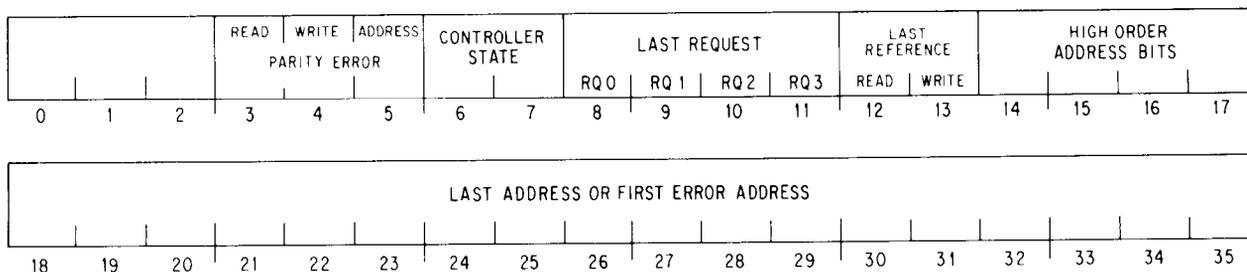
3-5 These are error flags for the storage modules connected to this controller. Setting a flag locks bits 8-35 on the identification of the current reference.
