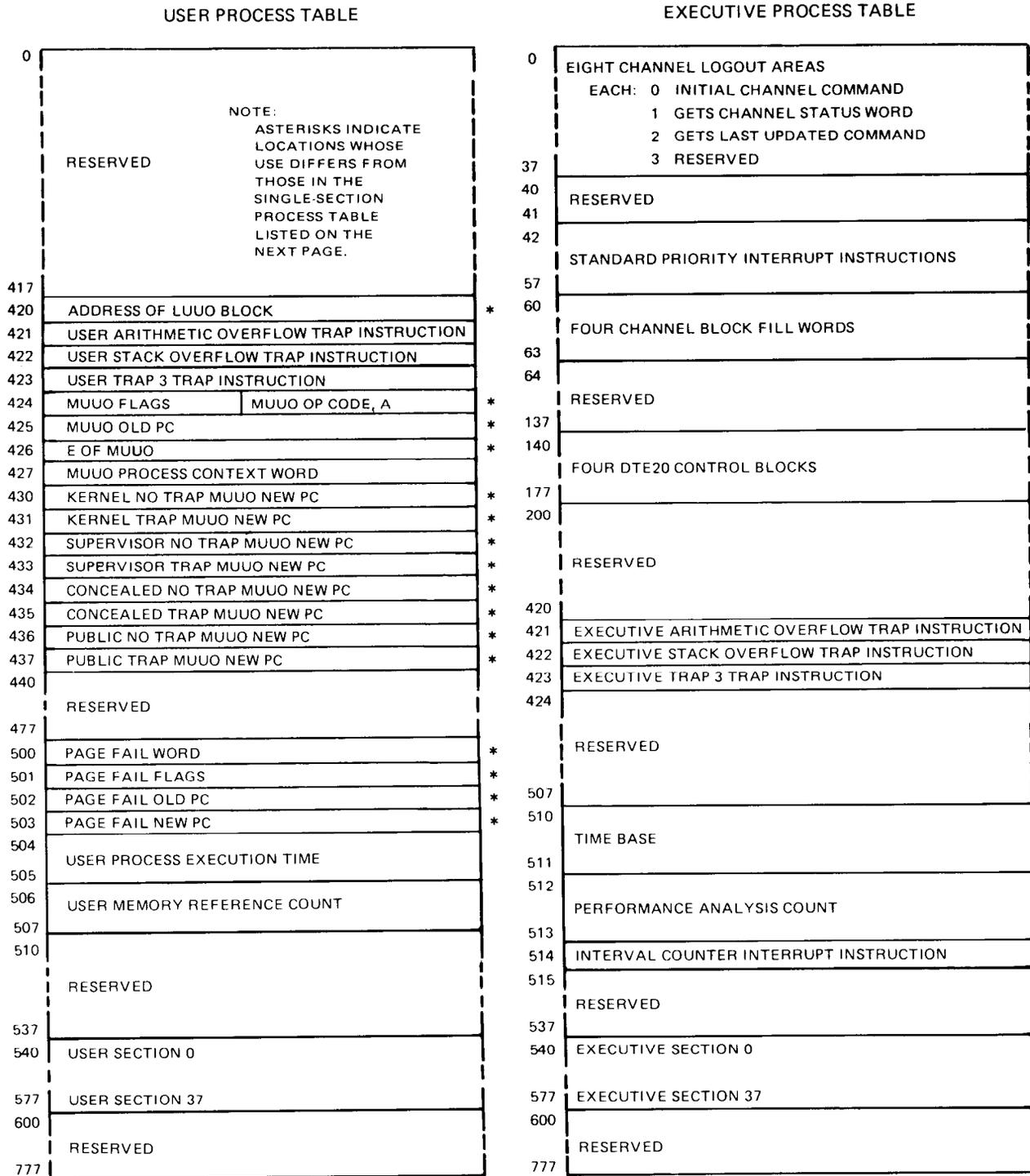
**Figure 3.5: Single-section TOPS-20 Process Table Configuration**
