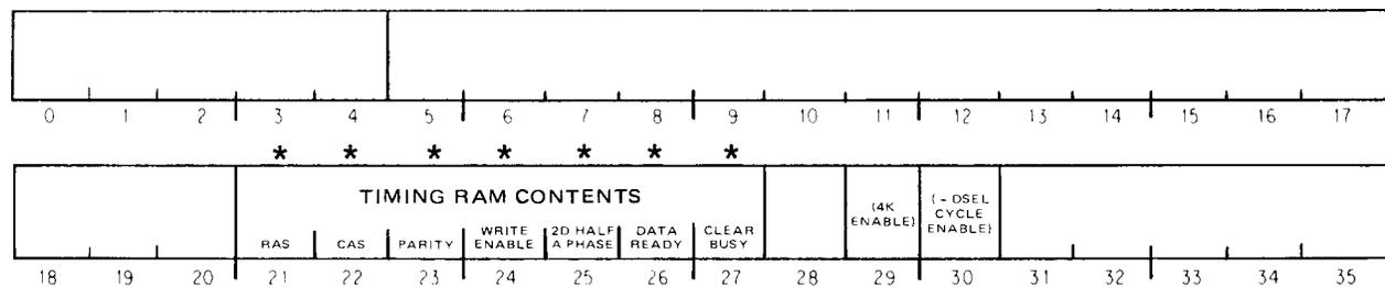
The software must set up the timing characteristics of each controller for the MOS RAMs used with it. To time various signals the clock steps through the locations of a timing RAM, whose bits control the on and off states of those signals. If bit 20 out is 1, the contents of bits 21-27 (adjusted for odd parity) are loaded into the timing RAM at the location specified by bits 13-19. Whether loaded or not, the contents of the selected location are returned in the same bits.<sup>4</sup>
