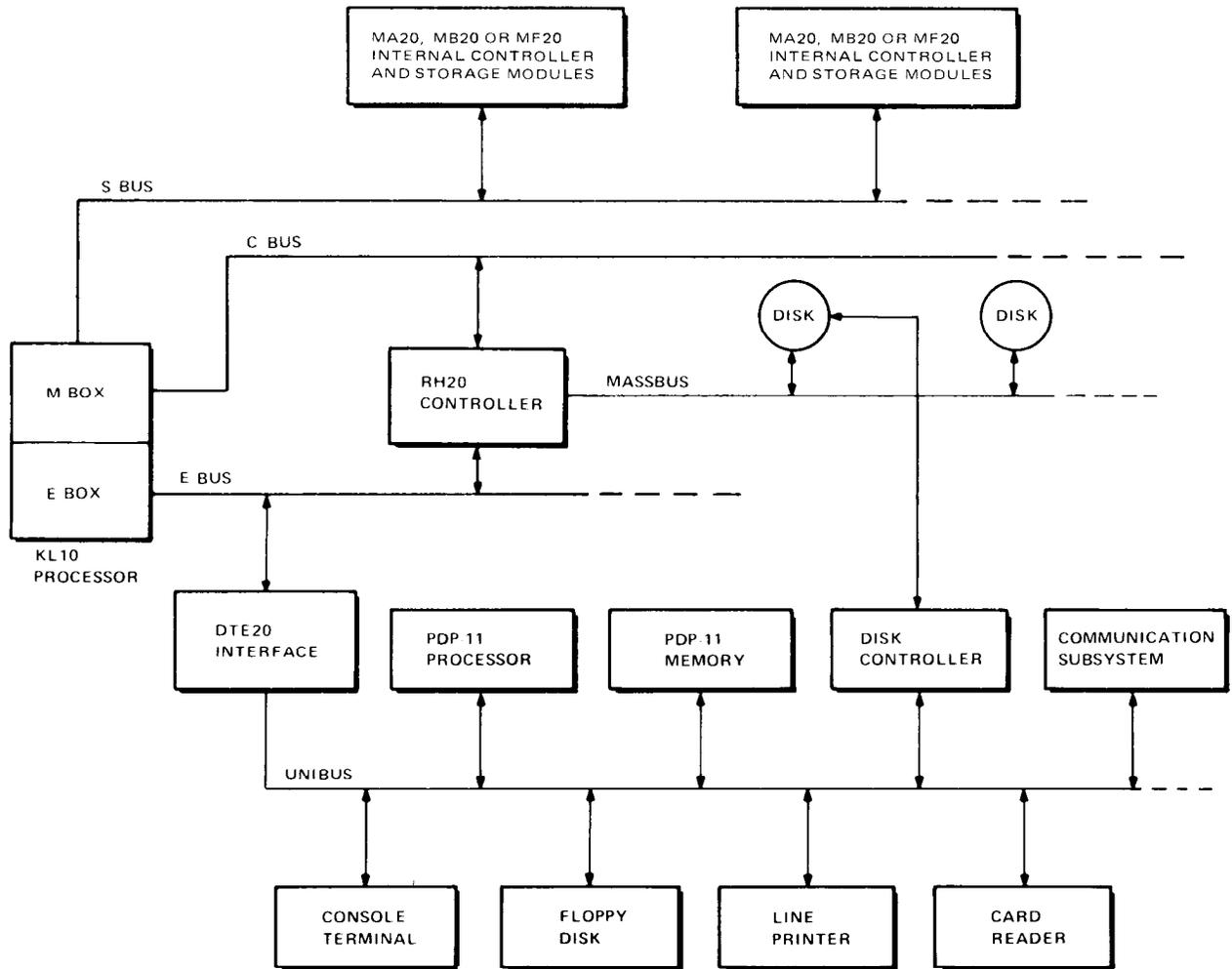
Figure 1.2: KL10-based DECsystem-10
