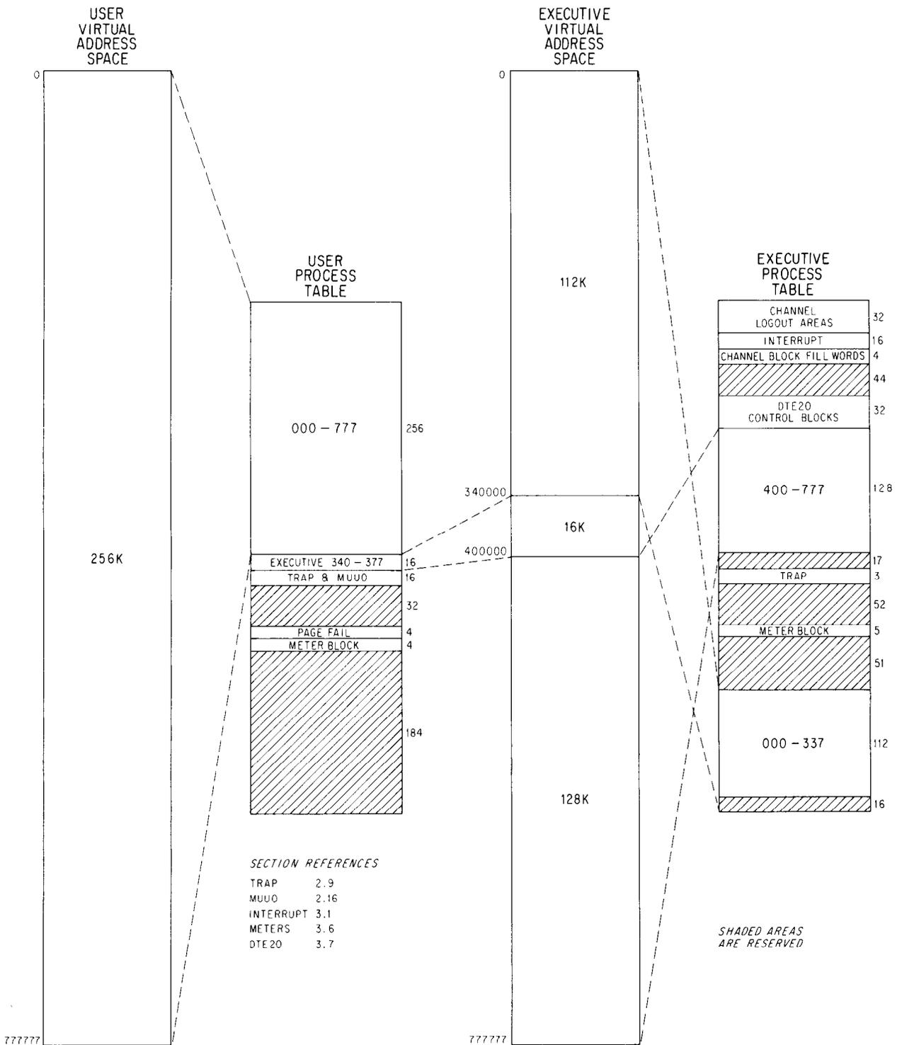
**Figure 3.2: TOPS-10 Process Table Configuration**
