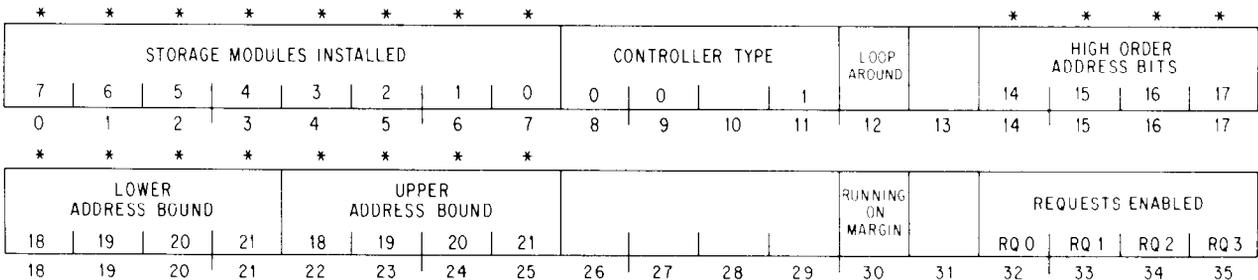
0–7\* Storage modules installed on the controller are indicated by 1s in these bits. At present the maximum is four.
