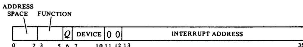
The microcode acts from a function word whether there is one or not; its absence is taken as a zero function. The DIA20 returns the word supplied over the IO bus or simulates a zero word. Bits 7–10 identify the device by its physical number, but this is supplied by the interrupt hardware, not the device. The meanings of the other bits in the word are as follows.
