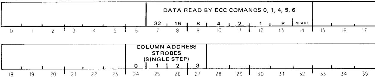
Bits 24–27 of the return contain the present values of the column address strobes to the four array boards in the group selected by the single step address given by function 5. Other information in the return (in some or all of bits 7–14 or occupying the entire word) depends on the ECC command in bits 25–27 of the function. These commands are as follows.
