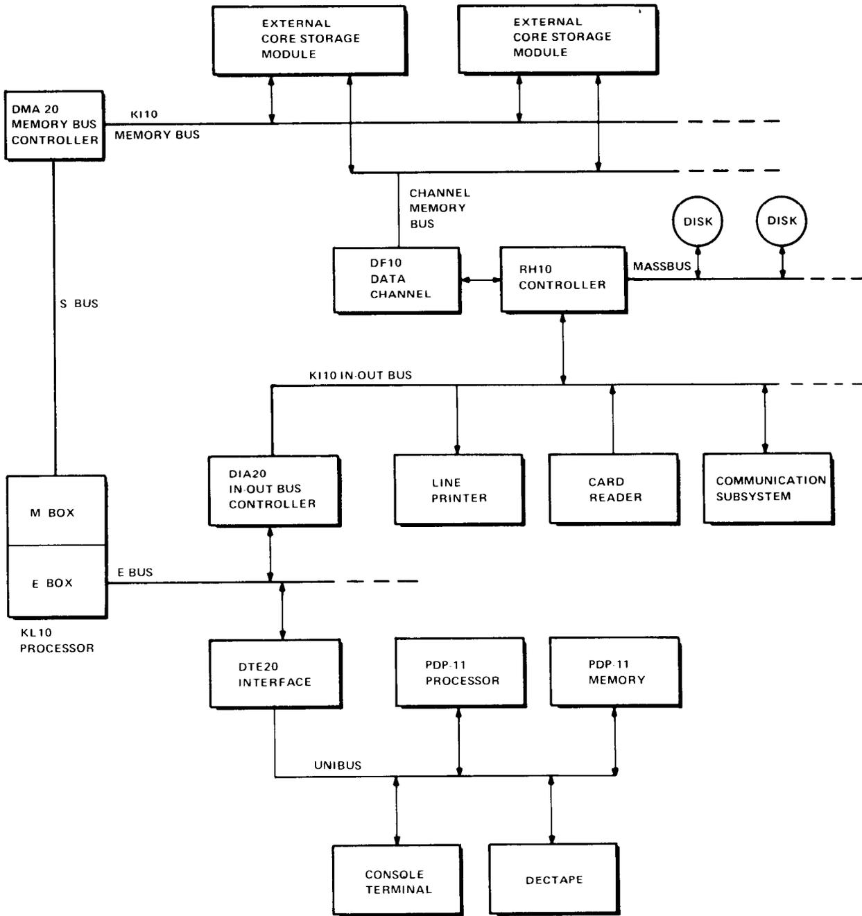
Figure 1.3: KL10 Processor Simplified
