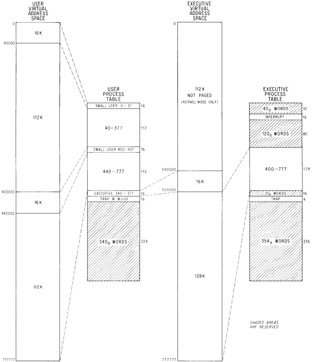
**Figure 5.2: Process Table Configuration**
