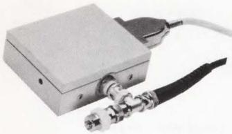
The ThinWire Ethernet Station Adapter (DESTA) converts a standard 15-pin A.U.I. station to ThinWire cabling. The station adapter can be attached to standard-cable Ethernet controllers, allowing UNIBUS, Q-bus, VAXBI, and other devices to connect to ThinWire. It also allows Digital's 802.3/Ethernet communications controllers and terminal servers to connect to ThinWire.
