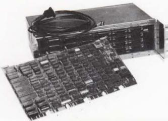
The DMZ32 is a 24-line asynchronous terminal interface for UNIBUS VAX computers running VMS or ULTRIX-32 operating system. It provides EIA-232-C compatibility and offers Direct Memory Access (DMA) output on all lines to optimize terminal to CPU I/O performance. The DMZ32 operates at speeds up to 19.2 Kb/s and features a distribution panel that can be located locally or remotely.
