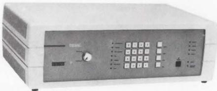
To help protect the security of network messages, Digital offers the DESNC Ethernet Enhanced Security System that selectively encrypts information across a network, without affecting other network nodes not requiring encryption.
