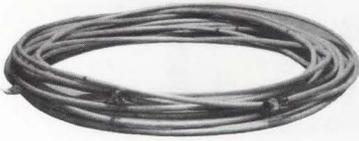
Standard baseband 802.3/Ethernet cable is the main transmission medium of a baseband network. The cable is available in four lengths (sections), which can be joined using barrel connectors to create segments up to 500 meters (1,640.5 feet) long. Local area networks can be extended beyond 500 meters by adding repeaters. Refer to "802.3/Ethernet Configuration Guidelines" in Appendix A for more detailed information.
