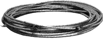
Ethernet baseband coaxial cable is the main transmission medium of an Ethernet baseband network. Coaxial cable is available in four standard lengths (sections). Sections can be joined using barrel connectors to create segments up to 500 meters (1,640 feet) long. Ethernet LANs can be extended beyond 500 meters by adding Ethernet Repeaters. Refer to Ethernet Configuration Guidelines in this section for more detailed information.
