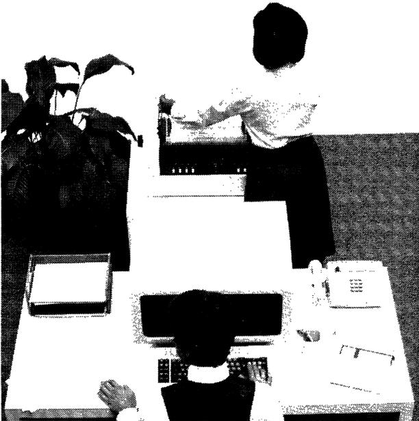
*The 5280 is IBM's diskette-based DDP system. A variety of communications features are available, including IBM 3270 emulation.*
