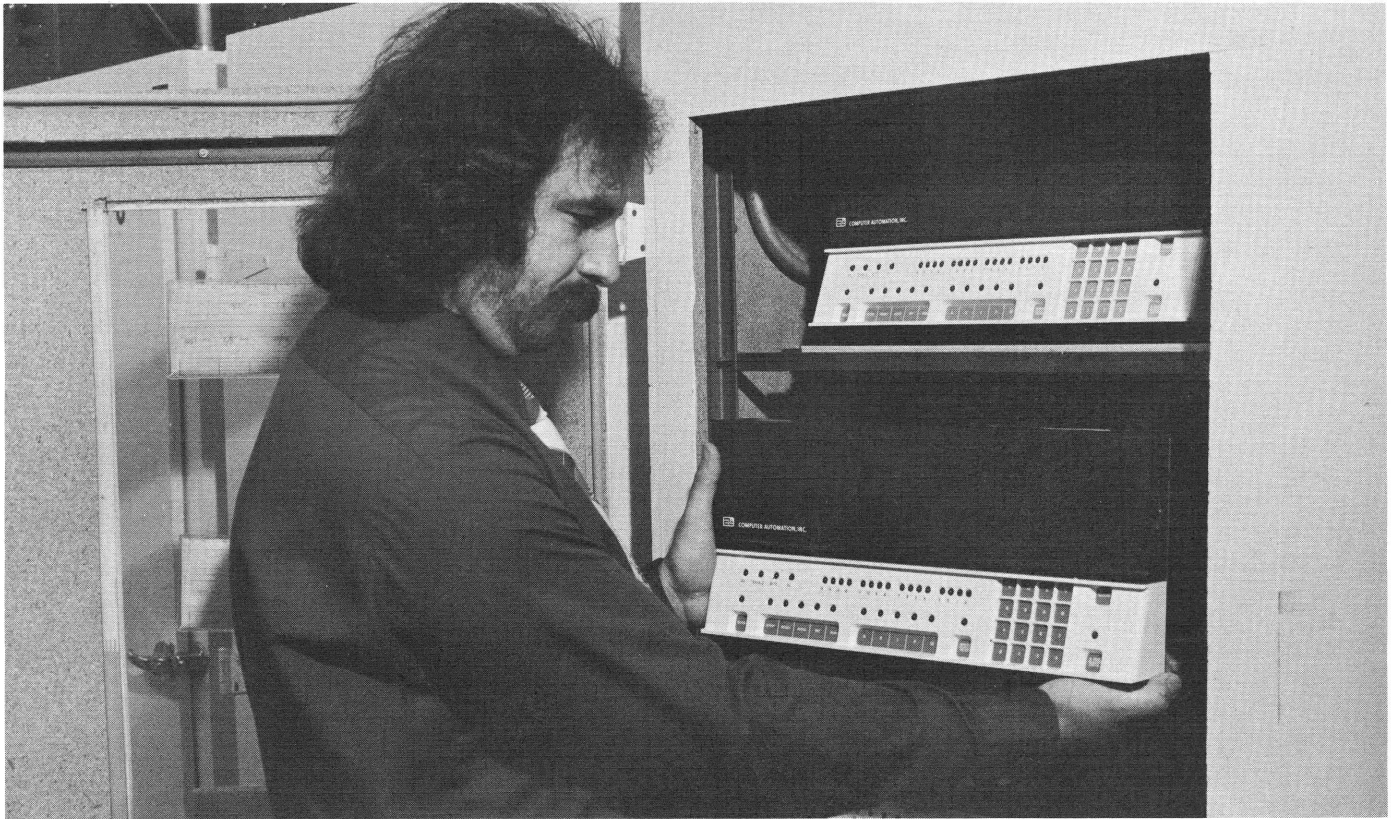
High temperature testing in an oven to verify long-term reliability. Test includes seventy-two hours at 50°C.
