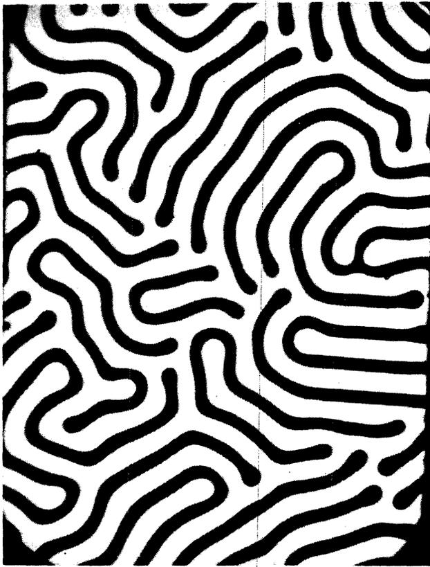
Figure 1—Strip domains, 1.5 mils in width, in a 1.7 mil thick platelet of  $\text{Sm}_{.65}\text{Tb}_{.35}\text{FeO}_3$  orthoferrite viewed by Faraday effect. Note the single wall domains. Bias field is zero
