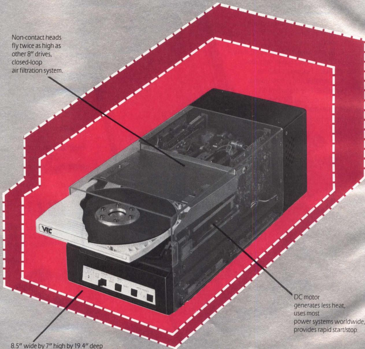
DC motor generates less heat, uses most power systems worldwide, provides rapid start/stop.
