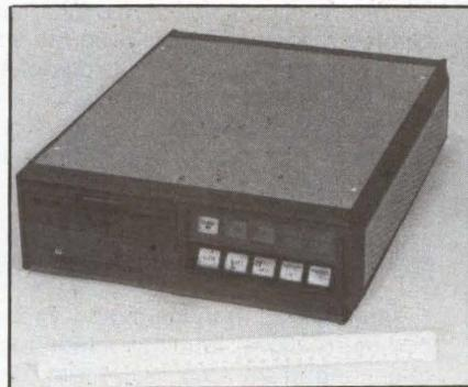
The Andromeda Systems 11/M12 incorporates an LSI-11/23 CPU, 256K bytes of RAM, a 10M-byte Winchester and a 512K-byte floppy disk drive in a 4-by-13-by-15-inch, 22½-pound package.
