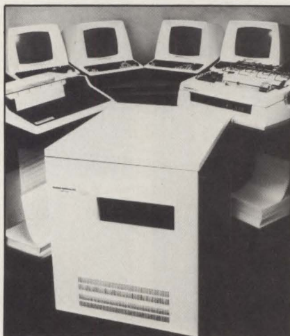
Pedestal enclosures are more compact and attractive than the high rack-style enclosures they replace in many small-business systems. From left to right, these systems from Apollo Computer, Symcro Systems and Micromation offer impressive power and look at home in an office.
