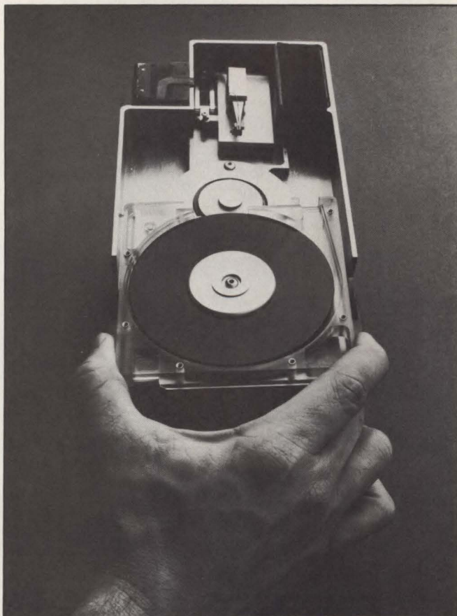
Fig. 1. The SyQuest SQ-360 3.9-in. Winchester drive uses 6.38M-byte removable cartridges, plugs into a Seagate ST-506 controller and is available in a fixed-media version. (Cutaway version shown.)
