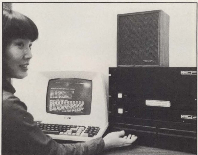
Fig. 1. National Semiconductor's Speech Editing System includes a Z80-based \mu c that supports 64K bytes of memory, two RS232 ports, dual double-density floppy-disk drives and the BLC-8281 speech processor board. Also included is the editor program and word library. Options for the MSC-6605 industrial system and Starplex development system are available.
