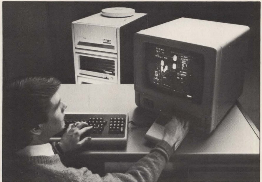
Digital Equipment Corp.'s VAX-11/730 32-bit minicomputer supports interactive graphics work stations using DEC's VS-11 terminal for engineering design, as well as educational and commercial applications with as many as 24 concurrent users. The VAX-11/730 uses 64K-bit RAM chips for a maximum memory of 5M bytes, and can be configured as a single-cabinet system with prices beginning at less than $50,000.
