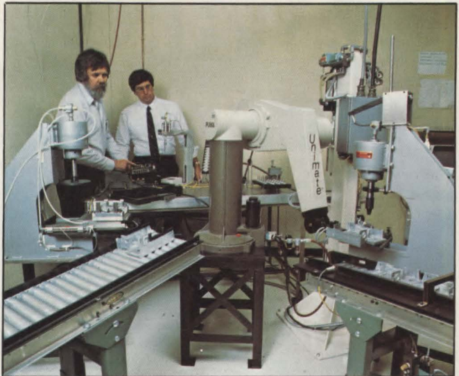
Shugart engineers Jack Brown (left) and Ron Albo, who pioneered the company's use of robotics, monitor the sub-assembly process of the SA410/460 family of 5¼-in. Minifloppy disk drives. Placement on an assembly line is scheduled for mid-1982.
