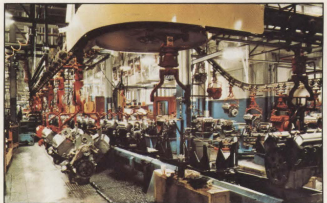
GM's production-monitoring system monitors more than 150 machines for fault detection and more than 3000 stations within machines for scheduled tool changes and quality-control checks.
