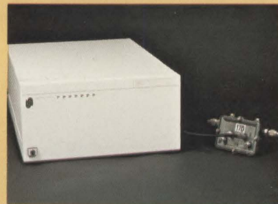
The Ungermann-Bass hardware for its broadband implementation of Net/One uses standard CATV industry components. Above is a network interface unit connected to a standard CATV tap.
