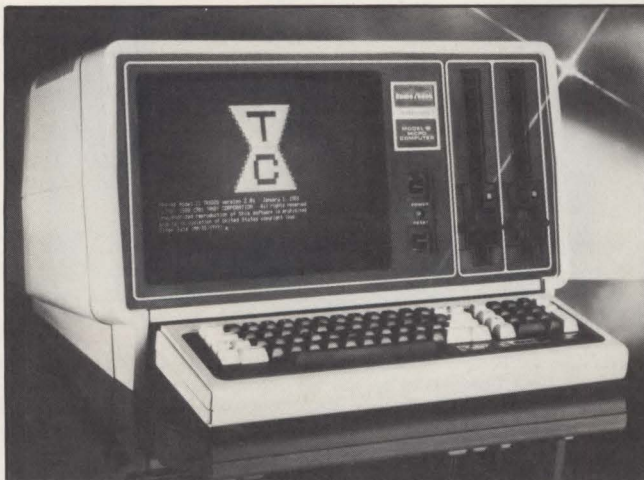
Desk-top small-business computers put processor, memory, off-line storage and display terminal on one work surface, often in the same enclosure. The dual processor (68000, Z80A) Radio Shack TRS-80 model 16 (left) incorporates two 8-in. diskette drives and supports two slave terminals. The Durango 900 features an integral Winchester disk and printer and supports as many as five concurrent users.
