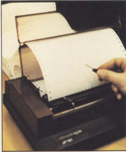
Olivetti OPE's ink-jet printer produces sparks through the ink cartridge (foreground). The JP 101 may be priced as low as $500.
