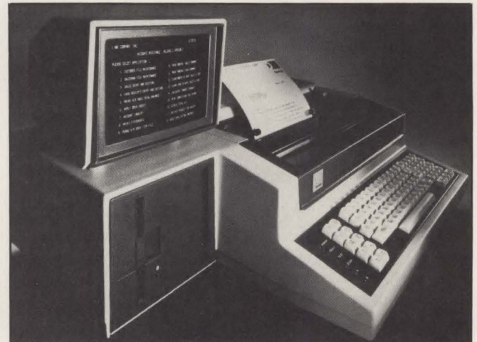
Desk-top small-business computers put processor, memory, off-line storage and display terminal on one work surface, often in the same enclosure. The dual processor (68000, Z80A) Radio Shack TRS-80 model 16 (left) incorporates two 8-in. diskette drives and supports two slave terminals. The Durango 900 features an integral Winchester disk and printer and supports as many as five concurrent users.
