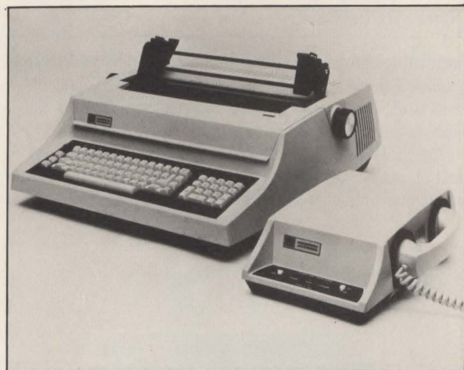
Desk-top teleprinters such as this Anderson Jacobson 860 are gaining popularity for office applications. With an accompanying modem the 860 communicates at 1200 bps and attains burst printing speeds of 140 cps.
