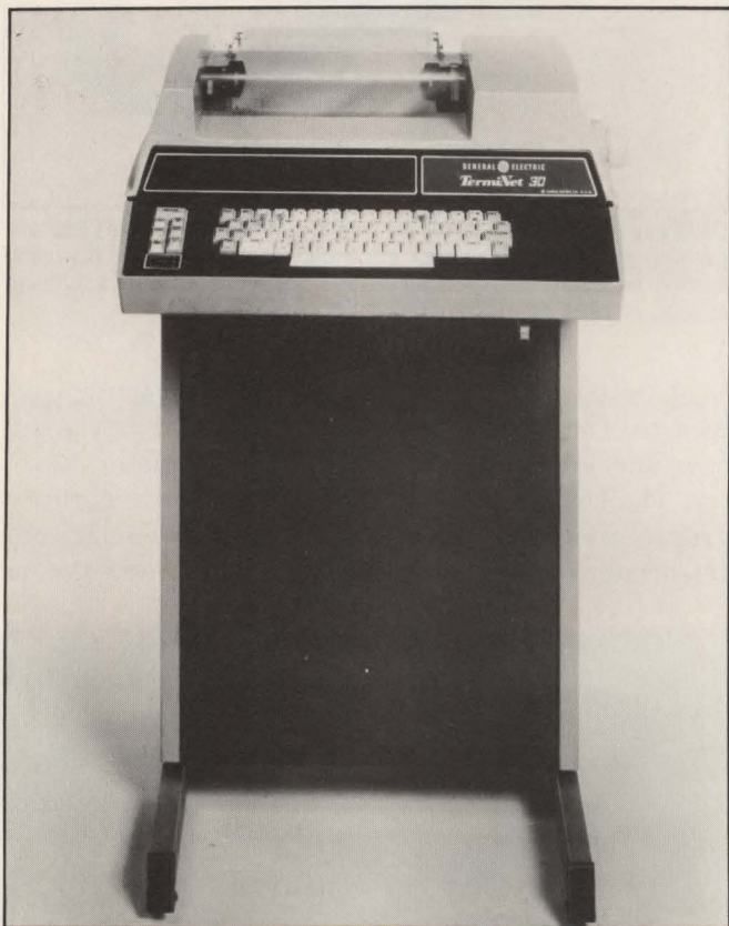
Pedestal-mounted teleprinters such as this General Electric unit are the most common physical teleprinter type. As brand identity gets harder to establish and office space gets more expensive, manufacturers will introduce more streamlined desk-top teleprinters.
