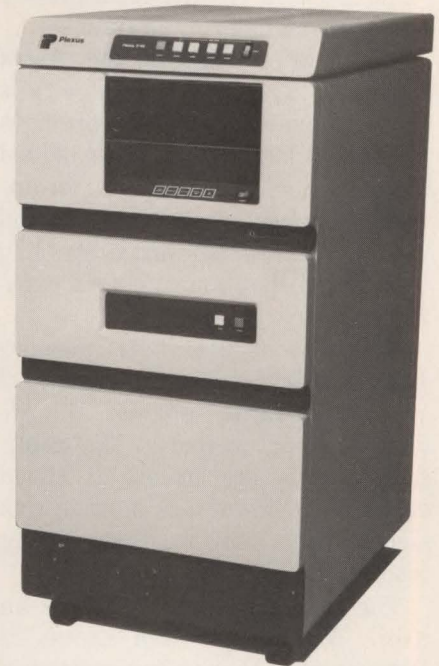
The Plexus small-business system incorporates a 16-bit Zilog Z8000 \mu p.
