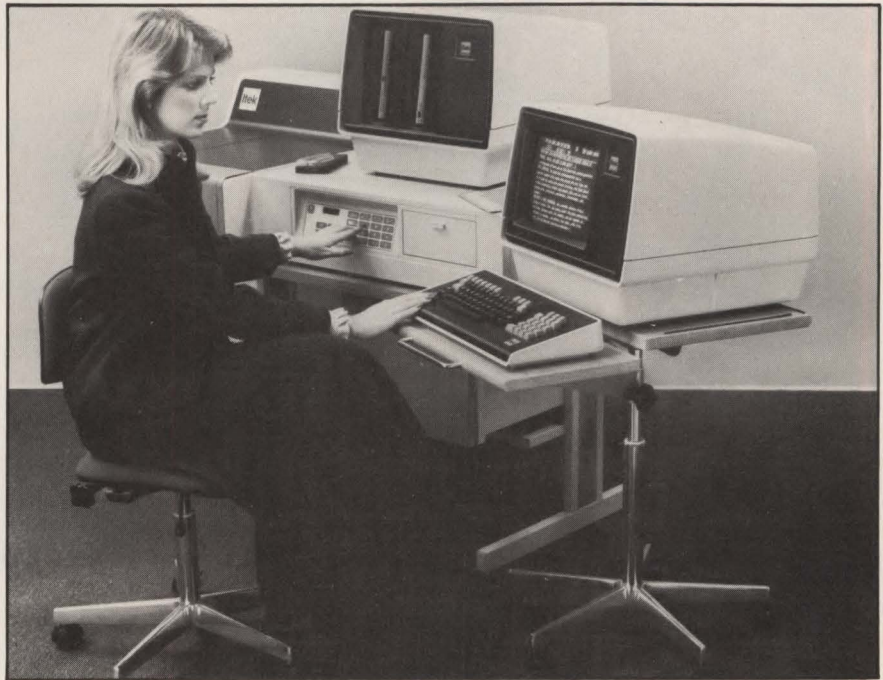
Itek's Quadritek 1400 and 1600 can queue nine phototypesetting jobs in memory for automatic printing. The screen indicates when a new job begins and informs the operator of required font changes.
