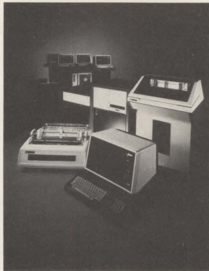
The Astra 270 is the new high end member of NEC Information Systems Inc.'s business computer line. The 270 can support as many as 16 work stations and support up to 256M bytes of disk storage.
