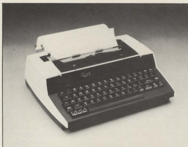
Portable teleprinters have given way to very portable teleprinters such as the Lexicon LEX-21 and the Quint Systems KSR-743. The Lexicon unit includes a telephone hookup and prints 40 columns while occupying the same desk space as a sheet of notebook paper. The Quint Systems unit prints full 80-character lines but doesn't fit in a briefcase.
