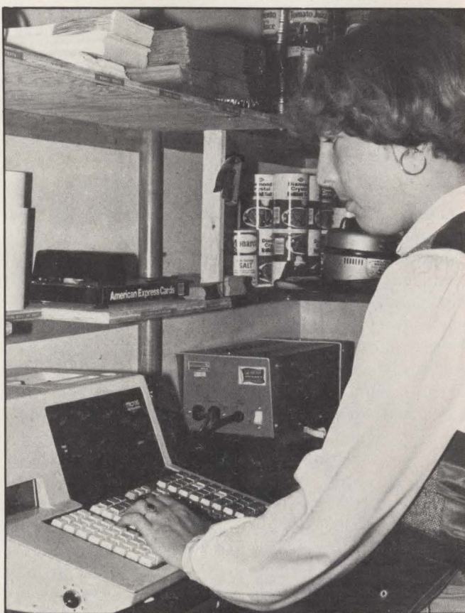
The MICROS electronic cash register is protected against noise and voltage fluctuations by regulator, in background.
