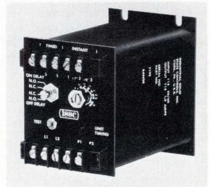
positive detent selector switch. Static output is rated for more than 100 million operations. The convertible unit also has an optically isolated ac control circuit with transient protection to 1,500 volts. Time ranges are from 0.02 to 2.6 seconds to 0.5 to 250 seconds.
