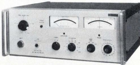
Our P2020 programmable Vector Voltmeter provides a wealth of information about signals and devices in the 1.5 MHz to 2.4 GHz frequency range. It measures insertion loss, gain, phase shift, group delay, scattering parameters—any measurements relying on accurate determinations of amplitude and phase.
