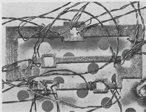
**Magnetic logic.** Four-stage logic structure (top) is building block of magnetic memory being developed for NASA. Lower photo shows how structure is wound.
