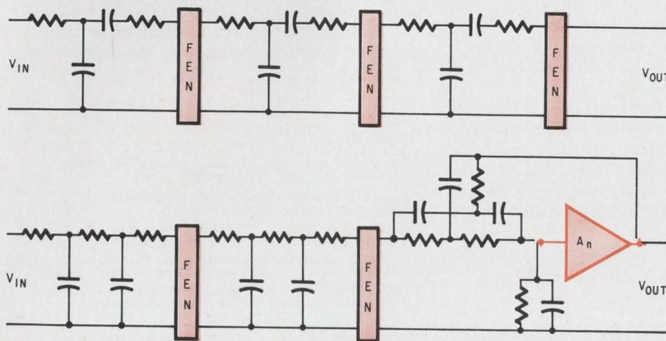
**FEN filter synthesis.** A sixth-order bandpass filter (top drawing) and a sixth-order elliptic lowpass filter (bottom drawing) are built with frequency emphasizing networks (FEN's). These units provide the RC networks with resonance properties similar to those of LC networks.
