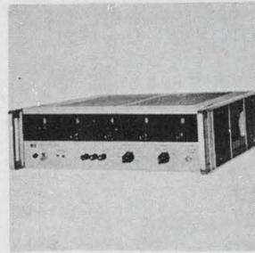
A-c calibrator 6921A has a 25-w output and supplies either a calibrated voltage or current to its load. The rms amplitude of its output is within  $\pm 0.25\%$  of selected value. The unit has 4 voltage ranges: 0 to 1.4, 14, 140, or 280 v rms. It has 5 current ranges: 0 to 1.4, 14, or 140 ma rms, or 0 to 1.4 or 5 amps rms. Hewlett-Packard Co., Locust Ave., Berkeley Heights, N.J. [366]
