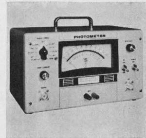
Solid state photometer, for use with photomultipliers, has an electrometer type current meter with a FET input for measuring currents from 300  $\mu$ a to 3 na. It has a 6-inch meter readout as well as a 5-v output with  $\pm 2\%$  accuracy. The built-in h-v supply is adjustable from 400 to 600 v and operates a load up to 2 ma. Schoeffel Instrument Corp. Westwood, N.J. [364]
