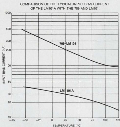
An order of magnitude improvement. The LM 101A has every advantage of the LM 101, but with 20 nA offset current and 100 nA bias current guaranteed over a  $-55^{\circ}$  to  $125^{\circ}\text{C}$  temperature range.
