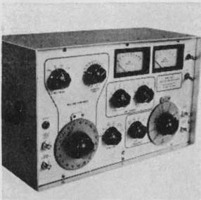
Power meter 6863-1 provides information on conducted EMI, displaying corrected EMI current, line impedance and calculated EMI power values. Current probes couple to the unknown impedance and measure impedance magnitudes from 0.3 to 1,000 ohms and phase angles  $\pm 180^\circ$  from 15 khz to 30 Mhz. Solar Electronics Co., 901 Highland Ave., Hollywood, Calif. [361]
