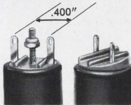
■ Here is the switch designed to meet your needs... to complement your package as "made-to-order"... at off-the-shelf prices! Controlled contact bounce... assured by the Clare PICOREED—"make" less than 500 microseconds and a consistent clean "break". Rugged... tested in accordance with MIL-STD-202C... meets shock to 35G... temperature -65°C to 85°C. Feather touch 4 oz. pressure... choice of lens shapes and colors certain to please.
