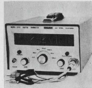
Seven ranges, covering resistances from 0.0001 ohm to 1 megohm, are offered in the model 8103-421 digital ohmmeter. One ohm minimum full scale is displayed as 1.0000 ohm to an accuracy of 0.1%. A large, illuminated digital readout provides a full 4-digit presentation with 10% over-ranging to the 5th digit. California Instruments Corp., 3511 Midway Dr., San Diego, Calif. [368]
