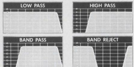
These responses are fully adjustable and may be set independently. This performance typifies the extra value you get from modern Krohn-Hite electronic instruments. Other values increase user confidence further by providing simpler, faster and lower-cost operation.
