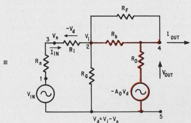
**Operating modes.** Terminal connections are indicated for both the inverting and noninverting modes of operation of an operational amplifier. At the right are the respective equivalent circuits for both modes.
