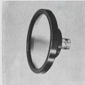
Silicon Schottky barrier photo-diode PIN-25 has an active area of  $7 \text{ cm}^2$ . Response time is 5 nsec or less. Capacitance at 90 v is less than  $100 \text{ pf}/\text{cm}^2$ . Linearity of response extends over 8 decades. Noise equivalent power is  $10^{-13} \text{ w}$  in a 1 hz bandwidth. Reverse leakage current is less than  $10^{-7} \text{ amps}/\text{cm}^2$ . United Detector Technology, 1732 21st St., Santa Monica, Calif. [441]
