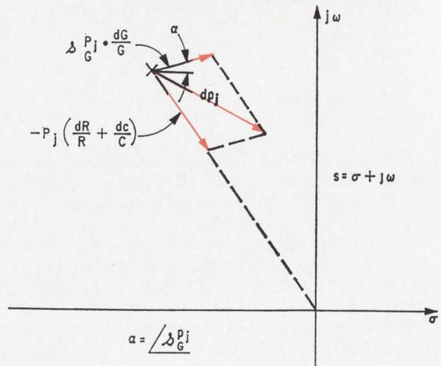
**Pole displacement.** The vector diagram represents the pole displacement for an active device  $G$  and resistors and capacitors. These passive components must track closely.
