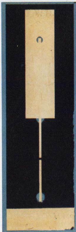
**Pulser.** This beam-lead microwave pluse generator was built at MIT.
