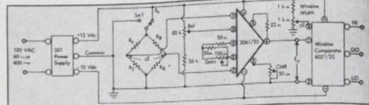
Figure 29. Resistor matching circuit, 1% to 0.1%.
