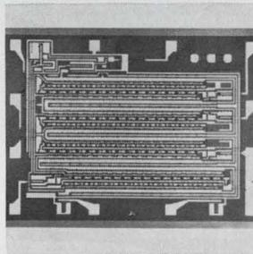
Two 64-bit shift registers, each with a single-phase clock, provide high speed operation from d-c to 1 Mhz and power consumption of less than 3 mw per bit. The MOS products are the 3305 quad 16-bit unit in a dual in-line package, and the 3306 dual 16-bit/single 32-bit unit in a TO-100 container. Fairchild Semiconductor, 313 Fairchild Dr., Mountain View, Calif. 04041. [442]
