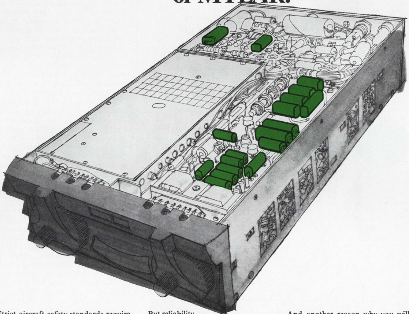
Strict aircraft safety standards require the most reliable navigation equipment available. That's why King Radio Corporation uses capacitors of MYLAR\* for their Distance Measuring Equipment. MYLAR can take temperature extremes from  $-60^{\circ}$  to  $+150^{\circ}\text{C}$ ; MYLAR remains constantly stable under humid conditions.
