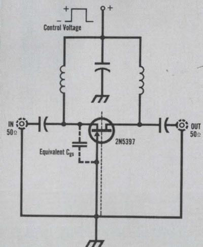
Turn this circuit off and the RF is shunted to ground through the FET's equivalent  $C_{gs}$ . OFF attenuation is greater than 65 dB for small signals. ON loss is less than 6 dB. With the 2N5397 these figures hold true around 200 MHz.
