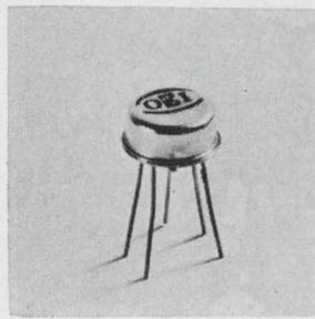
Monolithic voltage comparator model 5501 provides a maximum comparison error of  $\pm 1$  mv including gain and offset errors. Features include 80 db minimum voltage gain,  $\pm 25$  ma minimum output current,  $\pm 10 \mu\text{V}/^\circ\text{C}$  maximum input voltage drift. The unit is packaged in a 5-lead TO-5 low profile can. Price (1-9) is \$27 each. Optical Electronics Inc., Box 11140, Tucson 85706. [437]
