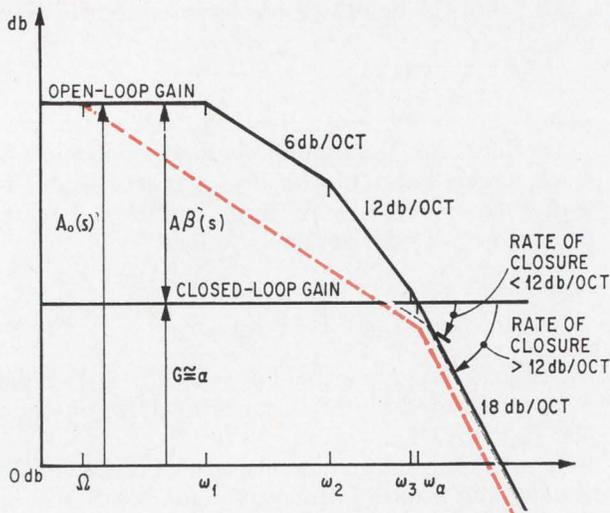
**Graphing the gains.** Bode plots for the open-loop and closed-loop gains of a typical operational amplifier. Dashed line represents the gain response of a modified op amp whose stability is assured by added RC components.
