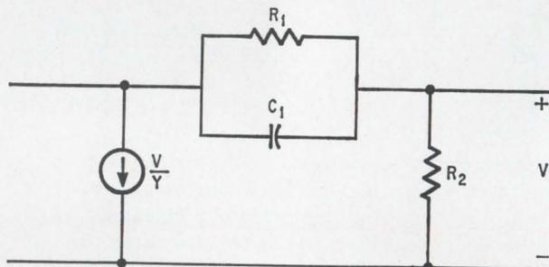
**Zero section.** A single transmission zero is produced in the right-half plane with this typical active-zero section.
