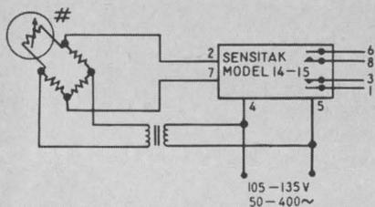
A four-arm resistance bridge may be used with a variety of transducers, to translate variations in temperature, pressure, etc., into proportional changes in resistance. The transducer, with or without auxiliary series resistance, forms one "leg" of the bridge. One or more of the other arms may be variable "set" type resistances for adjusting settings and ranges.
