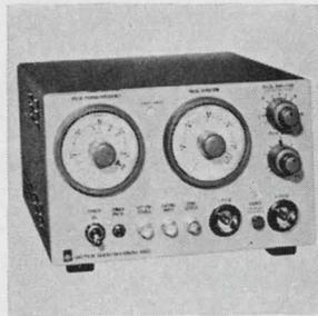
General purpose pulse generator type 1340 features wide ranges of pulse repetition frequency and pulse duration (both  $10^8/1$ ). Prf is as high as 20 Mhz or as low as 0.2 hz and pulse duration can be varied from 25 nsec to 2.5 sec. Ground-based positive and negative pulses are available simultaneously. Price \$395. General Radio Co., West Concord, Mass. 01781. [362]
