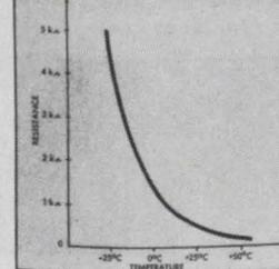
Figure 31. Typical Thermistor Response Curve—Resistance vs. Temperature.
