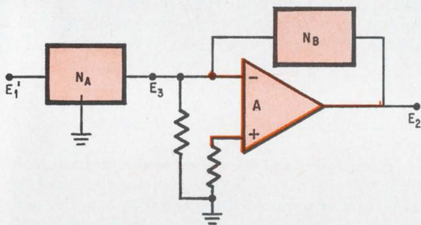
**Simultaneous operation.** A single operational amplifier is used to provide both the zeros and poles of a desired transfer function. It accomplishes this result through externally connected RC networks.
