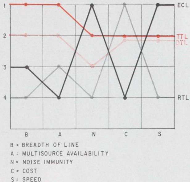
**Optimum choice.** TTL circuits have the best combination of characteristics desirable for a small computer.
