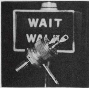
Bidirectional triode thyristors series BTV0400 handle up to 3,600 w and provide their own built-in electrical isolation. The case is fully insulated from the mounting stud. Five types are available for use with peak off-state voltages of 100 to 600 v. All types handle up to 10 amps of on-state rms current. Transistron Electronic Corp., 168 Albion St., Wakefield, Mass. [436]
