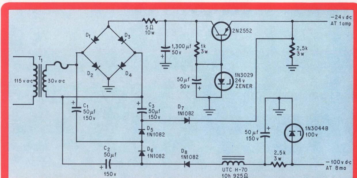
**Upstaging.** Capacitors  $C_1$ ,  $C_2$ , and  $C_3$  couple the transformer secondary to the multiplier diodes  $D_5$ ,  $D_6$ ,  $D_7$ , and  $D_8$ . Each multiplier stage will raise the no-load output voltage by about 1.4 times the rms voltage at the transformer output.
