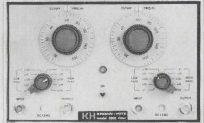
MODEL 3202 provides continuously adjustable high-pass, low-pass, bandpass and band-reject functions over frequency range of 20 Hz to 2 MHz. Two-channel bench unit shown; 5¼" x 8⅝" x 15¼"-rack units available.
