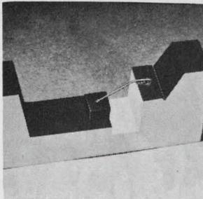
Schottky barrier mixer diode type CAY13A is a gallium arsenide device with an over-all noise figure of 6.5 db at X-band frequencies. Vswr is 2 max. I-f impedance is 350 ohms. Temperature range is  $-55^\circ$  to  $+155^\circ\text{C}$ . The unit is mounted on a ceramic carrier 1.9 x 0.8 x 0.35 mm. Metalized lands simplify bonding to substrate. Mullard Ltd., Mullard House, Torrington Place, London WC1. [440]
