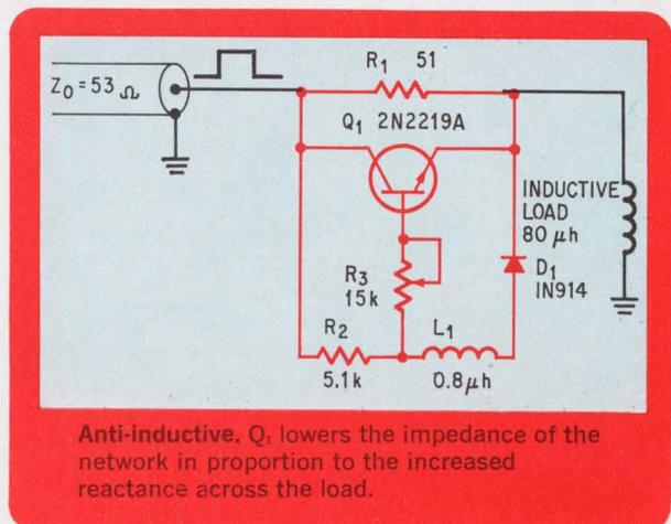
sistor circuit inserted between the cable and the load.
