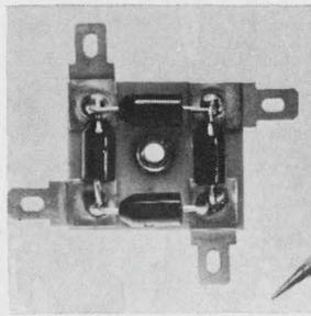
Industrial bridge rectifiers series B786-QD are now available with four quick-disconnect terminals that can be mounted simply and quickly into equipment by a 6-32 screw and push-on-terminals. The rectifiers use controlled avalanche devices. They are stocked in 2-amp and 4-amp types with piv up to 1,000 v. Solitron Devices Inc., 256 Oak Tree Road, Tappan, N.Y. 10983. [438]
