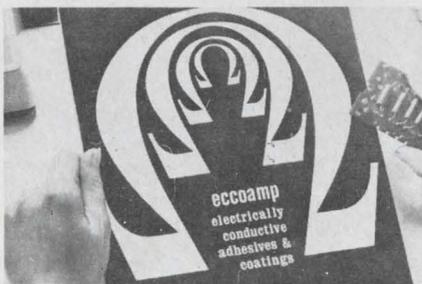
New four page folder describes materials from 0.0001 to 100 ohm-cm. Adhesive pastes to replace hot solder, thin liquids, silver lacquer in aerosol spray, glossy coatings, etc.
