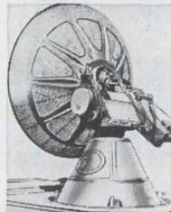
360 degree azimuth, 210 degree elevation sweep with better than 1 mil. accuracy. Missile velocity acceleration and slowing rates. Ampidyno and servo control. Will handle up to 20 ft. dish. Supplied complete with control chassis. In stock—immediate delivery. Used world over by NASA, USAF, MP-61-B, Type SCR-584. Nike Ajax mounts also in stock.
