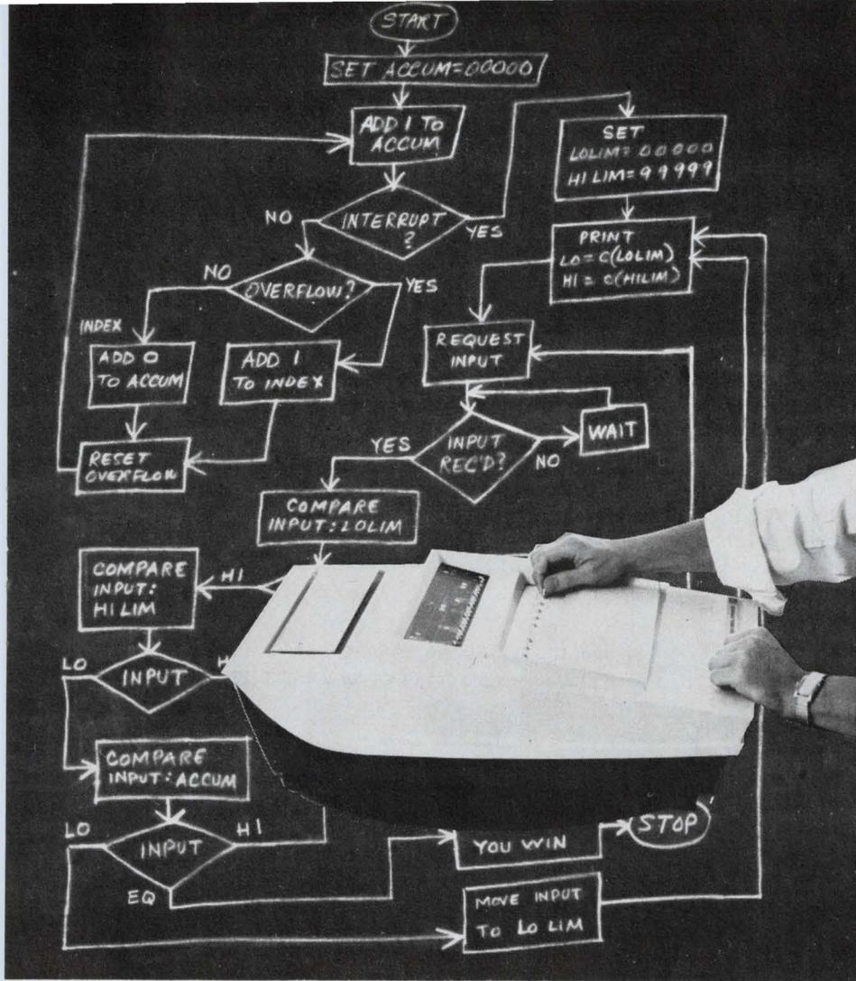
**Mighty midget.** Small though it is, the Nova has all the characteristics of a much larger computer, as the flow-chart in the background indicates. The chart itself represents the stored-program concept, the diamond-shaped decision blocks indicate conditional branches, and the operations at the upper left show how the program can modify itself. Strictly speaking, the read-only memory prevents direct modification, and current programming practice frowns on it, but the concept is still valid.
