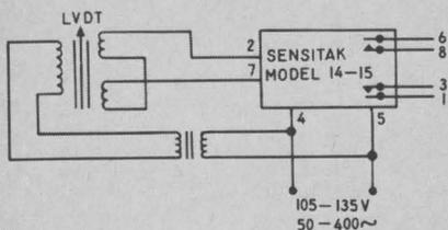
Linear variable differential transformers (LVDTs) can be used to provide the same type of signal system phase reversal.
