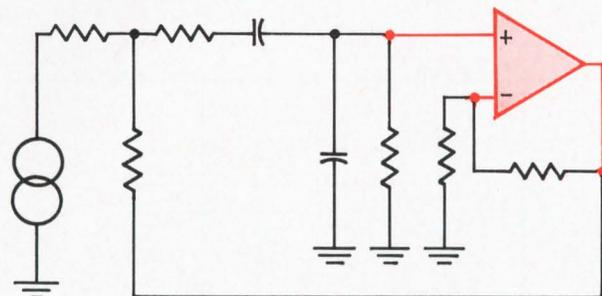
**Second-order transfer functions.** A typical circuit that can be used to produce second-order transfer functions is this one proposed by Sallen and Key. It assures stable frequency operation and is easily built with a small number of components.
