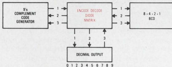
When one logic code must be converted to several other codes for processing, think diode matrices! Specify only *four* RM-84 diode matrices and form a 16 by 10 matrix array. Six conversions can be performed by this single bi-directional array... replacing approximately 80 logic elements.
