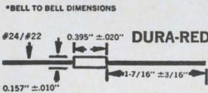
The "Dura-Red" is designed to MS-90537 with inductance range 0.10 $\mu$ h to 100,000 $\mu$ h with tolerance  $\pm 10\%$ . Stocked in 73 predesigned values.
