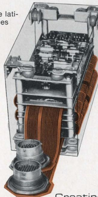
A unique 3-layer combination of flexible and rigid sections, the finished FLEXPRINT assembly in this airborne control system reduced volume 50%, with comparable savings in size and weight, installed faster and at lower cost. Wave soldering was made possible by careful material selection.
