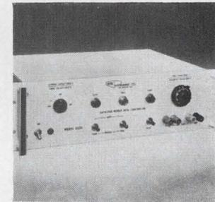
Capacitor winder auto-controller model 5332 provides continuous monitoring and control of final capacitor value during the manufacturing process. It is suited to high volume production of close tolerance metalized film or metal foil capacitors. Test frequency is 60 hz. Price is \$1,680; delivery, stock to 4 weeks. Micro Instrument Co., 12901 Crenshaw Blvd., Hawthorne, Calif. [428]
