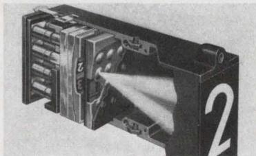
**Series 360H** Displays 2" high characters easily read from over 50'. Yet unit is just 3" H x 2" W x 7.75" D. New lens system provides bright, crisp display.
