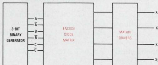
Suppose you need a three-bit binary output encoded into a four-bit binary shift code. Why use *five* AND gates and *four* OR gates? Simply combine these nine gate functions into *one* RM-30 six by eight diode matrix and save both time and money.
