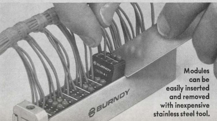
Modules can be easily inserted and removed with inexpensive stainless steel tool.
