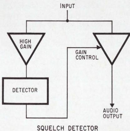
**Quiet.** The squelch detector shuts off the audio input when talking stops, in both the transmitting and receiving modes.
