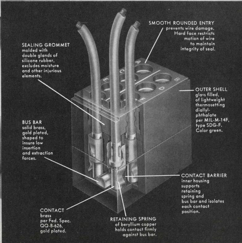
**SMOOTH ROUNDED ENTRY** prevents wire damage. Hard face restricts motion of wire to maintain integrity of seal.
