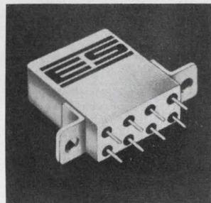
Military-type crystal can relay 79N is a low-cost, 2pdt dry circuit-to-3 amp unit that switches minimum current (100 ma to 0.5 amp) with the same reliability as dry circuit and load current. A new contact design permits the relay to meet a 100,000-cycle, no-failure test over its full range. Electronic Specialty Co., 19000 N.E. Sandy, Portland, Ore. 97200. [348]
