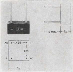
Single phase, silicon bridge rectifiers offer reduction in space requirements by handling max. power per unit size and withstanding high transient energy. High temperature capability, low leakage current and low forward voltage drop of these units with 6-amp current are offered in ratings of 50 to 1,200 v piv. Edal Industries Inc., 4 Short Beach Rd., East Haven, Conn. [436]
