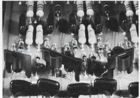
**Fan Top Dissipators for TO-5 and TO-18 cases** add almost nothing to board height. Don't need much room on the board either. Available for both metal and plastic cases. Spring fingers make installation simple. And Fan Tops cost just pennies.
