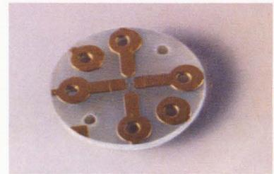
Included in L-band beamlead packages, dual Schottky diodes on fiberglass substrate (above) and matched pair (below).
