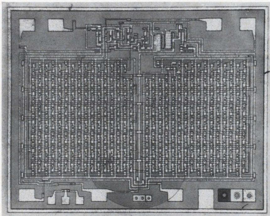
**Test case.** Experimental 128-bit recirculating shift register, made by TRW, has 780 metal oxide semiconductor transistors. It won't be put on market.
