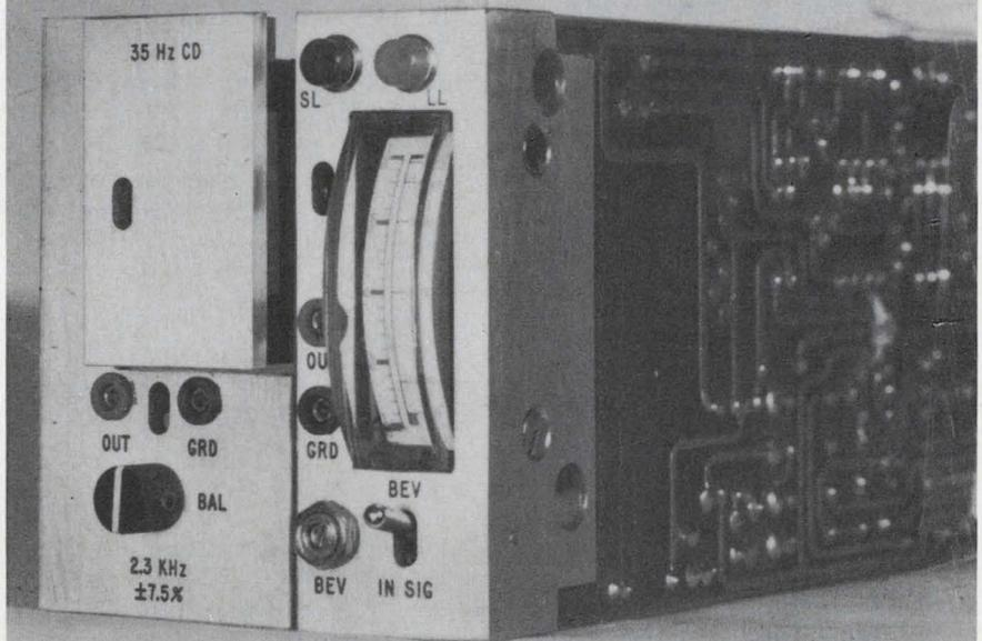
The SCD-5 phase lock loop discriminator represents the latest addition to the DEI F/M product line. Switchable loop filter bandwidths for operation within MI's of one and five are supplied as standard filters. Constant time delay input filter provides data distortion less than 0.3% at DR = 5.
