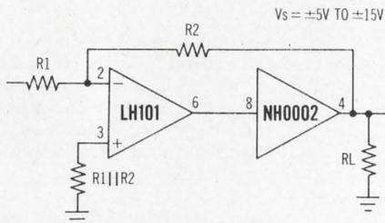
The NH0002 is something else. It has an output current of  $\pm 300mA$  into a load of  $50\Omega$ . The NH0002 buffer is useful in the loop in all your high current op amp applications. The price is \$20.00 in 100 to 999 quantities.
