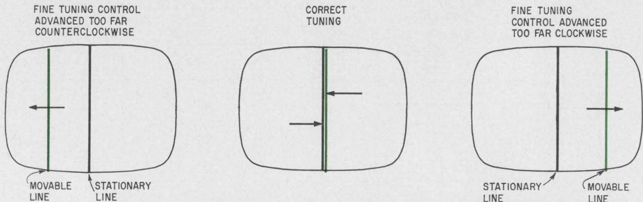
**Visual fine tuning.** This variation by Westinghouse on a basic AFT circuit presents an on-screen indication of the degree of mistuning by the spacing between movable and stationary lines.
