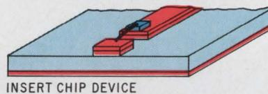
must be active. Round sections of ferrite are simply placed in holes in the ceramic board as an alternative to all-ferrite microstrip. A third approach, ferrite disks on top of the ceramic, is favored when mounting holes can't be drilled. But this requires an extra bonding step.
