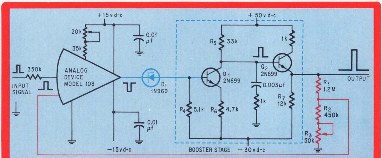
**Zener leverage.** Small voltage changes in the output of the operational amplifier cause wide swings in the collector voltage of  $Q_1$ , and thus in the emitter of  $Q_2$ . Resistor  $R_7$  gives the boosted voltage the capability of driving low-impedance inputs.
