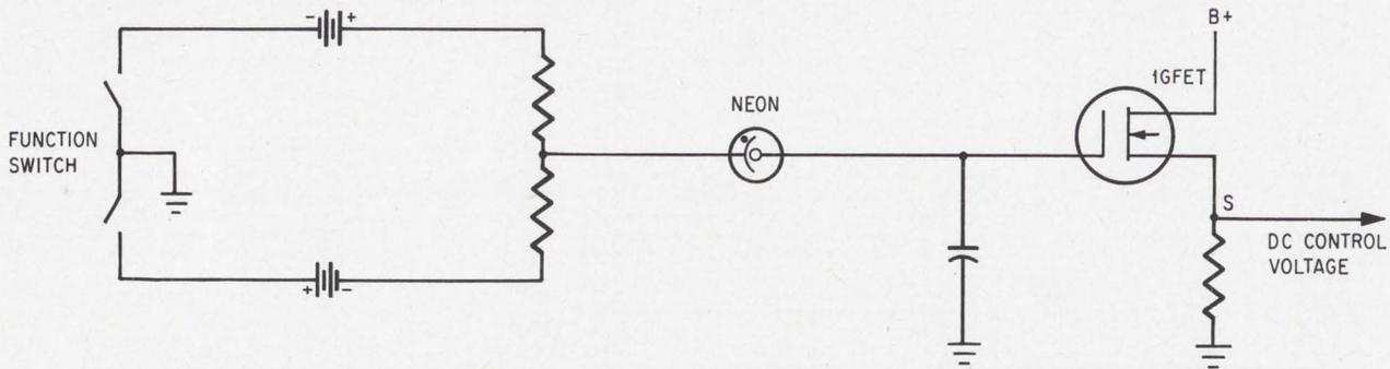
**Remote control circuit.** Continuously variable functions are handled by a "memory" module developed by Motorola. The neon lamp serves to isolate the timing elements from external circuitry when a function switch is open.
