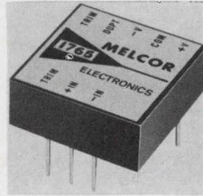
Low drift, FET input operational amplifier 1755 features high common mode rejection ratio, high power bandwidth, and high slew rate. It can be operated over a wide range of supply voltages and has an output swing of up to  $\pm 21$  v. Applications include control instrumentation and data logging. Melcor Electronics Corp., 1750 New Highway, Farmingdale, N.Y. [384]
