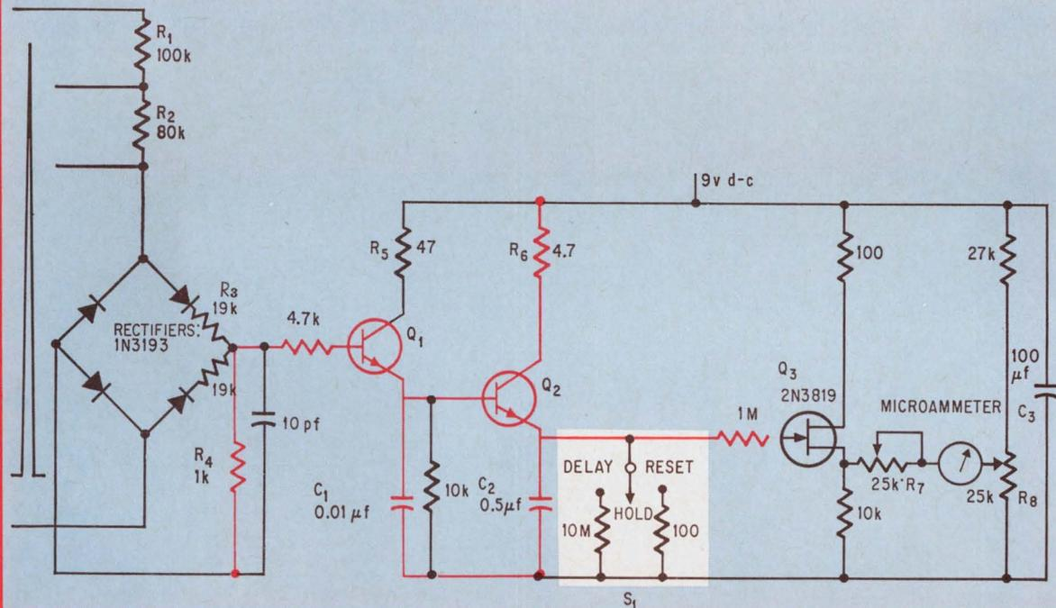
**Added strength.** The divided portion of a transient voltage increases in power as it moves from  $R_4$  in the divider to capacitors  $C_1$  and  $C_2$ . The high input impedance of the FET allows  $C_2$  to remain charged during the reading.
