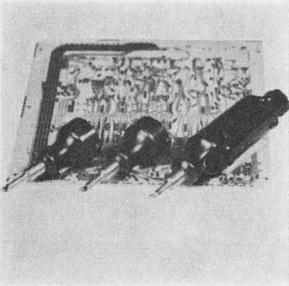
Air operated cut and bend tool BP-1 Bend Eze features interchangeable heads, which meet the circuit board at either 20, 30, or 45°. The quill has a max. o-d of 3/16 in. diameter. The tool will take an existing component wire, cut it off, and lay it flat to the circuit board to military specifications. Price is \$99.50. Henry Mann Co., Box 37, Cornwells Heights, Pa. 19020. [421]
