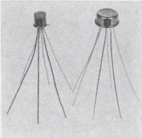
Small signal pnp and npn differential amplifier transistors will track over a wide temperature range with temperature coefficients as low as  $3\mu\text{v}/^\circ\text{C}$ . They offer matched gains to within 3%, voltages up to 120 v, leakage less than 20 pa and low level gains typically 100. They come in TO-78 and TO-71 cases. Solitron Devices Inc., 1177 Blue Heron Blvd., Riviera Beach, Fla. [440]
