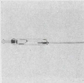
Reed switch WR126 is a mercury wet, spst Form A type that is bounce free and completely stable in its contact resistance and pull-in sensitivity. It is 1.63 in. in over-all length and 0.130 in. in diameter. Contact ratings are 50 w (d-c resistive), 50 va (a-c resistive). It switches 1 amp at 50 v d-c for  $50 \times 10^6$  operations. Gordos Corp., 250 Glenwood Ave., Bloomfield, N.J. 07003. [347]
