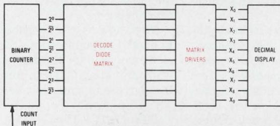
Why use ten logic gate packages to decode from binary to decimal for display read-out? Use only *two* RM-84 eight by five diode matrices. It makes no difference what weighted binary code you are working with, Radiation diode matrices can be easily customized to match.
