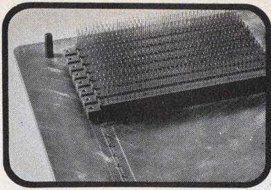
Alignment holes in HW Series connectors are polarized for fast, sure alignment.
