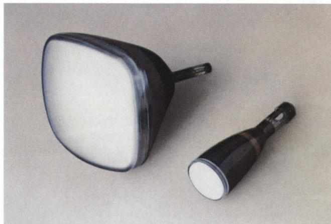
21" SC-4876 and 5" SC-4689 are typical of the range of multicolor tube types that can be made. Each is capable of displaying alphanumeric or analog information in 4 or more colors simultaneously, using a single gun.
