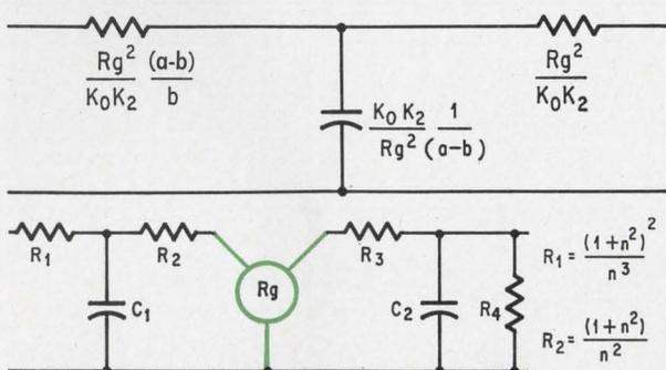
**Active-filter design.** Starting with a single gyrator flanked by two RC networks, the designer assumes the left one to be a T network. By synthesizing the over-all transfer function, he finds that the right network can be a series-parallel RC circuit. Values for all elements are shown on the drawing.
