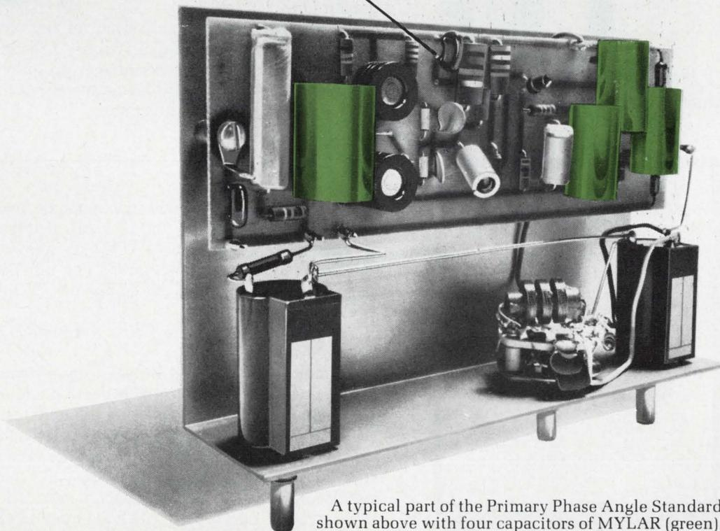
A typical part of the Primary Phase Angle Standard shown above with four capacitors of MYLAR (green).
