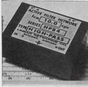
Active high-pass filter networks series HPB4 features the 4-pole Butterworth gain and phase frequency response characteristic. Attenuation over the operating temperature range of  $-40^{\circ}$  to  $+71^{\circ}$  C is  $3\pm 0.5$  db at cutoff frequency and  $24\pm 2$  db at one-half cutoff frequency. Standard cutoff frequencies are from 1 to 1,000 hz. Linear Networks Co., Box 1103, Bozeman, Mont. [383]
