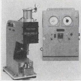
Intermediate-range ultrasonic welder W-150-AW is designed to meet thin metal joining requirements as found in the capacitor industry. Aluminum and tantalum foils are joined to respective tabs with bar-type welds quickly and easily. No external heat is introduced in the process, which eliminates oxide formation. Sonobond Corp., 310 E. Rosedale Ave., West Chester, Pa. [422]
