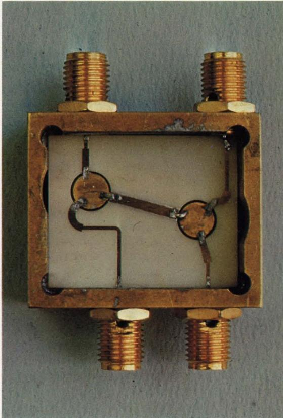
**Circulator.** This X-band, four-port circulator uses 20-mil thick alumina and handles 500 watts peak with an 0.8 db transmission loss and 0.4 db reception loss. The circuit provides 40 db isolation over a 25% bandwidth. Magnets are located below the ferrite disks, which are mounted in holes in the ceramic. The ceramic is 1 inch square. Thick-film techniques are used.
