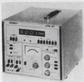
Utility test set UTS-41 combines capabilities of as many as 6 different devices (power supply, alternator, rheostat, counter and/or timer) formerly required for use such as calibration and performance testing of under- and over-voltage frequency relays. It features 100 msec power frequency measurements. Darcy Industries Inc., 1723 Cloverfield Blvd., Santa Monica, Calif. [365]
