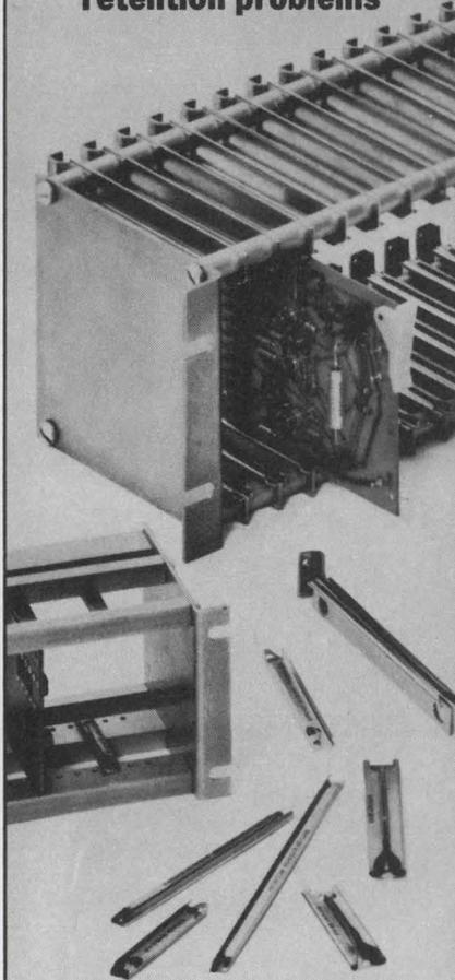
There are sizes and styles of Birtcher PCB-TAINERS to solve every printed circuit board retention problem. Simple installation. Provides excellent retention under severe shock and vibration and an excellent ground and thermal path. Made from steel or beryllium copper in choice of MIL Spec finishes. Or let Birtcher build the entire assembly. You'll be pleasantly surprised by the low cost and fast delivery.
