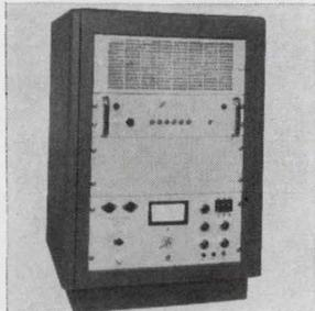
Amplifier system M402 is suitable for driving broadband antennas in testing rfi susceptibility. Capable of pumping 50 to 100 w of power into a 50-ohm load over a frequency range of 10 khz to 220 Mhz (nearly 15 octaves), without tuning or bandswitching, it creates the fields required by MIL-STD-826A and -461. Instruments for Industry Inc., 151 Toledo St., Farmingdale, N.Y. [382]
