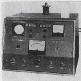
Corona test set model 4074 incorporates a Hypot with a 10 kv at 0.25 kva maximum continuously variable corona-free output. Output voltage crest factor is better than 5%. The corona detector consists of a scope with a verticle amplifier sensitivity of 3 mv/in. at max. gain. The 4074 is priced at \$2,250. Associated Research Inc., 3777 W. Belmont Ave., Chicago. [366]
