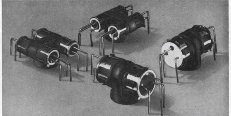
**Cool off microcircuit devices** with a choice of four new dissipator/retainers. Example: with natural convection, a typical microcircuit device dissipates 1.8 watts with case temperature rise of 103°C. Add IERC's model LBOC2-61B and retainer and you dissipate 5 watts with the same case temperature rise. Retainer-clip may also be used alone to mount package to conduction plane.
