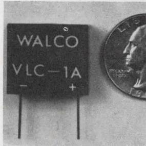
Solid state variable current limiters allow the user to obtain a continuously variable constant current with a ranging capability of 50 to 1. Current limiting capabilities are from 1  $\mu$ a to 50 ma with input ranges from 5 to 35 v. Level stability is an order of magnitude better than that of fixed current limiters. Wall Electronics Co., 3821 Commercial N.E., Albuquerque, N.M. [342]
