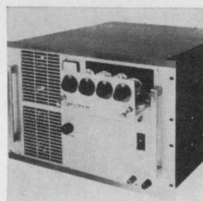
Power source model 1000 delivers 0-1,000 va, single phase. Units may be stacked for 2- or 3-phase operation. The basic unit is a power amplifier that will accept any of 40 interchangeable plug-in oscillator modules. These provide fixed or variable output ranging from 45 hz to 5 khz accurate from  $\pm 0.1$  to  $\pm 0.0001\%$ . Elgar Corp., 8046 Engineer Road, San Diego, Calif. [386]
