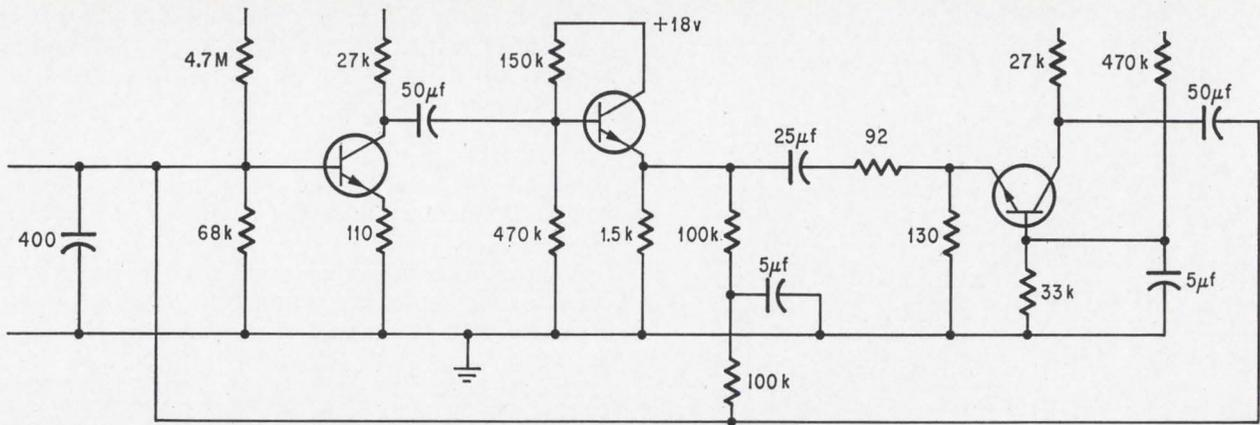
**Practical gyrator.** Three transistors are used to form this gyrator circuit. Gyration resistance is 118 ohms, and remains constant within a frequency range of nearly 3 decades. Entire network behaves as a passive device and neither consumes or adds signal energy. In the transmitting direction the circuit has a maximum insertion loss of 1.5 db; isolating direction 60 db.
