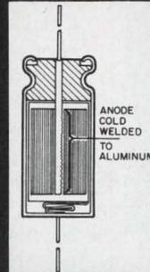
Featuring the exclusive CDE continuous cold weld connection of section to rod...insuring superior mechanical and electrical reliability. With far superior ESR to Temperature characteristics.
