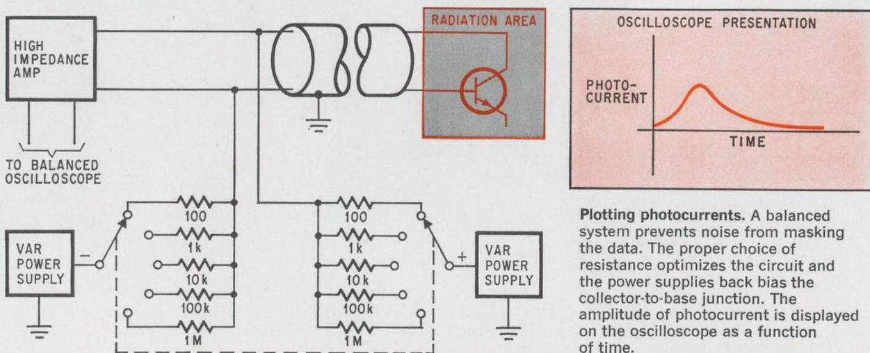
**Plotting photocurrents.** A balanced system prevents noise from masking the data. The proper choice of resistance optimizes the circuit and the power supplies back bias the collector-to-base junction. The amplitude of photocurrent is displayed on the oscilloscope as a function of time.
