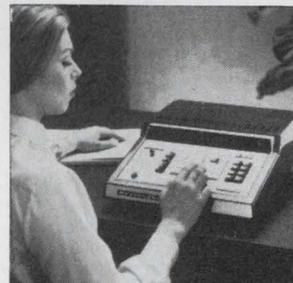
Electronic calculators series C3000 bring silent, instantaneous computing power to the desk top. The C3350, top model in a series of four, which can automatically extract a square root in less than  $\frac{1}{3}$  sec, features 2 independent core storage memories. Each memory provides 16 digit, 8 decimal storage capacity with minus total. Burroughs Corp., Detroit, Mich. 48232 [388]
