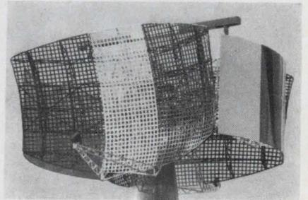
**Back to back.** Telefunken's upcoming air traffic control radar uses a pair of reflectors, each 29½ by 48½ feet. Waveguides aren't mounted on this unit, a model for wind-tunnel tests.
