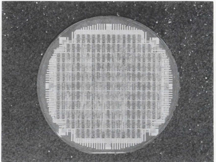
**Wire at will.** Large-scale array with third-level metalization from Texas Instruments was produced with discretionary wiring techniques.
