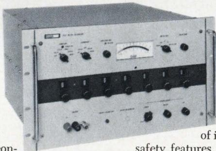
can operate the instrument simply and quickly. Dial up any parameter without range change or switching. We've put in a full complement of interlocks and other safety features so neither you nor the instruments under test are in danger. The 760A can easily be used by unskilled operators to calibrate virtually all multi-range, multi-function instruments.
