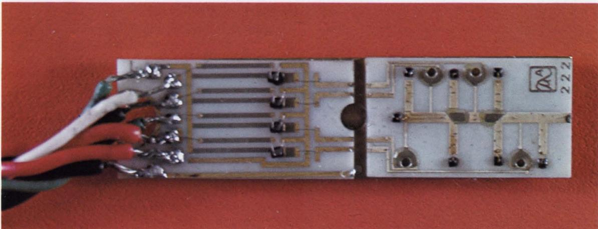
**Phase shifter.** A Ku-band, four-bit phase shifter, measuring only 0.220 by 1 inch, has two 20-mil alumina boards mounted on a supporting plate—one board for the thick-film phase shifter, and the other for the thin-film driver for the p-i-n diodes. The diodes are located at ends of various length impedance stubs, which act as transformers to translate the diode reactance to achieve the desired phase shift. The power level is 100 watts peak.
