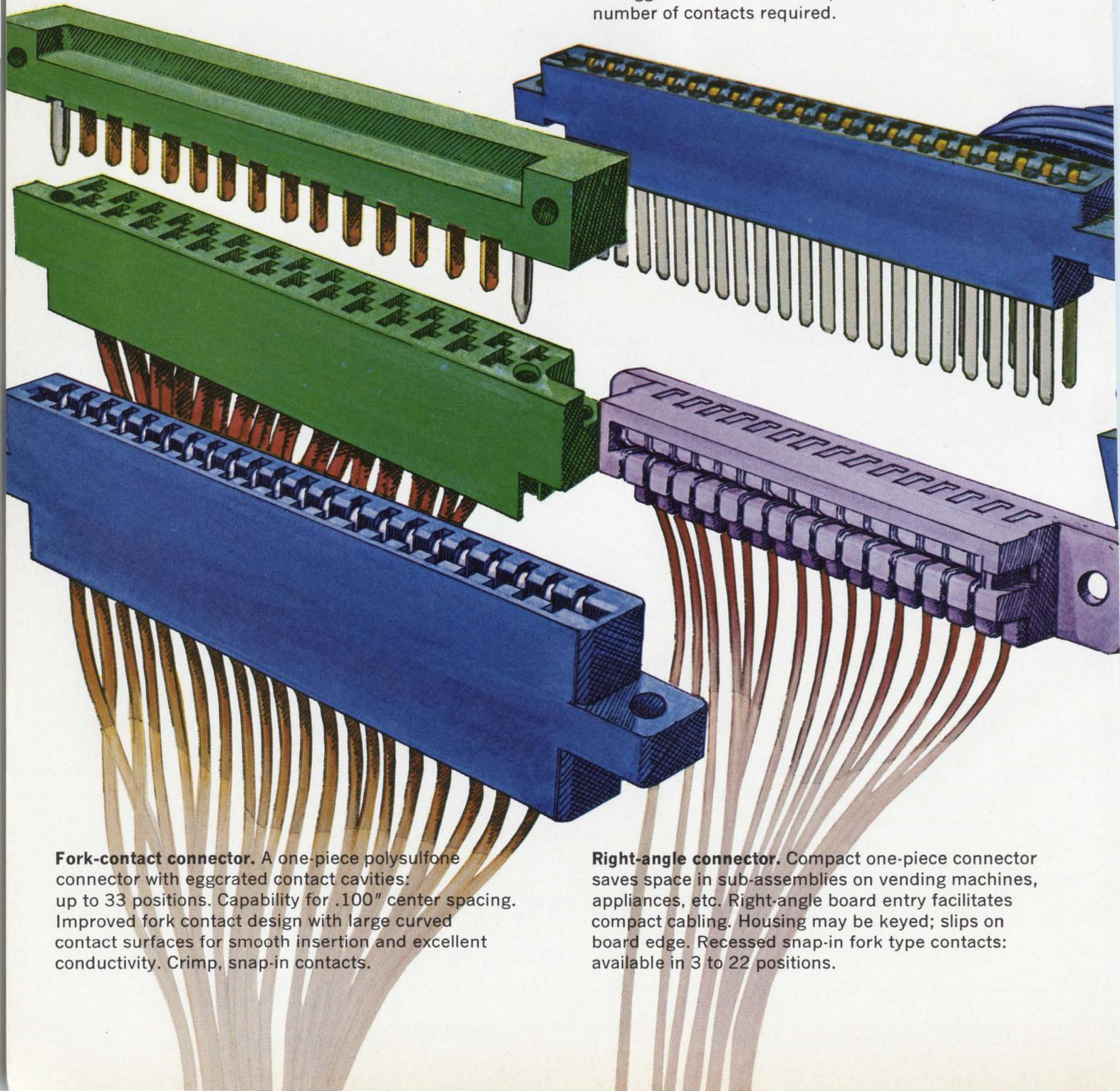
**Fork-contact connector.** A one-piece polysulfone connector with eggcrated contact cavities; up to 33 positions. Capability for .100" center spacing. Improved fork contact design with large curved contact surfaces for smooth insertion and excellent conductivity. Crimp, snap-in contacts.
