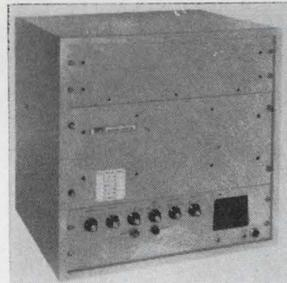
SSB transceiver CA-34 features automatic programming with simplified controls for ease of operation by nontechnical personnel. It is a 100-w unit developed as a multipurpose radio communications system for aviation ground stations. It will operate efficiently under temperature extremes from  $-30^{\circ}$  to  $+65^{\circ}$ C. Communication Associates Inc., 1208 Third Ave., New Hyde Park, N.Y. [387]
