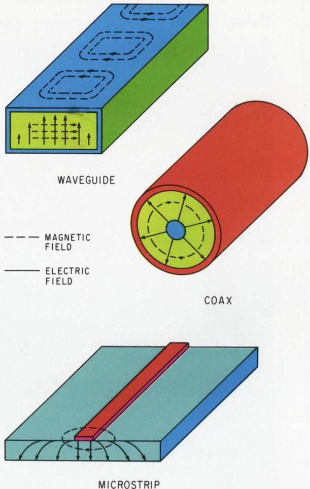
**Transmission modes.** Propagation of electromagnetic energy assumes distinct field patterns. Transverse electric mode is shown for waveguide structure, and transverse electromagnetic modes for coaxial configuration, and IC microstrip.
