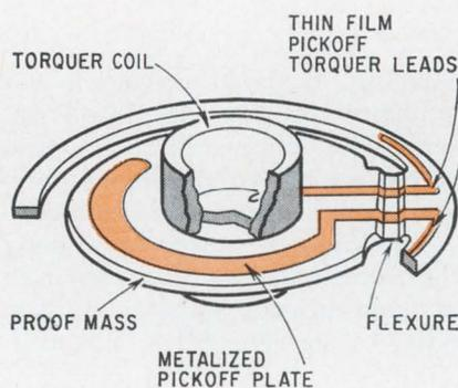
**One piece.** Proof mass, flexure and support are chemically milled from a single quartz blank.
