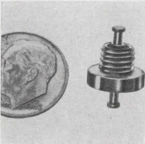
EMC/RFI filters series 75000, for use in low voltage circuits, combine high capacitance-low voltage ceramic capacitors and high current inductors in a sealed device. Measuring 0.400 in. diameter x 0.370 or 0.100 in. body length, units have max. d-c resistance at 25°C of 0.1 or 0.01 ohm, respectively. Electro Materials Corp., 11620 Sorrento Valley Rd., San Diego, Calif. [341]
