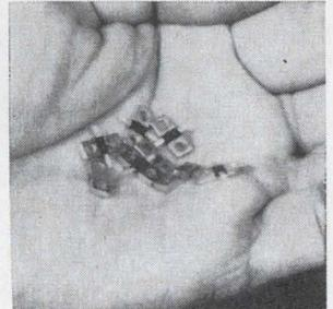
P-i-n diode 5082-3040 can be used as a modulator or switch over a wide range of microwave frequencies—from vhf up to Ku band. It behaves as a smooth section of 50-ohm transmission line when the diode is unbiased or reverse-biased. Insertion loss is typically 0.4 db at X-band; vswr, less than 1.6 up to 18 Ghz. Hewlett-Packard Co., 1501 Page Mill Rd., Palo Alto, Calif. [443]
