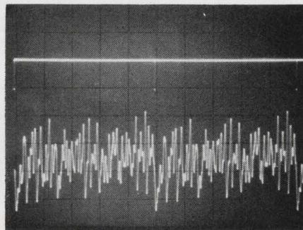
The Hewlett-Packard 3722A Noise Generator now lets you harness noise so that it becomes a defined and calibrated input to your system. It allows you to synthesize and reproduce at will noise signals of constant noise power with a probability density function (pdf) in the classical Gaussian construction. This unique new instrument uses computer techniques to synthesize noise patterns of selectable length that are thoroughly defined and repeatable.
