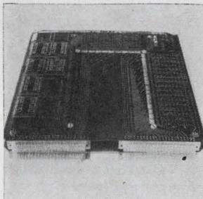
Ferrite memory core stack has a capability of 4,096 words with 16 or 18 bits/word and a fast 1.2  $\mu$ sec cycle time. It was developed for small-scale, low-cost, computers intended for process control data terminal applications. It contains 65,536 individual 30-mil ferrite cores in the 16 bit/word configuration. Data-Ram Corp., Route 206, Princeton, N.J. 08540. [385]
