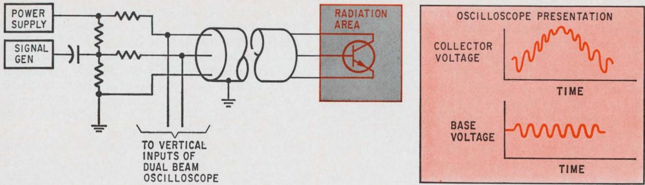
**Gain degradation.** A transistor biased by external resistors and a power supply is driven by a sine-wave generator. By dividing the collector voltage by the base voltage, an engineer can find the gain degradation of a transistor. How fast and to what degree the transistor recovers are determined from the amplitude of the collector waveform as a function of time.
