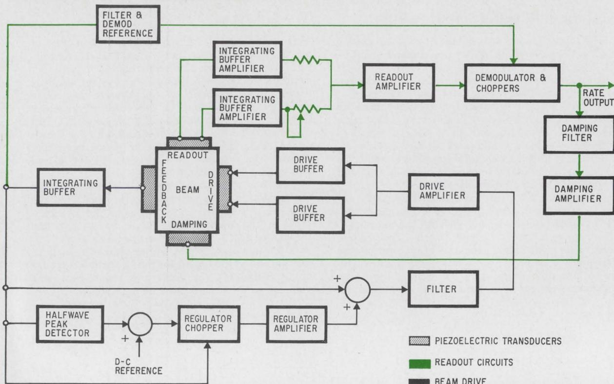
**Two major functions.** Beam drive and readout mechanization requires only dc power for the sensor and uses minimum power because of the resonant operation.
