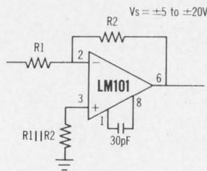
Old faithful LM101 is both general purpose and no-sweat in operation. It's short-circuit proof and has a large differential input voltage allowance. Moreover, frequency compensation is simple, and there is no latch-up problem. The price is \$40.00 in 100 to 999 quantities. (There is also a commercial version, the LM201, priced at \$8.80.)
