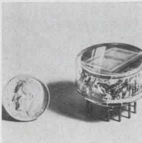
The Digivac readout tube has 7 triodes with a common anode and cathode sealed in a rugged glass envelope. The anode of each triode forms a segment about 8 mm x 1 mm which is covered with fluorescent material that ensures high visibility characters. Viewing distance is over 40 ft.; viewing angle, 150°. Tung-Sol Div., Wagner Electric Corp., 1 Summer Ave., Newark, N.J. [346]
