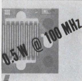
Medium power n-channel junction FET's U221 and U222 are for power amplifiers to 30 Mhz and vhf oscillators to 100 Mhz. High 50-v breakdown permits operation from supply voltages up to 28 v with over 30 db power gain at 30 Mhz. Power output at 100 Mhz is 0.5 w. Units are mounted on high dissipation TO-5 headers. Siliconix Inc., 1140 W. Evelyn Ave., Sunnyvale, Calif. [441]
