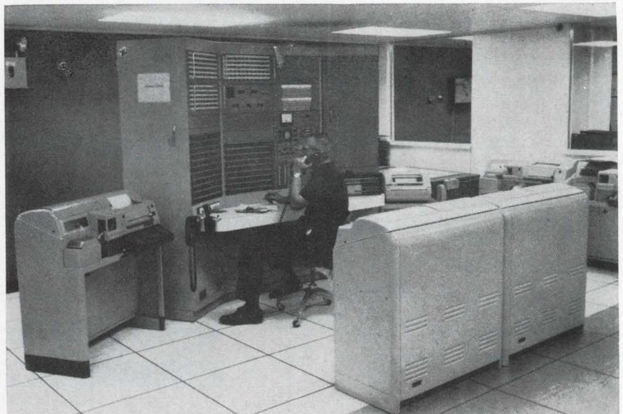
What's going on—and in? Technical Control center monitors operation of the processors and peripheral equipment.
