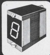
Displays 0-9 numerals by illuminating miniature lamps. Combination of lamps can be controlled with a matrix circuit (not supplied). Decimal points can be used as colon when 2 units are placed together. Indicator provides high illumination with a low voltage and current. Colored filters available. 6 & 12V. Figures 25/32" high. 20,000 hr. bulb life.
