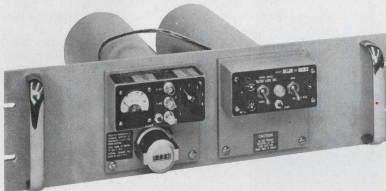
The heart of the 2.5C Frequency Standard is a selected crystal that is monitored continuously for 90 days under precisely-controlled conditions to insure an absolutely minimum drift rate.
