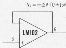
The LM102 voltage follower is the first monolithic amplifier that has combined low input current with high speed. Slew rate is  $10V/\mu s$ . The maximum input current is an incredible  $10nA$ . Input currents better than  $10nA$  at  $125^\circ C$  are guaranteed. The price: \$30.00 each in 100 to 999 quantities. The  $-25^\circ C$  to  $+85^\circ C$  LM202 is priced at \$12.00, LM302 commercial at \$5.40.
