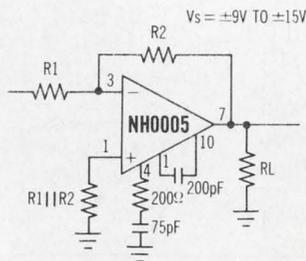
When we say high output current, we *mean* high. The output current on this, the NH0005, is  $\pm 50mA$  into a  $100\Omega$  load. The price in 100 to 999 quantities is \$45.00. And there's a commercial version, the NH0005C, priced at \$22.50.
