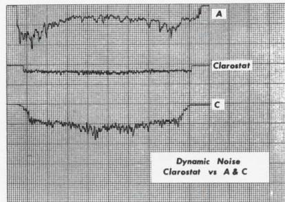
A measurement of any spurious variation in the electrical output not present in the input, noise is expressed as a percentage of the total resistance measured over the nominal effective rotation.
