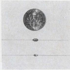
Doubly hermetically sealed glass diodes meet MIL-S-19500 specs. The 5-w diode has a 0.085 in. max. body diameter and a 0.155 in. length. The 750-mw unit has a 0.065 in. body diameter and a 0.100 in. length. They range from 2 nsec, 2 pf switching devices to 1,000-v rectifiers, including zeners from 5.5 v up. Micro Semiconductor Corp., Playa Court, Culver City, Calif. [438]
