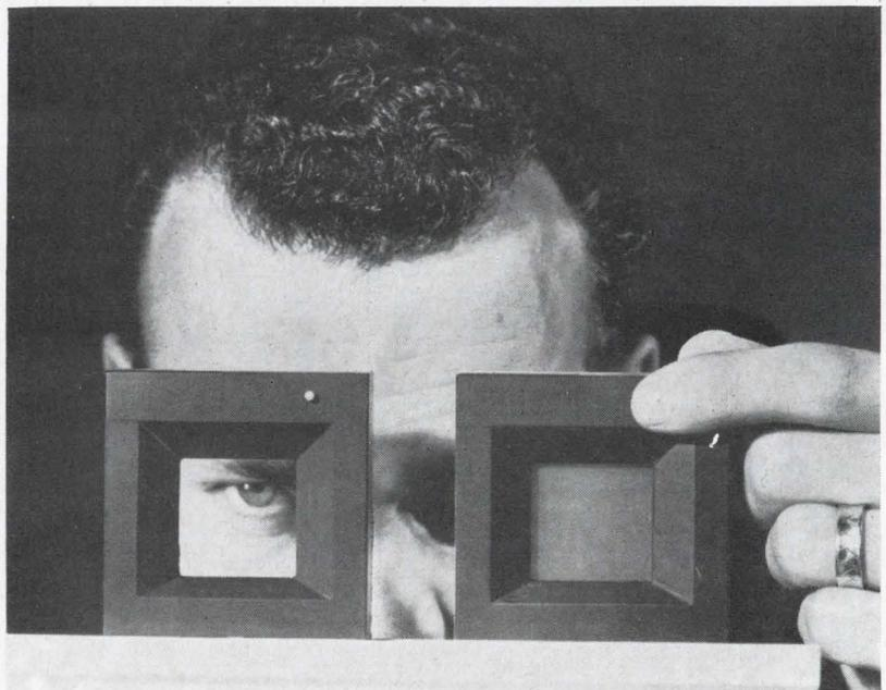
**Afterglow.** RCA's liquid crystal display becomes frosted, right, when voltage is applied. Company says the thin-screen display, which uses low power and ambient light and is compatible with IC's, will be competitive with vacuum-tube displays. Thus far, RCA has an alpha-numeric display and a light shutter. Other firms are also doing work in this area, including Sylvania and the Marks Polarized Corp. [Electronics, July 25, 1966, p. 41].
