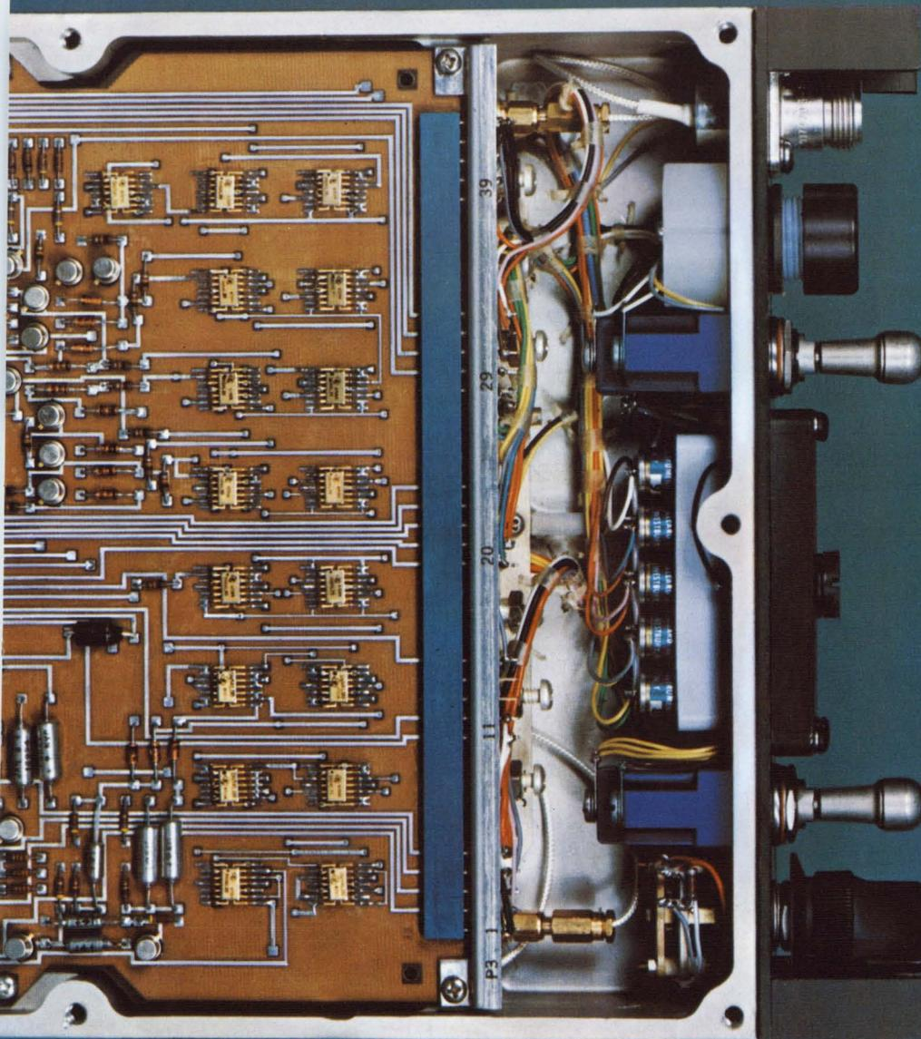
Linking soldier to satellite . . . that's the job for these seventeen low-power TTL integrated circuits from Texas Instruments. They help form the "intelligence center" for an *Alert Receiver Terminal* — part of an advanced new communications system being developed by Collins Radio Company for the Tri-Service TacSatCom (Tactical Satellite Communications) program. Prototype receiver terminals are being built for the U. S. Army under a Tri-Service contract administered by the U. S.
