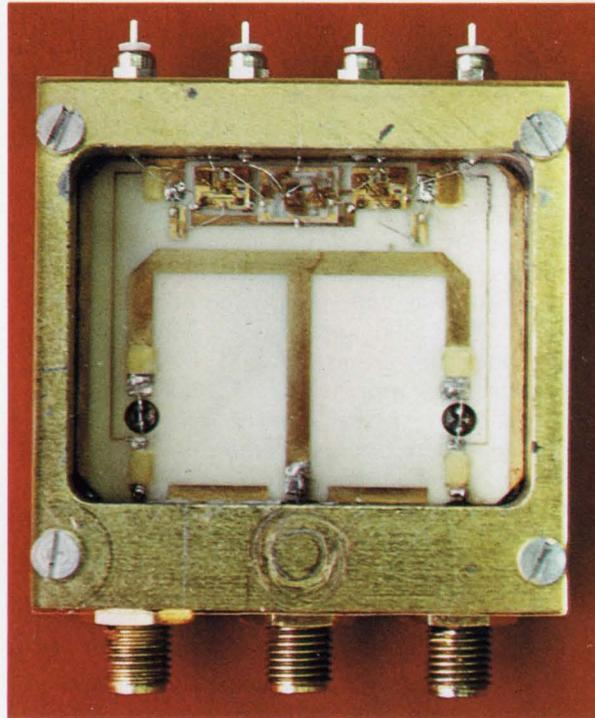
**Switch.** An L-band single-pole, double-throw switch handles 2 kilowatts peak power at 0.001 duty cycle. The alumina board measures 2 by 2 inches and is 60 mils thick. Conductors are deposited on the board by thick-film process. Signal input is through the center conductor and shunt diodes direct the signal to one of the two output arms. Insertion loss is 0.5 db.
