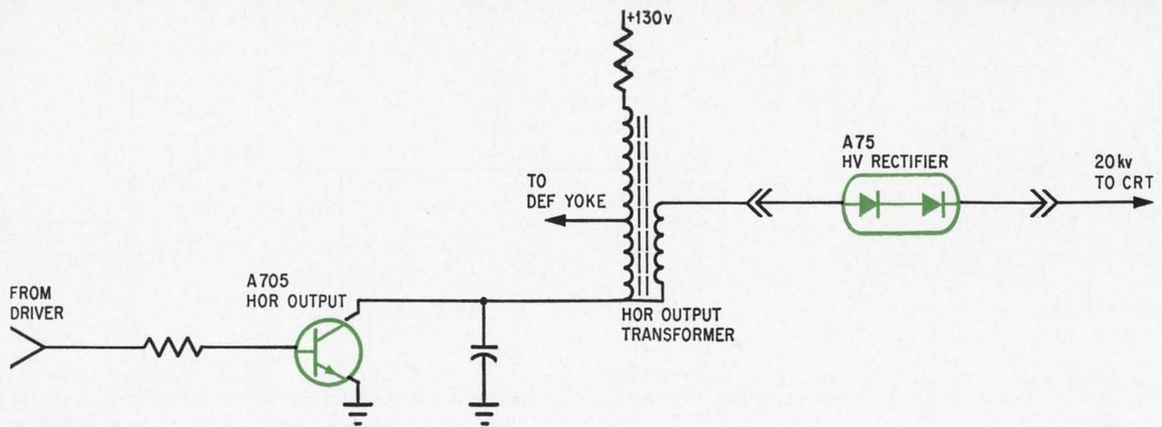
**Solid state deflection.** Horizontal deflection circuit developed by Amperex for a large-screen, all-transistor black-and-white tv sets operates directly from off-the-line 130-volt power supply.
