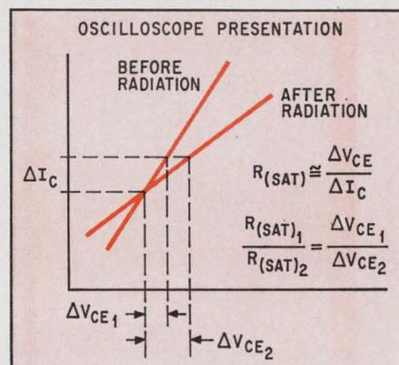
**Saturation resistance.** A sawtooth generator supplies a ramp voltage that is applied simultaneously to the transistor—biased into saturation—and the horizontal-drive circuits of an oscilloscope. A plot of the change in collector-to-emitter voltage for a fixed change in collector current indicates the value of saturation resistance.
