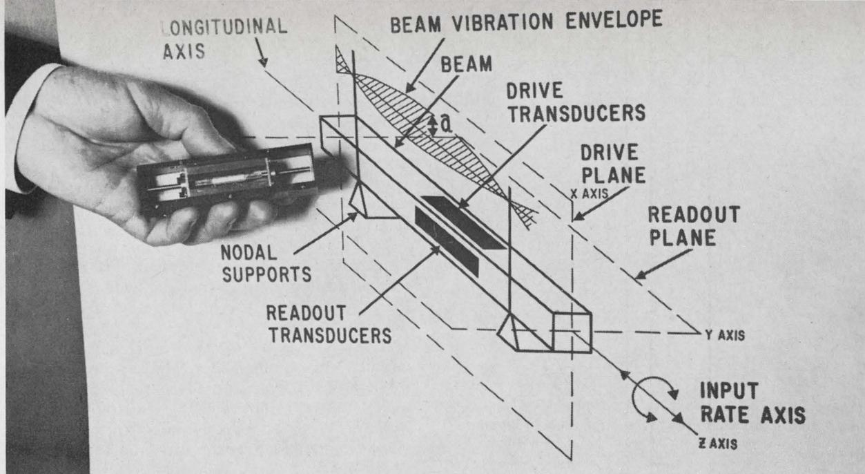
**Basic sense.** Sinusoidally vibrating metal beam senses changes in angular input applied about its long axis. The Coriolis effect sets up a sinusoidal signal at the readout transducer that is a function of the input rate.
