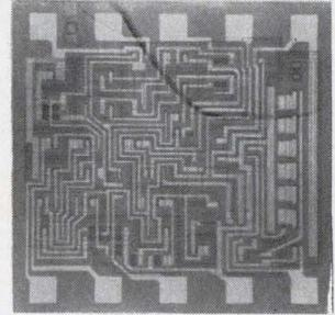
Differential preamplifier model  $\mu$ A727 is a monolithic linear circuit featuring input impedance of 300 megohms over a  $-55^\circ$  to  $+125^\circ\text{C}$  temperature range. Input offset voltage drift is  $0.3\mu\text{v}/^\circ\text{C}$ ; input offset current drift, 2 pa/ $^\circ\text{C}$ ; input offset current, 2 na; long term drift,  $5\mu\text{v}/\text{wk}$ . Fairchild Semiconductor, 313 Fairchild Drive, Mtn. View, Calif. 94041. [439]
