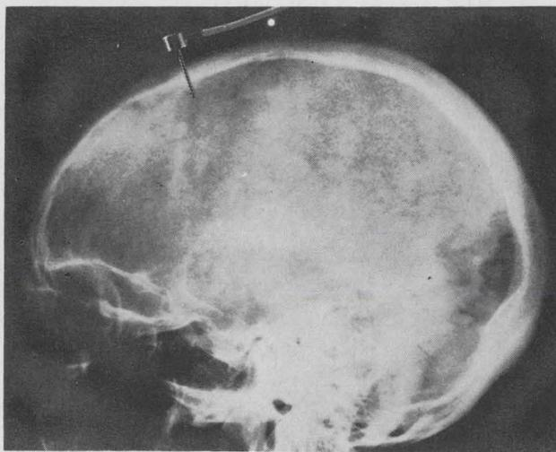
**Brain probe.** This thin-film strain gage (top), developed by Statham Instruments, is easily inserted into a patient's skull to monitor intracranial pressure, eliminating the need for a bulky catheter.
