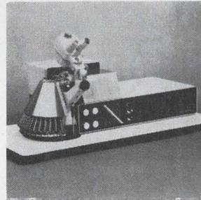
Automatic die classifier 2907 tests devices ranging from 0.020 to 0.125 in., round or square, at the rate of 3600 per hr. It features a vacuum feed device which deposits the devices gently in the test position. Vacuum is generated internally and controlled by valves to prevent them from sticking or scattering. Hughes Aircraft Co., 500 Superior Ave., Newport Beach, Calif. [426]
