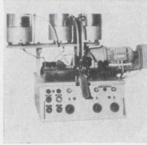
Automatic machine type 6.10, for the capping of cylindrical bodies used in the manufacture of resistors, will apply caps at both ends at speeds up to 5,500 units per hr. The caps and bodies are simultaneously fed from vibratory bowl feeders to a position where caps are applied. Capping pressure is easily adjustable. B. Freudenberg Inc., 50 Rockefeller Plaza, New York. [423]
