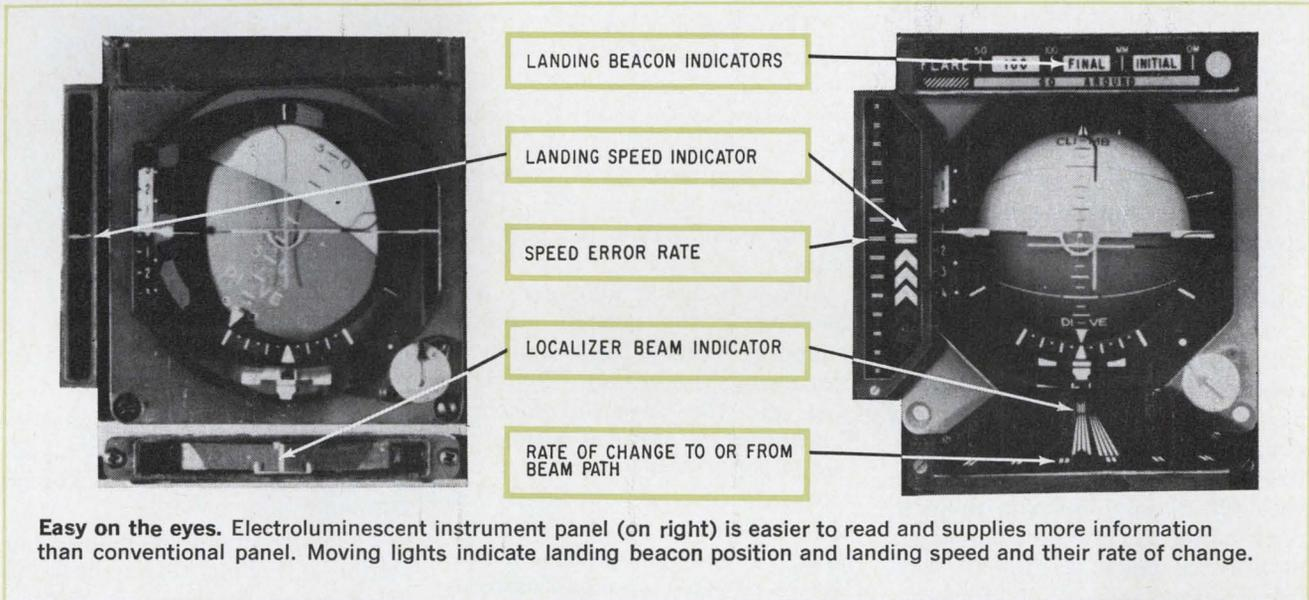
**Easy on the eyes.** Electroluminescent instrument panel (on right) is easier to read and supplies more information than conventional panel. Moving lights indicate landing beacon position and landing speed and their rate of change.
