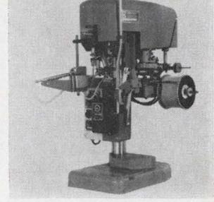
Coil-winding machine BV4-G is a carousel-type unit designed to wind electrical coils without forms at production rates from 160 to 1,920 coils per hr depending on coil design and size. Lead ends are automatically tinned. Low voltage electric heat is applied to the rotating tinning bath with electronic temperature control. Leeson Corp., 131 West St., Danbury, Conn. 06810. [424]
