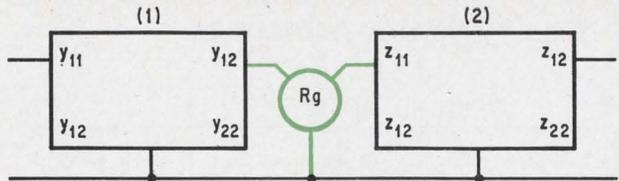
**Cascaded networks.** In this active-filter design, a single gyrator is cascaded with two RC networks, one defined by y parameters, the other by z parameters.
