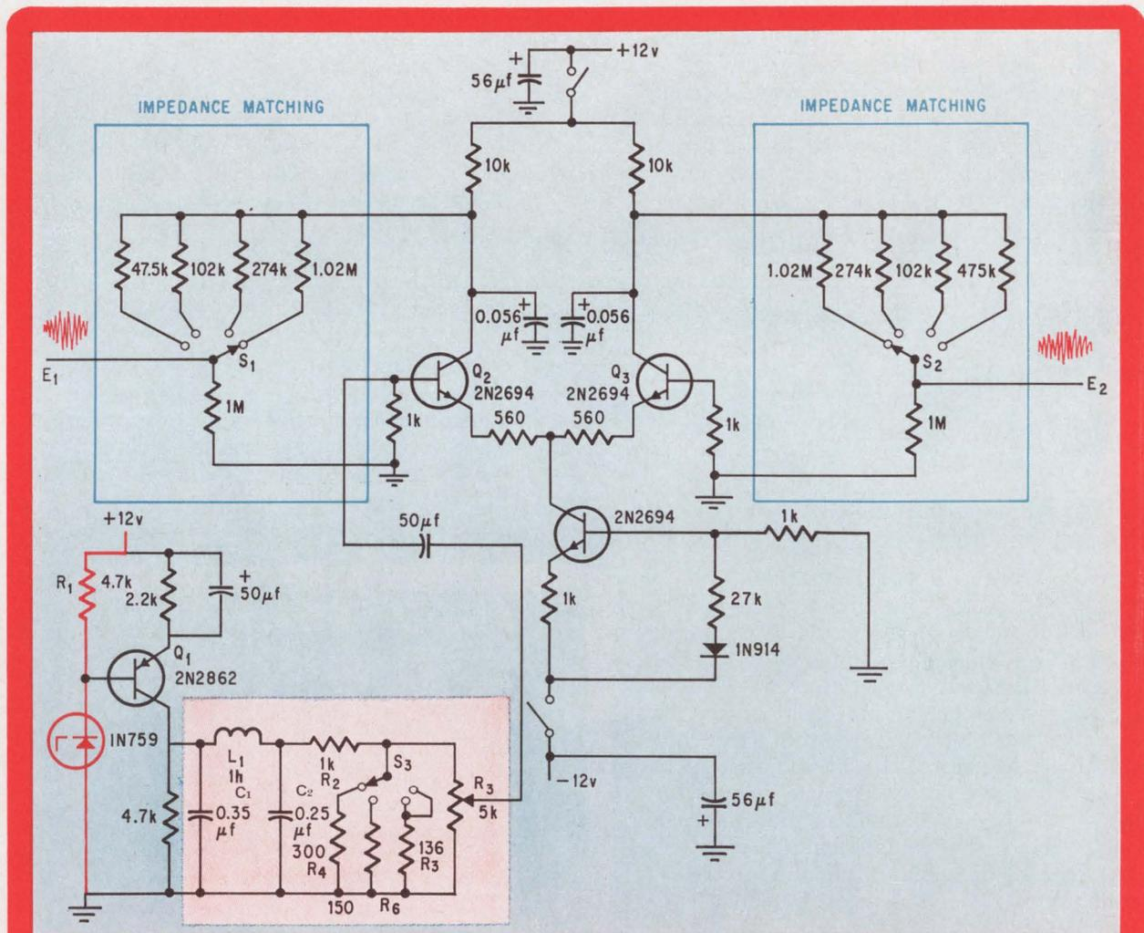
**Perpetual tension.** Myoelectricity—the white noise generated in a flexed muscle—is simulated by filtering and amplifying the noise from a zener during breakdown. The differential amplifier couples the signal into circuits that eventually manipulate artificial limbs.
