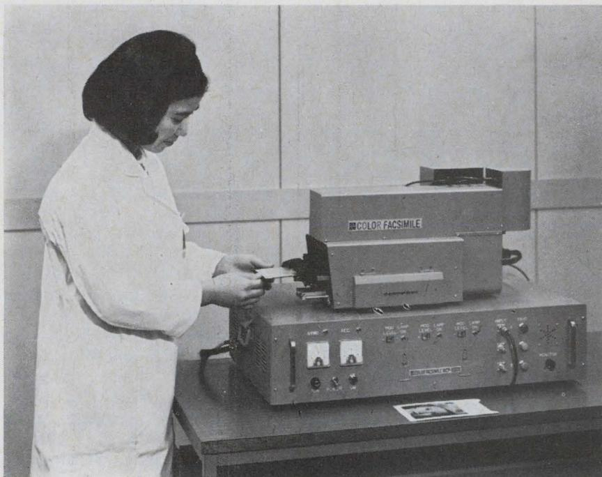
**Fast and faithful.** Primary colors transmitted simultaneously—and corrected individually—expose Polaroid film with high fidelity during 3.6-minute scan.
