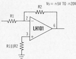
The LH101 is kin to the LM101. The essential difference is that all the required frequency compensation is *inside* the package. Current drain is low, even with the output saturated. There is no latch-up when common mode range is exceeded and there's continuous short circuit protection. Price for 100 to 999 is \$48.00. The commercial version LH201 is \$11.40.
