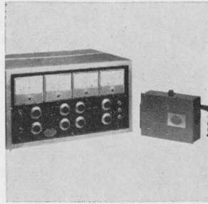
Mark II Colorgard meter will meet the requirements of color tv receiver manufacturers for quality control check on kinescopes and for setting color temperature and gray scale of color receivers on the production line. The instrument is not calibrated in color temperature values but in arbitrary R-G-B values. Television Zoomar Co., 870 High Ridge Rd., Stamford, Conn. 06905. [403]
