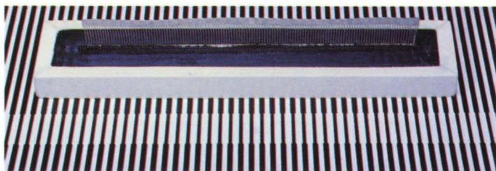
Chemical etching provides extremely precise control of lead width and inter-lead spacing. Alternate leads may be bent in opposite directions to facilitate soldered connections to a printed circuit module.
