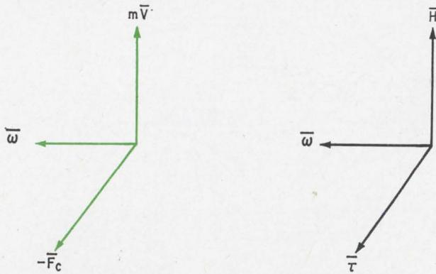
**Analogies.** Spring-restrained gyro's angular parameters, right, of torque,  $\tau$ , angular momentum,  $H$ , and angular velocity,  $\omega$ , have their counterparts of Coriolis force,  $F_c$ , linear momentum,  $mV$ , and input angular rate,  $\omega$ , in the vibrating beam sensor, left.
