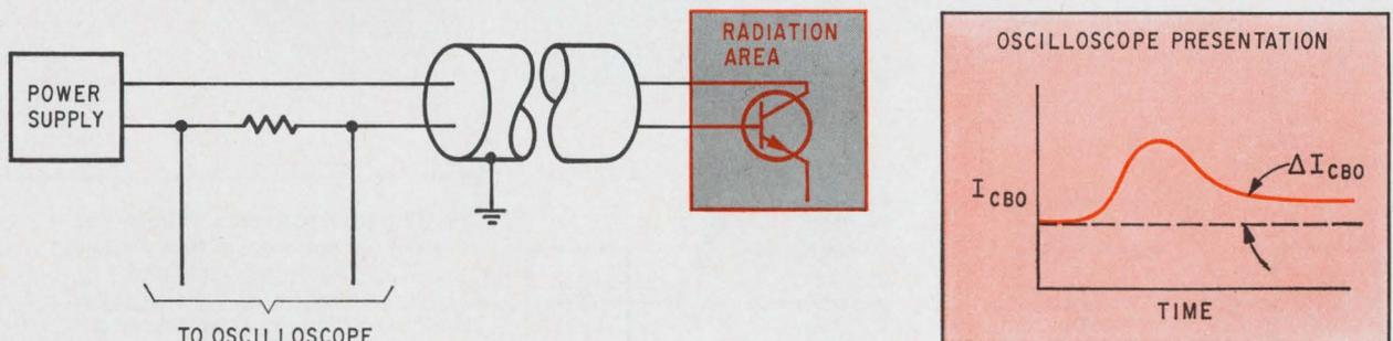
**Leakage current.** The collector-to-base junction is reversed biased by the power supply. By measuring the current flowing through the series resistor, an engineer can determine the magnitude of the leakage current,  $I_{CBO}$ , before, during, and after irradiation.
