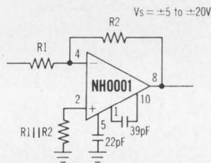
The typical dissipation of the NH0001 is but 1.8mW at  $V_s = \pm 15V$  and 0.6mW at  $V_s = \pm 6V$ . Something of a record, no? And further, the mighty NH0001 will deliver over  $\pm 10V$  into a 2K load from  $V_s = \pm 15V$  supplies. It's priced at \$48.00 in 100 to 999 quantities.
