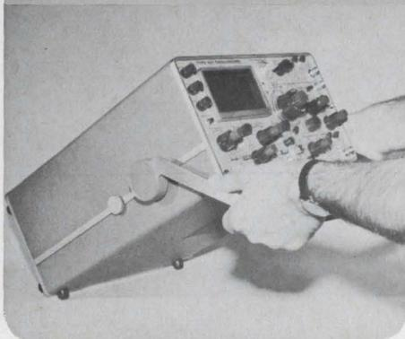
Don't worry about damaging the front panel and knobs—they're protected by a cover that also carries the accessories.
