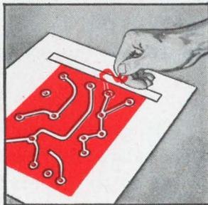
Now carefully peel off the film as outlined leaving a completed mask, positive or negative, that corresponds exactly to the desired pattern.
