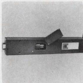
Variable set point pressure transducer model 107A is completely self-contained and can be manually set anywhere in the range from 0 to 120 psig. It produces a nominal output of  $-1.5$  to  $+1.5$  v d-c over a range of  $-20$  psi to  $+20$  psi about the set point. Linearity is better than  $\pm 1.0\%$  over the  $\pm 20$  psi range. Robinson-Halpern Co., 5 Union Hill Rd., West Conshohocken, Pa. [362]
