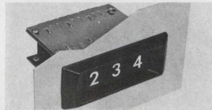
**Series 220H** Miniature, plug-in, rear-projection readout meets MIL-R-39027. .62" H x .62" W viewing area. Special lens system increases character brightness 50%. Excellent readability from wide angles and long distances.
