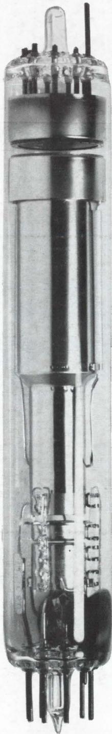
"Refresh" your alpha-numeric display with the exciting new Alphechon storage tube. Smaller than any other single-ended, non-destructive read-out storage tube previously available, this entirely new device can accept incoming signals (even over telephone wires), store them, and read them out as TV signals.
