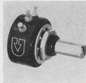
Precision pot model 1090-1001 offers advantages in applications involving high signal frequencies and need to minimize noise during adjustment. Specs include max. capacitance of 1.5 pf, max. inductance of 0.15  $\mu$ h, total resistance of 1,088 ohms  $\pm$ 10%. Linearity is 1%, temperature coefficient +20 ppm/°C. Digilog Electronics Corp., 701—3rd Ave. North, Seattle 98109. [344]
