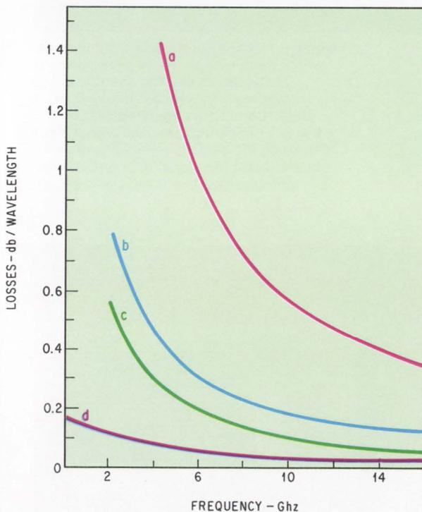
**Lower loss.** Because of alumina's high resistivity, its losses are low—lower than those in silicon. Curve "a" indicates the dielectric loss in 1,000 ohm-cm silicon, 10-mils thick; curve "b" shows dielectric and conductor losses for 5,000 ohm-cm silicon, 10 mils thick; "c" is dielectric loss for 5,000 ohm-cm silicon, 10 mils thick. Curve "d" represents dielectric and conductor loss in alumina that is 20 mils thick.
