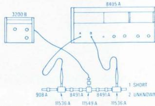
Below 100 MHz, the method illustrated above is especially convenient. Signal power is equally split, and the voltage drop across the unknown impedance is compared against the drop across the known. Results are easily entered on the Smith Chart for rapid determination of impedance.
