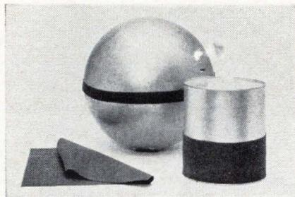
A high-loss, flexible silicone material, when bonded to a metal surface, prevents the flow of microwave currents. It reduces the backscatter or reflectivity of metal structures in cases where this is caused by surface currents. It can also be draped over objects to alter reflectivity characteristics. Radiation patterns of antennas can be modified by the application of Eccosorb CDs, to elements, dishes, and horns.
