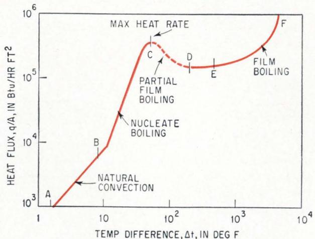
**Boiling curve** indicates relationship between heat flux and difference between temperatures of heat source and liquid. Heat is removed rapidly from heat source until at point C vapor film forms and impedes heat transfer.
