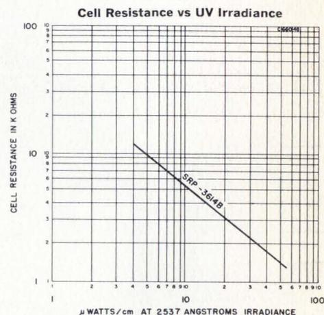
A shortcoming of many ultraviolet detectors is that they're also sensitive to infrared radiation. Thus it's often difficult, if not impossible, to use them to detect just UV in an ambient containing both infrared and ultraviolet radiation. Last year, Sylvania introduced a UV cell with attenuated infrared characteristics. Now, an improved version of this device has greater sensitivity and shows even better infrared attenuation.
