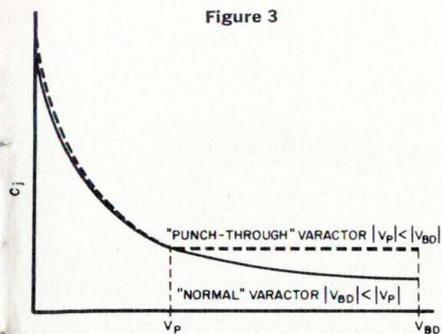
the variation of  $C_j$  as  $V$  increases. One is the maximum allowable applied reverse voltage, with the reverse breakdown voltage  $V_{bc}$ . At  $V_{bd}$ , avalanche multiplication takes place and a large current flows through the diode.
