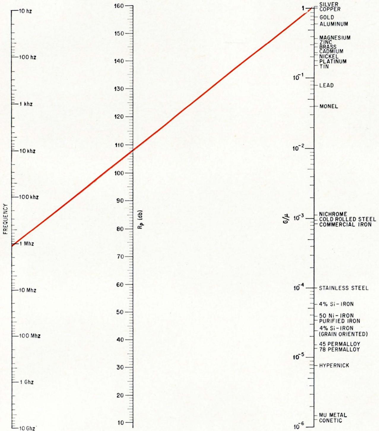
Plane-wave reflection losses  $R_p$  are calculated easily by a line connecting the frequency with the appropriate value of  $G/\mu$ . A plane wave will exist only if the source is located at least five or six wave lengths from the circuit that is to be shielded. An enclosure designed for magnetic and electric fields will also be effective for plane-wave fields.
