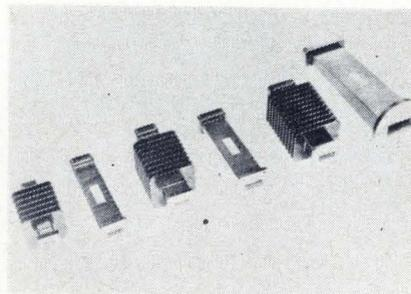
Twenty-one air-cooled dummy loads are lightweight devices, yet handle very high power levels. For example, the model LKuM1 weighs 4.8 oz and handles 25 w average power, while the model LCH100 weighs 3.6 lbs and handles 2,000 w of average power.
