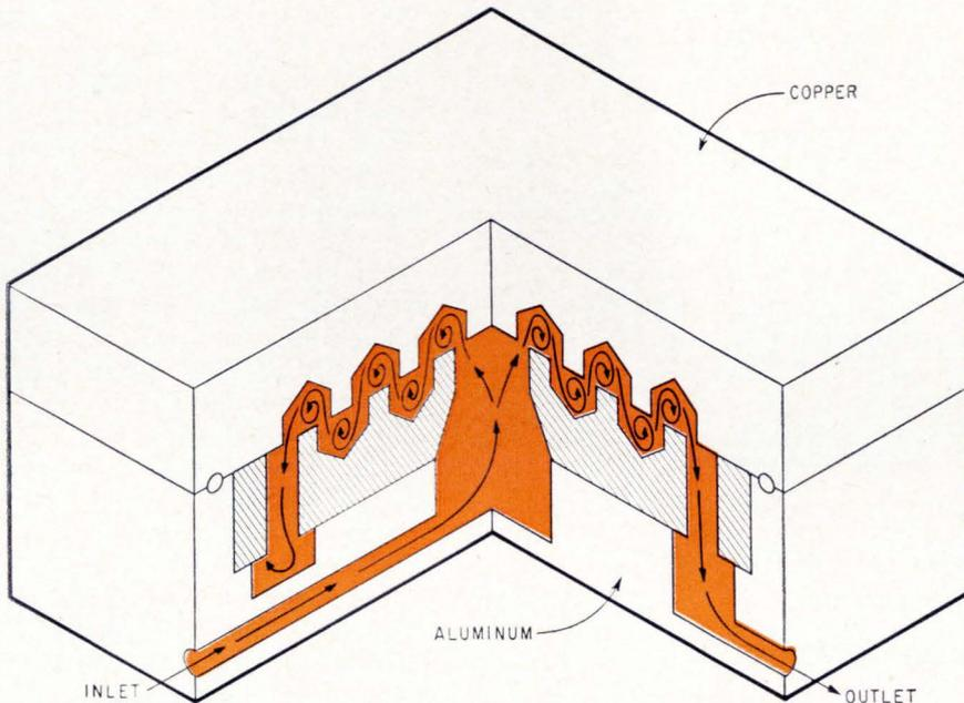
bly consists of three parts: an aluminum body, a machined insert, and a copper counter-body. The insert, now made of stainless steel, can be copper, aluminum, or even plastic, its developers say, and it could be cast instead of machined to reduce cost.
