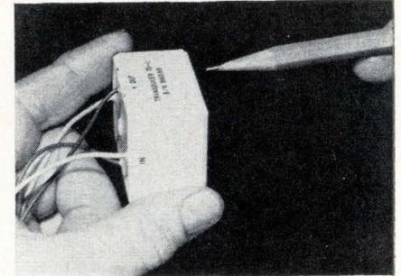
Requiring no power supply for activation, a solid-state, voltage-to-current analog squaring transducer serves as an accurate, low-energy, completely passive squaring device. Model TD-1 Transquare performs accurately for all input levels up to 200 mv. Operating frequency is d-c to 1 Mhz.
