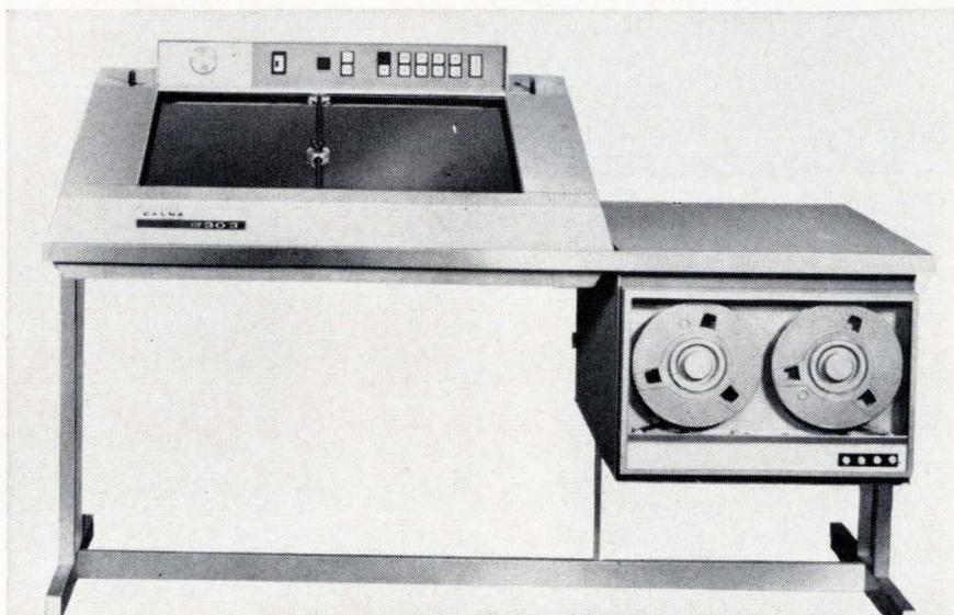
Working almost as an x-y recorder in reverse, a new graphical digitizing system allows an operator to trace curves with a stylus without worrying about outpacing the digital output recorder. Heart of the system, says the manufacturer, is "variable interval programed" digitizing.
