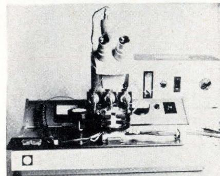
Thick and thin film devices are ultrasonically die-bonded by a multiple-head instrument. Incorporating three transducers, each with a different bonding tip, permits feeding of devices of different sizes.
