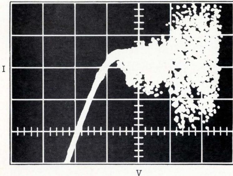
Extensive further studies produced these observations of both the Gunn transit-time and the large amplitude modes of oscillation. This large amplitude oscillation is now often called the Limited Space Charge Accumulation mode or LSA.\*\*
