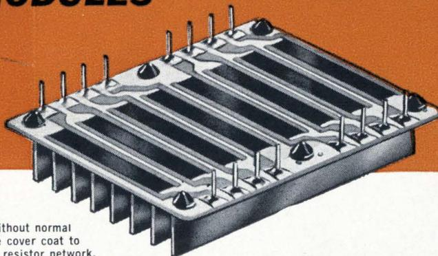
Shown without normal insulative cover coat to illustrate resistor network.
