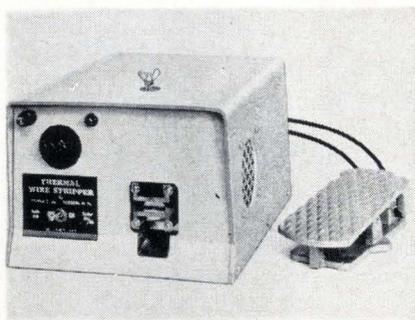
Any type of plastic covering, including Teflon insulation, can be removed by a bench wire stripper
