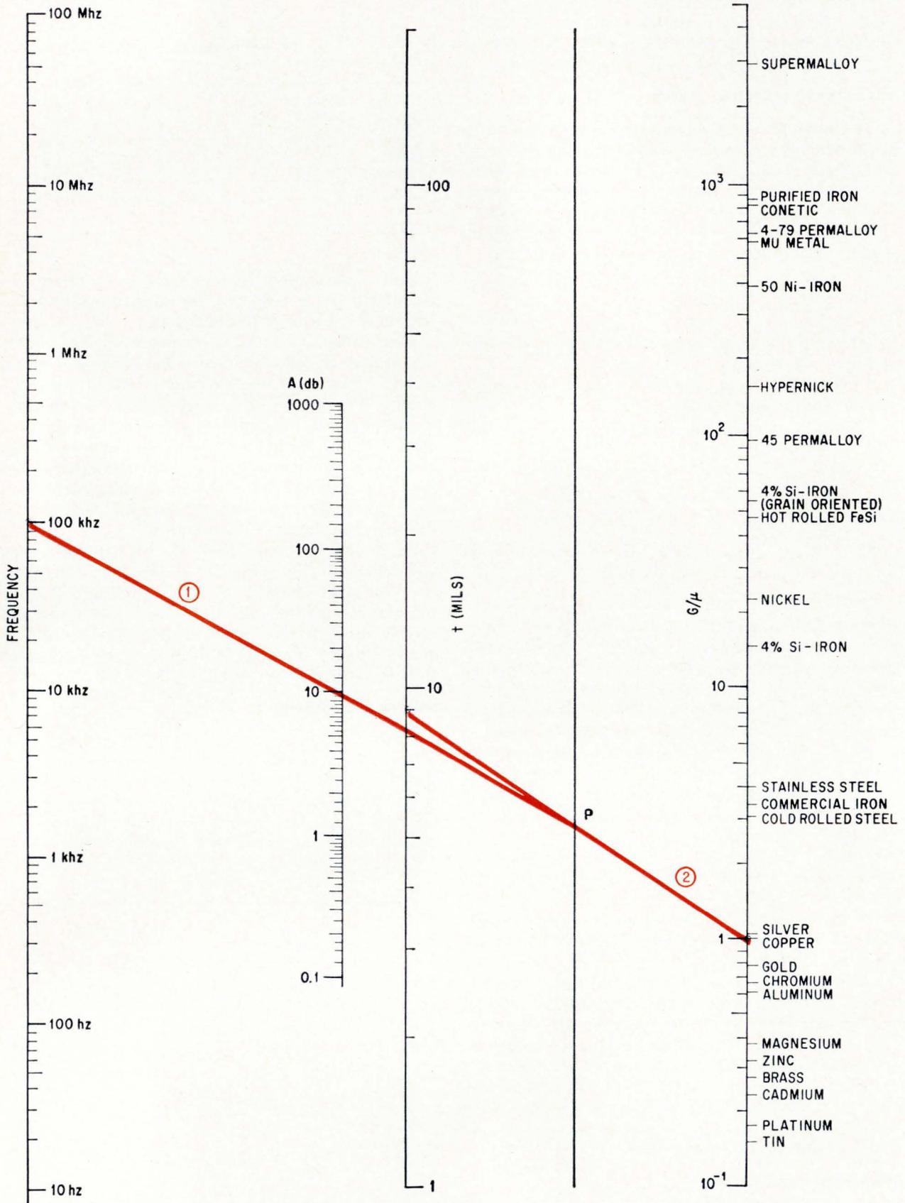
This graph selects material or material thickness for a specified absorption loss. The lines in color are plots for an absorption loss of 10 db at 100 khz. Line 1 intersects the unmarked scale at P. This new point and the material (copper) fixes line 2 and determines the thickness, 9.2 mils.
