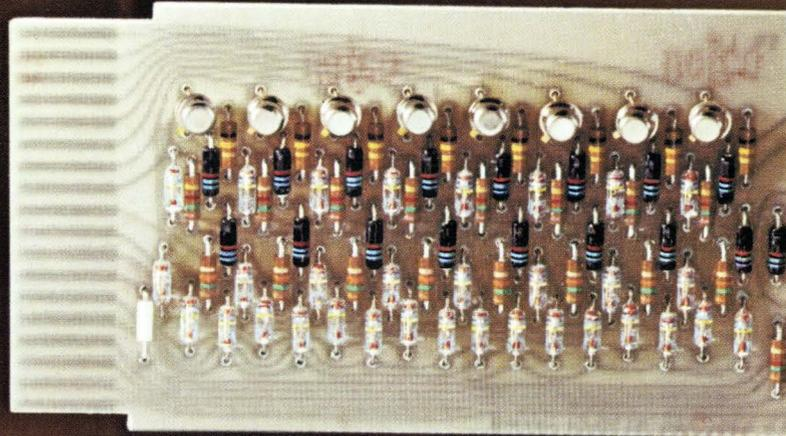
**FLIP CHIP T.M. Modules**—The Digital Equipment Corporation trademark for a new kind of digital system module uses Allen-Bradley hot molded resistors exclusively.
