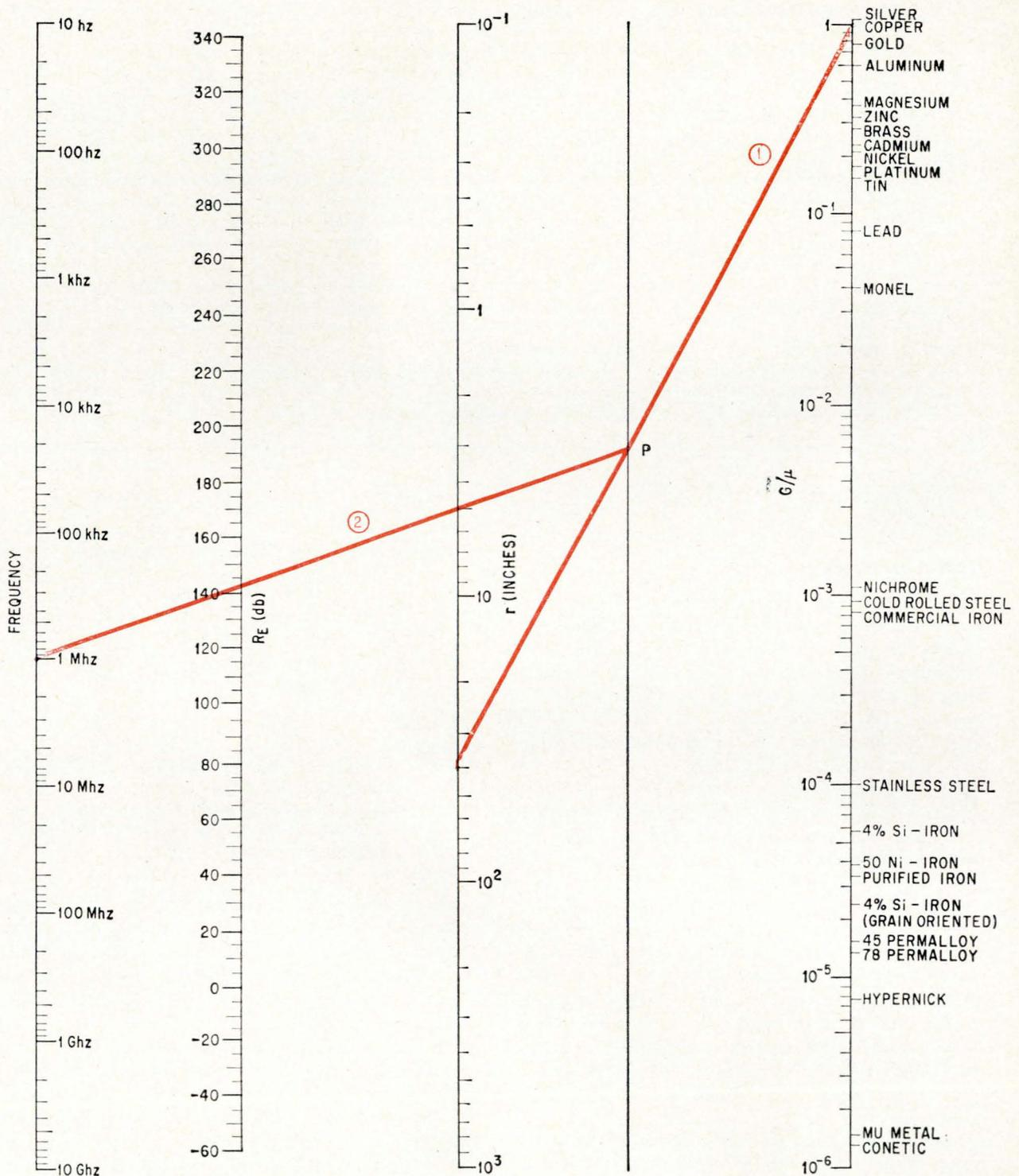
Electric field reflection loss is determined from this nomogram. The distance from the source,  $r$ , is 40 inches and the material is copper. Line 1 is drawn through these points intersecting the unmarked scale at P. Line 2 through P and the frequency (1 Mhz) intersects  $R_E$  at 142 db. Negative values of  $R_E$  indicate increased coupling that can occur at certain combinations of parameters.
