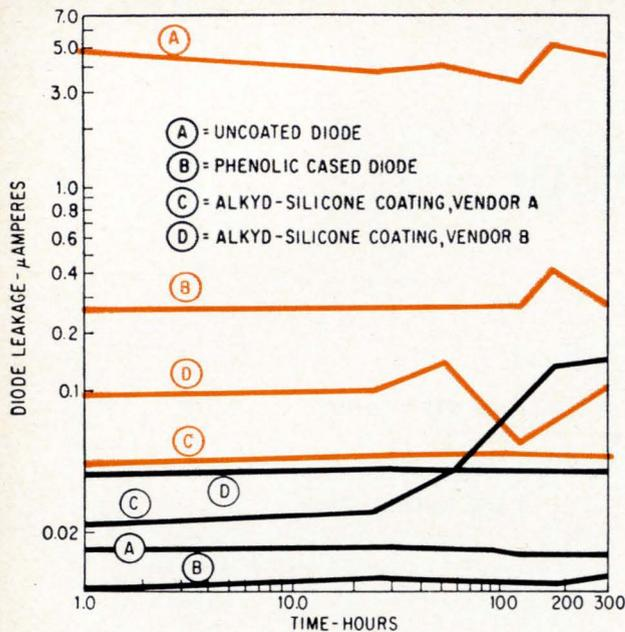
**Leakage currents of microdiodes react under exposure to dry ammonia (curves in color). The curves in black represent the same devices in a dry nitrogen atmosphere.**
