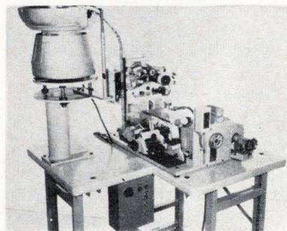
Up to 12,000 transistors an hour can be labeled by a machine designed to print the tops and sides of transistors in TO-5 and TO-18 cans and other configurations. Two transistors are printed with the completion of each cycle of the U-1166 machine.
