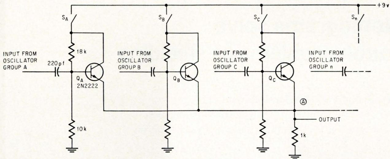
Conducting transistor associated with an oscillator group back-biases the other transistors, isolating group outputs.
