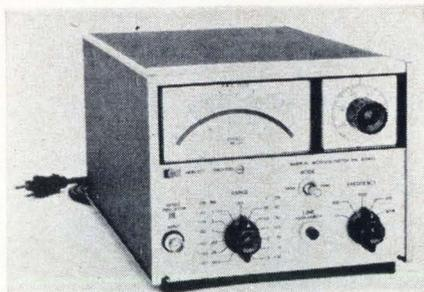
Signals as small as 300 mv rms in the frequency range between 25 hz and 60 khz are measured with full-rated accuracy by an a-c microvoltmeter. The instrument has 13 sensitivity ranges, from 3- $\mu$ v full scale to 3-v full scale in a 1-3-10 sequence. It also measures signals in a frequency range between 5
