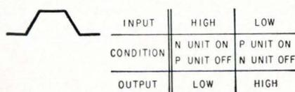
**Input and output waveforms with corresponding high- and low-level circuit conditions.**
