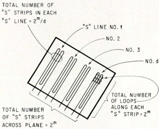
Each sense line on a plane runs through all the memory cells on the plane associated with a common digit.
