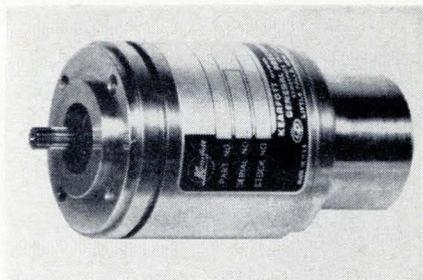
High torque-to-inertia ratio is offered in a 400-hz braked servomotor. Consisting of a size 15 servomotor and a friction brake controlled by an electromagnet, this component, designated CTO-1711 006, can maintain a constant reference position in a servosystem subjected to shock and vibration extremes. In operation, the brake element, when deenergized, effectively stops and holds the motor's rotor and shaft at a desired position.
