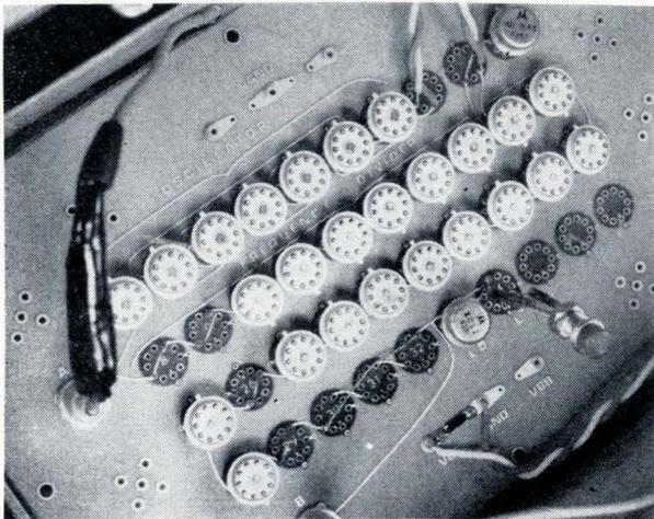
**Experimental cooling chamber** is simply a housing with a close-fitting plastic cover and tube sockets for connections through housing walls. Lamp at front of housing flickers when test circuitry is operating.
