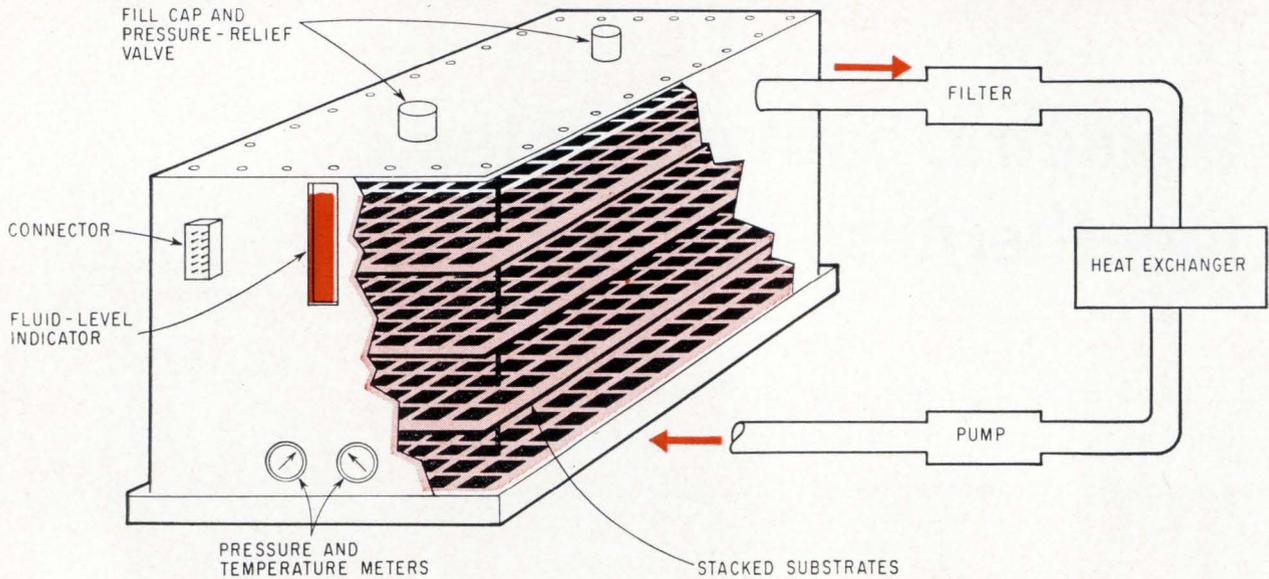
**Integrated-circuit chips** or packages could be put close together on substrates stacked in liquid-cooling housing. In some applications, external heat exchanger could be replaced by cooling fins on the housing.
