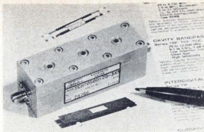
are capacity loaded, iris-coupled  $TM_{010}$ -mode cavities of 0.05-db Chebishev design. The devices are narrow band, with 3-db bandwidths from 0.1% to 1%. Power capability, although high, is limited by the type of connector used on the filter.
