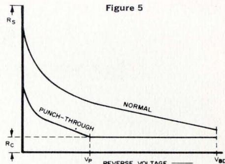
sistance of the epitaxial layer,  $R_n$ , is the dominant component of  $R_s$ , and is given by  $R_n = P_n L / A = P_n (t - w) / A$ .  $P_n$  is the resistivity of the epitaxial n-layer, and  $L$  is as shown in Figure 2.
