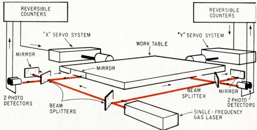
Light beams, shown in color, are the measuring elements in a laser interferometer that servopositions IC master plates with high accuracy.
