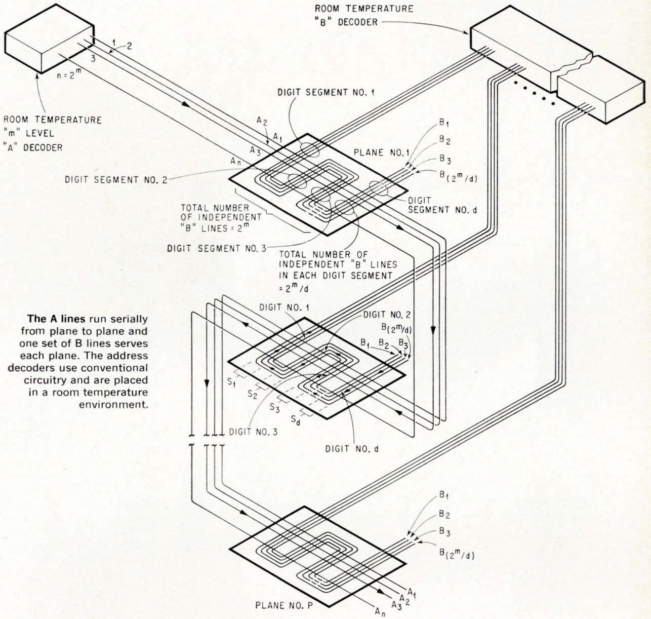
The A lines run serially from plane to plane and one set of B lines serves each plane. The address decoders use conventional circuitry and are placed in a room temperature environment.
