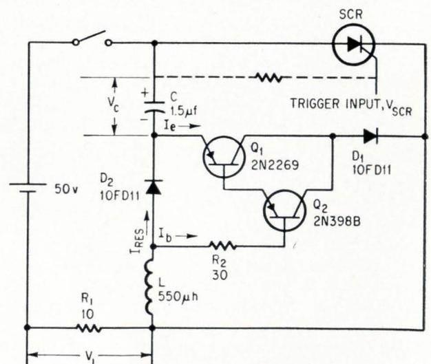
When SCR conducts, resonant current,  $I_{res}$ , charges C to a voltage opposite to the polarity shown.
