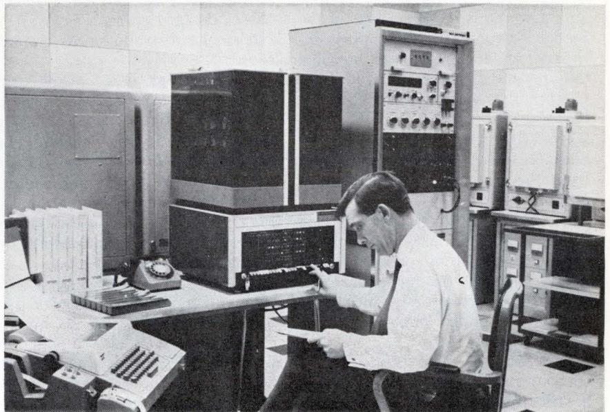
Components on trial for reliability characteristics are closely monitored and analyzed by computer in center of product test facility. Mounting frameworks for thin-film circuit modules are attached to the doors of test chambers at right.
