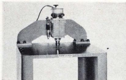
Continuous-duty printed-circuit board routing of materials from  $\frac{1}{16}$  to  $\frac{1}{2}$  in. thick as well as stack routing up to  $\frac{1}{4}$ -in. thickness is accomplished with an accurate, heavy-duty machine. Several design features incorporated in the Model 9001 minimize template wear, increase positioning accuracy, and assure efficient cutting.
