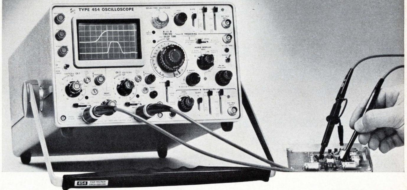
**The Tektronix Type 454** is an advanced new portable oscilloscope with DC-to-150 MHz bandwidth and 2.4-ns risetime performance where you use it—at the probe tip. It is designed to let you make convenient measurements of fast-rise pulses and high-frequency signals previously outside the range of conventional oscilloscopes.
