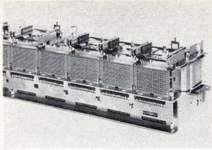
670 cubic inches. Binary operation with a wide range of input-output arrangements is provided. Palladium-silver contacts require no wetting voltage. Due to V-type positive-lock contacts, no sustaining power is needed. Power interruption will not affect the locked program.
