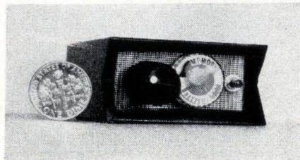
A peak voltage sensor to be used with solid state circuitry detects transients as short as 10 microseconds. The Memorette variable-threshold peak indicator has a completely floating input, making
