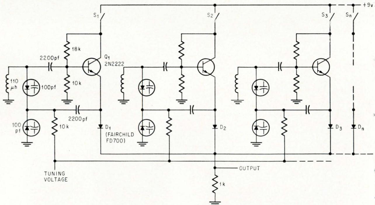
With  $Q_1$  conducting, diodes  $D_1, D_2, \dots D_n$  are back-biased, isolating the respective oscillators from the common output lead.
