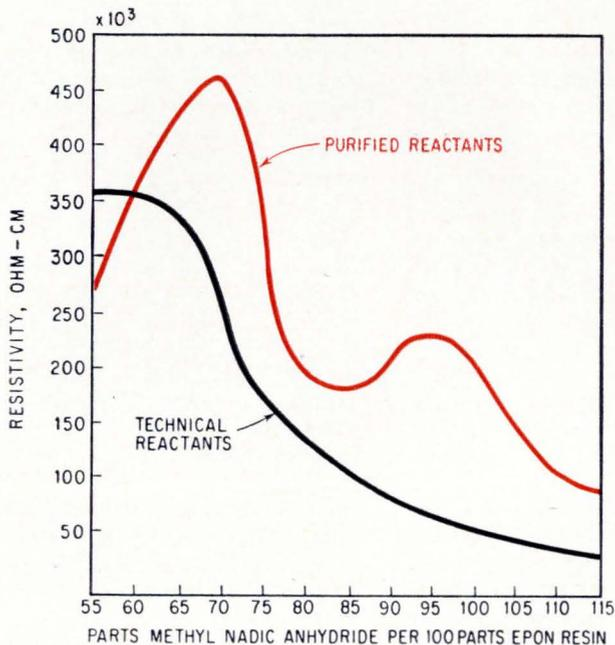
The ratio of hardener to resin affects the volume resistivity of the plastic encapsulant. Technical reactants are commercial-grade chemicals; purified reactants are those that have been further purified to remove contaminants.
