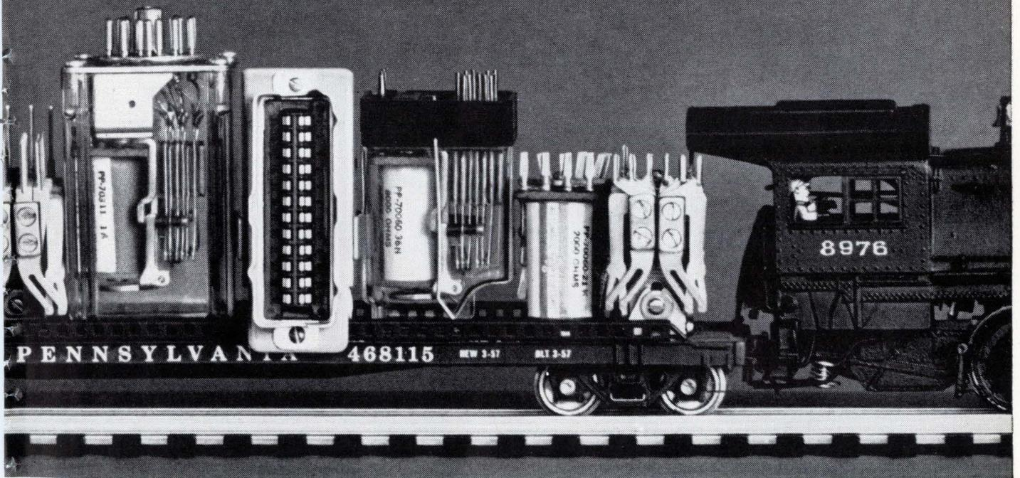
E Relays are available in hermetically sealed enclosures with either hook terminals or plug-in headers. Or plastic dust covers that snap on to the chassis- or printed-circuit type of socket.
