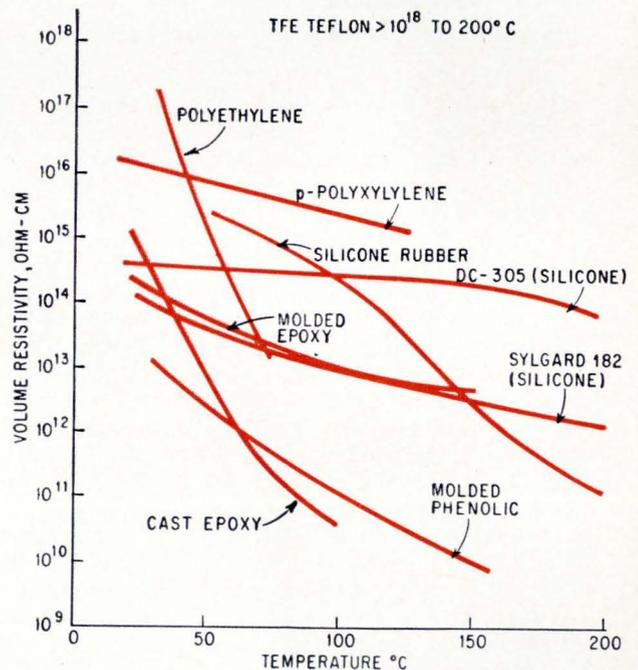
Volume resistivity of plastic coatings varies with the type of plastic. It decreases with rises in temperature. Molded epoxy gave results similar to the Sylgard 182, and resistivities for a molded phenolic sample ranged from 10<sup>13</sup> to 10<sup>10</sup> ohm-cm.
