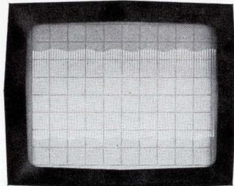
Measure 10 mV, 5 Hz amplitude modulating
