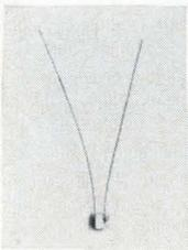
The Sippican Expendable Bathythermograph System accurately and rapidly measures and records the temperature of ocean waters down to depths of 1,500 feet. Heart of the system is an 8-inch probe, that carries, as its temperature-sensing element, a miniature-sized thermistor, shown on the left.
