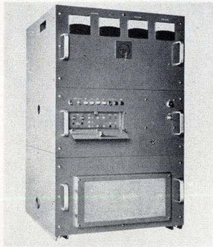
Audio and ultrasonic testing is provided by a 5-kva power amplifier that has numerous applications in sonar calibration systems, high intensity acoustic systems, vibration test systems, and industrial process
