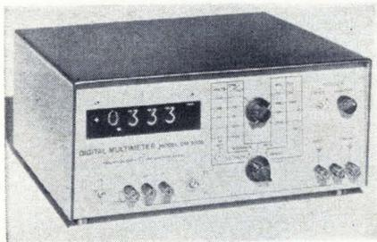
A general-purpose digital meter combines the features of three commonly used laboratory instruments in one compact, economical unit: a 100- $\mu$ v-resolution, d-c digital voltmeter, a greater than 1-Mhz multi-function electronic counter, and an electronic integrator. The extensive use of ic's and plug-in modules in the DM5000, along with circuit sharing, enhances maintainability, and accounts for the \$950 price.
