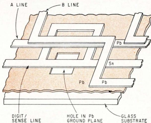
**Typical loop cell** has four superconductive layers separated by silicon monoxide insulating layers (the insulating layers are omitted for purposes of clarity). The hole in the ground plane produces more inductance in the portion of the loop which crosses over it than in the other three sides of the loop. The flux produced by current flowing over the hole is trapped in the loop and causes a circulating current, which corresponds to a stored logic binary 1.
