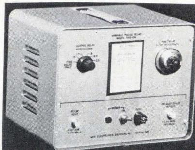
An all-solid-state unit capable of delaying pulses up to 3 microseconds with a resolution of better than 1 nanosecond has been introduced by MCC Electronics. Two or more of these pulse-delay lines can be connected in series to increase delay times.
