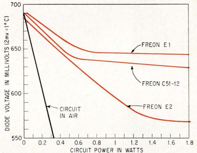
**Integrated circuit** operated in air quickly heats up, as indicated by sharp drop in diode voltage (black curve). In dielectric fluids, same circuit remains relatively cool at several times the applied power (color curves).
