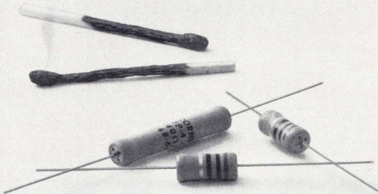
The fact is, new CORNING® FP Resistors just won't burn. Even if a circuit smacks one with an overload of a hundred times or more, it won't burn. It knows how to fail gracefully. It will open up, but no flame and no short. But don't just take our word. Test this new resistor yourself.
