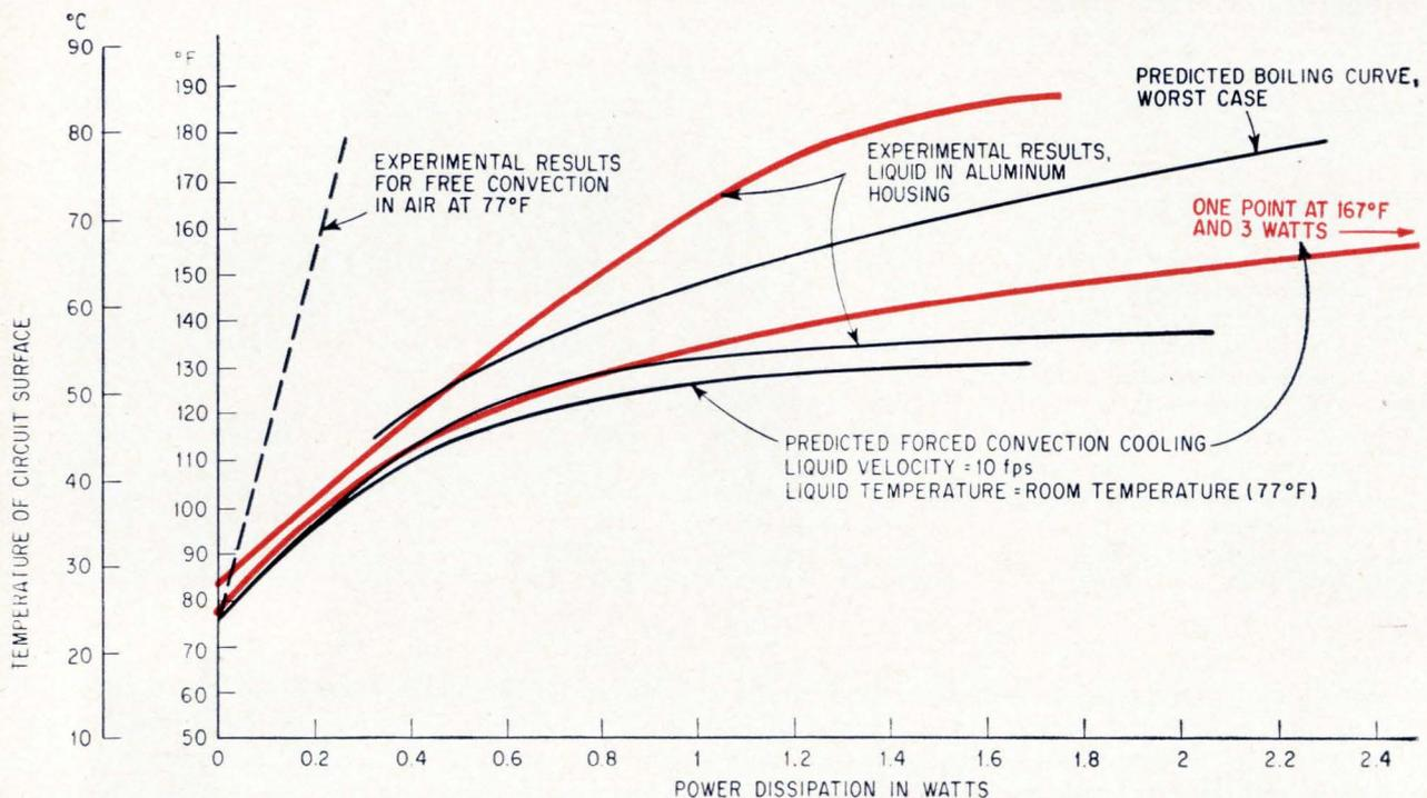
Experimental results are contrasted with calculated cooling rates for Freon C51-12 (black curves) and Freon E2 (color curves). Even without forced convection, a circuit in Freon E2 gets no hotter than a circuit in air despite a five-fold increase in applied power.
