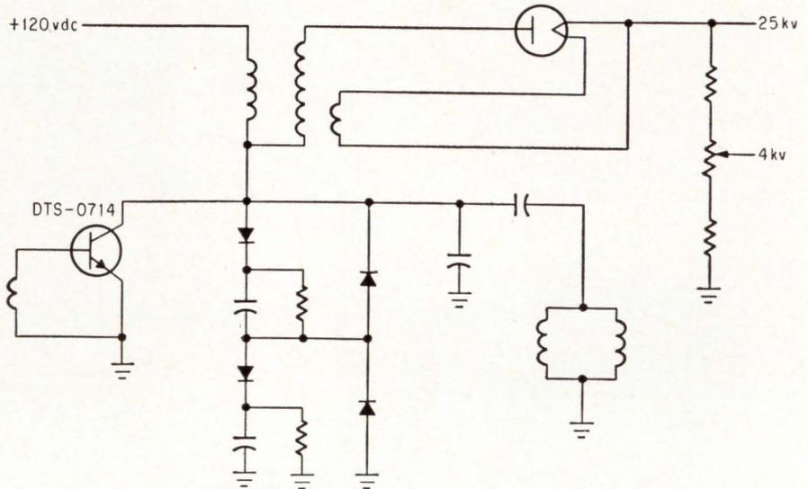
A silicon transistor has been developed that can withstand a retrace voltage pulse above 1,000 volts generated in the horizontal deflection system of a large-screen television set. The Delco Radio division of the General Motors Corp. is now demonstrating a modified 25-inch Zenith color set in which the new 1,200-volt transistor can switch the 3,800 volt-ampere load line of the horizontal deflection system (see circuit).
