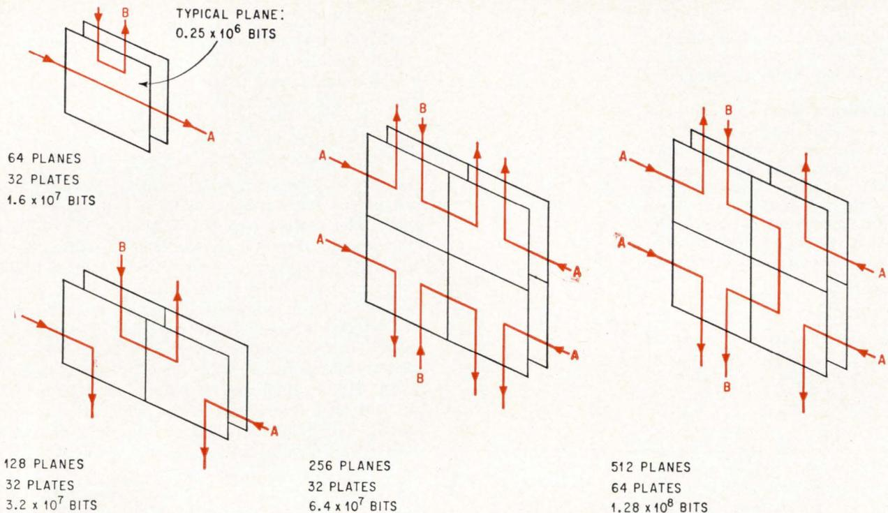
With a 250,000-bit memory plane as the basic building block, four ascending-order memory plates are depicted with A and B select lines. Each plate uses the basic planes arranged back-to-back. A 10<sup>8</sup>-bit memory thus may be built with 512 planes of 250,000 bits each. The A and B line currents would be 100 milliamperes, and the sense line current 20 ma. Power dissipation is estimated as 81 milliwatts at 3.5° K.
