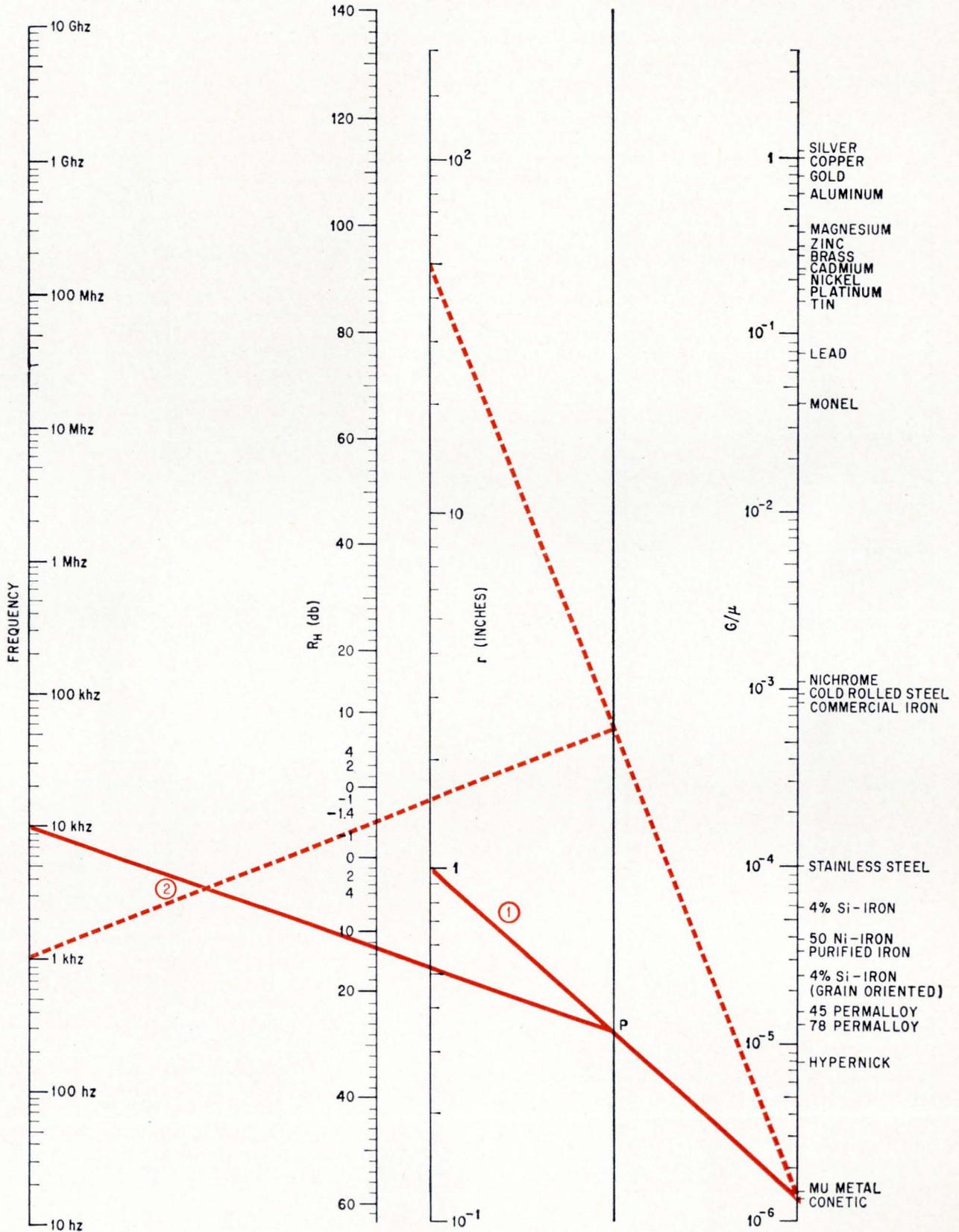
Magnetic field reflection loss,  $R_H$ , is calculated in the same way as the electric field loss. Solid line in color is for a Conetic shield located 1 inch from a source of magnetic field. Line 1 fixes point P on unmarked scale. This point and the frequency (10 kHz) fixes line 2 and the value of  $R_H$ —13 db. Broken line in color indicates that at certain distances and frequencies coupling to the shield is enhanced.
