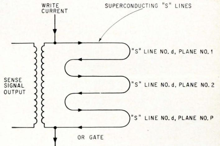
The sense lines serving a common digit on each plane are connected in series through the stack.
