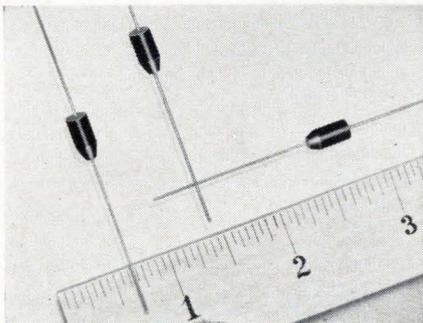
Four tiny (0.07 cu. in.) avalanche rectifiers in a single phase bridge will deliver as much as 2 kw at  $50^{\circ}\text{C}$  ambient temperature.
