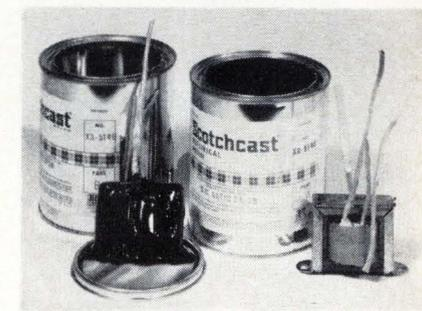
Pressure-sensitive components can be encapsulated with a black, semi-flexible epoxy resin, which has a low temperature curing cycle. Curing starts at 65°C and may range as high as 120°C. Gel time is 23 minutes at 121°C.
