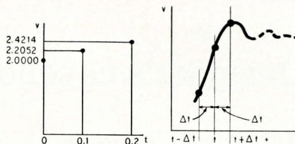
The first term on the right represents the voltage at time  $t$ , the second term is  $dv/dt$  at time  $t$ , the third term is  $dv/dt$  at time  $t - \Delta t$ , etc. See the output response curve above. Next, the program applies a corrector formula and calculates the voltage at the same time interval. The corrector formula is given by:
