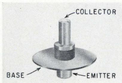
A new overlay transistor in a coaxial package takes 0.316 watt at its input and delivers a 2 gigahertz output of 1 watt. The manufacturer claims this is about 4 times the power previously available from commercial transistors operating at the same frequency. As an oscillator, the transistor has produced 1.5 watts at 1 Ghz.
