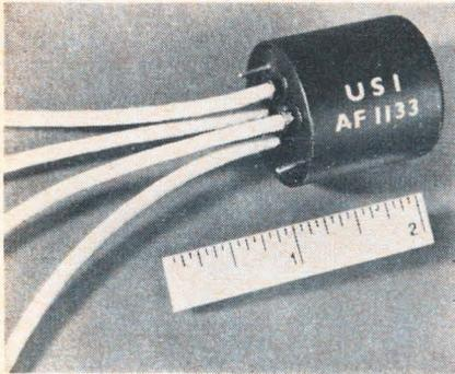
A coaxial transfer relay with a rated life of 10 million cycles and an 80-decibel isolation at 50 megahertz has been developed by United Standard Industries Inc. Its long life and high isolation characteristics are due to reeds instead of the conventional electromechanical armature and coil.
