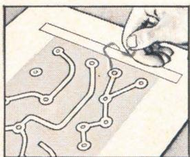
Now carefully peel off the film as outlined leaving a completed photo mask, positive or negative, that corresponds exactly to the desired pattern.
