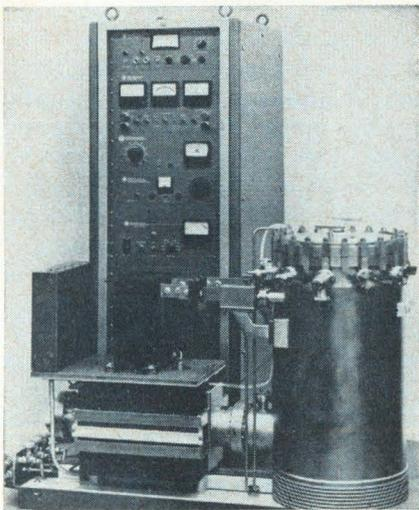
Vacuum brazing, degassing tests and long-term space simulation studies can be carried out with a new vacuum furnace that combines high stability with precise control. The furnace is also suited for annealing and heat-treating of refractory metals and alloys. It can
