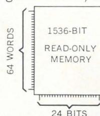
The circuit requires only 33 Radiation RM-34 "custom patterned" matrices, 11 RD-220 Hex Inverters, and four RD-234 Hex Interface Inverters. Assembly is simplified because the memory consists entirely of TO-84 packages.
