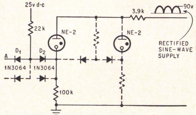
**Lamp turns on** when  $D_1$  is at ground. Lamp turns off when  $D_1$  is connected to the 25-volt supply which applies a 20-volt bias to the lamp.
