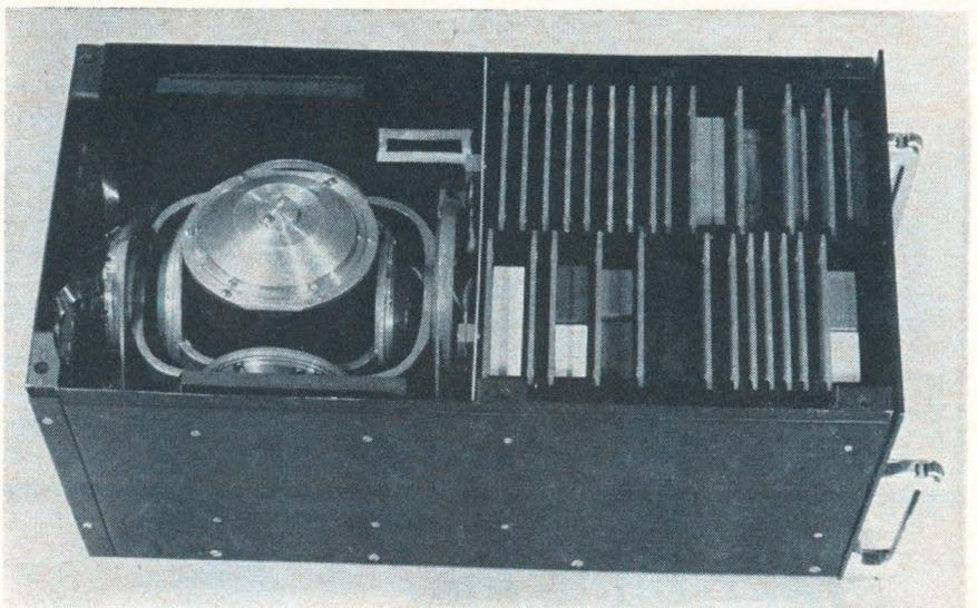
Inertial navigator, built by AC Electronics will guide Boeing's giant jet transports with an accuracy of better than 1 nautical mile per hour.
