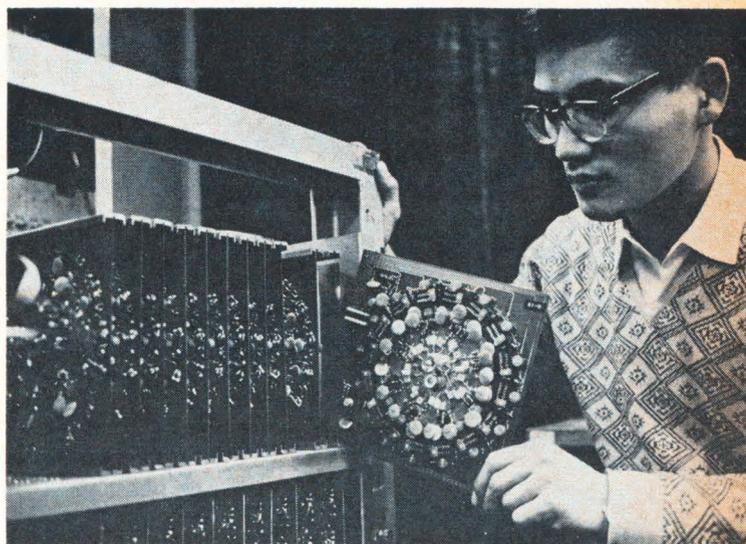
Capacitor memory's storage circuits are rack mounted in groups of 16.
