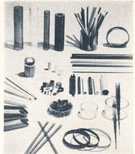
Epoxy tubing is now being centrifugally cast to concentrate the dense fillers and pigments in the outside wall area. This process produces a glassy-smooth, voidless inner wall surface for superior component encapsulation and positive bonding of the end seals.
