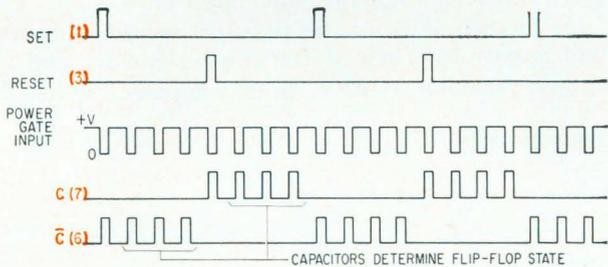
**Reduction in power from milliwatts to microwatts** is achieved by gated or pulsed power operation of commercially available digital integrated circuit. Stored charge on capacitors  $C_1$  and  $C_2$  represents state of flip-flop, obviating need for power during off interval.
