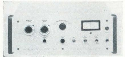
HR400A95, which incorporates the following specifications: r-f tuning range, 8.5 to 9.6 Ghz; noise figure, 9 db; i-f bandwidth, 120 Mhz; i-f center frequency, 160 Mhz; minimum pulse width, 10 nsec; instantaneous dynamic range, 30 db; video output capability, 5 v into 50 ohms.
