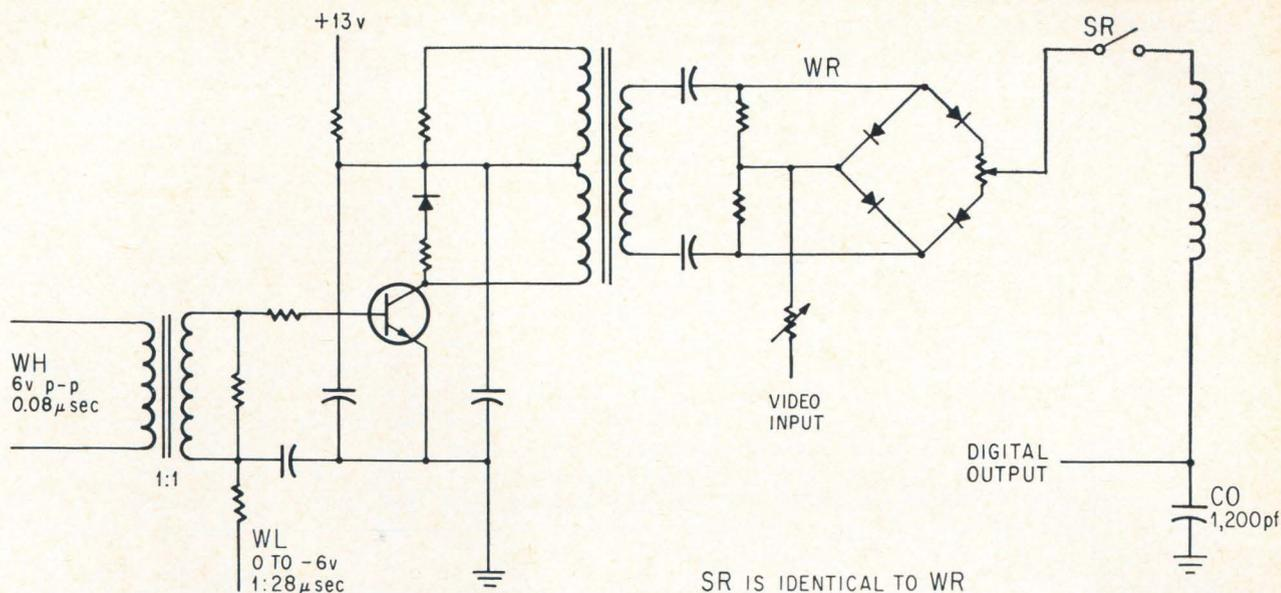
**Diode-bridge switching circuits** are conditioned by low-speed pulses WL and triggered by high-speed pulses WH. Writing switch SW stores a line element as a charge on memory capacitor CM. This charge is resonantly transferred to output capacitance CO when reading switch SR opens.
