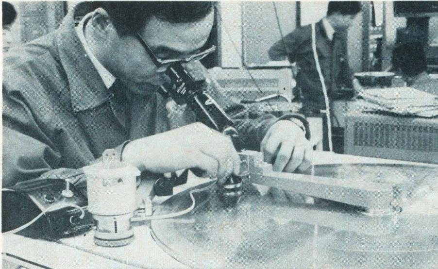
**Scientist inspects read heads on stationary brass plate which forms part of the magnetic recorder delay line. A disk of magnetic tape material is supported at the center of the plate and rotates past the heads.**
