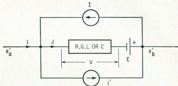
Standard circuit branch is the basic building block of ECAP. It comprises an impedance, a fixed voltage source, and an independent and dependent current source.
