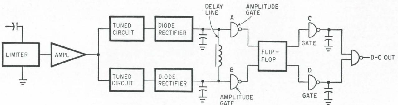
Receiving circuit at station separates the two control pulses in tuned circuits, rectifies them and delays the first pulse so two pulses combine to trigger one of the amplitude gates. Capacitors near the output are charged during alternate fields and will trigger the output after a few frames.
