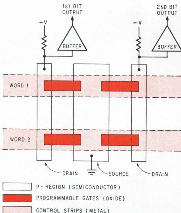
**Relationship of various layers** in the MOS read-only memory. The p-region is deposited first, then the gates and finally the metal control lines. The read-only memory's organization is more sophisticated than this simplified diagram would indicate, but the layers are deposited in the same order.
