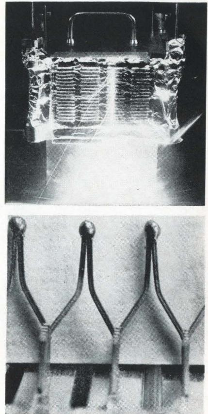
metals and a few applications in assembling integrated circuits. Now there's another: welding the thousands of connections in ferrite-core memory stacks for System 360 computers. It's being done at International Business Machines Corp.'s Kingston, N.Y., plant.
