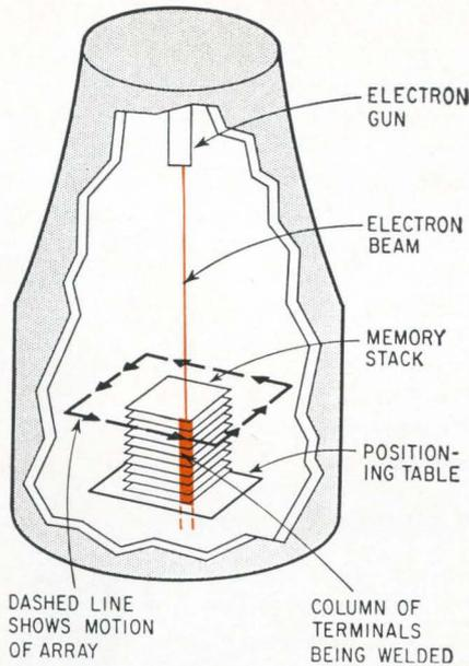
**Electron beam welds** whole column of terminals on a stack of core planes for a computer memory. Details of the process are in the cutaway drawing of the electron beam welder. The photos at the right show the welding operation (top) and the final welded nuggets (bottom).
