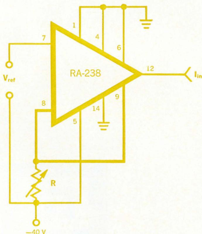
Design ultra-precision DC current sinks with Radiation IC Amplifiers in unity-gain configuration
