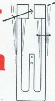
Bulova's American Time Products division has a patent pending on an important innovation in tuning forks: By affixing to the fork's tines a pair of vanes which can be slotted, notched or pierced as desired, the fork can be made to chop light or similar energy beams—making possible optical effects never before achieved.
