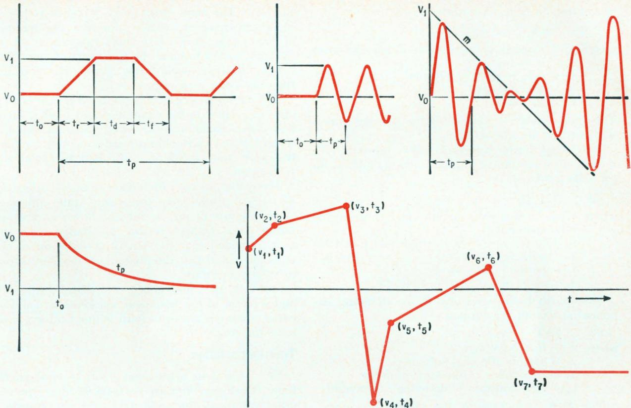
The NET-1 program can handle any of five classes of time-dependent voltage sources, as follows: a trapezoidal pulse, a sine wave, a sine wave that is linearly amplitude modulated, a decaying exponential wave, and a tabular waveform. The parameters that are called out are those needed to specify each pulse. In fourth waveform,  $m$  is the slope of the modulation envelope; in last waveform,  $t_p$  is the time constant.
