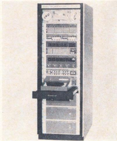
**Incoming inspection**, engineering, production and quality control areas are expected to benefit from a fully automatic system that tests many types of multilead devices, including integrated circuits, circuit boards and modules. With the Auto Data 9400 system, programming of stimuli, measurement, comparison and switching functions is accomplished with a high-speed tape reader that uses inexpensive, versatile paper tape.
