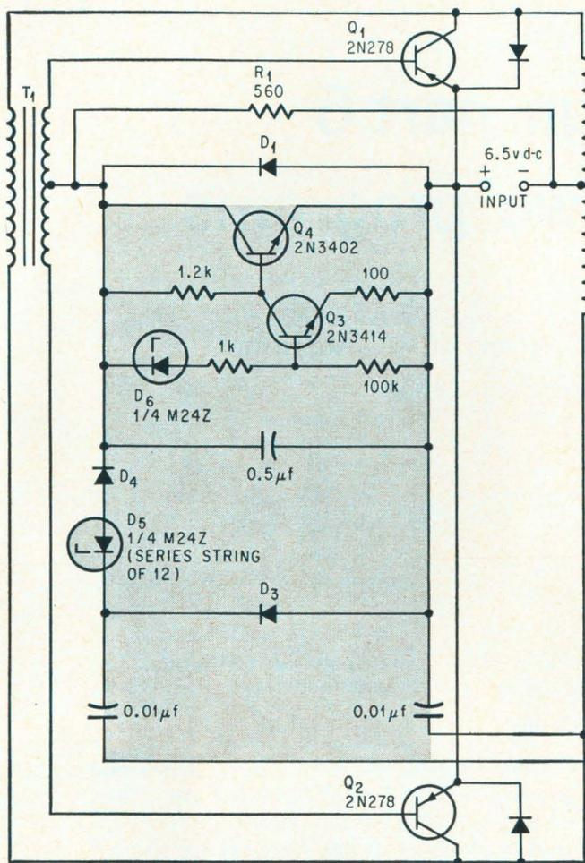
**Current source transistor Q<sub>4</sub>** driven by the feedback regulation circuit, replaces diode D<sub>2</sub> in the preceding schematic. An a-c voltage from the secondary of T<sub>2</sub> energizes the feedback circuit that controls the base current to switching transistors Q<sub>1</sub> and Q<sub>2</sub>, thus improving the converter's regulation.
