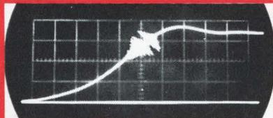
C. Same crystal filter as in (B) above, with 1/10 the sweep width (100 Hz/Div.).
