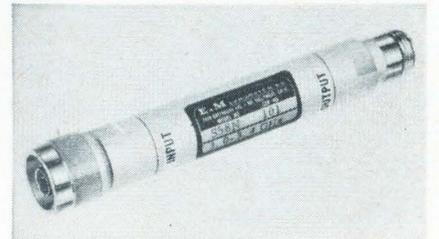
Missile and satellite systems are included among the applications for a series of low-loss, lightweight coaxial isolators. Covering the frequency range of 2 to 3 Ghz, the units offer a 40-to-1 front-to-back ratio in a magnetically shielded package 3/4 in. in diameter by 5 1/4 in. long over-all.
