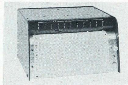
ance, 0.5 second full scale pen speed and adjustable damping. Quality construction features include fully enclosed motors and slidewires, sturdy aluminum outer structure and provisions for an optional built-in disk integrator. Dohrmann Instruments Co., CP Recorder division, 1062 Linda Vista Ave., Mountain View, Calif., 94040. [372]
