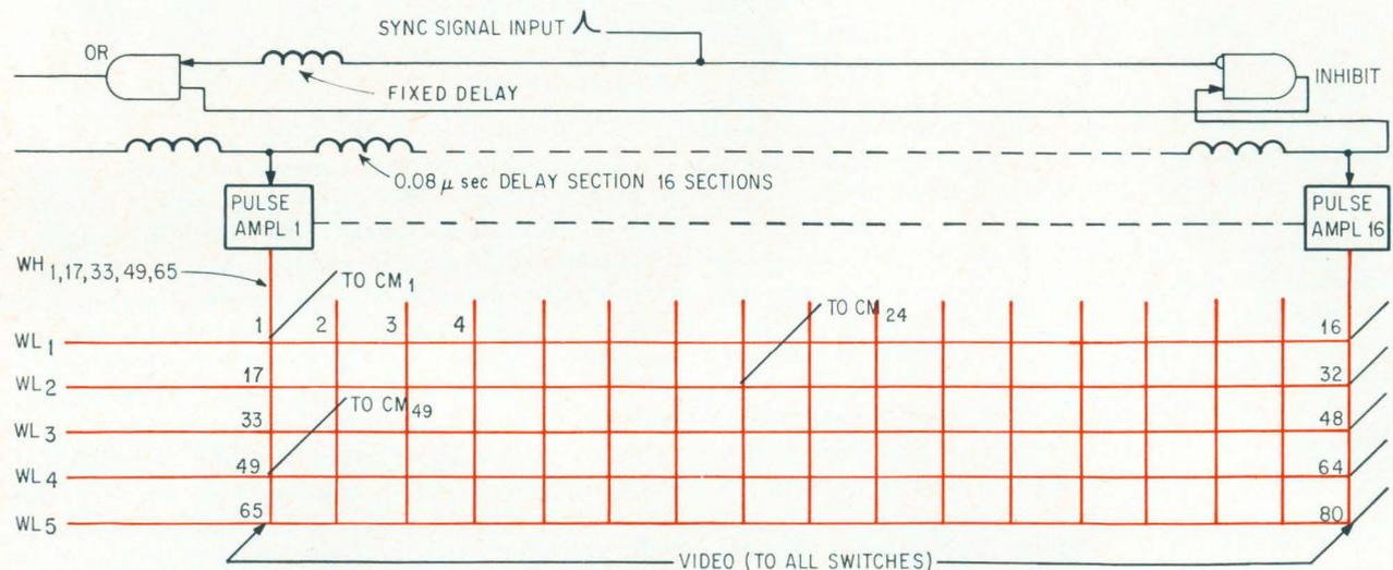
Matrix representation of the writing format. High-speed pulses  $WH_{1-80}$  open switches at the points where they coincide with low-speed pulses  $WL_{1-80}$ . This chops up the video line into 0.08-microsecond elements that are sequentially stored. The arrangement requires only 16 high-speed pulse amplifiers and allows 80 line elements to be stored for up to 6.4 microseconds.
