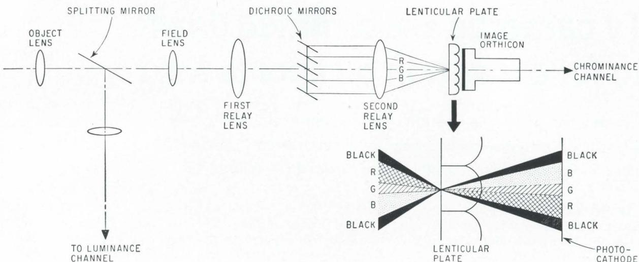
**Experimental** two-tube color camera uses crossed dichroic mirrors and lenticular plate instead of primary-color stripe filter, as in Type I and Type II cameras. Placing the lenticular plate behind the mirrors achieves the effect of a color filter with many sets of stripes.
