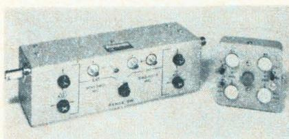
Automatic Smith chart impedance plotters are available in both coaxial and waveguide units.
