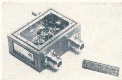
Solid state vhf-uhf preamps cover the band of 200 to 550 Mhz with a noise figure of 2.5 to 3.5 db over the band. They are ruggedly constructed to operate in all types of field environmental conditions. A special case and filters protect against radio interference generated by transmitters and other nearby equipment. The unit was designed to replace parametric amplifiers in tropo scatter systems operating in these bands.
