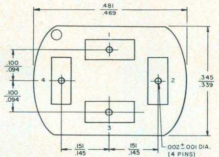
A broadband radio-frequency transistor with lead inductances so low they can't be accurately measured is now being offered as a developmental type by the semiconductor division of the Radio Corp. of America. The emitter lead inductance is approximately 0.1 nanohenry; the base lead inductance is about 0.2 nh.
