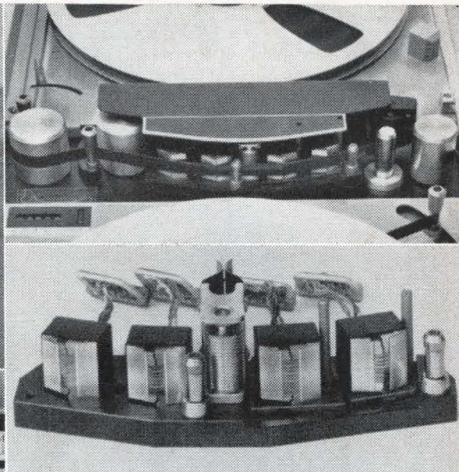
Both record and reproduce heads are pre-aligned on a single precision baseplate that mates directly to the transport casting—virtually eliminating the need for adjustment. Assemblies are easily replaced in the field.
