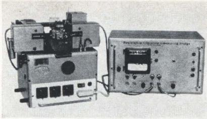
slot path on all types of resistors with an accuracy of  $\pm 0.25\%$ . It handles resistors with or without leads and over a very wide resistance range.
