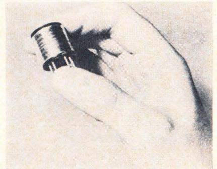
A miniature audio amplifier designated model 614A can be used as a power and line amplifier for tape recording or as a microphone pre-amplifier, tape playback and magnetic cartridge preamplifier. Extremely low noise and minimum distortion, even in the severest applications, make it also particularly adaptable for use with hydrophones, accelerometers, biomedical sensors and transducers.
