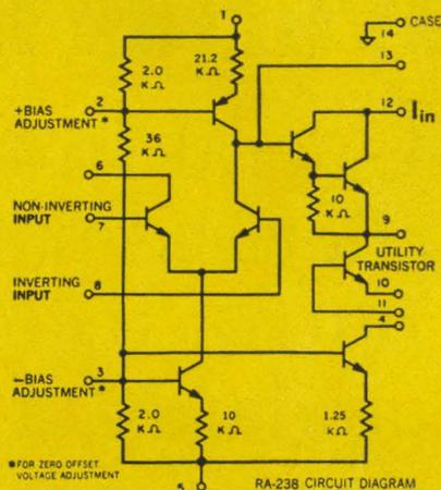
Use of Radiation's RA-238 Operational Amplifier greatly simplifies design of DC current sinks, as illustrated at left. First, absolutely no external stabilization is required. And second, in a practical system, this stable dielectrically isolated amplifier contributes typically less than 0.04% error in the total sinking current.
