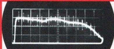
A. Frequency response of broad-band video/amplifier, 500 kHz to 20 MHz.
