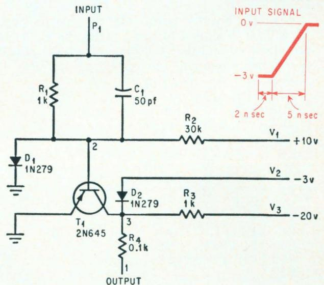
Inverter circuit serves as an example for d-c and transient analysis by NET-1.
