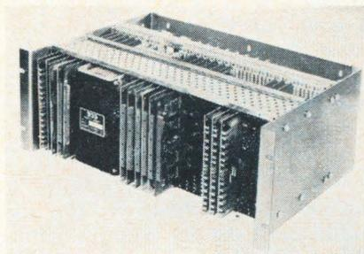
Latest addition to the manufacturer's family of core memories offers features of both off-the-shelf and custom designed systems. The CE-100 has a 1-microsecond cycle time; it comes in modules of 4,096 four-bit words, and is expandable to 4,096 words of 36 bits in four-bit increments. Expansion is accomplished by the addition of bit-oriented, plug-in logic boards and selection of magnetic modules.
