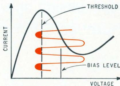
**Current-voltage curve**, in black, for LSA diode exhibits uniform negative conductance—indicated by the portion of the curve directed downward to the right. Oscillations, in color, below the threshold level suppress space charge that forms in Gunn-effect devices.
