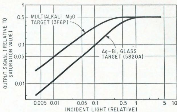
**Sensitivity** at low light levels of 3-inch, 3F6P image orthicon with multialkali photocathode and improved magnesium oxide target is much greater than sensitivity of conventional 5820A tube. Target spacing for both tubes is 55 microns; photocathode sensitivity for the 3F6P is 123 microamps per lumen, about twice as high as for the 5820A.
