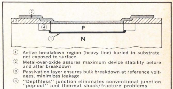
before breakdown . . . keeps the units at consistent, uniform voltage levels.
