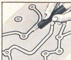
With sharp blade, outline the areas to be masked. Do not cut through the backing sheet. The Ulano Swivel Knife does the job quickly, easily.
