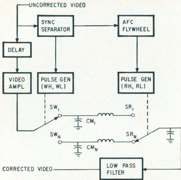
Uncorrected video line signals are stored sequentially in memory capacitors  $CM_{1-N}$  by the writing switches at the left. The digital pulse train is read out through the output capacitor and converted back into a corrected analog video signal by the filter.
