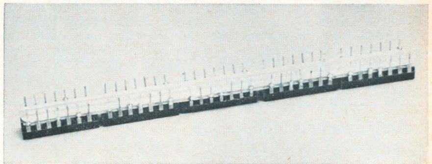
two center rows of holes in the terminal board. To make handling easier, the leads can be bent 90° so they will rest on the oval pads.
