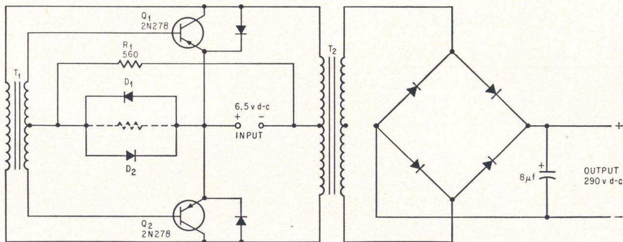
Back-to-back diodes  $D_1$  and  $D_2$  replace the 30-ohm base return resistor in a conventional converter circuit, saving power on start-up.
