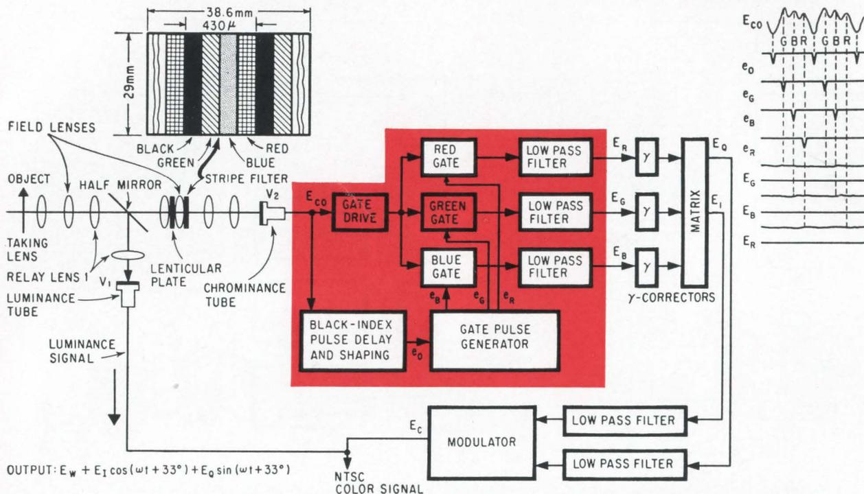
**Input signal** to two-tube color camera splits into luminance and chrominance signals. Chrominance tube scans signal passing through primary-color stripe filter, then feeds it into dot sequential-to-simultaneous converter. Stripe filter has about 80 sets of stripes in early Type I design, as many as 100 sets in Type II cameras. Luminance and chrominance channels are combined to form NTSC color signal.
