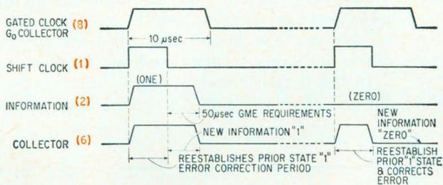
**Triply-redundant shift register** of  $n$  stages, incorporating power-saving pulsed power mode and error correction, operates reliably despite power supply variations and large changes in repetition rate.
