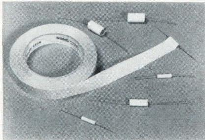
**Bondable backing** and a thermo-setting, pressure sensitive adhesive make this polyester film electrical tape suitable for wrapping capacitors and small diameter coils. The 2-mil-thick film provides sufficient body and the bondable backing resists the tendency to lift when the tape is applied to small-diameter objects.
