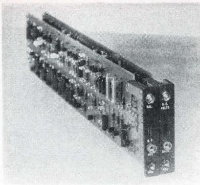
in a standard 19-inch rack with a panel height of only 3½ inches. Over 200 discriminators fit a standard 72-in. rack.
