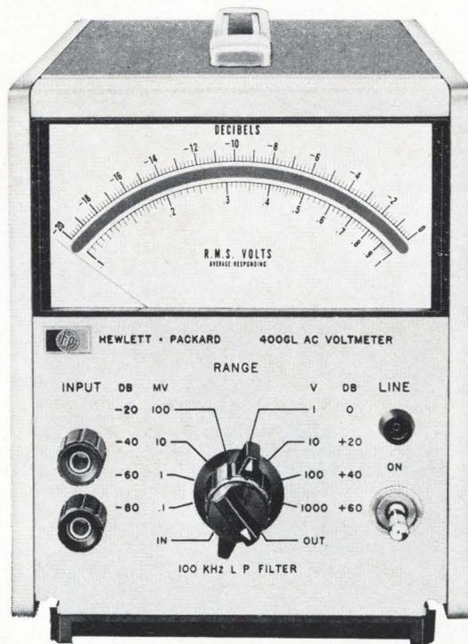
This voltmeter was especially designed to increase efficiency and speed of acoustic and sonar measurements. It can be used in calibration laboratories because of its speed of response, accuracy, high sensitivity and low noise.
