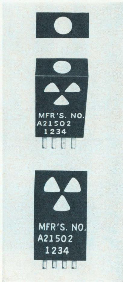
To circumvent the shortage of maintenance technicians the Defense Department has ordered the installation of fault indicating devices on most avionic equipment—down to the module level. Eventually the Defense Department plans to include indicators in almost all their gear. These indicators are termed BITE—for built-in test equipment.
