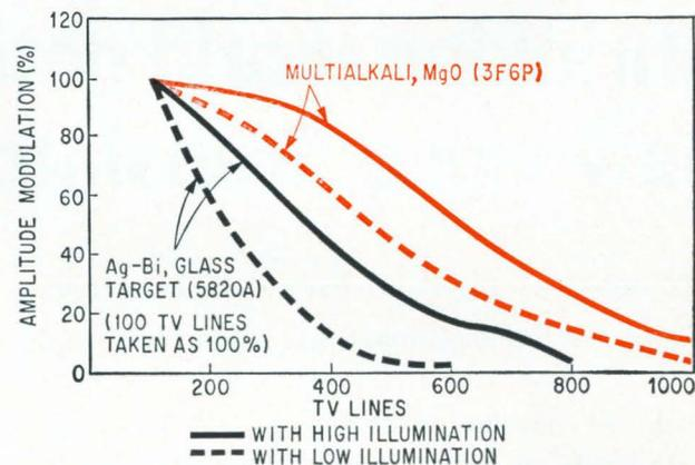
**Resolution** of 3-inch, 3F6P image orthicon is greater than resolution of conventional 5820A tube at both high and low light levels. Low light level is taken as 1/16 of the maximum value of illumination shown in the sensitivity curves.
