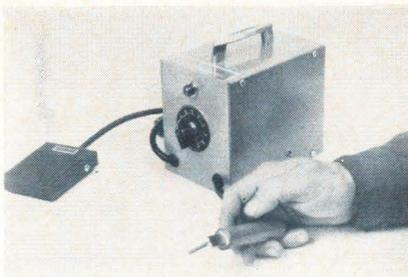
A solder tool can silver-solder small parts and wire as fine as 0.3 mil. It is used almost exactly as the
