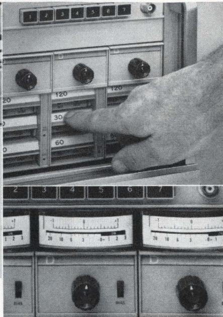
Individual meters for record modules give continuous display of signal or bias levels: bias and calibration adjustments, as well as test points, are readily accessible.
