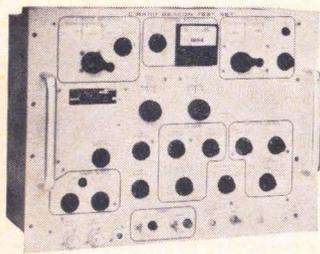
Because this compact, multi-functional test set generates pulse test signals from 5.4 to 5.9 Gc to **completely** test any C-Band beacon. Also because its direct reading wave meter function is accurate to 0.01%. The set measures frequency, power, receiver band width and sensitivity. It simulates coding, and all pulse widths are continuously variable.
