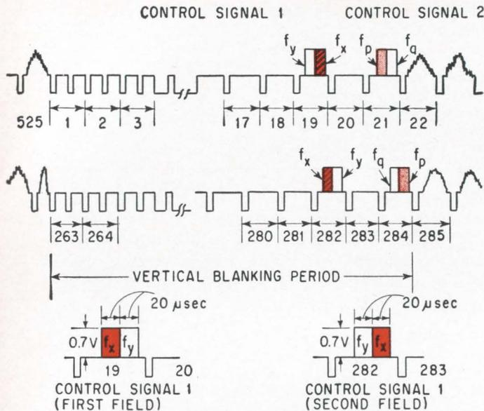
Control signals, in color, are added to the two fields that make up a television picture frame. The frequencies of each pair of control signals reverse in successive fields. Control signal 1 identifies the type of tv program while control signal 2 performs a switching operation at the remote stations. The video waveform is shown with the polarity generated at the television studio.
