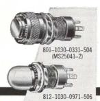
Checks lamps—instantly—without removal from the assembly. Light pressure on the lens cap assembly breaks the normal circuit and makes a test circuit. If the lamp lights when pressed in, it is proven satisfactory. If the lamp fails to light when pressed in, it is defective; (lamps can be quickly replaced from the front of panel). Release of finger pressure restores the lens cap assembly to operating position.
