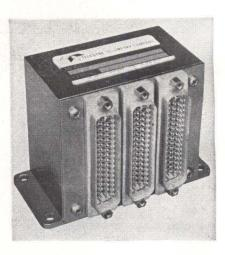
Using integrated circuits, the 710 pulse code modulation systems require less than one-third the volume of systems with discrete com-
