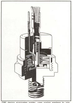
CBE design eliminates solder, uses spring washers to join thyristor elements by compression. Result: higher surge, current and I<sup>2</sup>t ratings.
