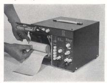
What about operator convenience? Thanks to its unique snap-in, front chart-loading and convenient pushbutton selectable chart speeds, the DG 5511 is the easiest-to-use direct-writing recorder available today.
