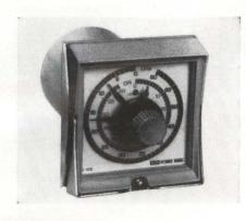
Plug-in electromechanical timers, designated the HG100 series Flex-opulse, repeatedly close and open their single-pole double-throw contacts. They perform tasks formerly requiring two separate timers in a flip-flop arrangement.
