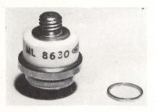
Gold-plating planar triode tubes are helping to reduce size for distance measuring equipment and transponder devices in air traffic control systems. The unit has a thin coating of 24K gold on all exposed metallic surfaces. This permits easy solderizing of connections of the tube to the associated circuit components inside the equipment, thus enabling the design of more compact control units
