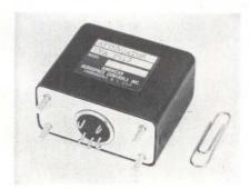
Current variable attenuators utilizing magnetoresistors designated type CVA 3012, are infinite resolution and noiseless attenuators. They can be used for remote volume or gain control circuits as well as electrically isolated signal mixing and
