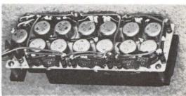
An array of three laser diodes with lenses and pulsers seen from the front (left) and back. Each section of the array, clearly indicated in the front view, generates 10 to 15 watts peak power through the entire system. The unit is less than 3 inches in length and 1 inch in depth and width.
