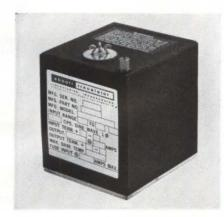
fail-safe, short-circuit protection is available on U3 models. In addition these converters feature complete isolation of inputs and outputs and an adjustment range of 12% from the nominal output voltage. Design characteristics insure close regulation (0.2%) for line variations of 105 to 125 v a-c. Output ripple is less than 0.2% rms.
