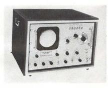
A spectrum analyzer has been designed for ssb and narrow-band r-f transmitters and exciter waveform envelopes. Model MD500E, with an input center frequency of 500 khz, serves as a bandpass monitor when used with communications receivers for narrow-band, high-resolution analysis of communication channels.
