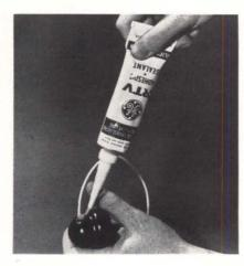
RTV-118, a clear, precatalyzed liquid silicone rubber is packaged in applicator-type tubes and cartridges as well as bulk containers. The silicone can be used as a potting compound for detailed electrical terminals and apparatus, or as a coating that provides mechanical protection for components. It has a low viscosity (approximately 350 poises at 25°C) in the uncured state.
