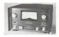
instrument's dual range peak reading panel meter or observed on an oscilloscope. The instrument can make flutter measurements at all standard tape recorder speeds from 1% to 120 inches per second. A peak eliminator circuit removes output transients caused by tape dropouts and 60 decibels of limiting suppresses amplitude variation effects. The instrument's bandwidth and filter characteristics comply with the recently revised IRIG standard at the seven standard tape speeds.
