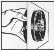
■ Time and money saving installation—just cut-out hole for fan and slide neoprene rubber mounting ring over venturi—and the Skipper is instantly secured in position. No mounting holes to drill... no nuts and bolts to handle.
