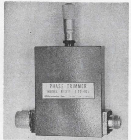
A noise-free coaxial phase trimmer, model Rf311 has no sliding metal-to-metal contacts. It is used as a coaxial line stretcher where a fine control of phase of a microwave signal is required. Control is manual with a micrometer drive for ease of calibration and assurance of resettability. A lock nut on the micrometer prevents accidental change of setting.
