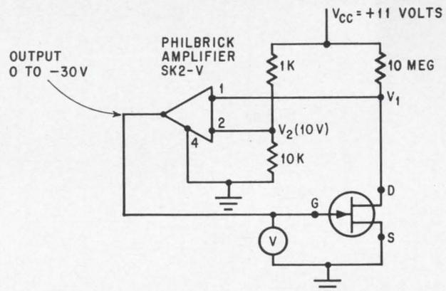
FET drain-to-source pinchoff voltage is obtained indirectly, by measuring gate-to-source voltage that causes  $I_D = 0.1$  microamperes.
