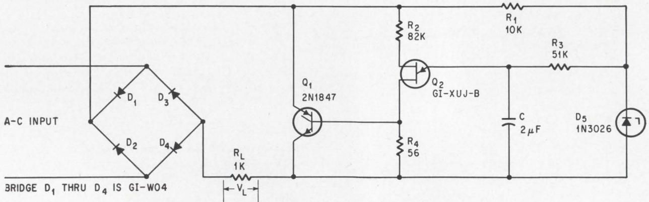
Firing angle of the silicon controlled rectifier varies with amplitude of the input a-c voltage; this variation maintains constant average voltage across load  $R_L$ . Load voltage can be adjusted by changing the value of  $R_L$ .
