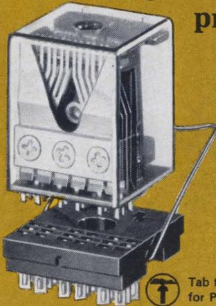
Type LBP Relay sockets offer choice of two terminal styles; elongated-hole solder type terminals for wired assemblies or tab terminals (insert) for PCB mounting. Maximum height for plug-in wired assembly mounting, 1½ inches; for PCB mounting, 1¾ inches. Relay shown actual size.
