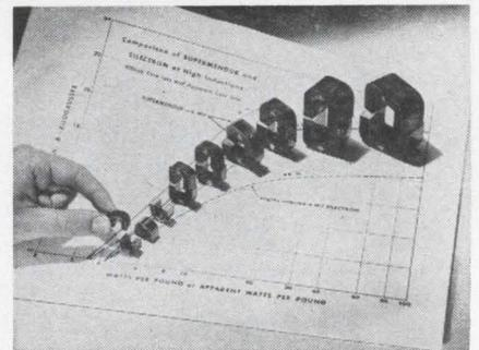
A line of C-cores now on the market is made of Supermendur, a space age alloy of 2% vanadium, 49% iron and 49% cobalt, that permits practical savings in volume from 15% to 40% and weight from 10% to 30%. Performance capability is comparable to C-cores that are ⅓ larger.
