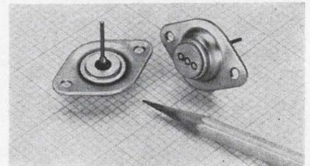
A series of diffused-junction, 25-amp silicon power diodes are mounted in heat sinks identical to the TO-3 case configuration, yet are competitive in price to unmounted press-fit diodes. Designated P50S through P400S, the diodes are rated 25 amps output at  $100^\circ\text{C}$  in piv ratings from 50 to 400 v, and are available in forward or reverse polarity.
