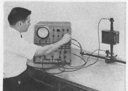
Frequency-response curves and return loss curves, calibrated directly in decibels, are traced out continuously during microwave swept-frequency tests by a plug-in model 1416A for the model 140A oscilloscope.
