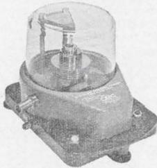
CEC's 6-201 Primary Pressure Standard has long been accepted as the finest of all pneumatic piston gages.
