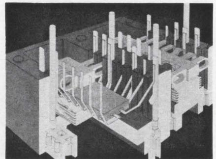
As many as 20 flatpacks and 14 layers of interconnect wiring can be packaged in 1.2 cubic inches with the Omni-Comb interconnection system. The system consists of five basic off-the-shelf parts that can be combined in a prototype or production stage to produce analog or digital subassemblies in practically infinite variety.
