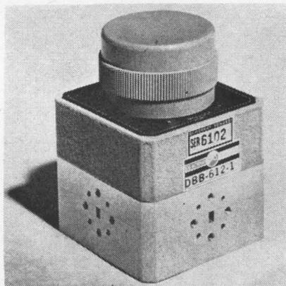
A B size (50 to 75 Gc) manually operated waveguide switch, model DBB-612/614-1, offers maximum insertion loss of 0.2 db, typical isolation of 65 db, and typical vswr of 1. Total weight of the switch is 12 oz. It is 2 in. square by  $2\frac{1}{8}$  in. high. Both single-pole double-throw and double-pole double-throw configurations are available.
