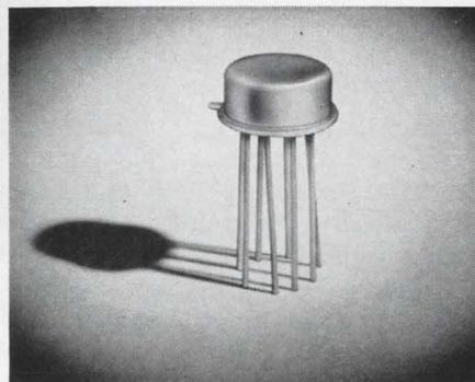
Commercial HLTTL circuits are packaged in this hermetically-welded TO-5 can with 1/2" leads.
