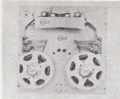
A high-speed photocell punched tape reader and matching tape spooler is announced. The units are designed as input devices for numerical control systems, digital computers, automatic drafting ma-
