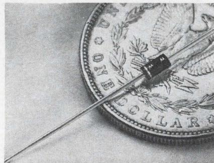
A one-watt zener diode occupies only 0.0016 cubic inches (about the size of a ¼-watt diode) and is priced below one dollar. The IN4728-64 zener series has a 1-w rating at 50°C ambient and is capable of up to 3 w with heat sink. The devices are available in voltages from 3.3 to 100 v in standard tolerances of  $\pm 5\%$  and  $\pm 10\%$ .
