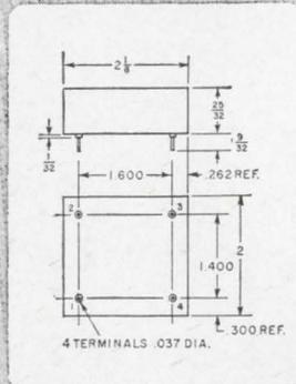
A precision quartz crystal and solid state oscillator circuitry are encapsulated in modules for flat mounting on PC boards. Optimum design assures accurate output by elimination of spurious response and correlation considerations. Frequency Range: 15 kc to 100 mc
