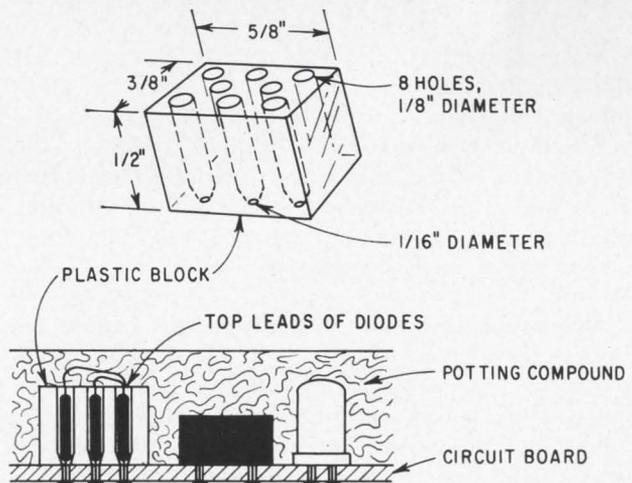
Molded plastic blocks let axial-lead components stand vertically, provide clearance and help in potting. Leads of several diodes can be run through nearby hole.
