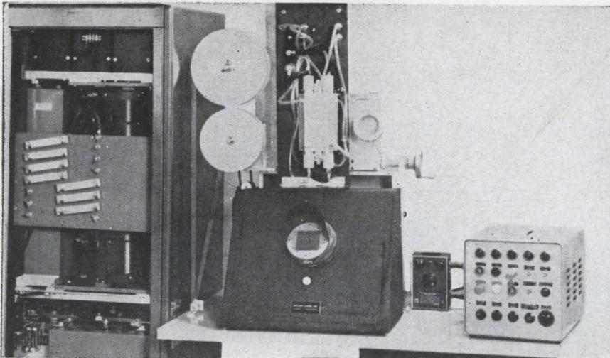
A laser welder that also drills and removes metal has been introduced by Applied Lasers, Inc. To perfect the system, the company had to overcome a problem as old as laser technology: how to vary pulse intensities enough to perform different metalworking tasks.
