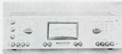
A self-contained instrument, the model B-40 Kelvin bridge comparator, requires no external batteries or external null detectors. Resistance deviations are read directly from the meter without making a null adjustment. The meter ranges are  $\pm 1\%$ ,  $\pm 0.1\%$  and  $\pm 0.01\%$  full scale.
