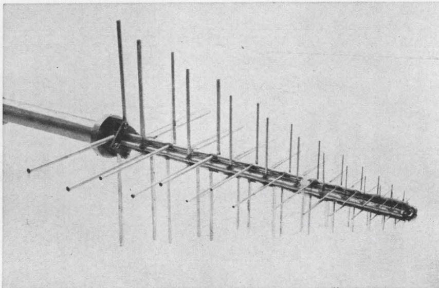
Take two log-periodic antennas, mount them at right angles to each other on a common axis so that their radiation patterns are independent, and the result is an unusually versatile antenna. It combines the broadband characteristic of log-periodics with an ability to provide any field pattern polarization or combination of polarizations.
