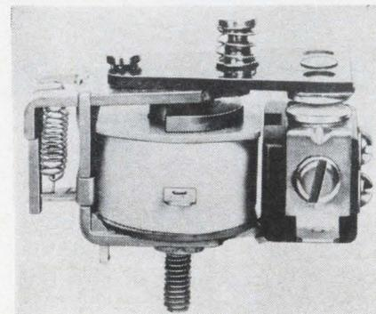
A medium power relay, the 25PD rated at 25 amps, is said to offer greater reliability and better performance than other competitively priced relays. The manufacturer claims extremely long mechanical life for the relay; electrical life is dependent on load characteristics. An important advantage is lower pull-in voltages (d-c: 75% of nominal voltage; a-c: 76% of nominal voltage).
