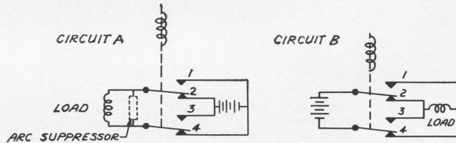
Circuits A and B are both commonly used for reversing polarity, but circuit A has an advantage not often recognized.
