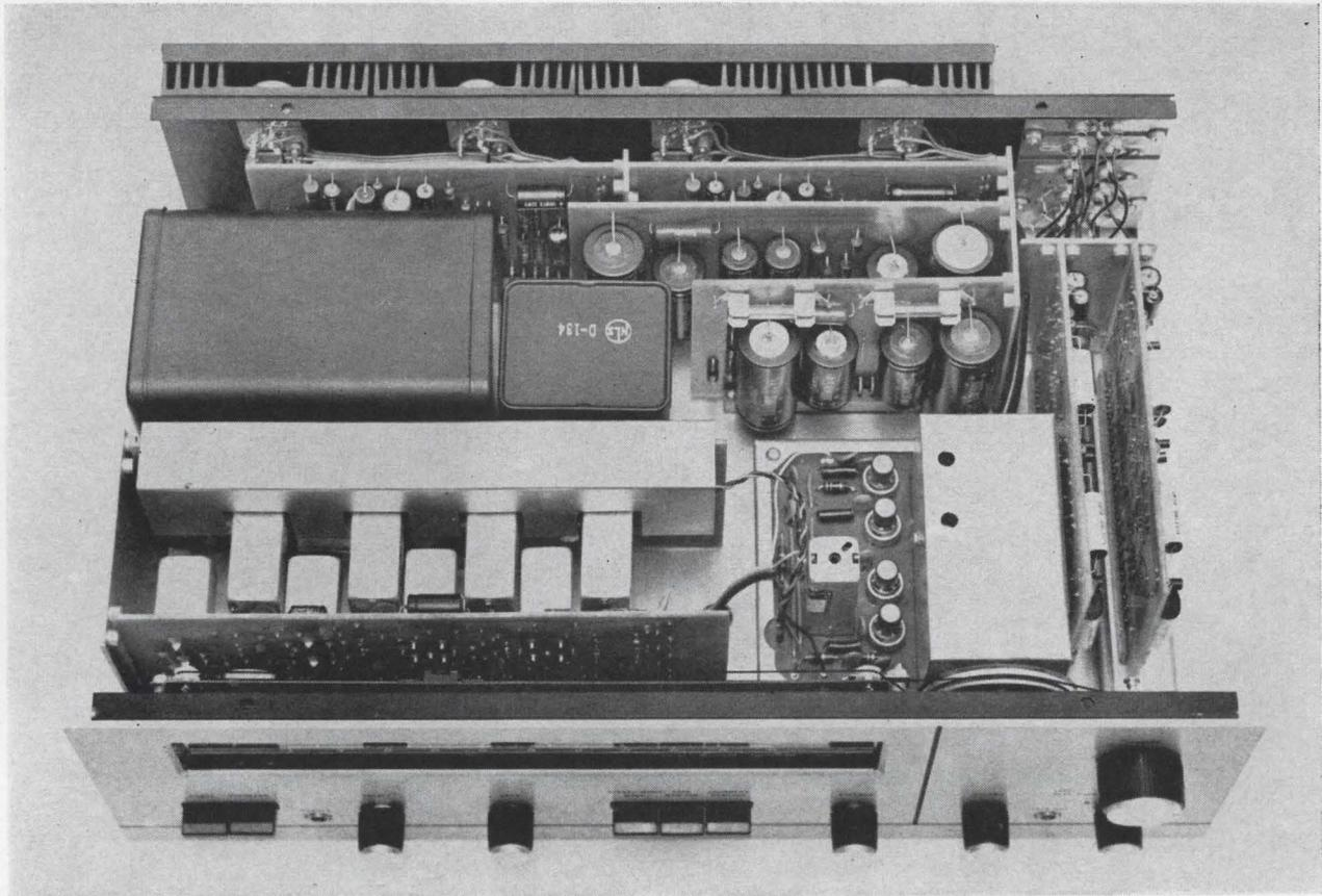
Vertically mounted plug-in printed-circuit boards reduce space requirements. The two cases at upper left are the power and driver transformers. Stereo receiver and dual 40-watt amplifiers fit in 18 in. x 11 in. x 6½ in. cabinet.
