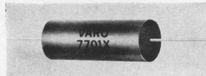
Series 7701X diffused silicon rectifiers is in production, featuring high voltage and fast recovery time. Piv ratings are 2 to 20 kv with a guaranteed reverse recovery time of 300 nsec maximum at forward current of 2 ma and reverse current of 2 ma.
