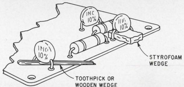
Toothpicks will raise components off board but they must be removed after soldering. Styrofoam blocks, shown on the board at right in the photo above, melt away. Placement of the foam pads is shown in the sketch.
