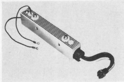
A full-kilowatt, X-band traveling wave tube, the QKW1132, has a unifilar, helix-type wave propagating structure and employs an integral permanent magnet. The rated 1-kw output with an average gain of 40 db applies over the tube's frequency range of 7 to 11 Gc. The conduction-cooled twt is designed for pulse operation with a maximum duty cycle of 0.01. Output vswr is 2:1.
