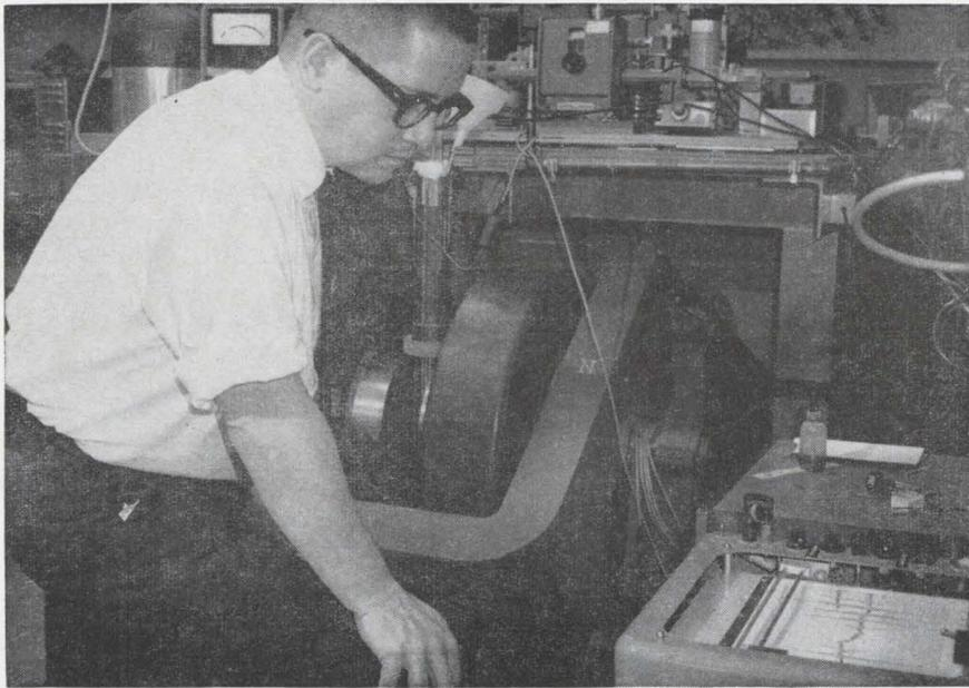
**Scientist watches readout** of electron-spin resonance device (to his left) that is testing a sample of human tissue for cancer. The device detects malignancy because of the peculiar way the diseased tissue reacts in an intensive magnetic field.
