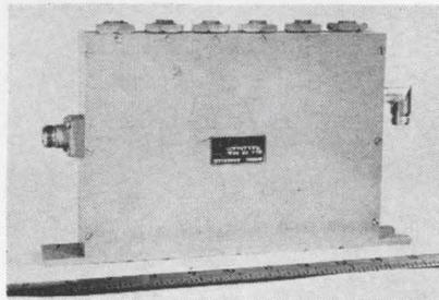
The 500FN series of bandpass filters has a maximum vswr of 1.15 at center frequency and a minimum rejection of 77 db at center frequency  $\pm 13$  Mc.
