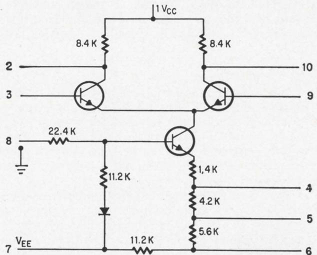
Monolithic differential amplifier MC1525 uses this basic circuit. Additional resistors have been included, which the customer may use or omit depending on the current level of operation. Numbers on the circuit identify leads.
