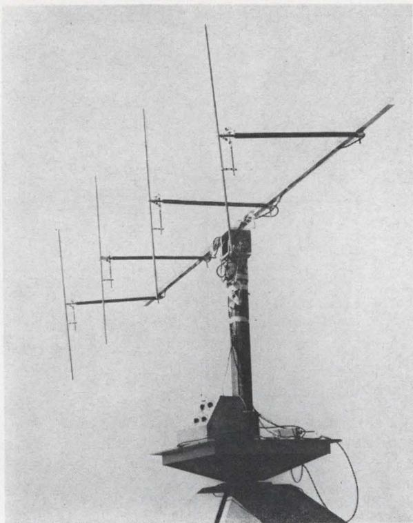
**Steerable-beam array** made up of four antennafer elements spaced a half-wavelength apart. Beam position could be controlled by a series of four ganged potentiometers.
