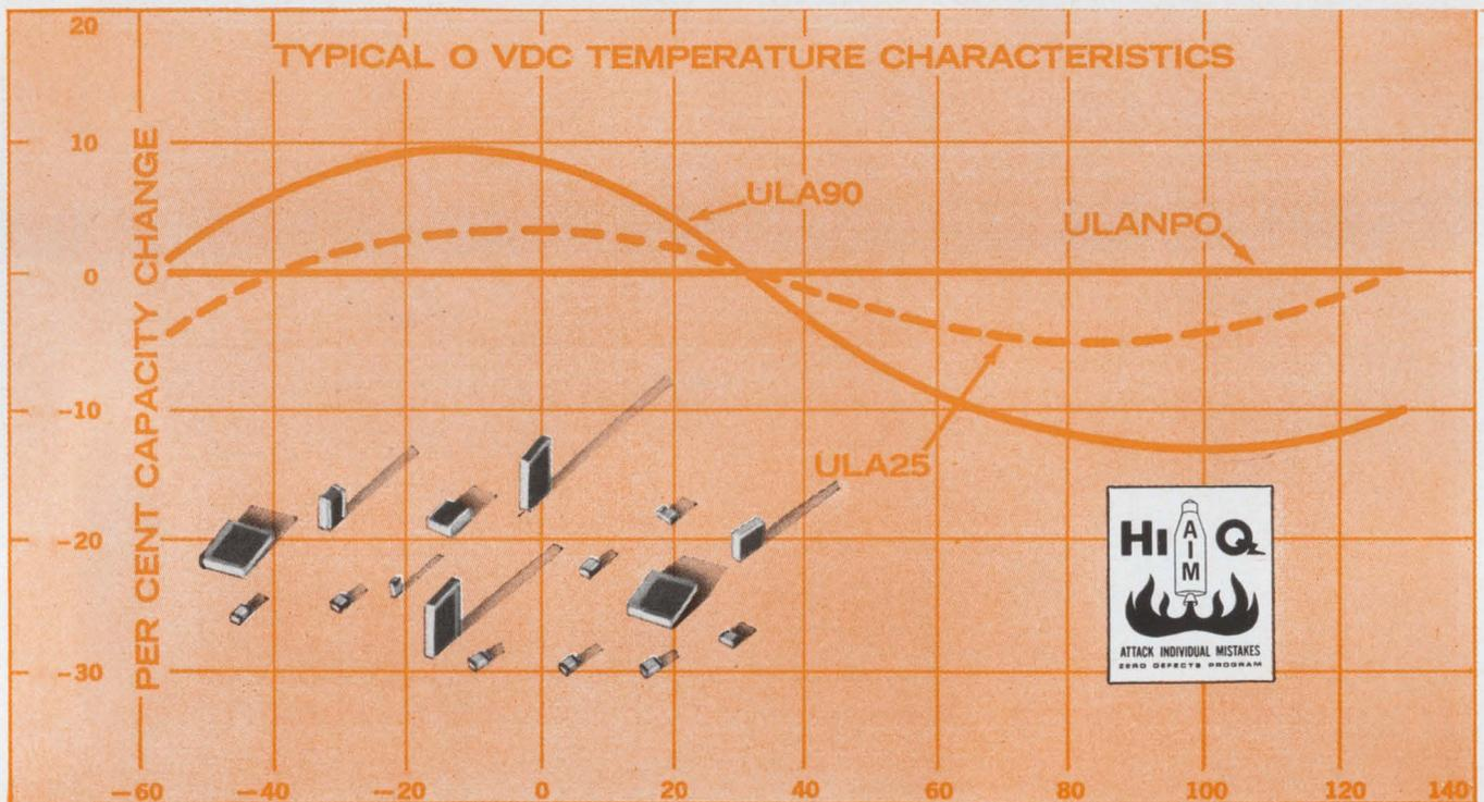
The CERLAM capacitor is a rugged, monolithic block of ceramic dielectric and metallic plate laminated into an extremely dense unit. Because of their unique structure they can be supplied unencapsulated, ready to solder into the circuitry, saving appreciably on volume.
