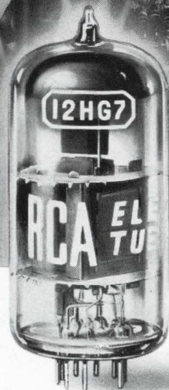
Now, you can eliminate one stage and reduce the number of components in your video-amplifier circuit with the new RCA-12HG7 COLOR-TV RECEIVING TUBE. This FRAME-GRID, Sharp-Cutoff Pentode offers these benefits to the circuit designer:
