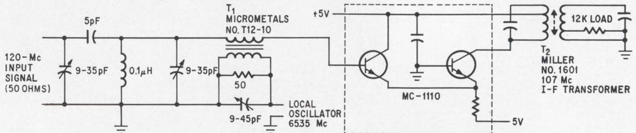
**Differential amplifier integrated circuit used as harmonic mixer.** Local oscillator operates at half of the intended mixing frequency, and odd-order harmonics are canceled in the mixer. Wide separation of oscillator and signal frequencies allows more effective rejection of spurious responses. A conversion gain of 33 db from 120 Mc to 10.7 Mc can be attained with available integrated circuits such as MC-1110. Low-frequency crystals can reduce cost in vhf range.
