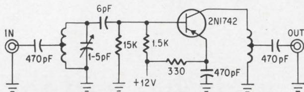
Vhf transistor, which forms the active portion of the dipole antenna, in a test amplifier.
