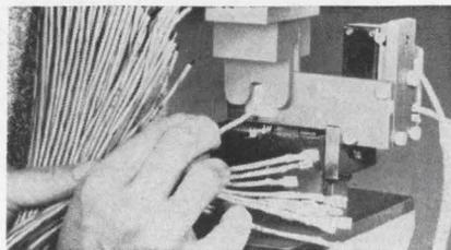
This triggering device is reported to speed up the application of terminals to wires by 40% to 65%. Applicable to wires as fine as 26 gage stranded, the terminal trip device uses a mechanically actuated sensing plate to energize a highly sensitive switch. The switch, in turn, cycles ordinary terminal installation tooling.
