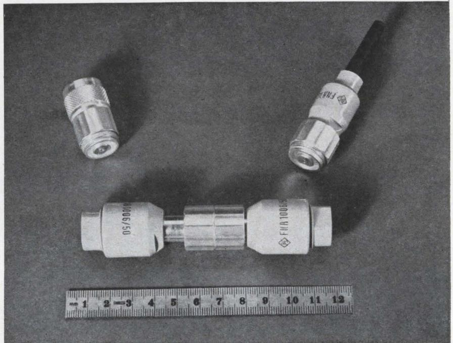
In microwave applications, a coaxial connector has a demanding job, particularly where precise measurements are required. It must withstand thousands of make and break operations and still:
