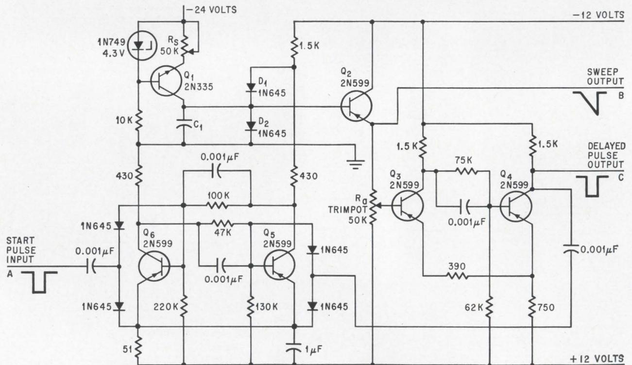
Slow speed sweep generator can be used to keep a camera shutter open to photograph radiation patterns on an oscilloscope. Speed of sweep is determined by  $R_a$  and  $C_1$ .
