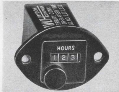
Instantaneous zero reset by a convenient face-mounted push button is featured by these microminiature elapsed time indicators. The units offer a three-digit display of hours or hours and tenths. They may also be allowed to recycle automatically and thus count beyond 999, or 99.9, as applicable, if desired. The indicators are synchronous motor driven.
