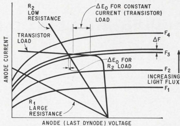
Multiplier phototube characteristics. Sensitivity is greater with a transistor load than with a resistor load.
