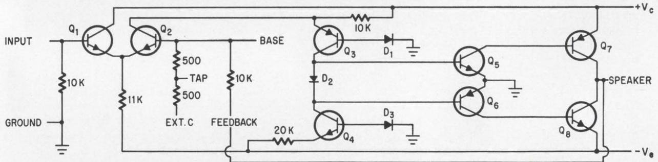
**One-watt integrated-circuit audio amplifier** has negative d-c and a-c feedback applied to one side of a differential input stage; signal is applied to the other side. With balanced power supplies, the output d-c voltage remains at ground potential, allowing a loudspeaker to be driven directly without a large d-c decoupling capacitor. The integrated circuit is the MC1524, a commercially available multi-chip device.
