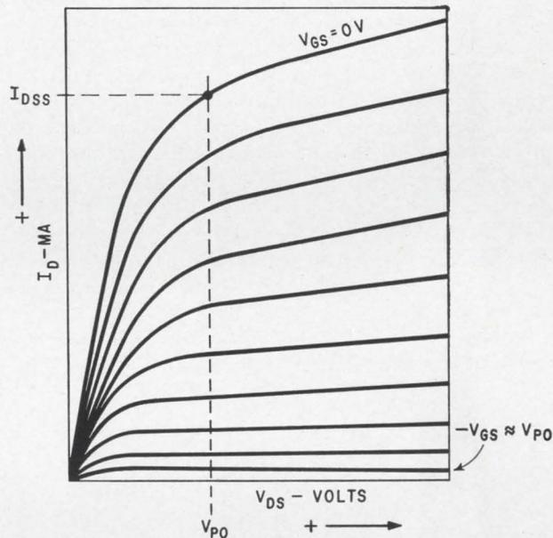
Typical FET drain characteristics.  $V_{PO}$  is drain voltage that causes little or no change in  $I_D$  when  $V_{GS} = 0V$ .
