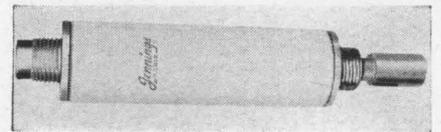
A vacuum switch has been developed for high-voltage r-f switching. Type RP230A is less than  $5\frac{1}{2}$  in. long and  $1\frac{5}{16}$  in. in diameter but it will withstand 50 kv peak test voltage and carry continuous r-f currents of 40 amps rms at 30 Mc. Switch inductance is less than 0.05  $\mu$ h; contact capacitance, only 1.3 pf.
