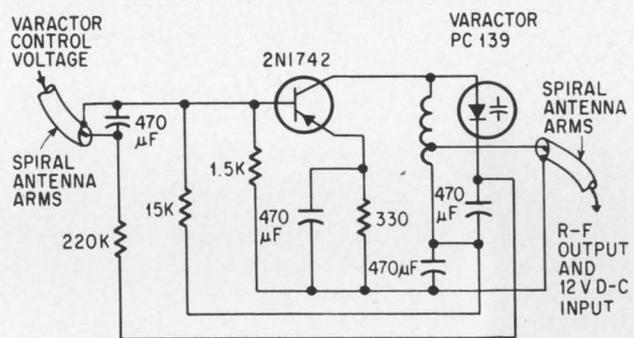
Varactor-tuned transistor amplifier is built into the tip of a conical spiral antenna. Antenna arms are formed by the external sheath of a coaxial cable.
