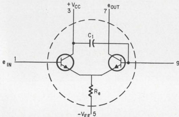
**Simple differential r-f amplifier.** Advantages of this single-ended circuit over a single-transistor tuned stage include higher power gain, negligible parasitic effects, symmetrical transfer characteristics, lower admittance, greater stability, easier alignment and fewer components. One circuit of this type provides a 26-decibel power gain and a 4-decibel noise figure at 100 megacycles. Automatic gain control is easily achieved by varying  $V_{BE}$  which in turn determines the current level.
