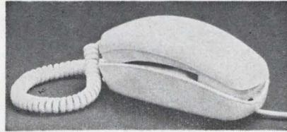
**Dial-in-the-handset telephone** introduced by Bell System. Printed circuit fits into curved handset, which weighs only two ounces more than a conventional handset but contains the dial, wires, other gear.
