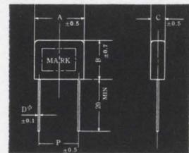
50 volts D.C. Working unit: mm
