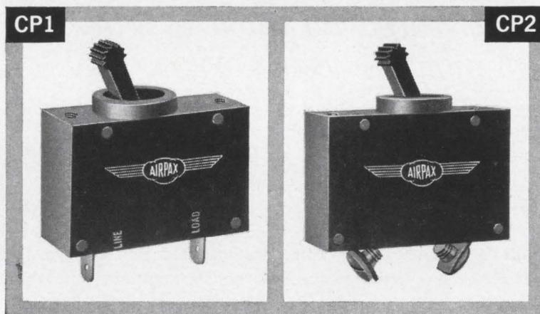
The Type CP electromagnetic circuit protector is Underwriters' Laboratory tested and recognized for motor and appliance protection. ■ This low cost protector is for use with loads up to 20 amps at 32 volts DC, 7½ amps at 250 volts AC and 15 amps at 125 volts AC. ■ CP protectors may be supplied with instantaneous, fast or slow trip characteristics. Current ratings down to 50 ma permit use in electronic circuits and instruments.
