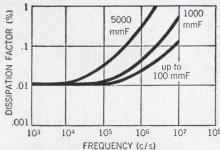
**Low dissipation factor** (usually even lower than for mica capacitors) is provided by Styroflex capacitors... making them specially suitable for filter circuits.
