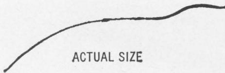
we start with tungsten wire .0005" and draw copper tubing over it at .0036" diameter. Wall thickness is .0015".
