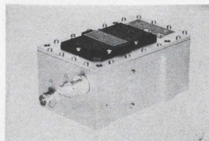
Combining solid state devices and vacuum tubes for optimum reliability, this cavity amplifier delivers 30 watts output power in a severe aerospace environment. The 30-ounce unit operates at signal frequencies from 215 to 265 Mc. Gain is 10 db minimum.
