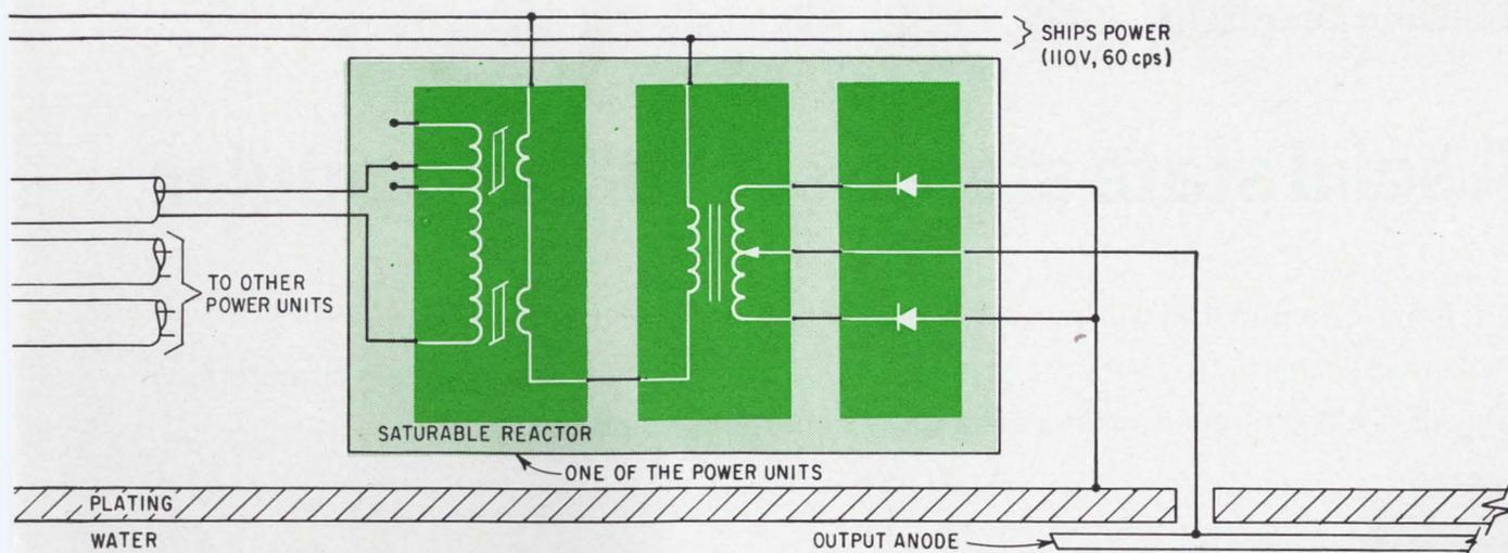
magnetic amplifier chain raises the power level to the several kilovolt-ampere level needed to drive the output anodes. These anodes supply the ion-current flow in the sea water that interacts with the ship's hull to change its voltage several hundred millivolts. The feedback sensor electrode measures the actual hull-seawater voltage differential.
