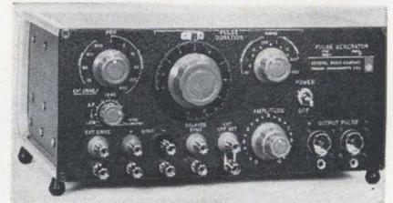
Type 1398-A pulse generator is a self-contained, general-purpose pulse source featuring rise and fall times under 5 nsec, 60-ma positive and negative pulses that can be supplied simultaneously, a prf range from 2.5 cps to 1.2 Mc, and a duration range of 0.1  $\mu$ sec to 1.1 sec. Positive and negative 8-volt, 150-nsec prepulses and a delayed-sync pulse are also supplied at front-panel terminals.
