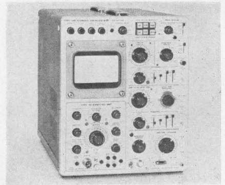
Type 549 oscilloscope combines the features of the 545B with the added versatility of storage capability. It has what is believed to be the fastest-writing bistable storage crt. The 6-cm by 10-cm display area is divided into two 3-cm by 10-cm independently controlled targets for split-screen applications, plus a nonstoring "locate" zone at the left and a "run-over" storage area at the right.
