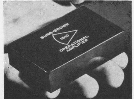
An all-silicon d-c operational amplifier, model 1510, has a bandwidth of 30 Mc with full power response to 1 Mc and a slewing rate of 100 v per  $\mu$ sec. Output is  $\pm 10$  v at 30 ma with only 12 ma quiescent drain from the nominal  $\pm 15$  v external power supply. D-c gain of 30,000 and stability of  $\pm 10$   $\mu$ v/ $^{\circ}$ C and  $\pm 0.5$  na/ $^{\circ}$ C are typical.
