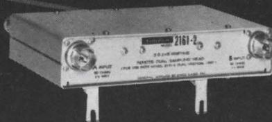
**REMOTE** dual feedthrough sampling head (for the Lumatron Model 120A Sampling Oscilloscope) brings the sampling to *your circuit*, eliminating hookup cable losses and distortions. You measure what is actually taking place at your circuit. In addition, the *straight* feedthrough coax is free of distortions caused by elbow bends.
