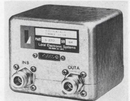
A series of tracked/isolated YIG electronically tunable microwave filters are said to offer lower insertion loss, improved tracking characteristics, broader bandpass and lighter weight than those introduced by the manufacturer a year ago. The 2200 series units provide two r-f filter sections within the same magnetic tuning structure—a concept that enables the units to be used in advanced electronic equipment, such as doppler radars, ecm/ecm systems and frequency agility radars.
