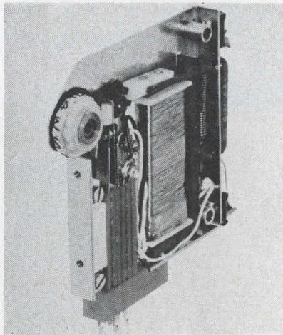
Model WR-25 single decade printer incorporates an escape mechanism that permits the counter to be zeroed with only one 400-msec pulse. Presently, all similarly designed printers must provide a series of pulses in order to be zeroed.
