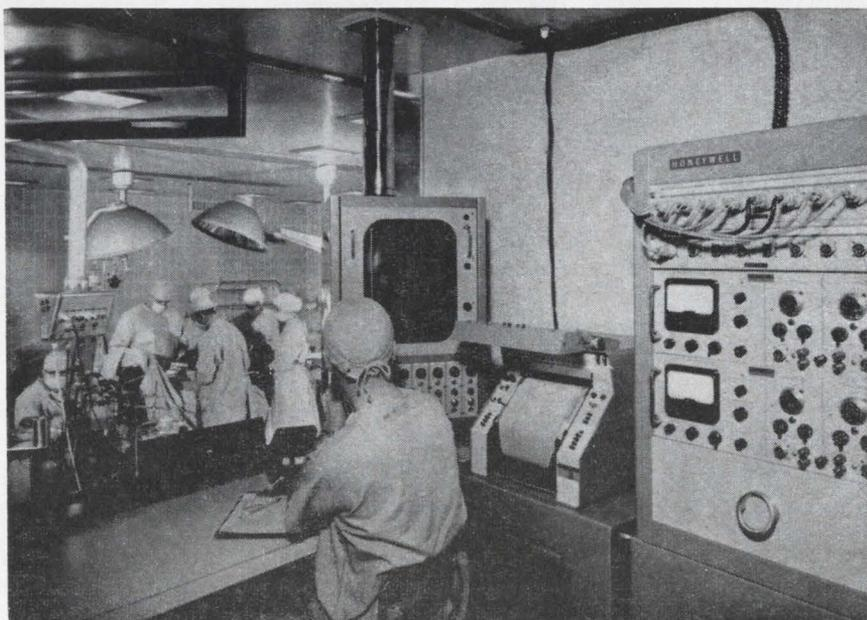
**During heart operation,** condition of the heart is monitored by doctor (foreground) on the oscilloscope in front of him. The graphic recorder at his right makes a permanent record.
