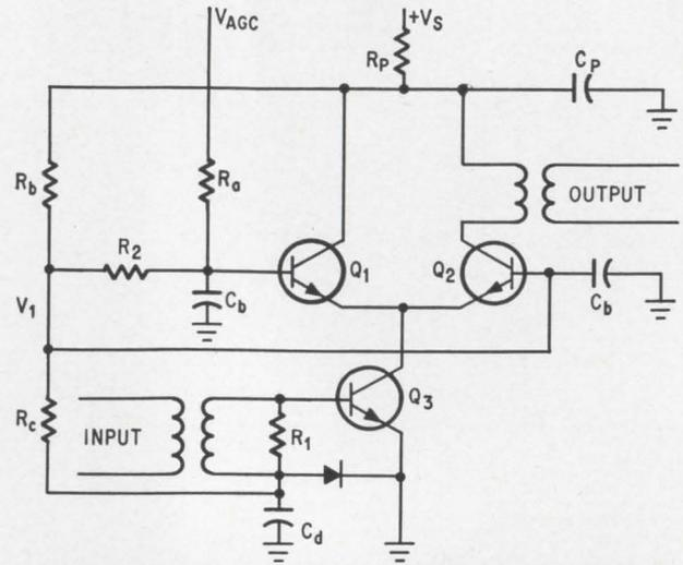
**This circuit maintains constant impedance levels while shunting the signal into either the output transistor or the non-output side of a differential pair.** This minimizes problem of bandwidth variation and interstage detuning with automatic gain control in tuned i-f cascade amplifiers. The AGC, applied as a differential d-c voltage between the bases, determines the amount of signal shunted to each side. Stage gain is 20 db at 60 Mc.
