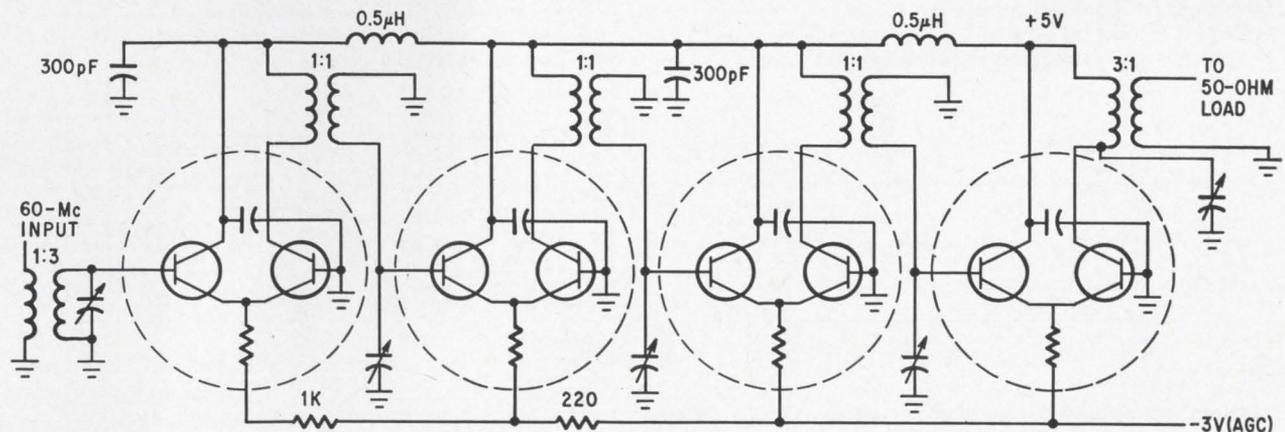
60-Mc intermediate-frequency f-m limiter formed by four differential-amplifier integrated circuits. The circuit provides 80-db power gain at 60 Mc, with a 6-Mc bandwidth and a 6-db noise figure. With microminiature toroid transformers and compact trimmer capacitors, the entire i-f strip package is about 0.2 by 1.2 by 2.3 inches.
