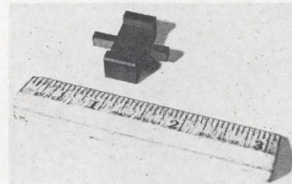
These fixed attenuator pads cover EIA waveguide sizes WR28 to WR90. The units, spanning the frequency range 8.5 to 37 Gc, have a maximum vswr in most cases of 1.20 or less and find wide application in test bench set-ups and local oscillator portions of waveguide subassemblies due to their compact size and excellent electrical characteristics.
