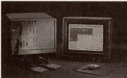
three independent timing generators (stimulus, response, and control). Tests can be synchronized with other equipment for mixed-signal testing.
