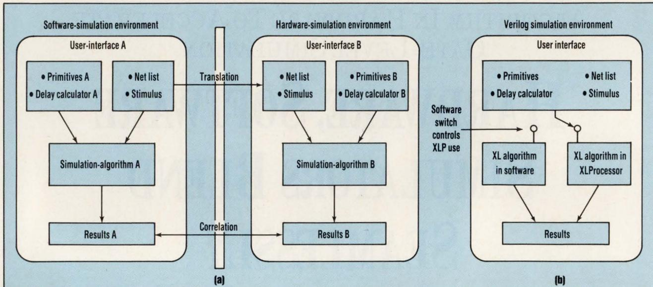
**THE SEAM BETWEEN** hardware- and software-simulation environments caused by different user interfaces, simulation algorithms, primitives, and delay calculators can produce different results and incur a large amount of overhead (a). The Verilog environment has no seam because the hardware and software simulators use the same primitives, delay calculator, net list, stimulus, and user interface. A software switch determines if the simulation is sent to the hardware accelerator (b).
