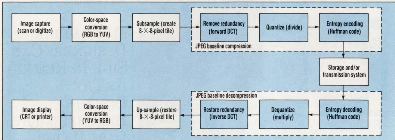
**1. THE JPEG BASELINE ALGORITHM** can be augmented with optional functions for applications needing additional compression and decompression features. The extended system enables the encoder to handle pixels with greater than 8-bit precision, additional data-interleaving schemes, and more color components. It also provides arithmetic coding for up to 10% better compression, and progressive build-up to successively improve an image as more data becomes available.
