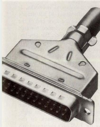
3. Among the elements of a shielded connector are its metal shell with 360° cable-shield termination, high-conductivity backshell/shield material, 360° backshell-to-connector contact, and grounding indents on the connector-mating face.
