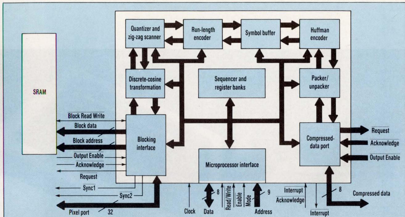
**2. THE STI140 CODEC** receives raster-scanned data through its 32-bit pixel port at up to 27 Mpixels/s. After JPEG processing by the codec, compressed data exits through an 8-bit port at the same data rate for synchronous or asynchronous operation.
