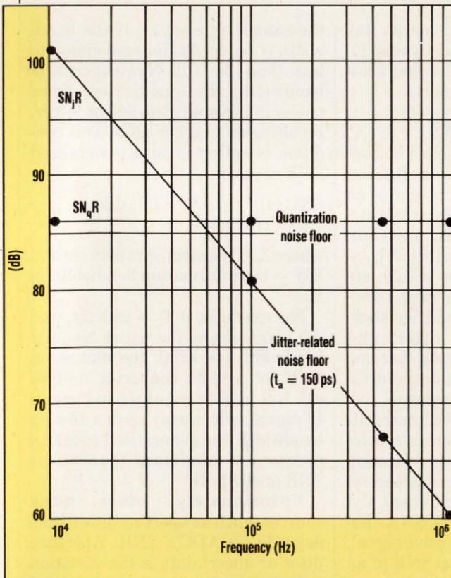
**5. DESIGNERS CAN PREDICT** the theoretical limits of the rms-signal-to-rms-aperture-jitter noise ratio, SN<sub>J,R</sub>. For an rms aperture uncertainty,  $t_a$ , of 150 ps, performance begins to degrade above 53 kHz, approximately. Also shown on this plot is the maximum SNR that can be achieved if only quantization noise is considered.
