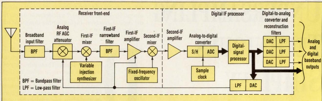
**2. BY USING DIGITAL COMPONENTS** (including a software-reconfigurable digital-signal processor) after the second IF amplifier, designers can simplify the receiver circuit and reduce costs.
