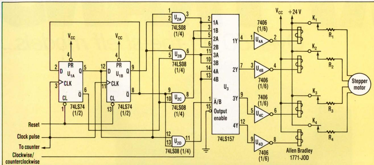
**THIS CIRCUIT IS A REVISION** of a previously published bidirectional stepper-motor sequencer. The new circuit uses four chips, with an option of using just three (the flip-flops and AND gates can be combined). The rate of clock pulses determines the motor's rpm. Switching transistors can replace the relays to increase the circuit's efficiency.
