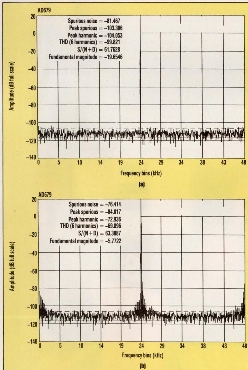
**6. LOOKING AT A CONVERTER'S OUTPUT** using fast Fourier transforms shows how noise and linearity specifications are affected by the magnitude of the input signal. These examples show the difference for inputs 19.6546 dB below full scale (a) and 5.7722 dB below full scale (b).
