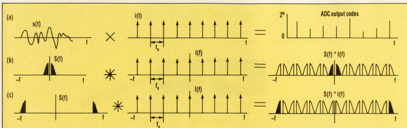
**3. IN THE TIME DOMAIN**, sampling is the multiplication of the analog signal and an impulse train with the same period as the sample clock (a). The equivalent in the frequency domain is convolution (b). If the analog signal is bandlimited to be less than one-half the sampling rate and doesn't cross a multiple of the sample clock, the converter can undersample the signal without causing aliasing (c).
