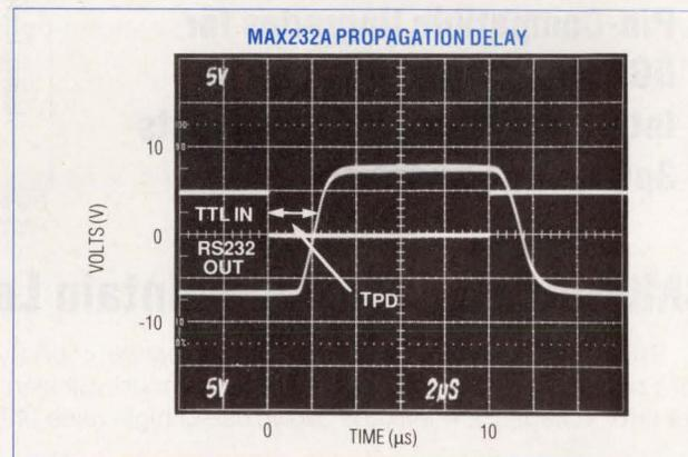
The MAX232A improves propagation delay and symmetry.
