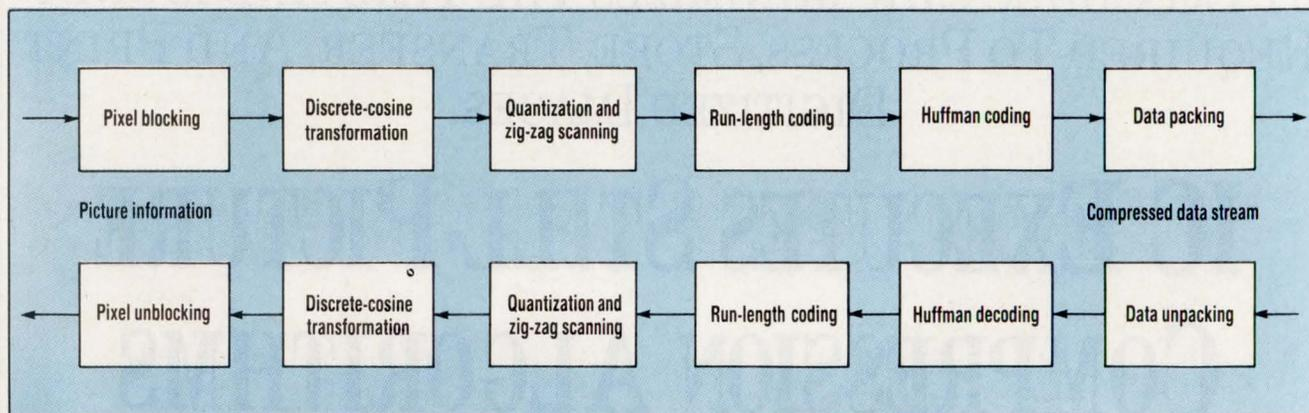
**1. THE JPEG ALGORITHM** performs pixel blocking, discrete-cosine transformation (DCT), and quantization coding. That's followed by a compression of the serial bit stream using run-length coding (RLC) and Huffman encoding. Marker codes inserted into the JPEG bit stream ensures agreement between encoder and decoder.
