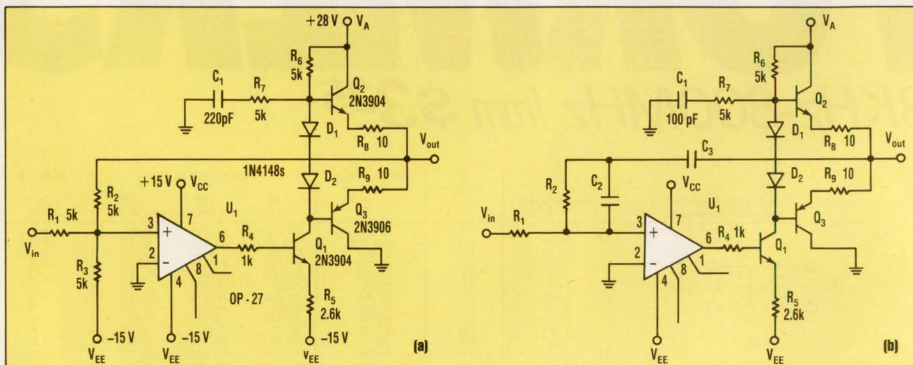
**THE OP AMP (U<sub>1</sub>) IN THIS CIRCUIT** operates from a standard  $\pm 15\text{-V}$  supply and its output is scaled from 5 to 25 V (a). With a slight modification, the circuit becomes an active lead-lag filter that can drive an rf or microwave voltage-controlled oscillator directly (b).
