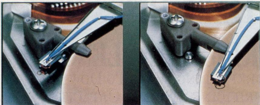
**2. THE RAMP-LOADING TECHNIQUE**, designed by PrairieTek, increases the drive's reliability by keeping the head from making contact with the disk. The head lays on the plastic surface when the disk is turned off.
