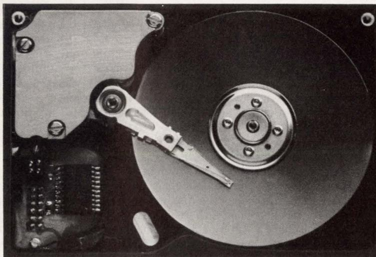
**1. CONTAINED IN A PACKAGE** that's about 2-3/4 by 4 in. (shown here in actual size), Seagate's ST9051A drive holds 40 Mbytes of data. The media is made of thin-film aluminum. The drive uses just 0.5 W in the standby mode.
