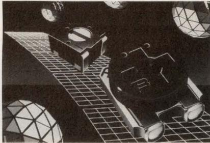
the devices with temporary seals that were either punctured or peeled off before adjustment, leaving the trimmer vulnerable to contaminants. The unit has the same resistance range as the 3-mm trimmer. Maximum CRV is 3%.
