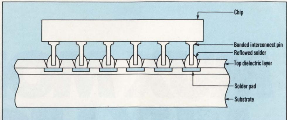
the sites. Then, the BIP chip is placed in position on the substrate and reflow-soldered to the interconnection sites.
