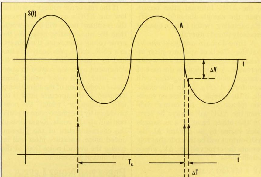
**4. THIS EXAMPLE OF A SINE WAVE** sampled by a clock of period  $T_s$  shows how the effects of aperture jitter increase with the input's slew rate. For a given jitter ( $\Delta t$ ), the voltage error ( $\Delta V$ ) increases as the slew rate increases.
