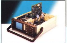
Designed for easy service. PM 3050 was designed to make any required service fast and simple. Swing-up PCBs make access easy, and flat ribbon cables allow instant disconnection. Each oscilloscope has a complete, built-in testing routine, to provide a quick assurance of correct operation.
