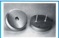
**LOW COST PIEZO SOUND TRANSDUCERS** MS-3 sound transducers are pre-assembled & pre-tested—for PC board insertion. Stainless steel & glass-filled polyester constr. Exclusive soldered crystal contacts for max reliability. Generates 70 to 80 dBA (2-5 kHz) at 2 ft. Freq., volume & mode are functions of drive circuitry you supply. 930" dia. × .255". Made in USA. 42¢ ea/1000 qty. **Floyd Bell Inc.**, 987 Higgs Ave., PO Box 12327, Columbus, OH 43212. 614/488-3193.
