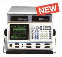
**NEW K450.** All high-speed channels: 10ns (100 MHz) across 48 channels or 5ns (200 MHz) across 24 channels. 5ns glitch capture on all channels with no loss of memory. 4K memory depth. Unique Auto Save for saving failures in unattended mode.
