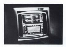
draws and edits schematics, handles hierarchical designs, automatically generates net lists, and checks rules. A built-in project manager takes care of back annotation. Together with the Apollo 3000, it costs \$19,400 for monochrome and \$27,300 for color versions.
