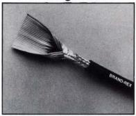
A line of FRF (flat-to-round-toflat) mass termination cables consists of 28 AWG stranded tinned copper conductors on 0.050-in. centers of 300-V PVC. The core of each cable, designated T-11302, is wrapped with an inner layer of aluminum/polyester and an outer braid of tinned copper, which results in a shield effectiveness of 70 dB at 100 MHz. A black flexible PVC jacket is extruded overall. Insulation resistance is greater than 10 M $\Omega$ (10 ft).
