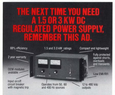
Delivering 1.5 or 3kW at 12 to 480 Vdc, these units are especially designed for high-power applications where tight regulation, low-ripple and high efficiency are critical. Features include: light weight, low panel height and high MTBF. Unique modular design and circuitry permit custom modification. Available rack-mountable or as OEM modules. Single or 3-phase. Call for complete details and custom design capabilities: 516-671-4400.
