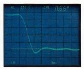
Overshoot and ringing measurement accuracy requires flat response in a probe/oscilloscope system. Tek probes and scopes are designed to work together.
