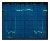
Calculated frequency takes only seconds. The time cursor measurement on the left can be converted to frequency with push-button ease and 1% accuracy.
