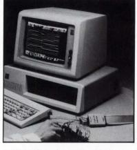
A 20-MHz logic analyzer has a 2-ns setup time, 10 to 15 times faster than most comparable units. Further, through an optional Doubler pod, the Logic-20 is capable of 40-MHz sampling over eight channels at double the standard 16-by-256-bit memory depth. The entire 16-channel system is incorporated into a single IBM PC expansion card and uses the computer as its controller.
