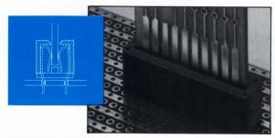
**DIGI-KLIP** MDR 100 Series gives you the edge with its exclusive, semi-bellows, beryllium copper wireform contacts that are heat treated AFTER forming for optimum spring temper, virtually eliminating field failures due to stress relaxation or contact "sag".
