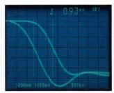
Propagation delay measurement accuracy is assured by built-in propagation delay matching. Delay between Channels 1 and 2 can be corrected to the probe tip.
