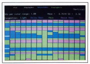
1. Congestion on a gate array as originally laid out shows up in red (left). But General Electric's ICmove can step in to produce a more easily routed layout (right).
