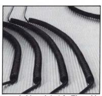
extended length is 6 ft. The cable consists of seven 26 AWG tinned copper, polypropylene-insulated conductors. These are covered with a Beldfoil aluminum/polyester shield and tinned copper spiral shield and a polyurethane jacket.
