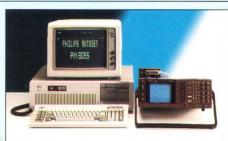
Fast computer hook-up. An add-on IEEE-bus option provides fast hook-up to a computer or controller, for use in ATE environments, quality control systems, training and many more applications. The ingenious separate IEEE option is readily interchangeable for automated scope calibration.
