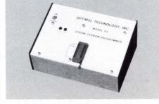
EPROM PROGRAMMER Model 93 with RS-232, 300 to 19.2K baud, hardware handshake, ACK/NAK. Compact instruction set including checksum, silicon identifiers supports 2758-27513, 2508-2564, MCM68764, new Intel Quick Pulse EPROMs; 2816A-28256 EEPROMS; 8748, 8749 and 8751 MPU. Formats include Intel, TEK-HEX, S-code, and ASCII for read, write, split byte commands. Price \$550, software MS-DOS, CP/M \$40. **Optimal Technology**, Earlysville, Va. 22936 804-973-
