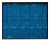
A period measurement is made on a 100 MHz clock using the extended accuracy and resolution of the Counter/Timer/ Trigger in the 2465 DVS.
