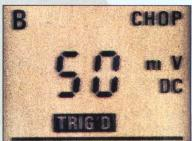
Versatile triggering functions up to 100 MHz. The PM 3050 family 'scopes have all the regular functions of auto, manual and single-shot triggering, plus smart, secure microcomputer control that 'thinks for you' in auto-triggering mode. Trigger bandwidth is an unmatched 100 MHz.
