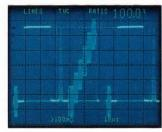
Calibrate cursors in IRE units with variable attenuation. Blanking level to reference white level is defined as 100 IRE units in NTSC video.
