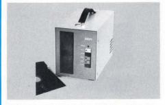
IBM PC COMPATIBLE RS232 EASI-DISK 51/4" FLOPPY DATA STORAGE & TRANSFER SYSTEM
