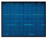
The Word Recognizer (with a binary word) is used to pick out a pulse train in a data stream. The time cursors measure pulse train duration.
