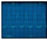
A frequency measurement is made with the same high precision. Simply press two buttons, and the period measurement on the left is converted to frequency.
