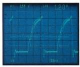
**Logic-level violations** can be spotted quickly on a TTL waveform (above) with measurement cursors set to define logic-level boundaries.
