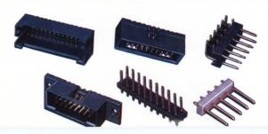
Shrouded and unshrouded headers include complaint pin versions for solderless insertion. Choose .025" x .025" or .031" x .062" post sizes, in single and double row configurations.
