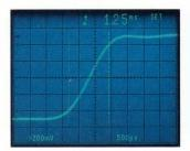
This fast-pulse rise time is nearly that of the scope. The 2465 achieves maximum bandwidth with minimum waveform aberrations. This level of pulse
