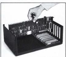
Put the power of the IBM PC into your OEM system with the new I-Bus Single Board Computer and Enclosures. Now you can make use of that vast array of PC-compatible expansion cards—for communications, graphics, data acquisition, peripheral control, and every other imaginable task.
