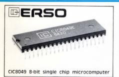
FIRST IN SOUTHEAST ASIA. FEATURES NMOS Technology • Internal Memory-2K × 8 ROM • 128 × 8 RAM • Internal Timer/Event Counter • Single level interrupt • Single 5-volt supply • Over 90 instructions. 70% Single Byte • Timer/counter interrupt available • Reduced Power Consumption • Compatible with Intel's MCS-80/85 peripherals • Easily Expandable Memory and I/O • Up to 1.36 µsec instruction cycle (11 MHz operation), all instructions 1 or 2 cycles. ERSO/ITRI
