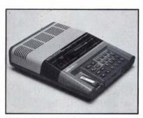
The Model 21A programs over 120 different MOS and CMOS EPROMs and EEPROMs having densities of up to 256k. At \$1450, the unit offers a variety of features that are commonly found only in higher-priced programmers.
