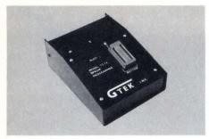
GTEK's Model 7228 (E)EPROM Programmer features Intelligent Programming Algorithms and supports the newest devices available through 512 Kbits and programs 6x as fast as standard algorithms. The 7228 programs the 2764 in one minute! It supports Intel 2764A and 27128A chips. It also supports Tektronics, Intel, Motorola and other formats. Priced at just \$549. GTEK, Inc., P.O. Box 289, Waveland, MS 39576; 601-467-8048.
