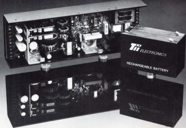
Optional battery backup in a switching power supply - a unique idea? Not according to our customers. With an EHVQ™ in your UNIX™ based system, lost data bases are a thing of the past. Our battery backup board has enough status signals to make interface with any operating system an easy job for hardware and software designers.
