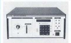
Vii's 2501 Video Generator is programmable providing a full range of test patterns at virtually any scan rate. Using keyboard entry in real numbers, it stores all pulse and proportion parameters for up to 69 raster formats, permanent EEPROM data storage, user-friendly with 16-character display with complete support manual. Only \$4950. Contact your Vii Rep or send for literature: Vii, P.O. Box 33, Xenia, OH 45385-0033. Telephone: 513-376-4361
