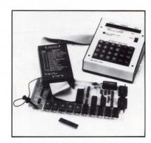
esigned to provide engineers with a portable stand-alone instrument for developing, testing, and maintaining 6502-based hardware and software, the DA6502-B in-circuit emulator costs less than \$600—considerably lower than comparable units. With the DA6502-B, the user can examine processor registers, read and modify memory locations, halt a program at a specific address, step through a program one instruction at a time, and stop a program at a location after a number of loops have been completed.
