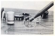
TP-102 SERIES SINGLE HOLE, PC MOUNTED TEST POINTS. • Direct replacement alternative to expensive "turret" type terminals. • Two styles accommodate complete range of popular "turret" hole diameters. • Spring tempered, flaired leads eliminate secondary staking operations. • Accepts all commonly used spring loaded test probes and clips. • Cunistan® alloy, comparable spring quality and strength to beryllium copper at less cost. COM-PONENTS CORP., 6 Kinsey Place, Denville, NJ 07834. (201) 627-0290.
