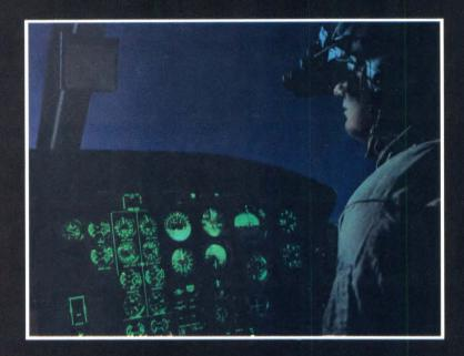
The new Vivisun 20/20 switches make a pilot's mission safer by night and easier by day. A unique optics system eliminates the veiling glare and halo effect that would interfere with ANVIS night vision goggles. When voltages are trimmed to night vision goggle flying levels, Vivisun 20/20 switches can still be read with the unaided eye.
