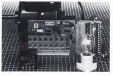
Analog and Power Control I/O...in a Single Board Computer. 6801 Micro Control System designed for DISTRIBUTED CONTROL or STAND-ALONE use: 6801 or 68701 MPU with 2K ROM or EPROM, 128 RAM, timer. Eight 12-bit analog inputs, 8-bit analog output, 8 AC or DC inputs or outputs, serial I/O, digital I/O, power supply. Wintek Corporation, 1801 South Street, Lafayette, IN 47904-2993. (317) 742-8428.
