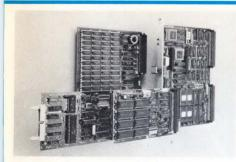
VME 68000 FAMILY MODULES Full MOTOROLA compatible but reinforced 8MHz/10MHz CPU modules with battery backed-up RTC & onboard CMOS RAM, 512KB and 2MB DRAM memory modules. Static 64KB RAM, ROM, Floppy I/F, Hard Disk I/F, Serial I/F modules. AMPERE, INC. Asahi Bldg., 5-chome, Nishi-Shirijuku, Shirijuku-ku, Tokyo Japan Telex J33101 AMPERE PHONE 03-365-0825.
