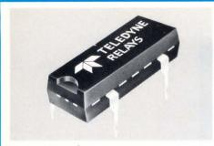
SOLID STATE AC/DC RELAY Teledyne's 640-1 is a solid state pin compatible replacement for DIP reed relays where higher reliability and long life are required. Switches AC or DC up to 50V. Low onresistance is 2 ohms. Control voltage range is 3.8 to 10VDC. Transformer coupling provides 1500 (P-P) isolation, low off-state leakage, & high switching speed. Employs hybrid microcircuits in TO-116 DIP. \$6.15 ea for 5000 pcs. Teledyne Relays, 12525 Daphne Ave, Hawthorne, CA 90250 (213) 777-0077
