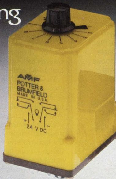
**CMOS controlled CG time delay.** Standard delays range from 0.1-1 sec. to 10-100 min. Delays to one year or more available. Repeatability is typically .05% for DC units, 0.1% for AC, including the first cycle! DPDT contacts rated 10 amps at 120V AC. Delay on operate, interval on or delay on release models.
