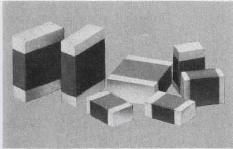
**HIGH Q MULTILAYER CAPACITORS** feature very high quality factors at microwave frequencies. Offered in three standard sizes: .050 x .040, .080 x .050, .125 x .095. Capacitance values from 0.1 pf to 1000 pf with close tolerance and voltages to 1000 VDCW. Johanson/Monolithic Dielectrics Div., Box 6456, Burbank, Ca. 91510, (213) 848-4465.
