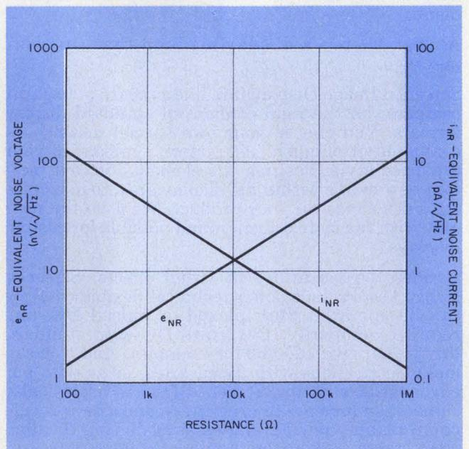
2. The equivalent noise voltage ( $e_{nR}$ ) and equivalent noise current ( $i_{nR}$ ) of a resistor may be quickly selected from this chart.
