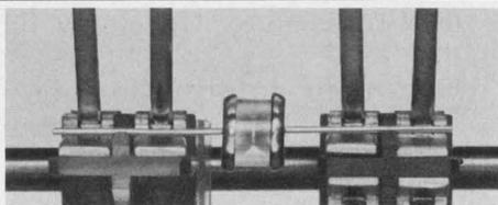
Companion Component Test Fixture, KeyTek Model 450, is shown holding a gas tube surge protector. The Model 450 provides fast, safe, 4-wire connections for both axial and radial lead components.
