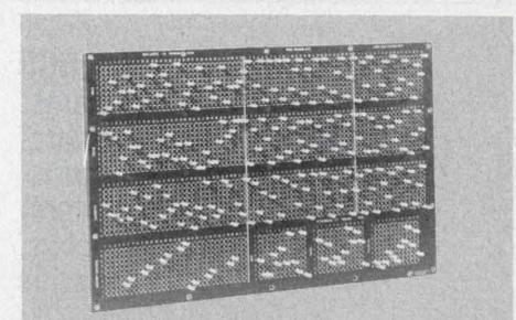
**Matrix Program Boards** designed to custom specification, provide a reliable and simple method for connecting complex networks while maintaining maximum switching flexibility. Units can be supplied on either .250, .125 or .100 centerlines, with up to 15,000 crosspoints; both Shorting and Diode Pins are available. Pricing for special prototype quantities starts at \$ .15 per crosspoint, delivery 4-6 weeks ARO. LVC Industries Inc., 135-25 37th Avenue, Flushing, New York 11354, (212) 939-9777.
