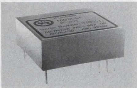
**Model P203 ultrasonic pulser module** drives piezoelectric transducers. Simplify ultrasonic system design. High energy negative spike output pulse typically has 7 nanosecond risetime and 230 volt amplitude into 50 ohms. Pulse repetition rate variable to over 10 kHz. TTL compatible sync output and external positive and negative trigger inputs. Operating temperature -40 to +70°C. Plug-in module measures 2.0 x 1.8 x 0.68 inches. METRO-TEK, INC., P.O. Box 101, Richland, WA. 99352. (509) 946-4778.
