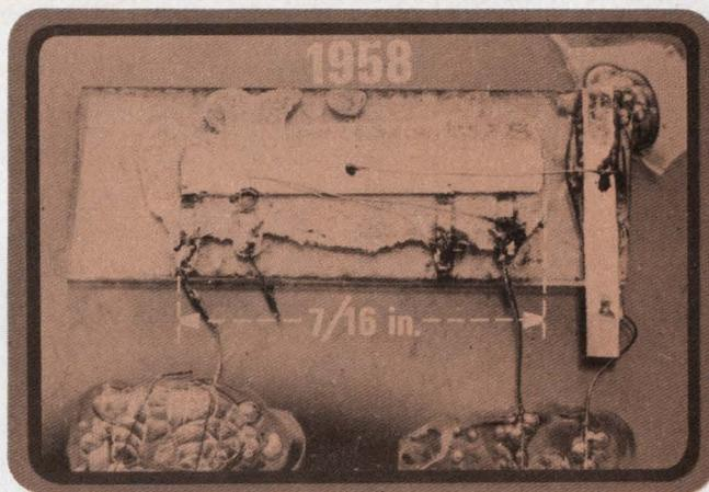
The first integrated circuit, developed by Jack Kilby at Texas Instruments, paved the way for today's pocket-sized computers and for men travelling to the moon.
