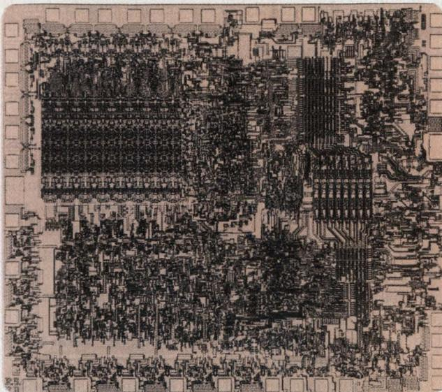
**Not quite computers on chips**, microprocessors do perform many of the functions of central processing units in conventional computers. The first emerged from Intel in 1971. It was a 4-bit unit called the 4004 (left). The
