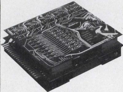
New Model ADC1215F converter from Phoenix Data is available in two basic models: Single-ended and differential.
