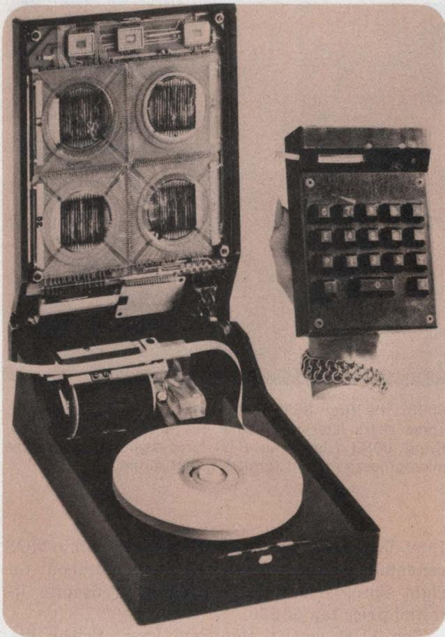
An IC array performs all computations in the first hand-held electronic calculator. From Texas Instruments, the battery-operated instrument prints answers without impact on a narrow strip of heat-sensitive paper tape.
