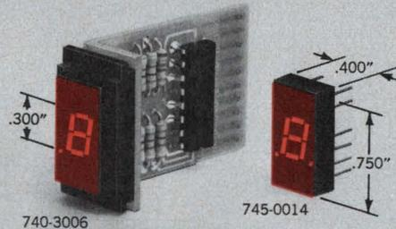
**745 SERIES** A new 0.300" LED character in a very bright red, seven-segmented readout . . . low power requirements. Standard 14-pin DIP . . . available with left and right decimal with  $\pm 1$ , and with and without on-board decoder/driver. Compatible with most TTL and DTL circuits. In 1000-lot quantities each **740-3006 . . . \$6.43. 745-0014 . . . \$2.10.**
