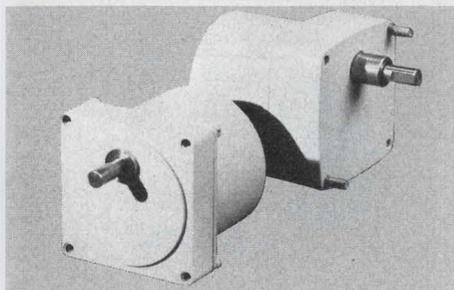
**Dual Speed Unidirectional Synchronous Motor** (Series 86000) offers advantages for instrument drives, especially strip chart recorders and telecopiers. Available torque to 35 oz-in. Choice of square or NEMA 2-11 gear box gives wide range of dual speed combinations. Fast start/stops eliminate need for clutching and prestarts. Available in 24, 120 or 240 VAC, 60 Hz, with CW or CCW rotation. Weight 30 oz. U/L listed. North American Philips Controls Corp. Cheshire, Conn. 06410 (203) 272-0301.
