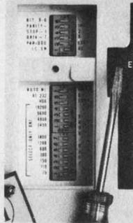
The 20 switches under the front name plate.
