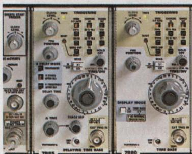
*Tektronix' new 7B80/7B85 Delta ( $\Delta$ ) Delay Time Bases are being used in the 7904 oscilloscope to measure pulse width in a minicomputer interface circuit.*
