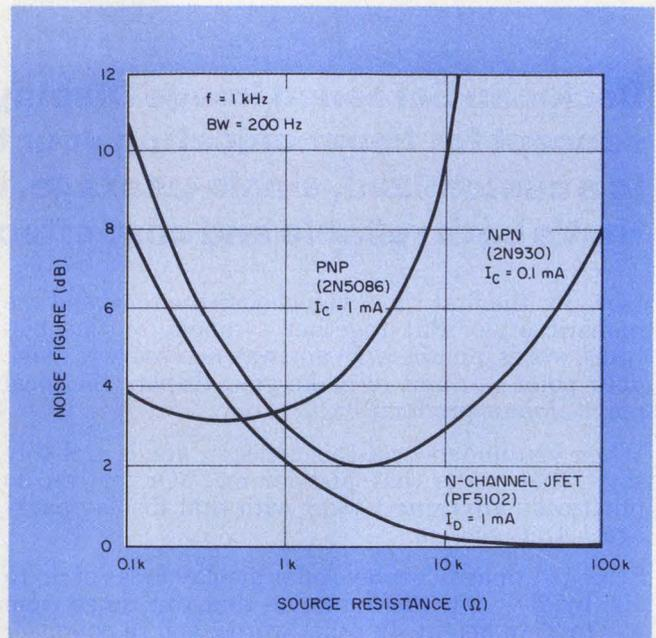
1. JFETs outperform bipolar transistors for low noise when source resistance exceeds 500 ohms.
