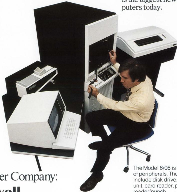
The Model 6/06 is offered with a variety of peripherals. The configurations shown include disk drive, CRT, tape cassette unit, card reader, printer, and paper tape reader/punch.
