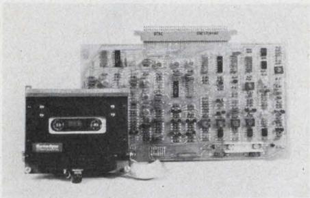
**Memodyne Model 763 High Speed Magnetic Tape Cassette Recorder.** For Computer or terminal peripheral storage. Records and playsback at 20 IPS. Searches at 120 IPS. Uses patented servo system for constant speed. Has only two moving parts. For literature contact Memodyne Corporation, 385 Elliot Street, Newton, MA 02164.
