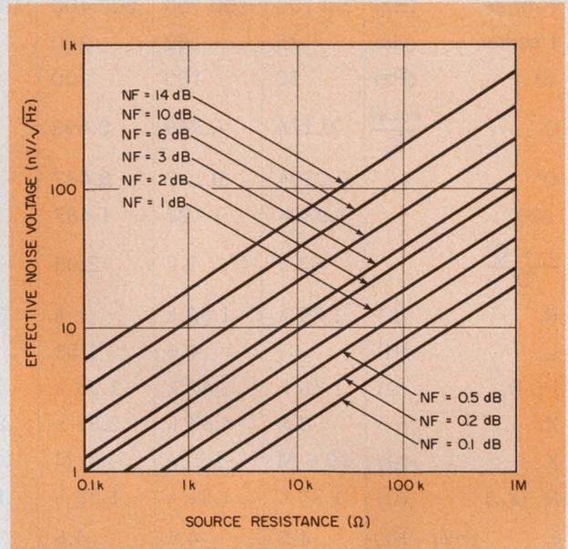
The effective noise voltage ( $e_{ne}$ ) can be quickly converted to noise figure (NF) once the source resistance is given.
