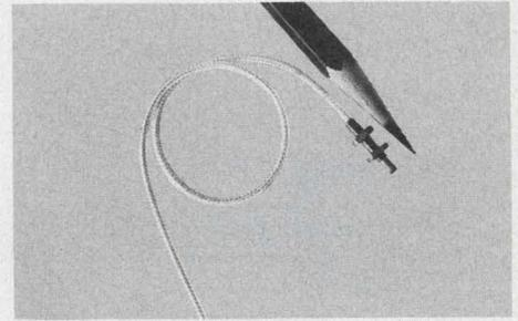
**World's Smallest Displacement Transducer.** Make precision, noncontacting displacement measurements at points never before possible. This new transducer, 0.080" OD, gives accuracy of  $<100 \mu\text{in.}$  in a range up to 0.020". Temperature stable. Repeatability and resolution is better than  $10 \mu\text{in.}$  Price \$485, including associated electronics. Kaman Sciences Corporation, P. O. Box 7463, Colorado Springs, CO 80933. (303) 599-1892.
