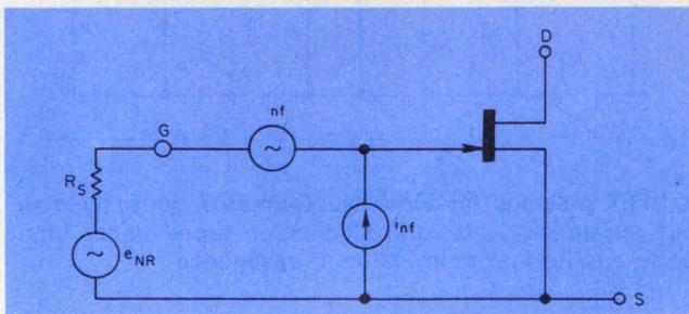
4. A simple JFET noise model may be constructed using thermal noise and shot noise sources.
