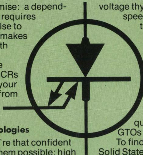
voltage thyristor technology combined with high speed transistor technology. You get everything a conventional 8.5-A SCR offers: normal inrush handling capability, pulse turn-on, operating range to 125°C. Gate turn-off capability is a bonus.
