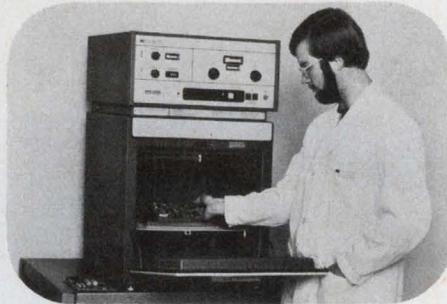
Use x-rays to pinpoint defects in small intricate devices, occlusions in castings, critical points in contacts, relays, or connectors.
