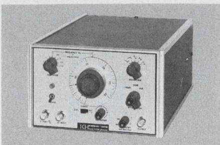
**MULTI-PURPOSE FUNCTION GENERATOR** Krohn-Hite's Model 5100A offers 8 types of waveforms; sine, square, triangle, pos. & neg. ramps, sawtooth, and pos. & neg. pulses from 0.002Hz to 3MHz. The symmetry control allows a 100:1 range for waveform variation. It has a 1000:1 (VCO) range and features a calibrated (dB) attenuator. Ideal for a broad scope of applications. Only \$495. Krohn-Hite Corp., Avon Industrial Park, Avon, MA 02322 (617) 580-1660
