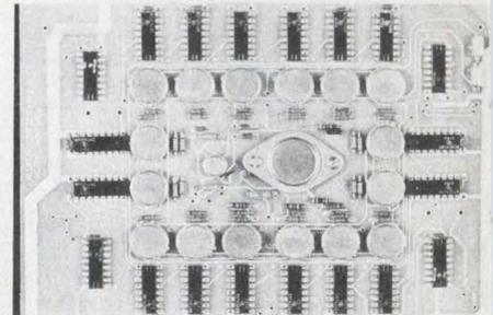
**The 5 bit A/D converter** constructed on single printed circuit card. Total thruput time 50 n sec, with 20 MHz update rate. Temperature stability over full mil range -55°C to +125°C with drift less than ±1 bit over entire range. For further information contact Ron Seibold, M.S. Kennedy Corp.; Pickard Dr, Syracuse, N.Y. 13211 (315) 455-7077.
