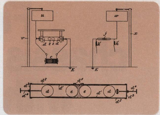
Marconi, in his U.S. Patent, issued July 13, 1897—his British patent was issued July 2, 1897—shows versions of a transmitter (left) and a receiver (right), and the blown-up section of the oscillator.
