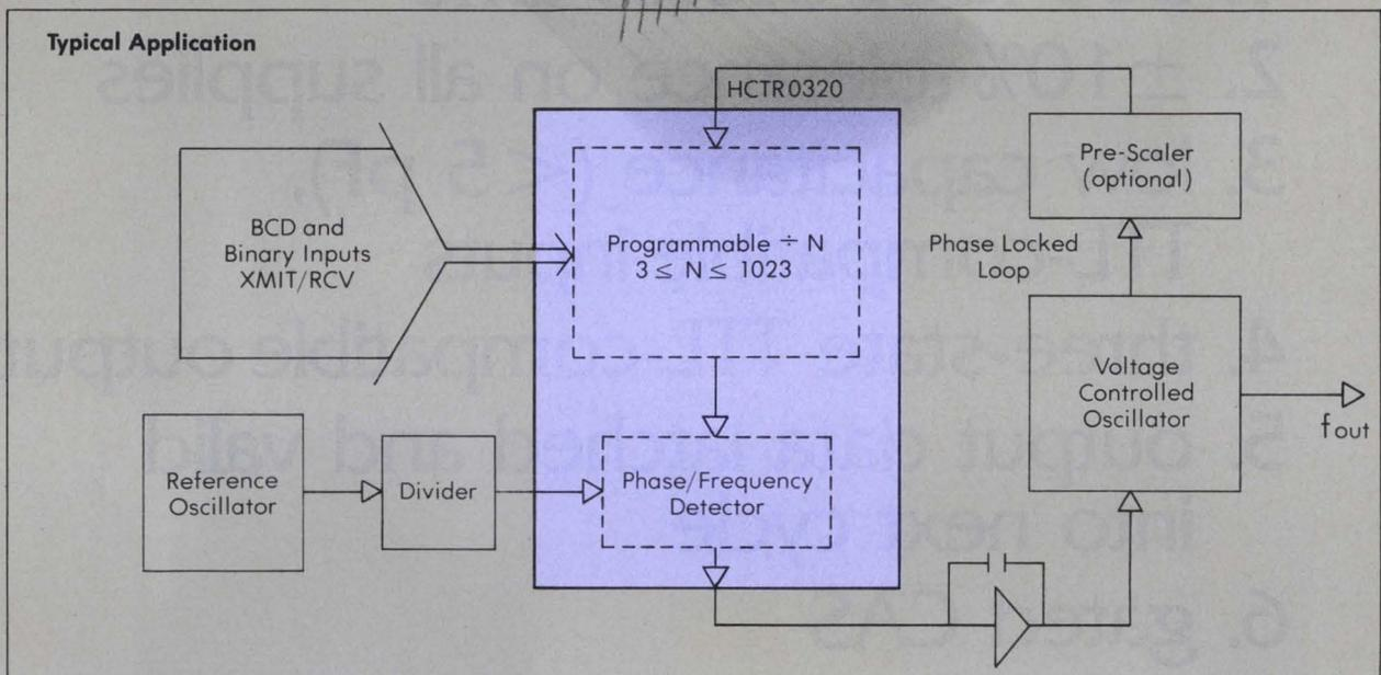
From the largest maker of watch chips comes a digital frequency synthesizer that provides up to 1,021 channels—all from *one* crystal.
