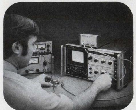
Use the HP 8447 preamp with a spectrum analyzer to make accurate measurements of low-level signals.
