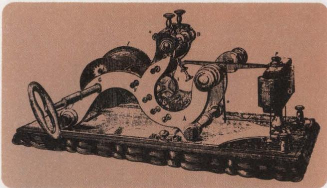
The original telegraph receiver wasn't the familiar keyed system but actually printed dots and dashes on paper with a stylus.
