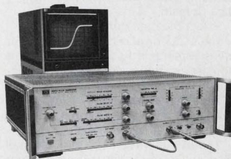
Sampling scope display of 8082A's 1 ns rise-time output pulse.
