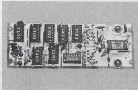
Low Cost Image Sensing Module contains a 1024 element (32-by-32) image sensor and all support circuitry on a single pc board. Digital video output may be displayed directly on an oscilloscope. Complete module (SE1024W) is \$150. Kit (SE1024K) is \$90. Cromemco, 1 First St, Los Altos CA 94022 (415) 941-2967.
