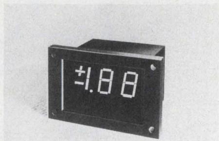
**DISPLAY ASSEMBLIES:** compact, expandable, easy to install. Utilizing 0.43" high character LED or 0.55" high character gas discharge display. The module contains all plug-in electronic components, including, indicators, decoder/drivers and current limit resistors. Accepts 4 lines BCD input. Available in 1½-, 2-, 2½- and 3 digit modules in two case-styles. CAN-YON ELECTRONICS, 2001 W. North Lane, Phoenix, AZ 85021 (602) 944-4421
