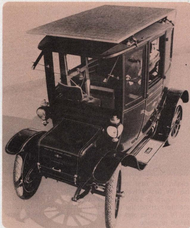
**Long before energy conservation became a burning issue,** International Rectifier in 1959 built a solar-cell energy source for autos and mounted the source on a 1912 Baker Electric. The solar cells put out about 200 watts.
