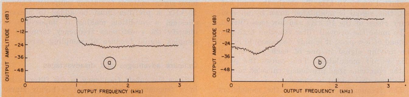
4. The output spectrum for broadband noise input with a 1-kHz low-pass setting (a) and a high-pass mode (b).
