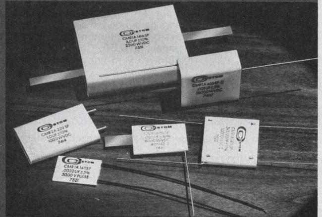
CMR "wrap and fill" mica capacitors offer maximum energy density within minimum volume. CMR types are wrapped in polyester tape, and have an epoxy compound end fill.
