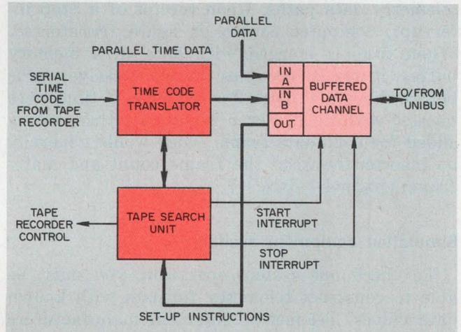
7. Time codes from separate tape channels permit addressable tape searches. The search unit controls the recorder and furnishes a start interrupt that informs the computer to begin processing the telemetry data.
