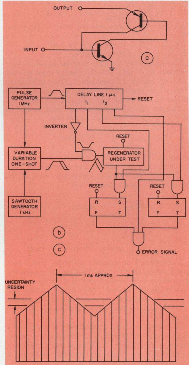
3. Typically, a regenerative circuit (a) follows a gate in a computing chain. When an arbitrarily small spike enters the regenerator, the circuit may delay in resolving the spike into a ONE or ZERO. The "uncertainty" can be measured (b) if an asynchronously modulated spike stream (c) is fed into the gate-regenerator and the error signals are monitored.
