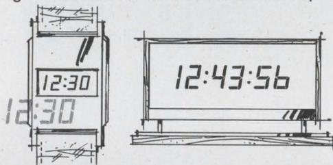
Producing an image — digital or other — simply requires a conductive surface the shape of the desired image on the glass plate toward the viewer. Current flowing from the conductive image on the front plate through the crystal liquid to the common-ground back plate causes the liquid to change from clear to a frosted appearance in the current-carrying area.
