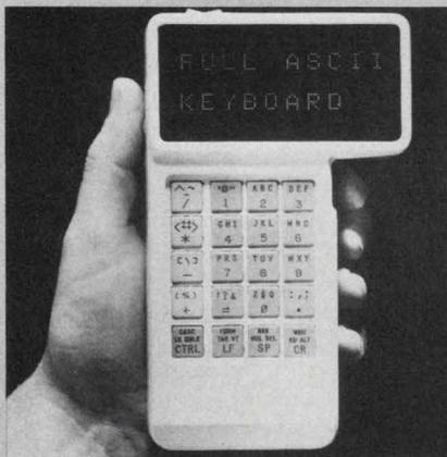
they appear as one or two-line displays. A display line consists of 10  $5 \times 7$  LED dot-matrix characters. When a line is filled, the display scrolls automatically. A 1000-character scrolling memory is built into the unit. And by operating one switch, the user can move forward or backward in this memory, to recover any part of a message that has been sent or received.
