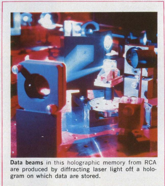
Data beams in this holographic memory from RCA are produced by diffracting laser light off a hologram on which data are stored.
