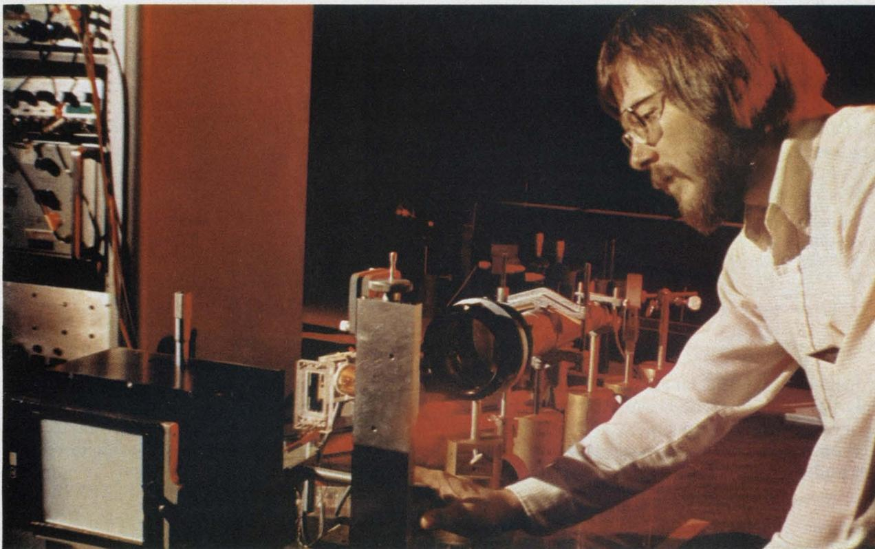
**Optical memories** like this one from Sperry Univac are being designed to store up to  $10^9$  bits of in-
