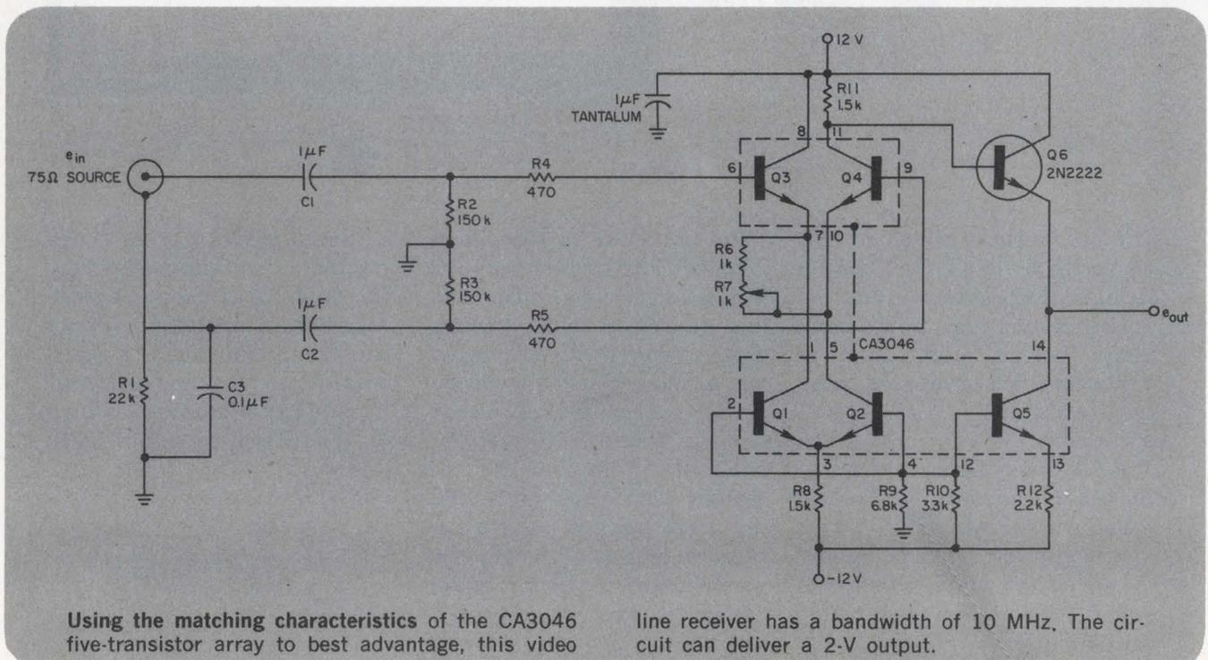
Using the matching characteristics of the CA3046 five-transistor array to best advantage, this video
