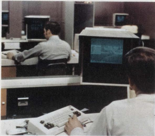
Four interactive graphics terminals, each linked to its own minicomputer, help design electronic circuits with Applicon's system. The host, also a mini, provides additional support for this star configuration and can act as a front-end to an IBM 360, which calculates the PC art-work routings.
