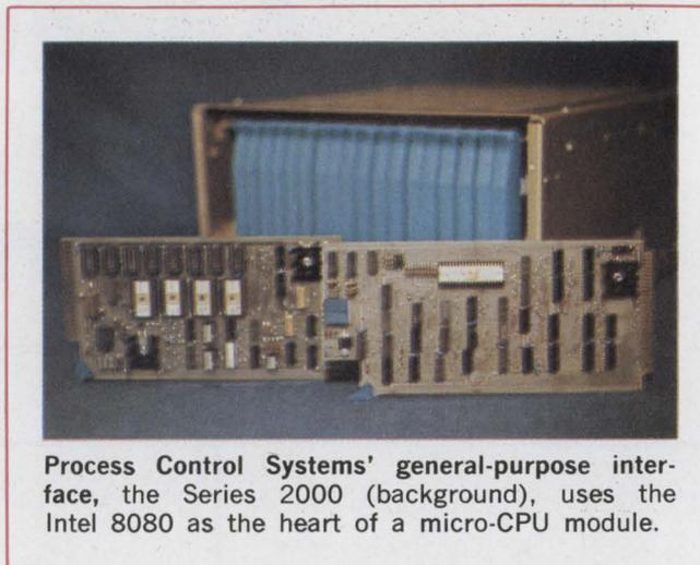
Process Control Systems' general-purpose interface, the Series 2000 (background), uses the Intel 8080 as the heart of a micro-CPU module.
