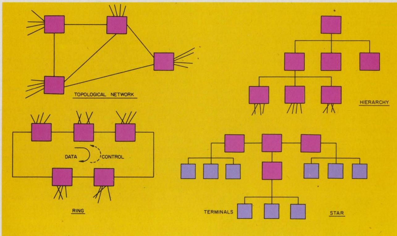
Configurations often seen in practical computer networks include the topological network, ring, hierarchy and star. The topological network handles distributed data communications, and the
