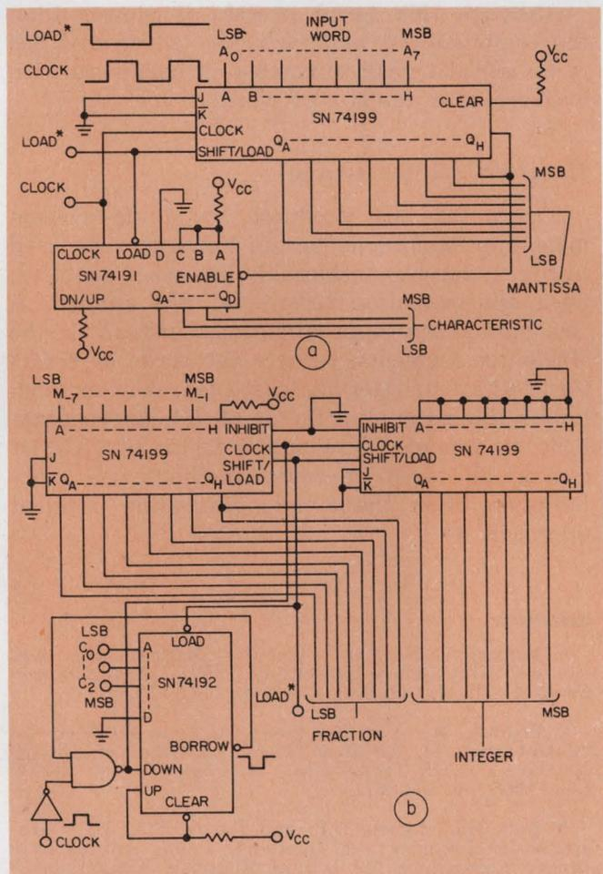
4. Sequential converters for log (a) and antilog (b) circuits require less hardware for handling larger numbers, but they need clocking circuits and they are much slower in operation than combinatorial circuits.
