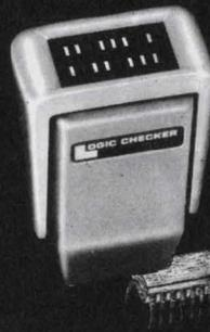
Displays logic state of most 14 or 16 pin IC's with no external controls. Simply clip over DIP package and appropriate LED will light to indicate a high logic state at each associated lead. For use on popular 5V systems. Completely portable for shop, lab, or field use—fully guaranteed. Detailed instructions and handy carry case supplied. Free set of 24 logic templates included. Post paid — \$99.95.
