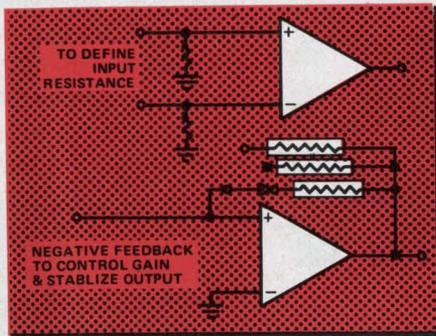
Victoreen MINI-MOX resistors are used widely to modify op-amp characteristics to: 1. Stabilize output and eliminate oscillation. 2. Define gain so measurements can be quantified. 3. Restrict bandwidth to the region of specific interest.
