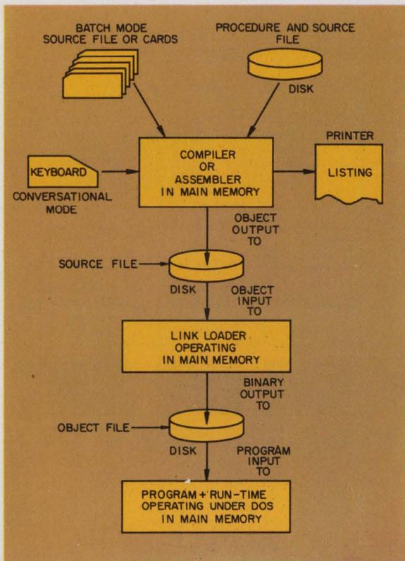
Inputs to this Lockheed System III language-processing subsystem are provided from source files containing symbolic code of programs in RPG II or in assembly language. The subsystem operating sequence for compilation or program execution begins with disc, card or keyboard inputs.
