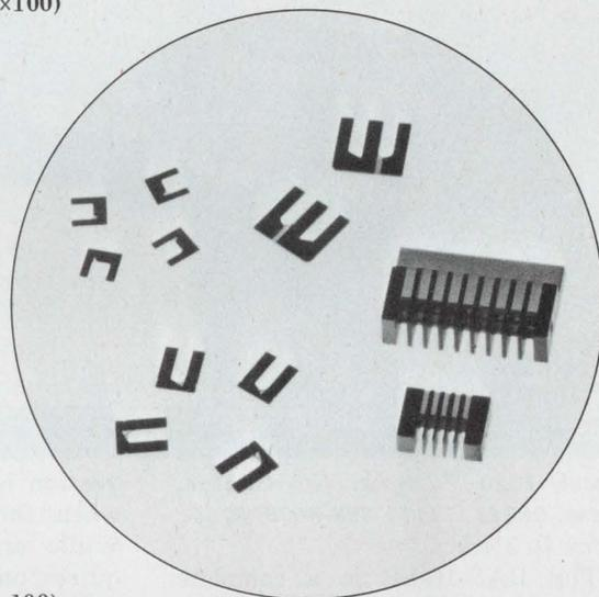
TDK is now producing manganese-zinc ferrite combinations with optimum performance characteristics for computer application. The crystalline powder of these ferrite materials is ground to uniform granular size, hot pressed and sintered into molded head pieces of high density. TDK's Mn-Zn hot pressed ferrite head pieces are free of voids, smooth in finish and have excellent contact wear resistance.
