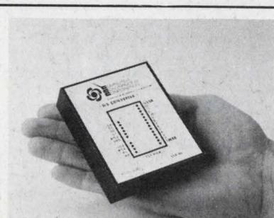
**Digital to synchro converters—14, 12 or 10 bit input, 11.8/90V, 400 or 60Hz transformer isolated output, accuracy  $\pm 4$ ,  $\pm 15$  or  $\pm 30$  min.** Driving 1VA, 2VA (2.6" x 3.1" x 82"H module) or 5 VA loads (4 1/2" x 9 1/4" pc card). Price from \$350 in qty. Computer Conversions Corp., East Northport, N.Y. 11731. (516) 261-3300.
