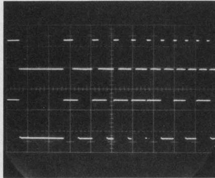
Upper trace: Constant Duty Cycle pulses over a 10:1 frequency range.
