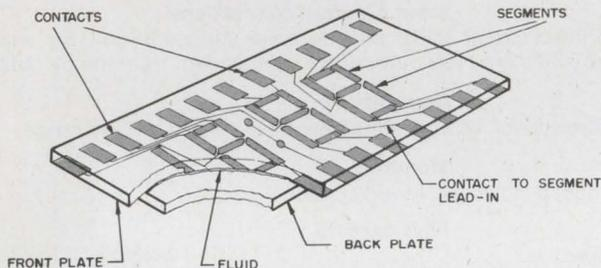
When the liquid is not electrically excited, its long, cigar-shaped molecules are parallel to one another in a position perpendicular to the plates. Thus, the liquid appears transparent. Applying an electric current creates ion activity which leads to turbulence and causes the liquid to scatter incident light. The visual effect is that of a frosted glass. LCD's can be made completely transmissive for back-lighting, reflective for ambient light or semi-reflective for dual mode operation.
