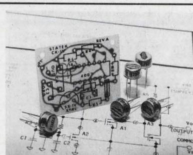
**Quartz Crystal Oscillator Kits for \$27.** Make bipolar series or CMOS parallel resonant oscillators. Kits include 5 or 6 SX-1 crystals (10 kHz to 240 kHz), in low profile TO-5 cans, a PC board (1.3" x 1.6") and design note. Statek Corp., 1233 Alvarez Ave., Orange, Calif. 92668. (714) 639-7810.
