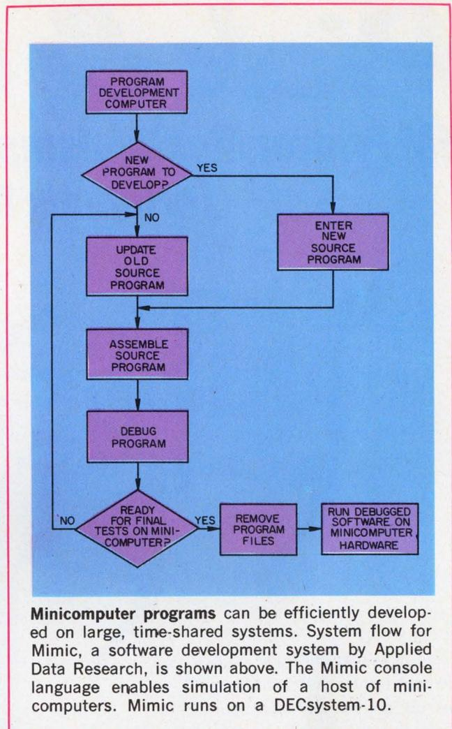
**Minicomputer programs** can be efficiently developed on large, time-shared systems. System flow for Mimic, a software development system by Applied Data Research, is shown above. The Mimic console language enables simulation of a host of minicomputers. Mimic runs on a DECsystem-10.
