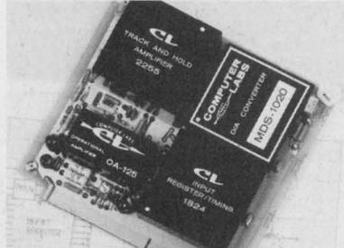
**The new Computer Labs DRA Series D/A's** eliminate harmonic distortion and produce clean "glitchless" pictures for reconstructed TV or other video signals. Input word rate for all models is 15 MHz with accuracies to  $\pm 0.05\%$ . Min. settling time to either 8-bit or 10-bit accuracies. Computer Labs, 1109 S. Chapman St., Greensboro, N.C. 27403.
