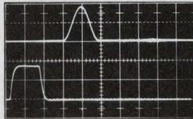
Sine<sup>2</sup> pulse (top waveform) and 100 ns pulse (bottom waveform).
