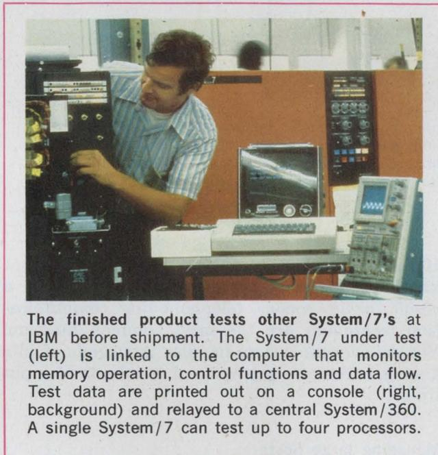
The finished product tests other System/7's at IBM before shipment. The System/7 under test (left) is linked to the computer that monitors memory operation, control functions and data flow. Test data are printed out on a console (right, background) and relayed to a central System/360. A single System/7 can test up to four processors.
