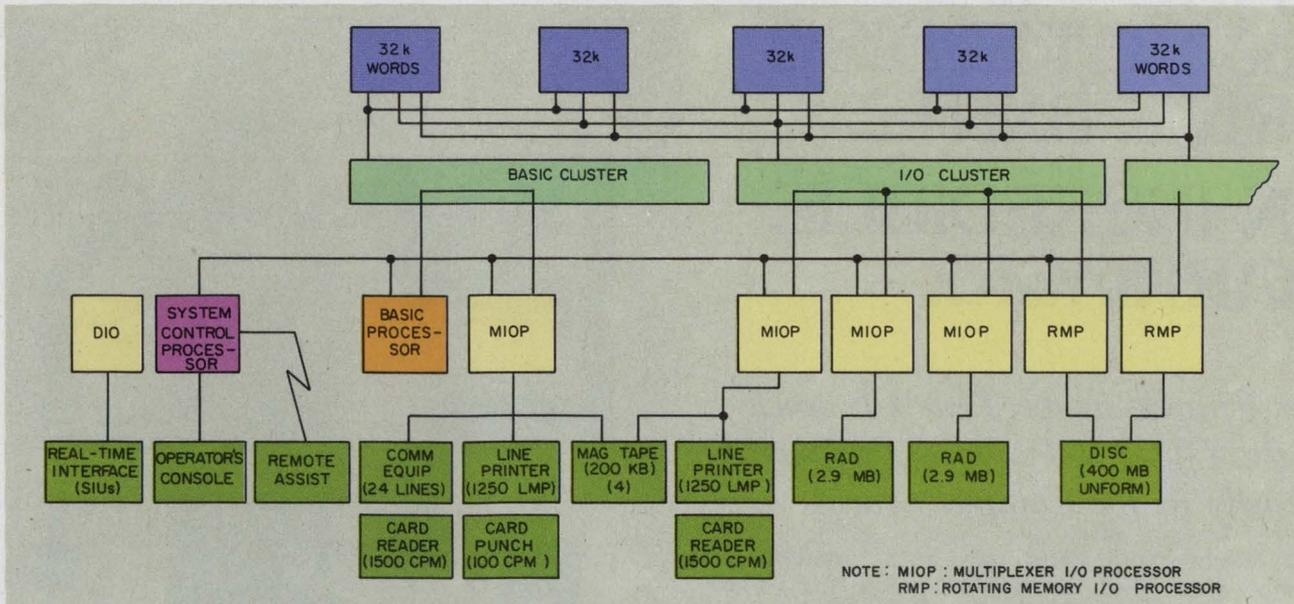
A very modern midi, the Xerox 560, makes use of an hierarchical architecture. Input-output and arithmetic processors have distinct functions but
