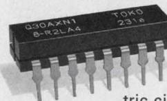
tronic circuits. There is also an increasing demand to combine active as well as activated elements into identical IC packages. In particular, the Dual In-Line Package (DIP) is gradually becoming the standard for IC packages. Used in electronic computers and other electronic machinery.
