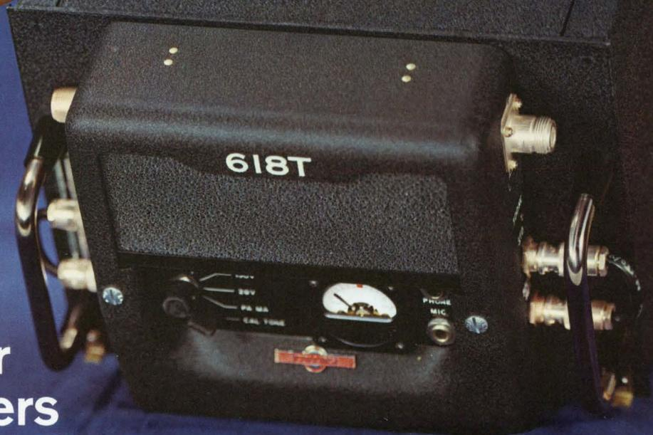
Single sideband radio demands precise frequency control. This is assured with Dale 1600 Series Trimmers. One application of these RT-12 wirewounds is in the RF oscillator circuit of the versatile Collins 618T/HF SSB Transceiver. Here, Dale wirewound trimmers provide: (1) The smooth resolution necessary for fast, accurate crystal adjustment during assembly; (2) Long-term stability which is a factor in the universal acceptance of Collins-built military and commercial radio equipment.
