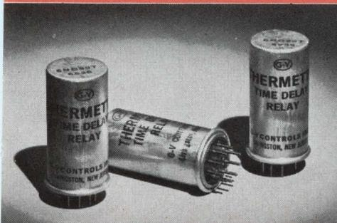
Metal enclosed thermal time delay is dust proof and shatter proof — designed for industrial applications requiring reliable operation and long life. **Features:** temp. compensated; time delays, 2 to 180 sec.; heater voltages, 6.3, 26, and 115V. AC or DC; contacts, SPST, NO or NC.
