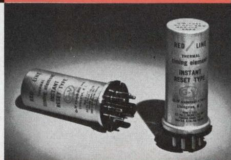
Instant reset during or after timing is available by combining G-V's unique instant reset timing element with a magnetic relay. Widely used in communication systems and data processing equipment. **Features:** delay time, 2 sec. to 5 min.; ambient operating temp., 32°F to 185°F.
