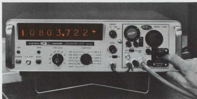
**2.** Adjust harmonic preset until the reading appears. Notice the counter reads "10,803.722 Mc," an actual microwave frequency presented with counter accuracy.
