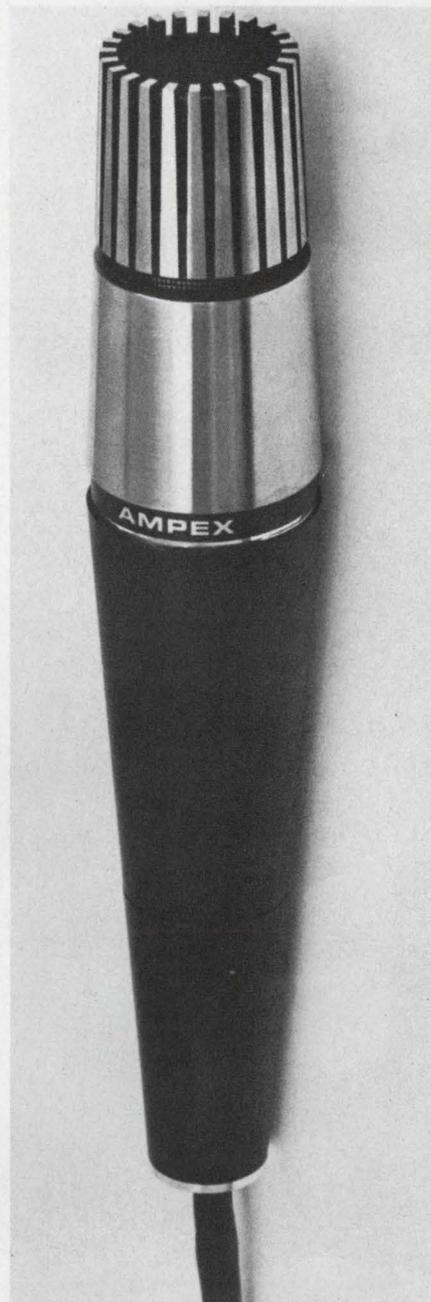
**Dynamic microphone** holds either of two coils in its barrel for high- or low-impedance inputs. Barrel unscrews for easy access to coils.
