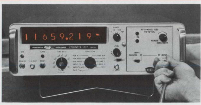
Quick as you couple the signal, a microwave reading appears. Notice the reading is "11,659.219 Mc," an actual microwave frequency—presented with counter accuracy because the input is phase locked. No calculations. No risk of human error. You simply plug in the ACTO for the range you're working in, then use the instrument just as though it were a simple frequency counter.
