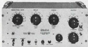
**Model B-7F** adds the following features to the basic specs of Model B-7B: (1) repetition rate is continuously variable from 2 Hz to 2 MHz; (2) output pulse rise or fall time may be independently degraded to approx. 1  $\mu$ sec; (3) either single or double pulse output available by front panel control.
