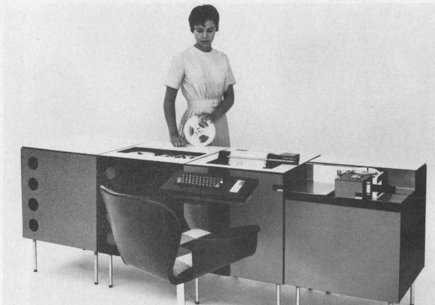
**Data station** transmits 8-bit ASCII at 120 characters/second. Design modularity allows system flexibility. Input/output capabilities include paper tape, punched cards, printer and keyboard-teleprinter units and an optical scanning input device.
