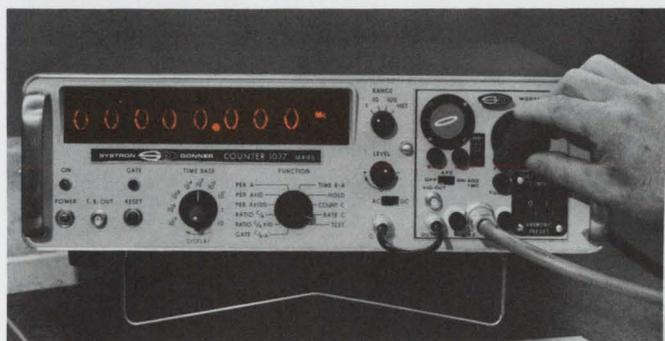
**1.** Tune transfer oscillator until a zero beat—any zero beat—appears on the built-in scope. The transfer oscillator is now phase-locked to the input.
