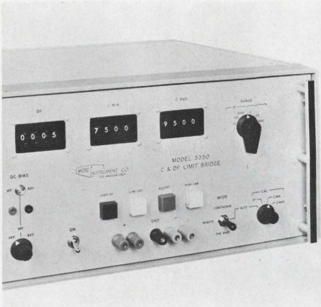
**Series capacitance** and dissipation factor measured. Strays have no effect. Page 250
