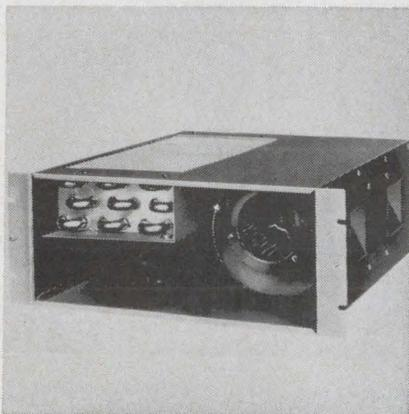
Designed to maintain 80°F max with a 1-kW heat dissipation, this heat exchanger employs chilled water from 66 to 70°F. Air is recirculated within the enclosure and cooled by the heat-exchanger in the blower case. More cooling may be obtained by using refrigerated water or direct refrigerant expansion. A higher ambient temperature may be maintained by the use of warm or hot water.
