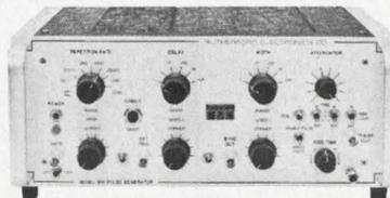
**Model B-16** all transistorized pulse generator offers a rep rate of 20 Hz - 20 MHz. Variable rise and fall times of less than 5 nsec to greater than 200 nsec. Pulse width is 0.015 - 10,000  $\mu$ sec. Amplitude is 0 to 10 volts, peak. Single or pulse pair operation. Rack mount available.
