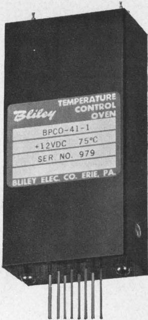
New type BPCO ovens maintain cavity temperature within  $\pm 0.1^\circ\text{C}$  with solid state noise-free circuitry. Ovens mount flat on PC board and provide eight wire lead connections for components.
