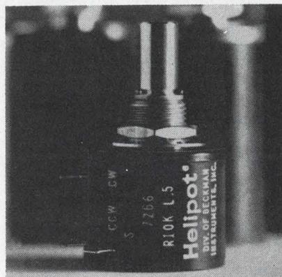
A wirewound, 10-turn pot has 7/8-in. diameter and is 3/4-in. long. Standard values are 10  $\Omega$  to 125 k $\Omega$ . Tolerance is  $\pm 3\%$  with  $\pm 0.2\%$  independent linearity.
