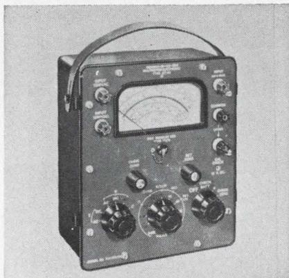
With more than 54 ranges, this solid-state multimeter covers dc and ac voltage and current, RF to 1.5 GHz and 2  $\Omega$  to 20 Megs center scale. Both Vac and dc have 11 ranges covering 12 mV to 1200 V full scale. Dc accuracy is  $\pm 2\%$  with 10 Meg/V input resistance. RF accuracy is  $\pm 0.5$  dB to 500 MHz. The meter is powered by 3D cell batteries.
