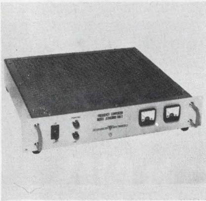
Series ATA frequency converters are stable sources of 400 Hz power operating from 50 to 70 Hz lines. Frequency stability, waveform purity and low dynamic impedance are reported. Output power is 100 to 1000 VA. Voltage regulation, from no load to full load, is 0.5%. Line regulation is  $\pm 0.5\%$  from 105 to 125 V.
