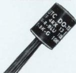
Electrostatically & magnetically shielded output transformer 1/4 D. x 1/4" H. Pri. 15K CT, Sec. 8K CT; max. level 50 mw; audio range response. To MIL-T-27B, grade 4.
