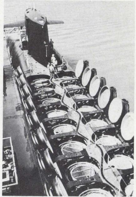
**Nuclear submarines** that now carry the Polaris A-3 missile will accommodate the Poseidon after modification of their missile tubes.
