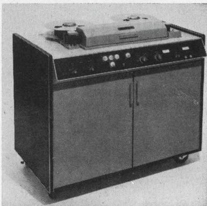
A mobile broadcast videotape recorder, the VR-1100E, is 39 in. high and weighs 550 lbs.
