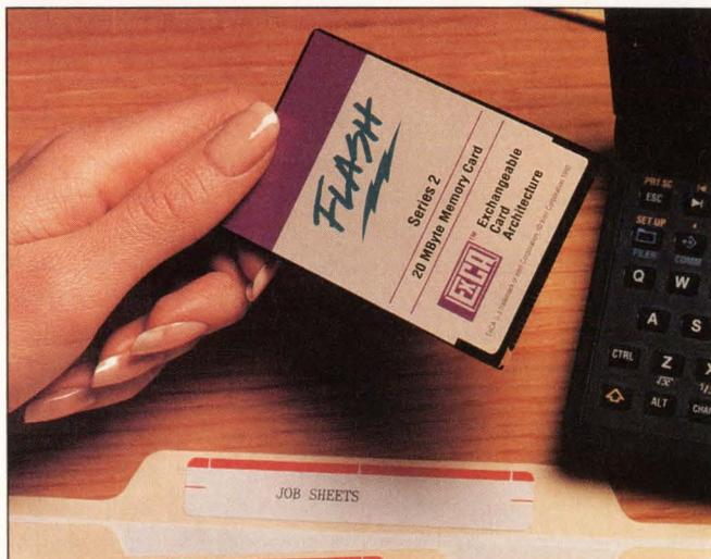
**As much as 20 Mbytes or more of flash memory will fit in a 3.3-mm-thick PCMCIA Type I card. Intel is the price leader in flash cards, selling its 20-Mbyte version for around \$600.**
