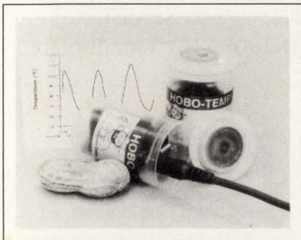
**Miniature data logger for MS-DOS PCs and Macintoshes.** The Hobo-Temp is a tiny pc board housed in a 2.1-in.-long  $\times$  1.3-in.-diameter plastic cylinder. The unit connects to an MS-DOS PC's or Apple Macintosh's serial port. You can obtain the loggers with integral or external sensors and with ranges of -39 to +123, -5 to +37, or -37 to +46 $^{\circ}$ C. The loggers receive
