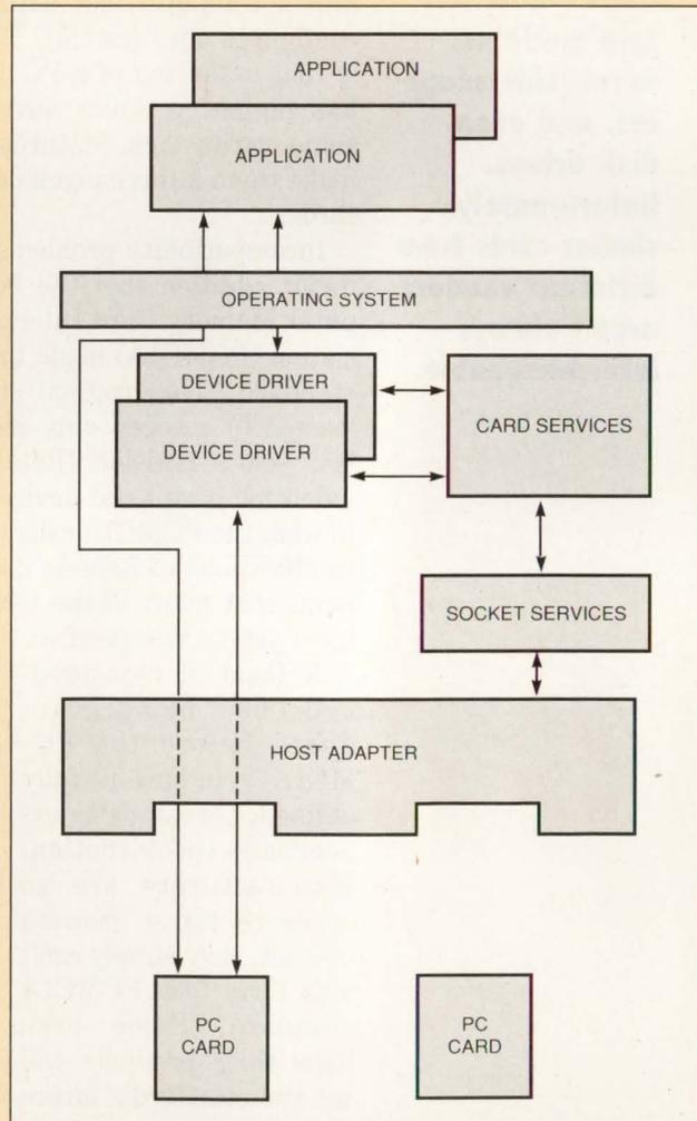
**Fig A**—Two software modules, Socket Services and Card Services, provide a standard software interface to PC cards. A host-adaptor IC connects a computer bus to one or more card sockets.
