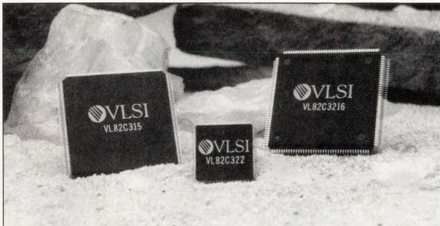
Your production line must be able to handle large, fine-pitch surface-mount devices, such as these from VLSI Technology, if you're going to design your own embedded PC.
