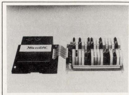
**Industrial controllers.** The MicroDAC handles up to 32 single-point I/O modules in any analog-digital combination. The unit can exchange ASCII messages at speeds ranging to 115.2 baud. The unit features 64 kbytes of flash EPROM and 64 kbytes of battery-backed RAM
