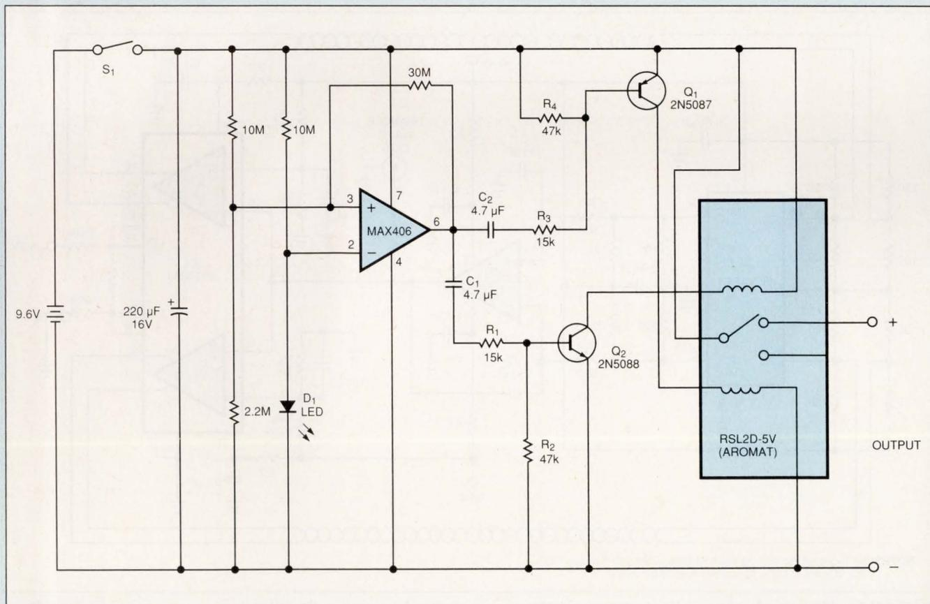
Fig 1—This circuit cuts off a low battery while and consumes only 3  $\mu\text{A}$ .
