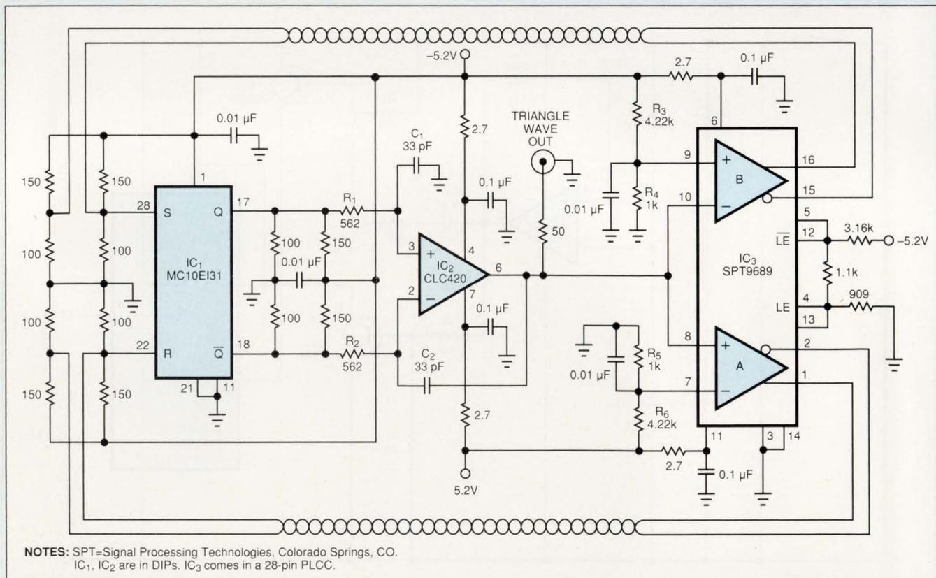
Fig 1—Using IC<sub>1</sub> to produce pure square waves and IC<sub>2</sub> as a nearly ideal integrator, this triangle-wave generator produces linear 10-MHz, 1V p-p triangle waves that exhibit low second harmonics of -51 dBc.
