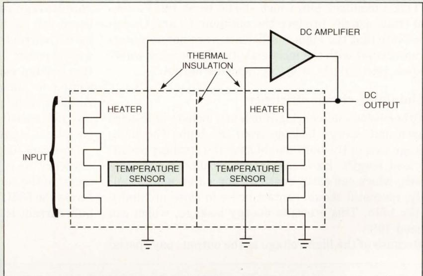
**Fig B**—The conceptual thermal rms/dc converter will reject ambient temperature shifts only if the heater sensor pairs are isothermal.
