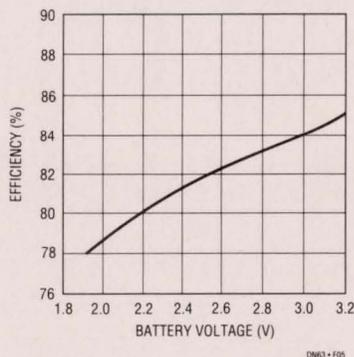
Figure 5. Step-Up Conversion Efficiency - 5V Output, 30mA Load
