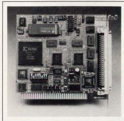
**Low-power, 50k-sample/sec, 13-bit ISA bus data-acquisition board.** The 410 is a half-size card that uses only two supply voltages, 5 and 12V, at 500 mW (operating) and 50 mW (standby)—attributes that suit it to data acquisition in several laptop PCs. The card provides 16 single-ended or eight differential analog inputs, a 3-channel counter/timer, and 16 digital I/O lines. The ADC, which has a  $\pm$ 5V range is pre-
