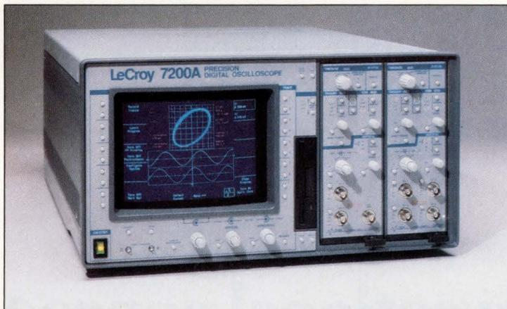
**From the front, the only difference you may note between LeCroy's 7200A DSO mainframe and its predecessor, the 7200, is the new unit's high-resolution color display. Internally, however, there are major differences. Although the same state-of-the-art acquisition modules plug into both mainframes, the new unit uses a PC motherboard and other standard PC components.**
