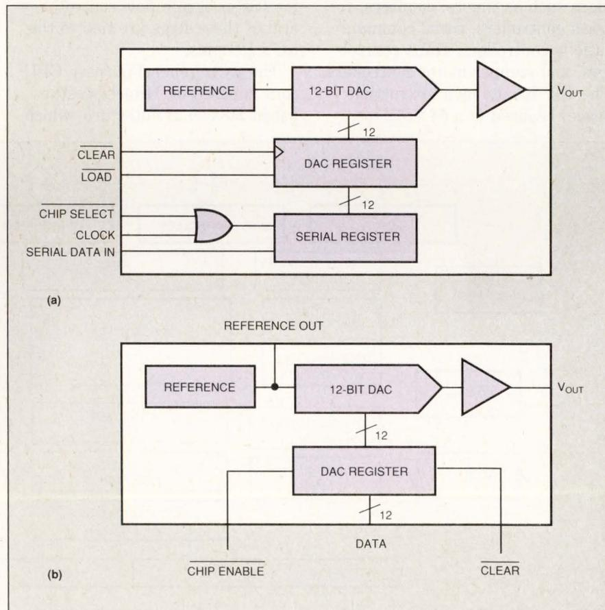
You need only a 5V supply to operate the serial 12-bit DAC-8512 (a) and parallel DAC-8562 (b). Both devices include an internal reference and output amplifier, which provides an output swing of 0 to 4.095V. The 8512 comes in an 8-pin SOIC or DIP.
