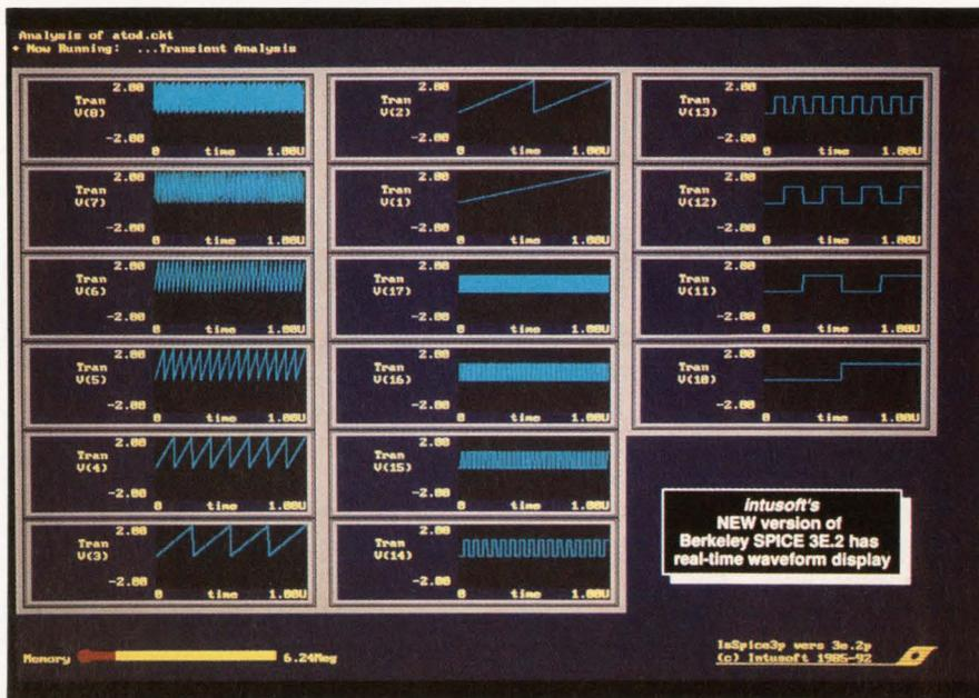
The IsSpice3 simulator from Intusoft is based on Berkeley Spice 3E.2. The simulator includes all the abilities of Spice 2G.6 and enhances its analysis and modeling features. The simulator provides backward compatibility to all vendor-supplied op-amp model libraries.
