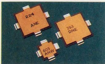
MICRO/Q® 3000 capacitors reduce noise associated with PGA and PLCC devices. Designed to be mounted under the device, take no extra board space. Can be used under MPUs, Gate Arrays, and ASICs. Choose from Z5V, X7R, and P3J dielectrics. Available in both thru-hole and surface mount versions. Several sizes available to fit all devices.
