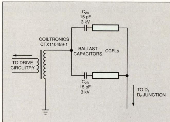
**Fig 2**—The drive circuit must deliver more power when the backlighting scheme involves two CCFLs. The transformer in this circuit can develop an 11-mA output—the transformer in Fig 1a delivers only 7.5 mA.
