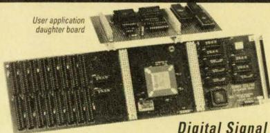
Digital Signal Processor development environment using TI's TMS320C30 40 MHz floating point DSP and the TI Compiler, Assembler, Linker and Debug software.
