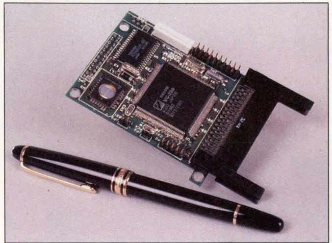
**All-in-one PC chip sets let embedded-control designers incorporate PC compatibility even with the most demanding space constraints. This example uses Vadem's chip set to provide a PC/XT with one PCMCIA card slot.**
