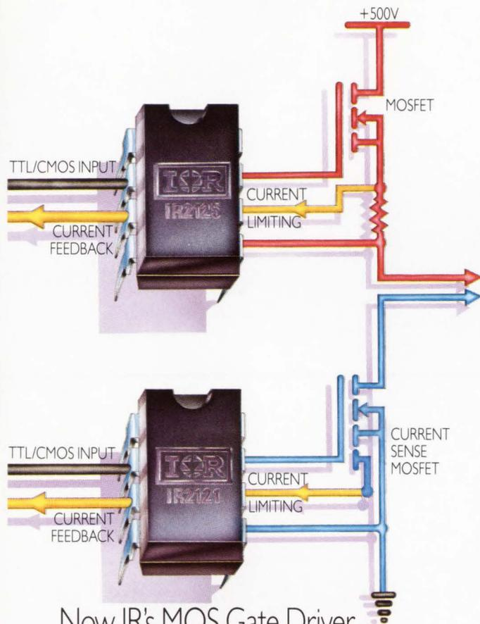
Now IR's MOS Gate Driver family includes high-voltage devices designated for applications where protection is paramount: Introducing the IR2125 and IR2121, designed to drive and protect motor controls and other circuits up to 30 kHz.
