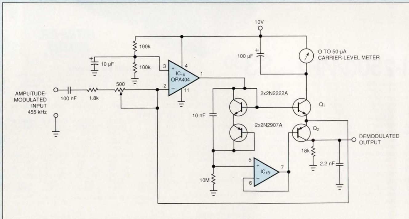
Fig 1—This circuit indicates the carrier level of a 455-kHz AM signal and produces a demodulated output.
