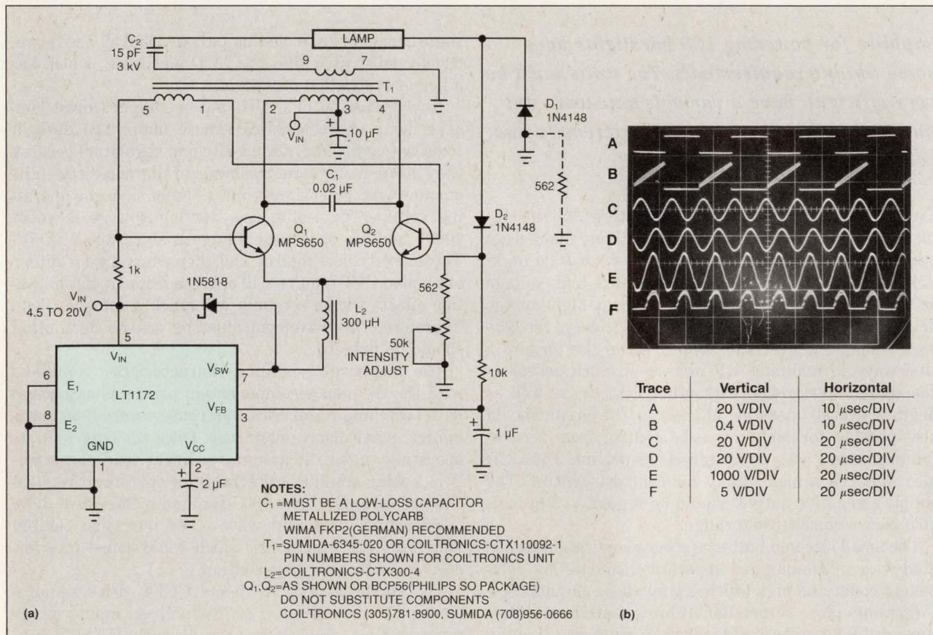
Fig 1—Efficiency for this CCFL drive circuit (a) equals 78% for a 4.5 to 20V input-voltage range. The circuit's operating waveforms are shown in (b). When power is applied, voltage at the LT1172 switching regulator's feedback pin is less than the 1.23V internal reference, which generates full duty-cycle modulation at the V<sub>SW</sub> pin (Trace A).
