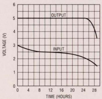
Figure 8. 3V to 5V Step-Up Switcher - LT1173-5, 30mA Load
