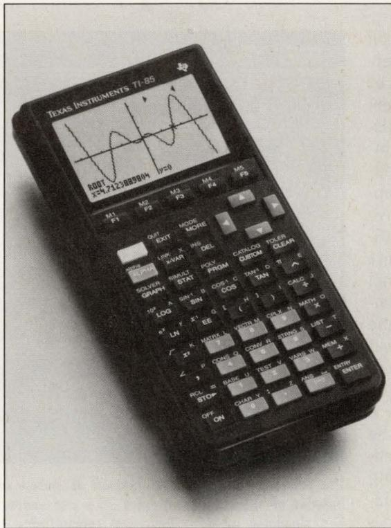
The TI-85's graphics display, cursor keys, and built-in functions allow you to perform numerous analyses on a graph as you view it.
