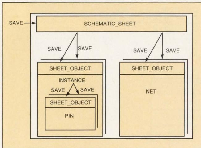
Mentor Graphics Corp developed its 8.x series EDA design tools using C++ and object-oriented approaches. The tools save sheets from hardware designs using the OOP principle of inheritance.
