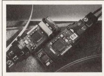
**Optical-link card.** The HOLC-0266 optical-link card transmits at 266 Mbps and complies with the ANSI Fiber Channel standard. The card connects the mother board or I/O-channel card of a desktop computer or workstation to a fiber-optic cable. The unit fully implements the FC-0 physical layer, incorporating the transmit and receive functions for both the electrical and optical interfaces. The card in-
