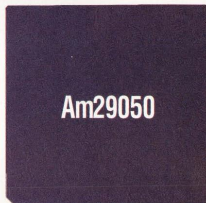
32-bit RISC processor with on-chip floating point.
