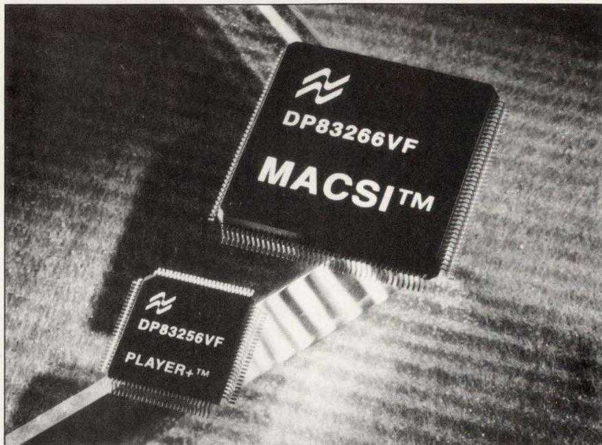
The DP83200VF chip set squeezes FDDI into just two chips, simplifying adapter-board design.
