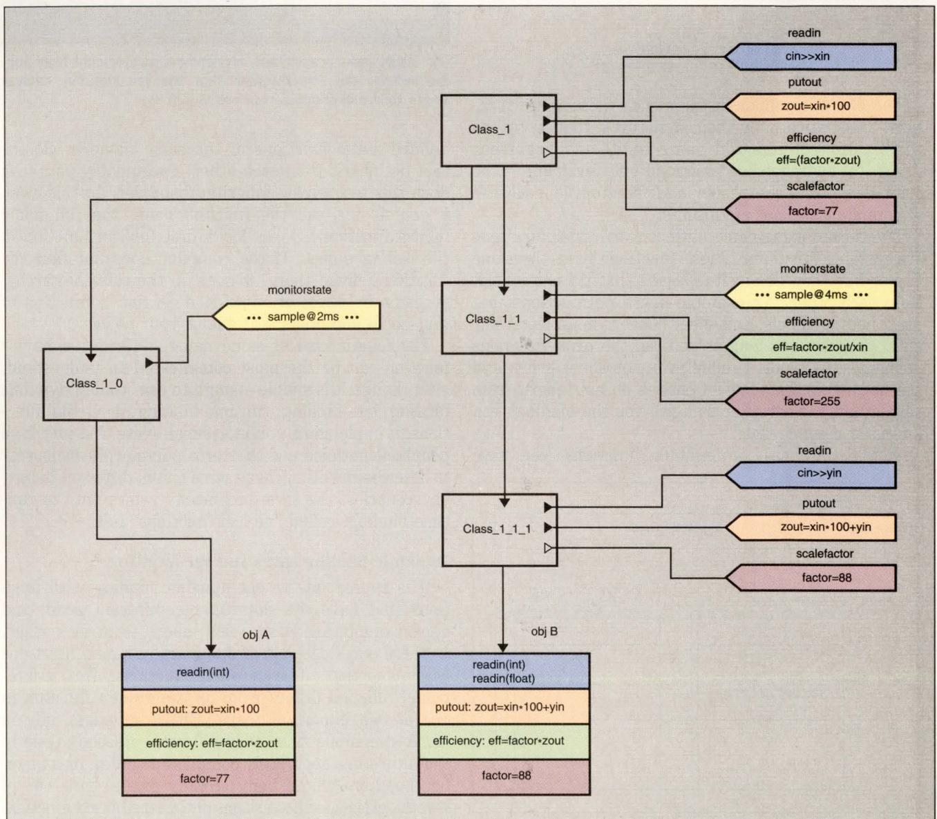
Fig 1—A hierarchy of classes, their associated member functions, and two objects illustrate four types of same name, different behavior relationships: overloaded, overridden, disjoint, and dynamically bound functions.
