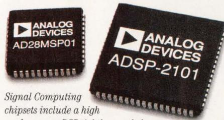
*Signal Computing chipsets include a high performance DSP tightly coupled with a mixed signal front end for optimum performance and flexibility with minimum design time.*
