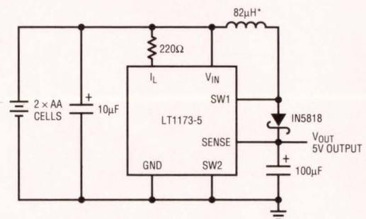
Figure 3. 3V to 5V Step-Up Converter
