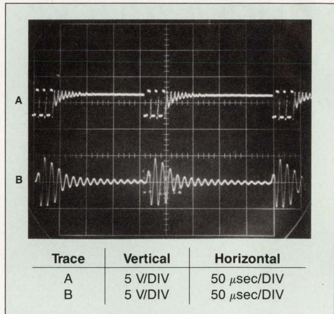
**Fig 4**—When the regulator comes on (Trace A), it delivers bursts of output current to the L<sub>1</sub>,Q<sub>1</sub>-Q<sub>2</sub> high-voltage converter. The converter responds with bursts of ringing at its resonant frequency.
