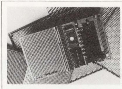
**Development board.** The DPSS-1 complies with the Sun Microsystems and SBus specification for slave devices. **Circle No. 453**
