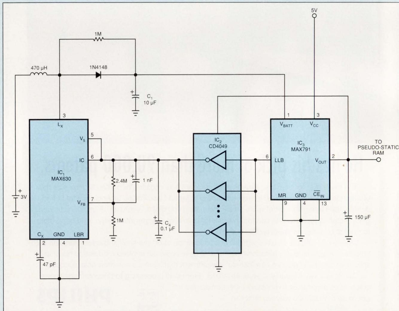
Fig 1—A power supervisor, IC<sub>3</sub>, uses a ganged inverter, IC<sub>2</sub>, as a miniature solid-state relay to power a step-up regulator, IC<sub>1</sub>, only when the main 5V supply fails. The backup supply can supply 4V from a single 3V lithium cell to keep pseudostatic RAMs alive.
