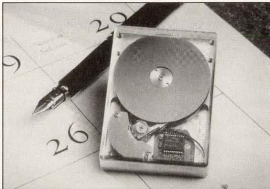
**Hewlett-Packard's 20-Mbyte, 1.3-in. Kitty Hawk disk drive (\$250 in OEM quantities) will soon be appearing in PCMCIA-compliant PC cards. PCMCIA Type III cards, which are 10.5 mm thick, can hold either a 1.3-in. or a 1.8-in. drive.**
