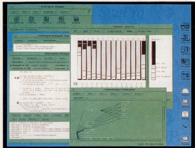
The SPARCworks professional development environment from Sun-Pro includes the Sourcebrowser that lets you statically analyze source code and program structure in C++.
