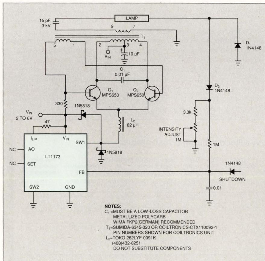
**Fig 3**—Optimized for low-current operation, this drive maintains control down to tube currents of 1 mA—a very dim light. This design suits applications that need to maximize battery life. Primary supply drain ranges from hundreds of microamperes to 100 mA with tube currents of microamperes to 1 mA.
