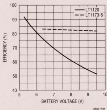
Figure 4. Step-Down Conversion Efficiency - 5V Output, 30mA Load
