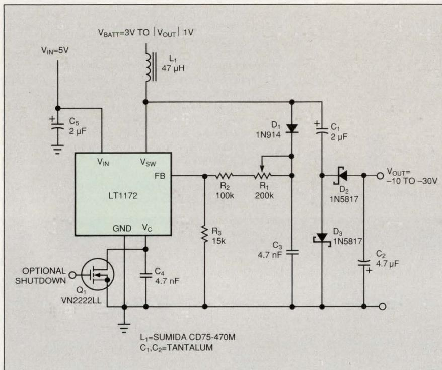
**Fig 6**—To generate negative bias for LCD drivers, this circuit combines switching regulator and charge pump techniques. The variable  $-10$  to  $-30V$  output can provide contrast control for the display.
