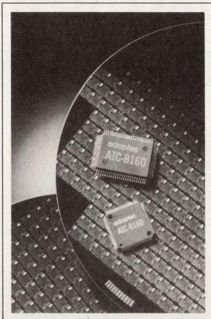
**IDE hard-disk controller.** The AIC-8160 hard-disk controller automates ISA bus I/O tasks that usually require a local  $\mu\text{C}$ . The chip provides 11 bits of error detection and correction and can continuously read while correcting.
