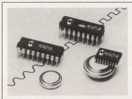
RC oscillator. After conversion, an interrupt awakens the core to store the converted data. The core operates at 20 MHz and incorporates a  $1024 \times 14$ -bit program EPROM. \$3.25 (10,000). **Microchip Technology Inc**, 2355 W Chandler Blvd, Chandler, AZ 85224. Phone (602) 963-7373. **Circle No. 412**
