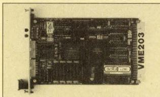
Micro-Link's VME203 SBC makes your design choice easy. Available in several configurations. VME203 prices start at less than \$1,025 in 100 piece quantities. Options include 68EC030 or 68030, FPU, 1 or 4 MB of DRAM with transparent refresh, burst mode Cache, up to 1 MB of EPROM, two RS-232 serial ports, and clock speeds of 16, 32 and 40 MHz. VME203 software support includes Microware OS-9®, CrossCode® C FreeForm™ and Microbug II.
