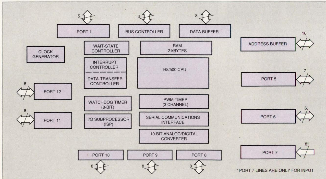
A microprogrammable I/O subprocessor with an 83 1/3-nsec instruction cycle on the H8/570 dual-processor μC allows you to create high-speed, custom I/O controllers. The chip also provides a number of standard peripherals.
