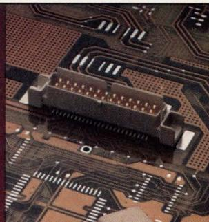
*An example of a typical Meritec solution is this 50 ohm, impedance matched, board-to-board Hermaphroditic Connector on .050" centers. The connector helped reduce costs and increase capability by freeing up board space for additional components.*
