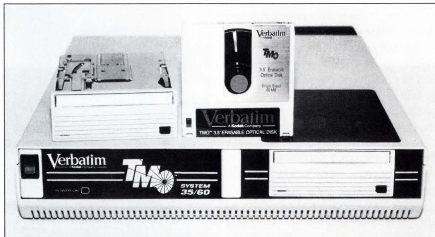
Providing a 30-msec seek time, the TMO System 35/60 by Verbatim challenges Winchester performance. It stores 60M bytes on a 3½-in. cartridge.
