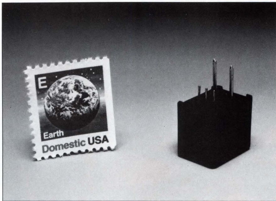
Fig 6—The CS line of miniature digital current sensors from Micro Switch includes models that sense current from 2.6 to 15A. These devices perform in-line current sensing at temperatures from -25 to +85°C.
