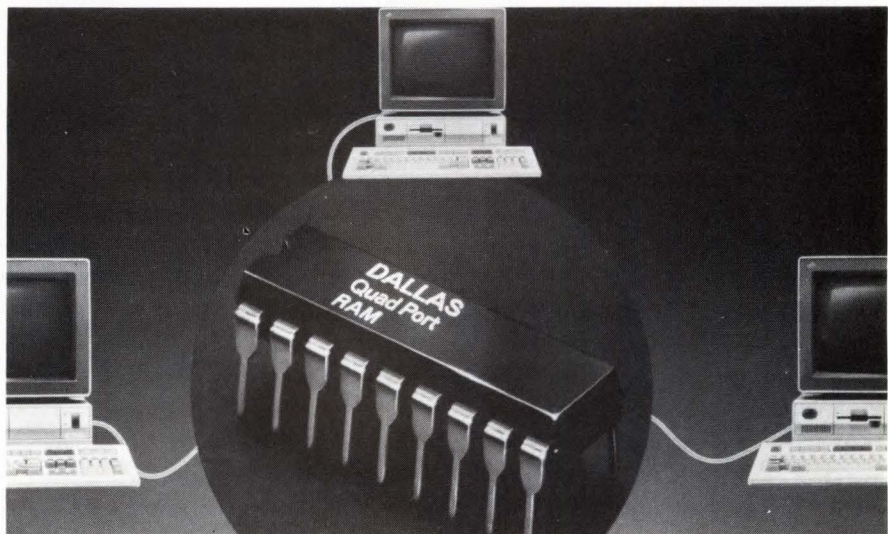
Providing 4-way access to a common memory, the DS2015 quad-port serial RAM lets you loosely connect as many as four independent computers.
