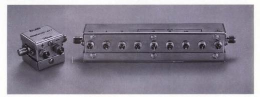
Operating over dc to 1 GHz, the MDA Series attenuators from Alan Industries feature total attenuation specs ranging from 15 to 127 dB, a switching time of 6 msec, and a switch life of  $10^7$  operations per bit.
