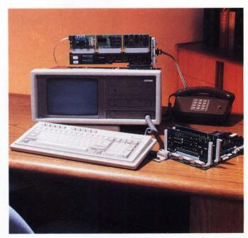
Hardware- and software-development tools, like this PC-based ISDN evaluation system from Siemens, help you with code generation, chip emulation, and test-measurement requirements.
