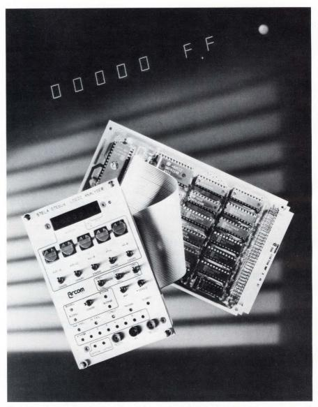
You can recreate the lights-and-switches look and feel of early minicomputers with bus-analysis tools that include front panels. One such tool is Arcom Control Systems Ltd's STELA for the STE Bus.
