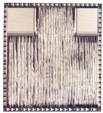
Suited to real-time embedded controller applications, the 16-bit RTX2000 core  $\mu P$  available in Harris Corp's standard cell library directly executes the Forth programming language, eliminating the need for assembly language programming.
