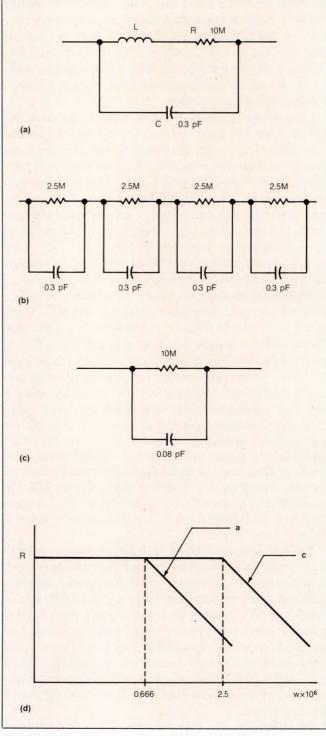
Fig 2—You can reduce the capacitance of a single resistor (a) by using several resistors in series as shown in  $\mathbf{b}$  (assume the inductance is negligible). This series resistor configuration has one fourth of the single resistor's capacitance (c) and extends the resistor's frequency response as shown in  $\mathbf{d}$ .
