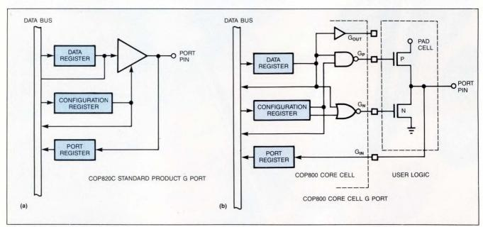
Fig 1—The I/O logic on the G-port of Sierra Semiconductor's COP800 μP core (b) gives you greater flexibility than that on the COP820C standard part (a). Connected to the pad cell as shown, it mimics the standard part, but it can also provide separate input and output lines, and push-pull drive to other on-chip logic.
