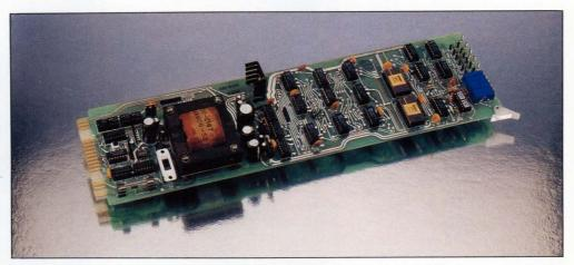
Cards like this one—Kepco's SN 488-B—are building blocks for programmable power systems. The cards plug into rack-mounted 8-slot and half-rack 4-slot chassis that interface with the IEEE-488 bus. Each card controls one supply.
