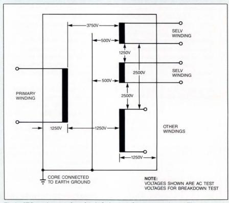
Fig A—IEC requirements for safety isolating transformers are stringent. The specs require  $> 3750 \mathrm{V}$  ac breakdown between the primary and the SELV secondaries and  $> 1250 \mathrm{V}$  ac breakdown between all windings and the transformer's case.
