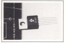
output-current rating of 3A max. Other specs include a typical input noise of 2  $\mu$ V from 10 Hz to 10 kHz and common-mode rejection of 70 dB. The CS-365 includes on-chip thermal-shutdown and safe-operating-area protection. In addition to its use in motor-control and power-supply applications, the CS-365 can deliver 18W into a 4 $\Omega$  load when used as an audio amplifier. The op amp comes in a 5-lead TO-220 package. \$1.44 (1000).
