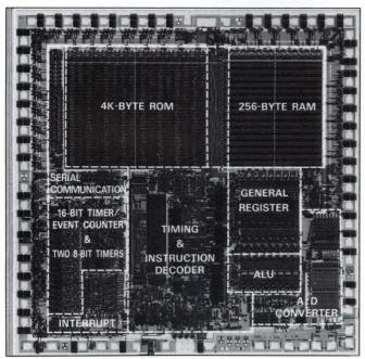
You can combine the  $\mu$ PD78AD core  $\mu$ P from NEC Electronics Inc with ASIC library megacells that are functionally compatible with the company's 72xxx and 71xxx Series peripherals.
