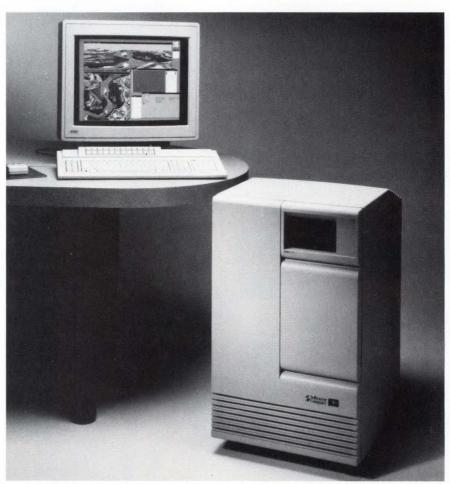
You can plug as many as four CPU boards into Solbourne Computer's SPARC-based Series4 computers; these computers can execute all programs written for Sun Microsystems' Sun 4 workstation family.
