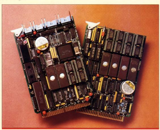
The ZT 88CT08 Single Board Computer and ZT 88CT25 Expanded Memory System are two new Ziatech STD Bus boards offering low power consumption and an extended temperature operating range of -40 $^{\circ}$  to + 85 $^{\circ}$  C.
