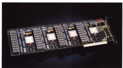
Because every Transputer-based-board vendor uses Inmos's interface chips, all Transputer-based add-in boards are very much alike. The DSI-T4 from Definicon Systems, for instance, includes 4M bytes of dynamic RAM per processor, as well as four bidirectional DMA links.
