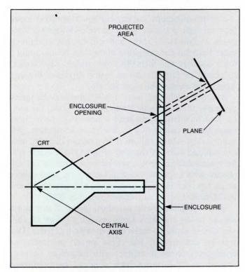
Fig 4—To prevent flying parts from reaching a CRT, the projected area of enclosure openings must not exceed 0.2 sq in. The purpose of this requirement is to prevent implosion of the CRT.
