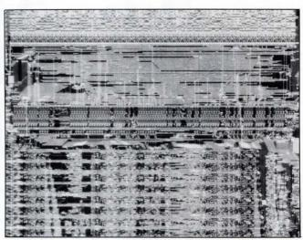
While retaining software compatibility with the NMOS 6502  $\mu P$ , this 65CX02 core  $\mu P$  from NCR Corp adds an additional 59 op codes, 14 new instructions, and two new addressing modes to the 6502 instruction set.
