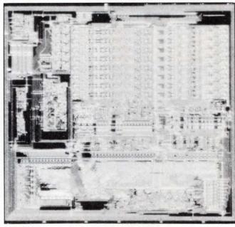
This 68C05 core  $\mu$ F from the ASIC library of NCR Corp illustrates the high silicon utilization attainable with a hard core. It executes the instruction set of Motorola's MC68HC05C4 microcomputer.
