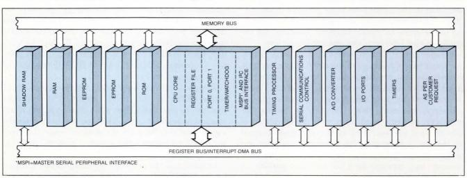
Fig 2—Designing a core- $\mu$ P system is like collapsing a pc-board-level system onto a single chip. This diagram from SGS-Thomson represents both the architectural and physical layout of a single core- $\mu$ P system.
