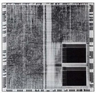
The L64801 32-bit RISC processor core from LSI Logic provides an implementation of Sun Microsystem's SPARC architecture. This year it will be introduced into the company's 0.7-µm channel-length LCB007 standard cell library.
