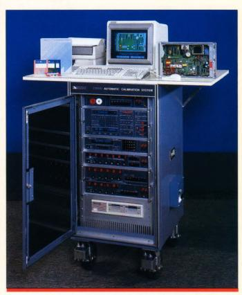
An automatic calibration system from Valhalla Scientific features two Ziatech GPIB interfaces.
