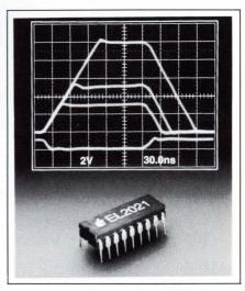
capability, allowing you to put the outputs into a high-impedance state for load monitoring. The slew rate is  $100V/\mu sec \pm 20\%$  with a slew-rate control input of 1V and typically offers a  $300V/\mu sec$  slew rate at higher control levels. To conserve energy, you can shut down
