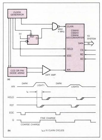
Fig 1—This circuit jams an A/D converter into its coarse-charge mode, so that the converter can better track step changes at its input.
