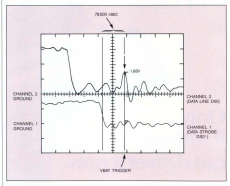
Fig 1-A timing violation is caught in the act by an Ultraview VBAT trigger board and a digital sampling oscilloscope. The spike on the least significant VME Bus data line (upper trace) caused the data line to exceed a TTL logical-zero voltage level while the data strobe, DS0\* (lower trace), was asserted (low).
