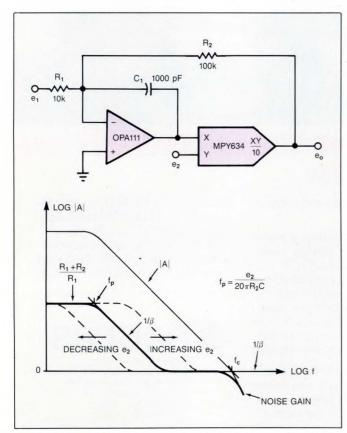
Fig 5—In this filter circuit, variations in the frequency characteristic of  $1/\beta$  make possible a changing  $1/\beta$  slope at the intercept.
