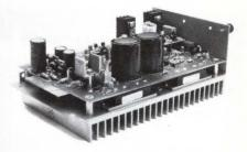
A major manufacturer of digital communication systems required a drop-in replacement AC/DC power unit for an existing multiplexer. The new power system specifications demanded increased reliability, added circuit features, international agency approval, and Bellcore quality compliance.
