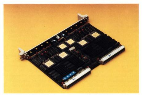
A Transputer-based add-in board for the VME Bus, the VMTM from Paracom runs under the Helios parallel-processor operating system. The board costs \$8375.
