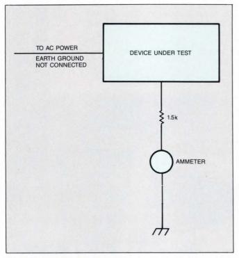
Fig 6—For equipment with no earth-ground return, you must test for leakage to ground. For such ungrounded equipment, the leakage to ground must not exceed 0.5 mA. If your equipment has a line filter, UL specs allow a maximum leakage of 5 mA.
