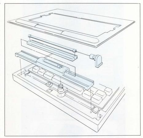
Fig 1—A roller coupled to an optical shaft encoder in the Isopoint provides one control axis, and a sliding cradle coupled to a second encoder through a rack-and-pinion gear train provides the other control axis.
