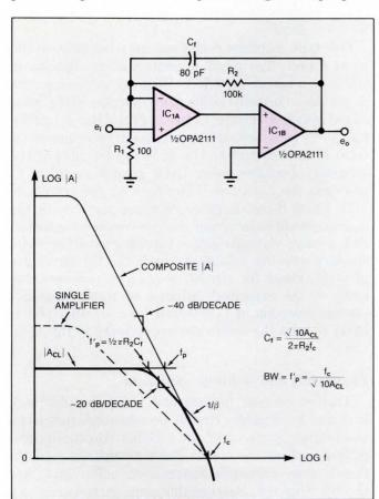
Fig 2—For greater bandwidth in high-gain circuits, you can provide phase compensation for the  $1/\beta$  response to retain a smooth open-loop response for fast settling.
