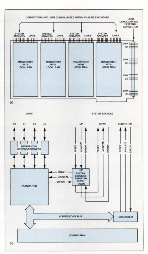
Fig 1—Representative of Transputer-based add-in boards for the PC/XT bus, the Part.6A board from Computer Systems Architects has external connectors for linking Transputers within the chassis and outside it (a). Differential driver/receivers can drive data across a room via link adapters (b). The System Services Repeater Logic enables the host computer to broadcast System Services signals over a Transputer network without signal degradation.
