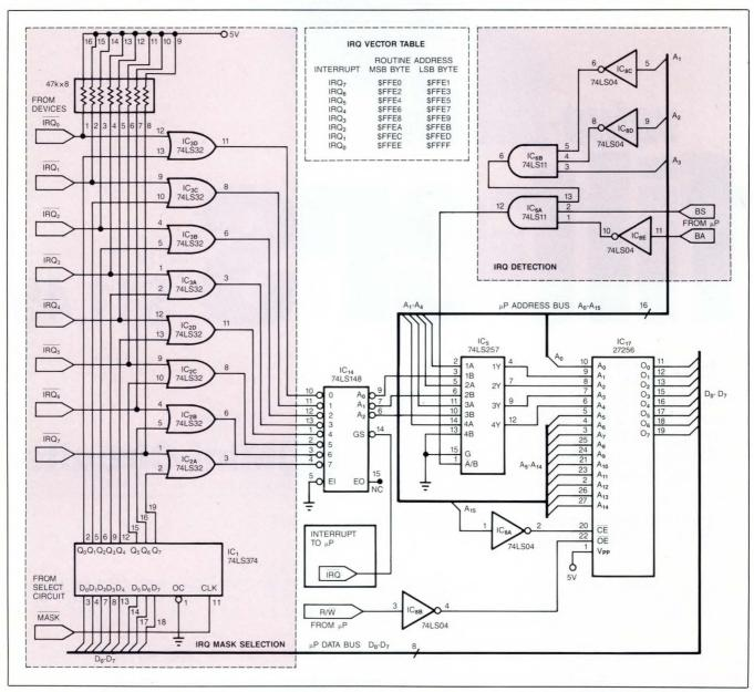
Fig 1—This circuit fools a 6809 into acquiring one of eight different interrupt-vector-routine starting addresses instead of just a single vector by disconnecting three of the  $\mu$ P's EPROM's address lines from the address bus momentarily and connecting them, instead, to the interrupt lines via a priority encoder.
