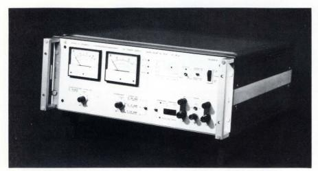
Front-panel-mounted meters that indicate a supply's status are features of many programmable supplies. This unit (from Rohde & Schwarz's NGPU Series) has analog meters, but other units sport digital displays.
