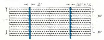
Magna/PAC is mounted between rows or columns of DIP and ZIP IC's and carries up to 5 Amps. On dense multilayer boards, Magna/PAC helps to equalize voltage. In some applications, internal power and ground planes can even be eliminated.
