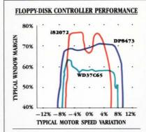
No other integrated data separator analog or digital—can give you a 70 percent window margin at ±8 percent variation in motor speeds.
