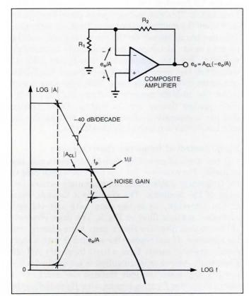
Fig 3—A phase shift of 180° causes oscillation only where the gain-error,  $e_0/A$ , is capable of independently supporting the output signal.
