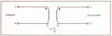
Fig A—In most instances, you can represent a transformer by its turns ratio.
