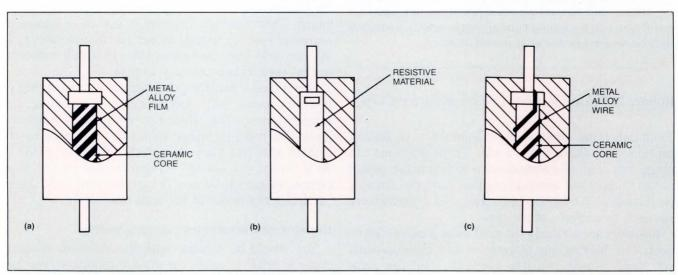
Fig 1—Film resistors (a) are made by cutting a spiral into a layer of metal or carbon deposited on a nonconductive core. Carbon composition types (b) have a solid core of resistive material; wirewound resistors are formed by winding resistive wire on a nonconductive core (c).
