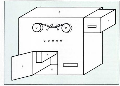
Fig 1—A typical piece of equipment for EDP applications has several protection mechanisms. The enclosure (A) provides basic protection against fire and shock dangers. The housing (B) protects personnel from fire, shock, and mechanical injury. The internal barrier (E) prevents access to hazardous areas inside the equipment. The bottom panel (D) keeps flaming material inside the equipment.
