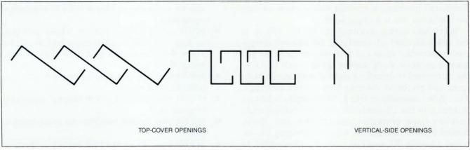
Fig 3—Openings in an enclosure must deflect falling parts. These drawings show cross sections of acceptable types of openings that keep out small metal parts that could otherwise cause short circuits and fires.
