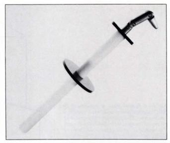
Fig 2—An articulated probe emulates the human finger. You use the probe to test the protective qualities of the openings in an enclosure. The IEC articulated test probe shown (you can also build your own from IEC-published schematics) is available from Compliance Design (Boxborough, MA).
