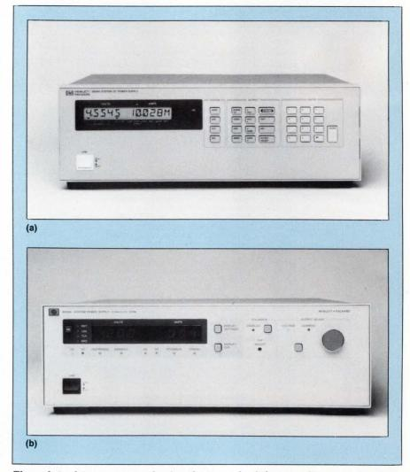
These photos let you compare the size advantage of switchers over linear supplies. Both supplies, from Hewlett-Packard, fit into a 5½-in.-high space in a RETMA rack. Model 6625A/26A (a) is a linear unit with four outputs that total 150W; Model 6030A (b) is a switcher that produces 1200W.
