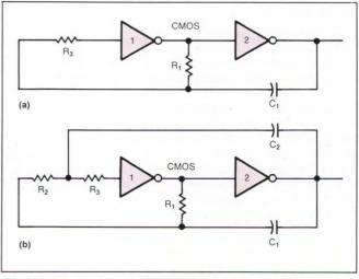
Fig 1—The conventional CMOS oscillator in a sometimes does not oscillate. Or, if it does oscillate, it can oscillate at a lower frequency than you have calculated. The circuit in **b** adds hysteresis to overcome these problems.
