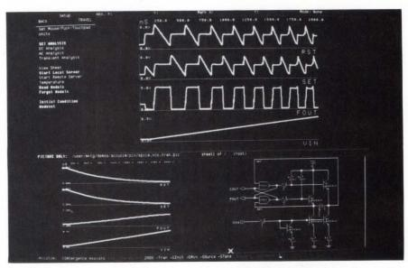
AccuSim's timestep control algorithm (upper right) correctly simulates the voltage-controlled oscillator circuit shown in the lower right. Simulating this circuit on a standard Spice 2G.6 simulator (lower left), the simulator drifts around the circuit's dc bias point without detecting the onset of oscillation.
