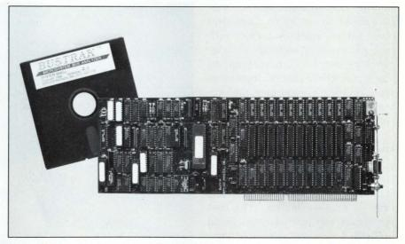
The well-defined environment of the IBM PC allows vendors of bus analyzers for the PC bus to include comprehensive test software with their hardware. (Photo courtesy Applied Physics Inc)
