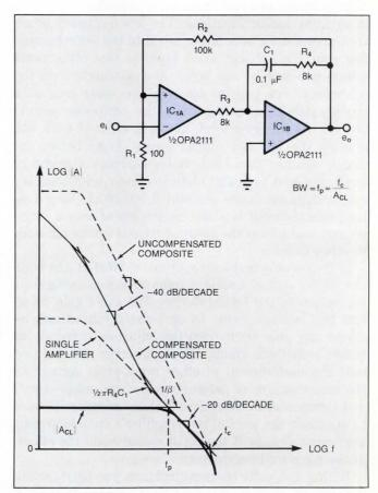
Fig 1—To utilize the boosted gain of the composite amplifier, traditional phase-compensation techniques tailor the gain-magnitude slope to obtain a stable region with a  $1/\beta$  intercept.
