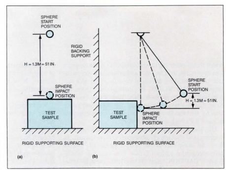
Fig 5—Enclosures must be able to survive contact with falling objects. In these tests for the top (a) and sides (b) of an enclosure, you drop a 2-in. steel sphere from a height of 51 in. The impact must not create openings that would permit the articulated probe of Fig 2 to make contact with live parts.
