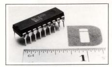
counts for the 8884A's immunity to momentary short-circuit conditions, which occur in gas discharge displays. All outputs consist of switchable and programmable current sinks, which provide constant current to the tube cathodes, even with high-tube anode supply tolerance. You can vary output currents over the 0.2- to 1.2-mA range for multiplex operation; you adjust the output current by connecting an external program resistor from  $V_{\rm CC}$  to the program input. \$3.15 (1000).
